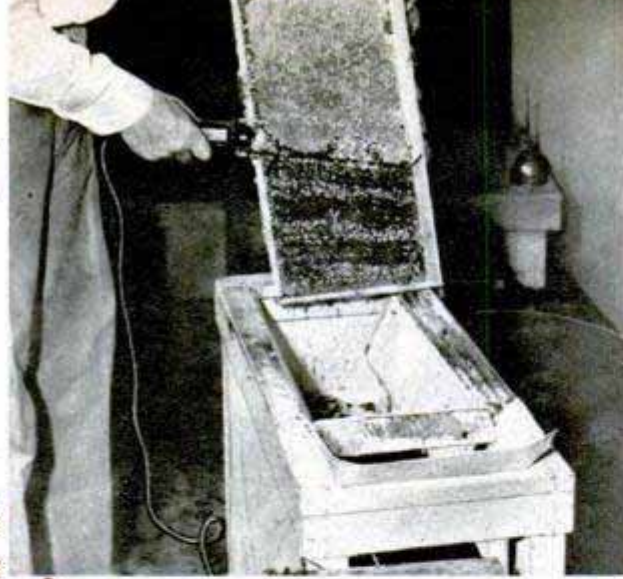
Uncapping knife heated by electricity slices away the wax foundation to expose honey for extraction
