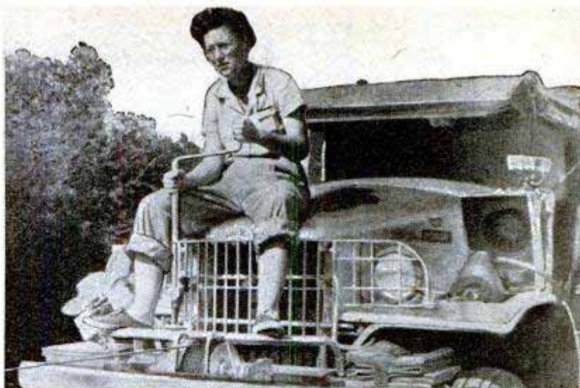
Hand crank can be substituted for the electric winch. The cable will help the "Tramp" across streams or lower Russell down a cliff
