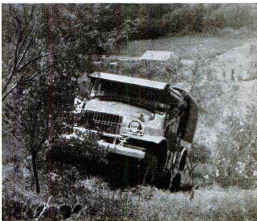
↑ In low-low with all four wheels churning, few grades are too steep
