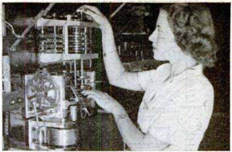
Above, operator adjusts the mechanism of the master crystal clock that sends out radio time signals from Washington
