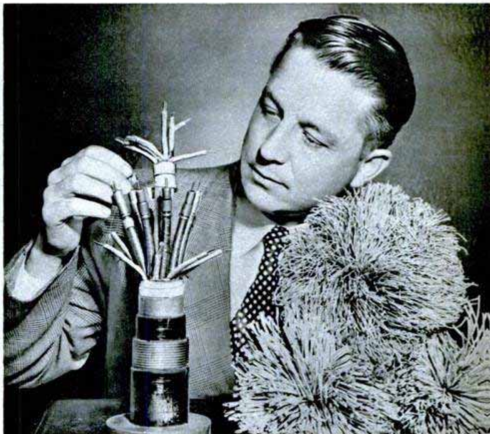
Coaxial cable (stripped at left) can carry more signals than three ordinary cables at far right
