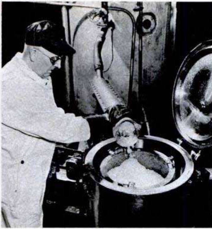
Left, silver-nitrate crystals, basic ingredient of photographic film, are piped into centrifuge basket for quick drying by new process. Right, previously the crystals were formed by slow evaporation in open dishes
