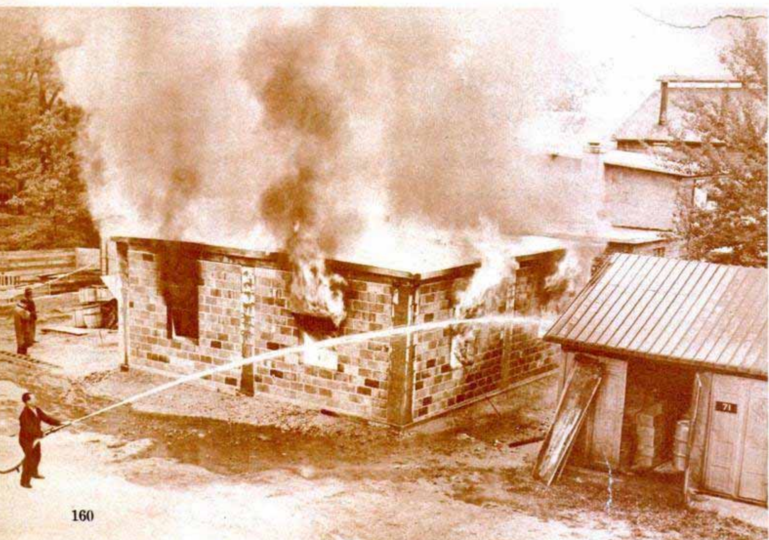
During burning building test below, the instruments above registered 450 temperature readings for various parts of building; temperature went to 2200 F.
