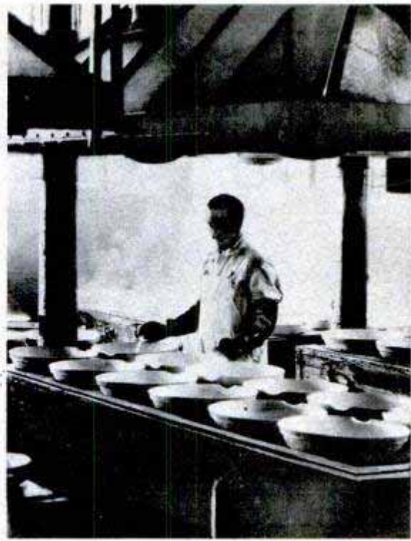
Left, silver-nitrate crystals, basic ingredient of photographic film, are piped into centrifuge basket for quick drying by new process. Right, previously the crystals were formed by slow evaporation in open dishes
