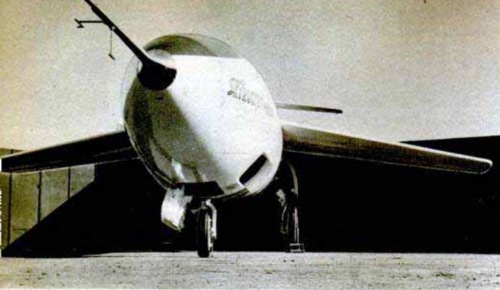
Instruments on nose are to measure plane's yaw and pitch characteristics. The "gill" at right is one of two air intakes for the powerful jet unit
