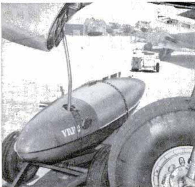
AUXILIARY GAS TANKS , mounted on old bomb trailers, are used as drain tanks in changing airplane-engine oil. A flexible tubing carries the old oil from the engine drain cock into the 150-gallon portable tank
