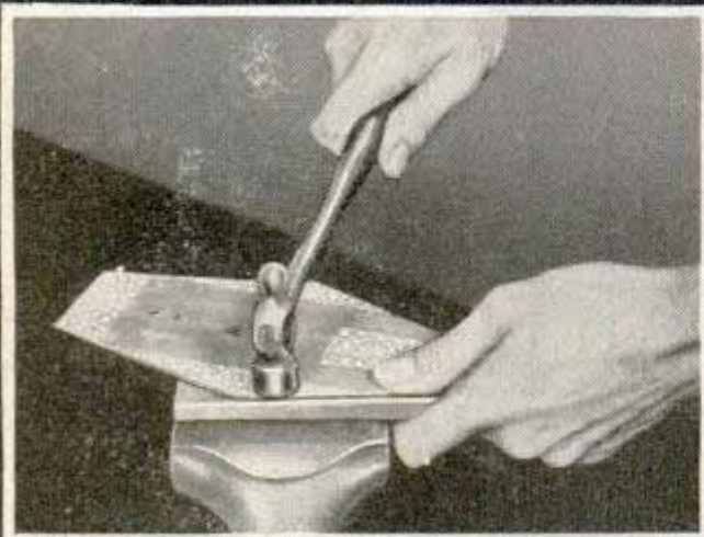
After hammer-finishing the areas indicated in the drawing, the entire edge of the plate is chamfered by tapping lightly with the flat face of a hammer
