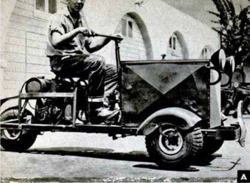
With its large package compartment above the front wheels, this scooter is popular with delivery boys
