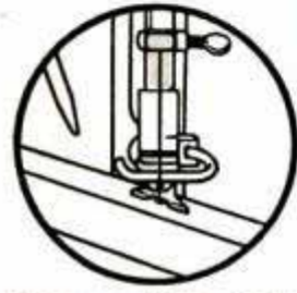
Because spring hold-down tilts with table to hold work firmly, you enjoy smooth operation always.
