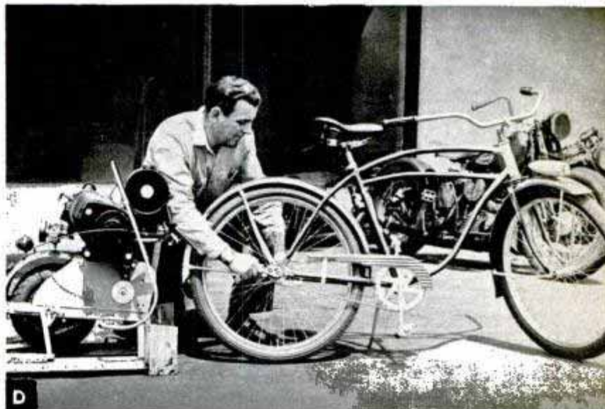
Above, rear wheel is replaced by the power unit at left to motorize the bicycle. Below, lightweight vehicle gets up to 125 miles on a gallon of gasoline
