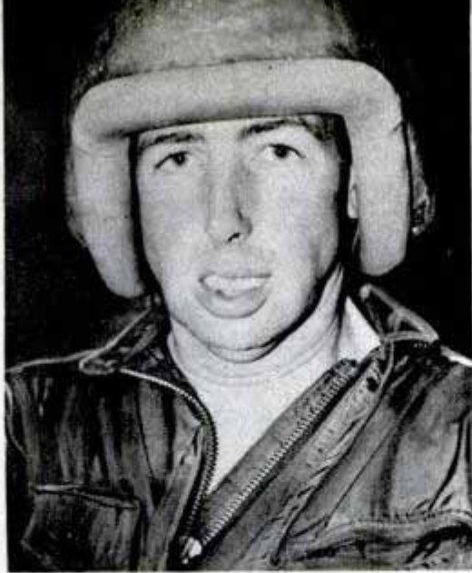
What 6 Gs (six times the force of gravity) does to the pilot. Automatic camera records, right, how his lips and facial muscles are pulled down by the force. Tests were made in giant centrifuge at the University of Southern California
