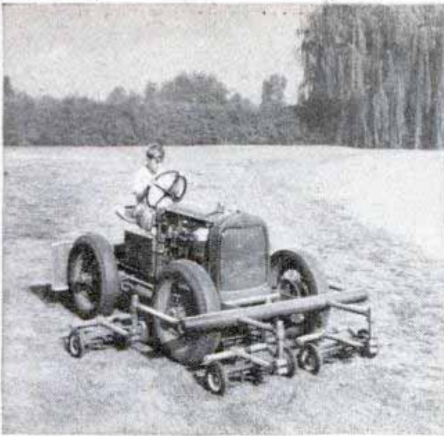
HOMEMADE MOWER uses a specially designed tractor to push five ordinary lawn mowers mounted so they cut an eight-foot swath. Mowing unit is easily removed
