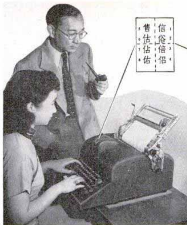
Left, typewriter uses system of combinations. Typist presses keys representing basic parts of word, then selects desired symbol from eight combinations appearing on indicator screen on top of machine (see insert). Right, white rollers flash combinations on screen. The 36 long printing bars in rear contain 8000 symbols
