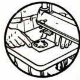
V-jaws of universal chuck hold files with 1/8" or 1/4" shanks.
