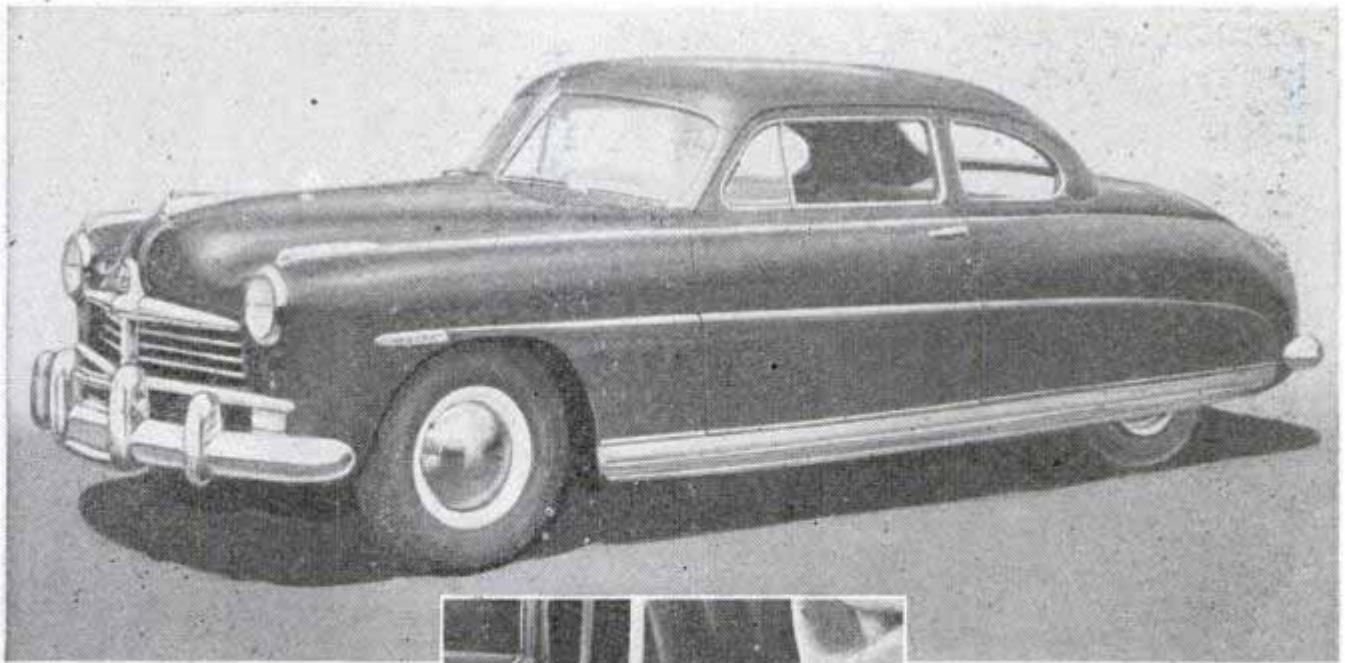
The 1948 Hudson is just five feet from ground to top of car. Passenger (left) steps down into car. Low floor gives extra headroom
