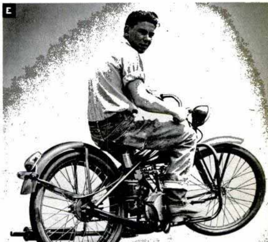
Above, rear wheel is replaced by the power unit at left to motorize the bicycle. Below, lightweight vehicle gets up to 125 miles on a gallon of gasoline
