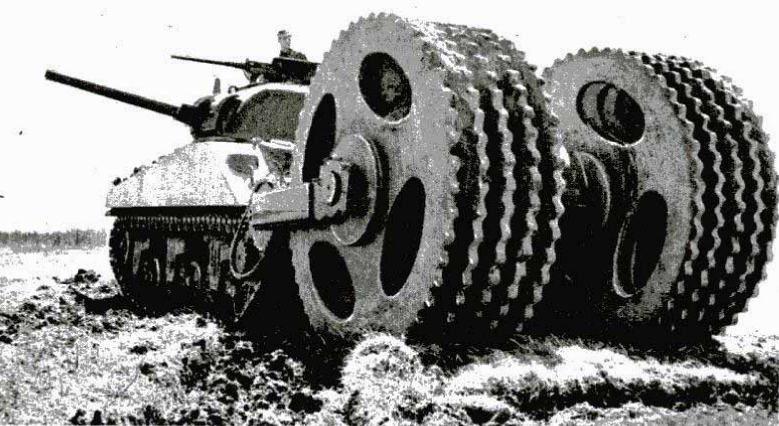
Mine exploder pushed by tank clears path 33 \frac{3}{4} inches wide before each disk section. Disks weigh 4600 lbs.
