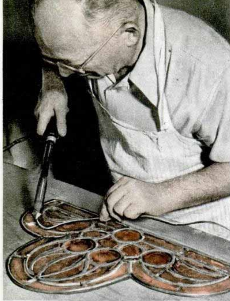
Came-lead strips are soldered to insure permanence. Below, the artist cleans a $10,000 window before re-painting part of the design. Window is 50 years old
