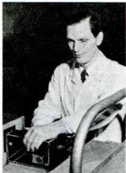
Movie camera is bolted to the X-ray machine prior to photographing bone movement in hand and wrist. Vertical strip shows completed pictures. Right, doctors adjust camera for filming heart's pumping action
