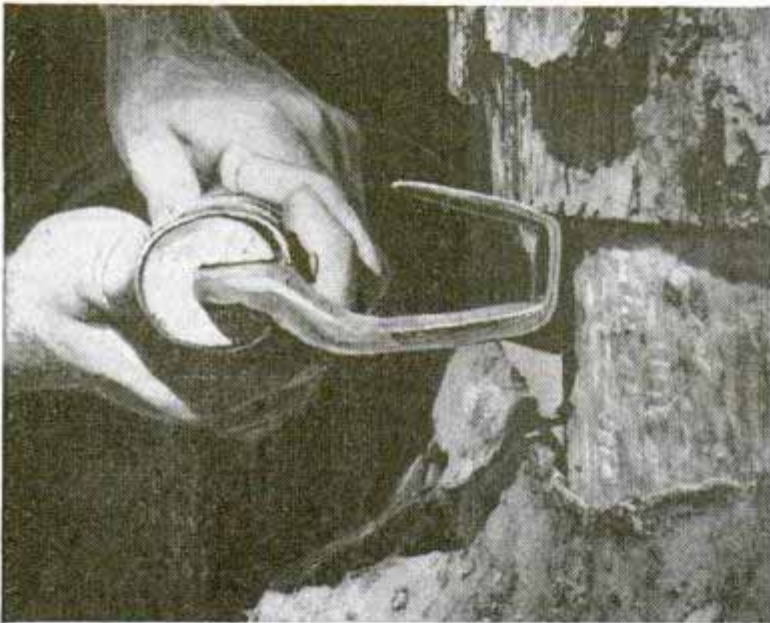
New bark-chipping hack was devised by Keith Dorman at the Olustee Experimental Forest in Baker County, Fla. Below, glass cup shaped like flowerpot catches oleoresin, or gum, from tree
