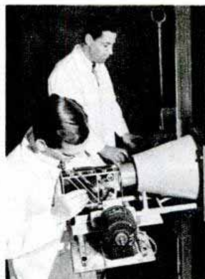
Movie camera is bolted to the X-ray machine prior to photographing bone movement in hand and wrist. Vertical strip shows completed pictures. Right, doctors adjust camera for filming heart's pumping action
