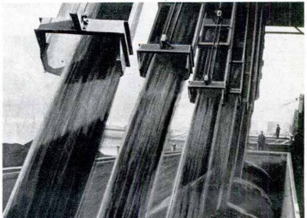
Above, enclosed in elevated passageway at the right, the conveyor belt pours coal into this 2000-ton tipple. A complex conveyor system inside the tipple carries the coal to the seven barge-loading chutes. Below, loading chutes fill barge with 900 tons of coal in about five minutes
