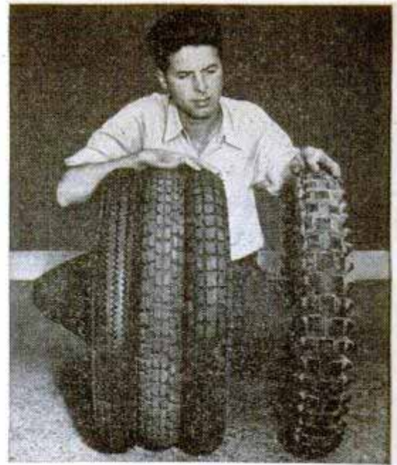
Left, ready and "raring to go," rider awaits start of endurance race. The motorcycle tires above are for use on pavement (left), pavement and dirt (two in center), hills and endurance contests (knobby tire at right)
