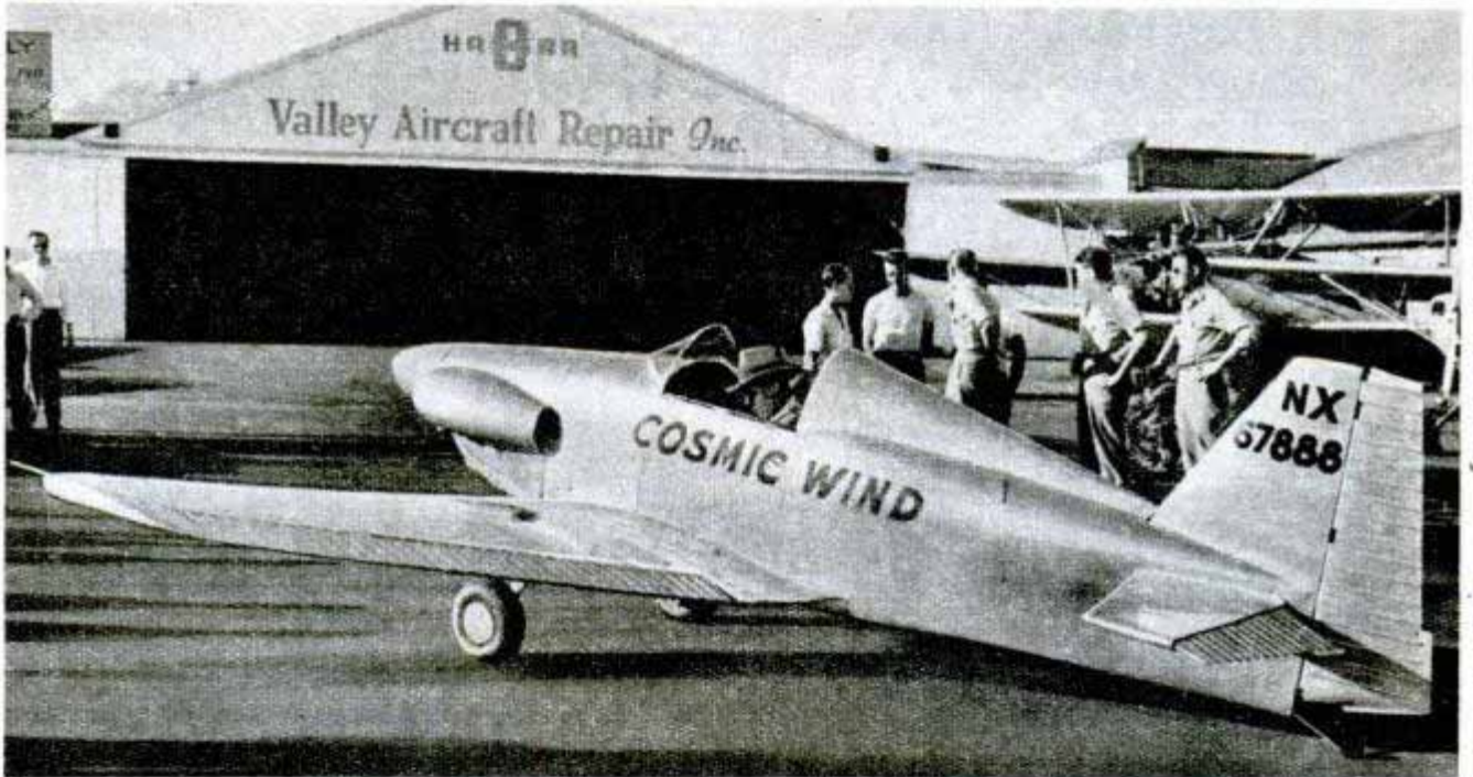
Nineteen-foot wing span of midget racer supports seven men and a child. Built by Tony Levier, Lockheed test pilot, it has a top speed of 200 miles an hour. With pilot and three hours' fuel, the craft weighs 800 pounds
