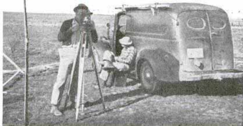
Surveyor on western prairie is reading off angles to his assistant who records and computes them as fast as he can to prevent any expansion of metal or settling of tripod from affecting accuracy
