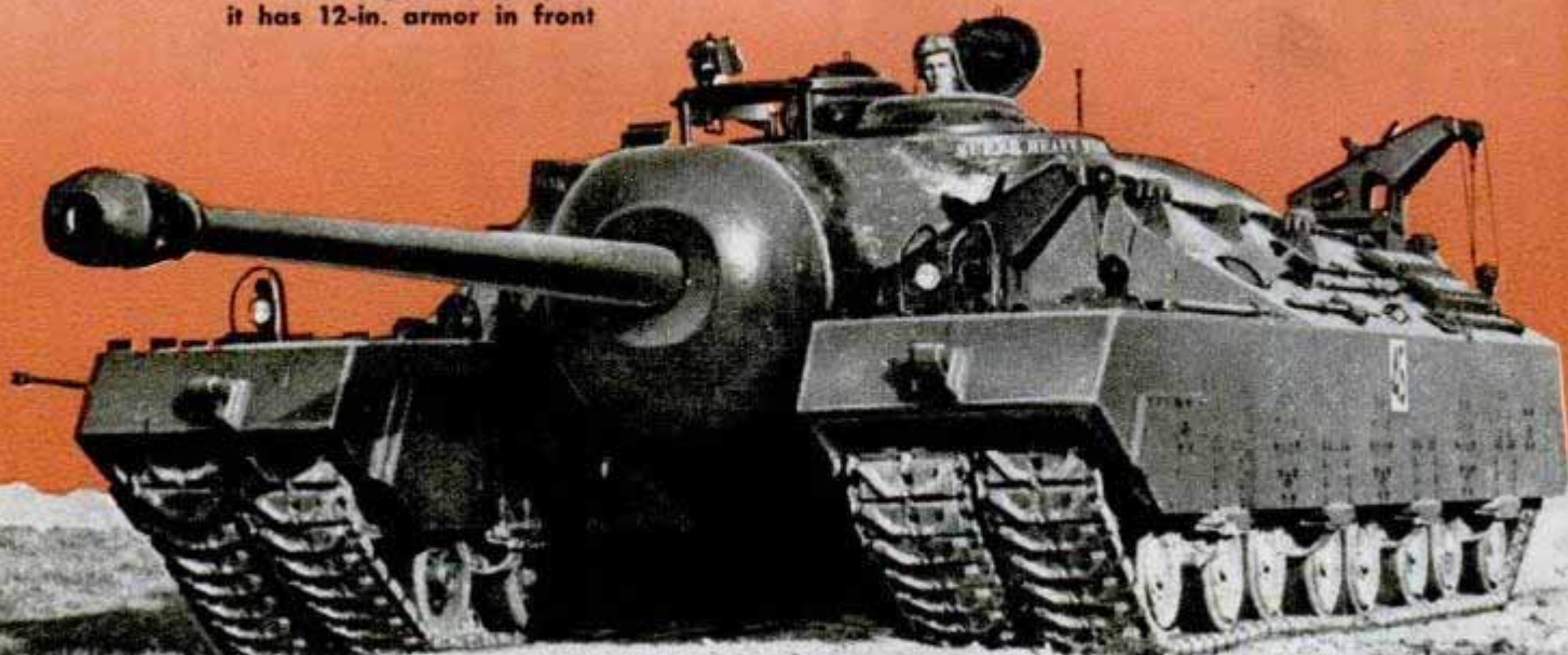
Below, new superheavy tank weighs 95 tons and mounts 105-mm. high-velocity gun; it has 12-in. armor in front
