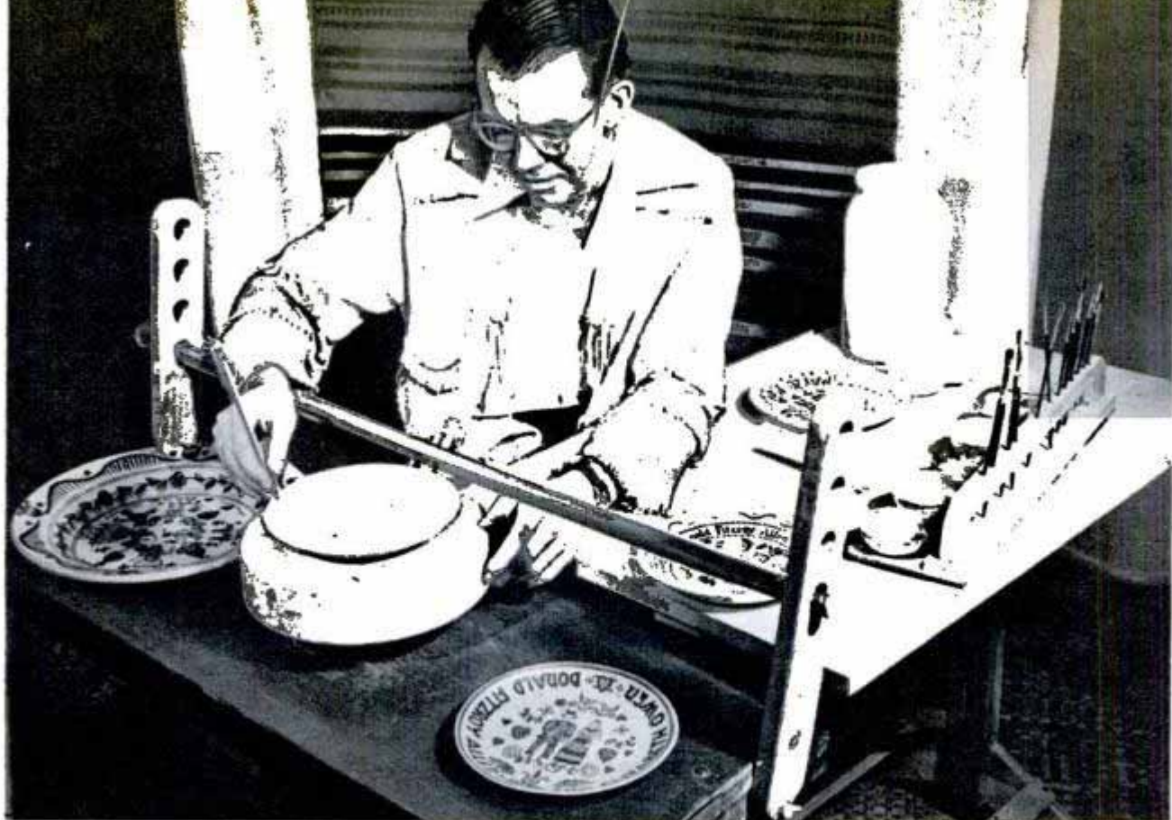
Designs depicting the romance are sketched on the plates in pencil. They are completed with metallic pigments
