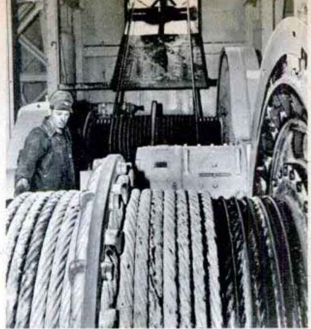
View inside the dragline shows drag drum in the foreground and hoist drum in background with motor between them. Machine has 2000 feet of steel rope
