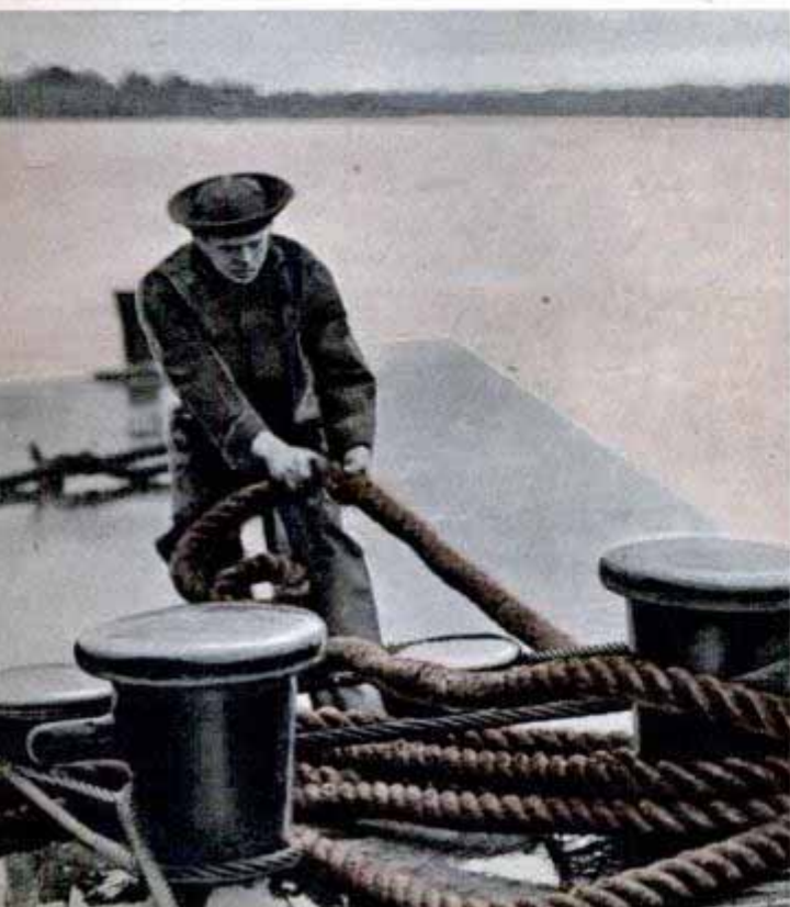
↓ Deck hand makes fast a heavy line around a barge's timberhead in preparation for a threatening windstorm. Right, the leadsman's "Mark Twain" signifies safe water and echoes the romance of early river-packet days
