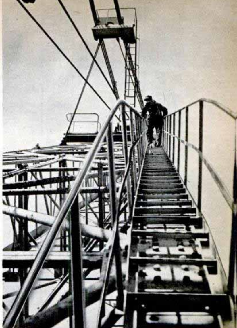
Looking up walkway of the boom which enables the oiler to inspect parts and oil them. Below, operator has two foot pedals and two hand-operated controls
