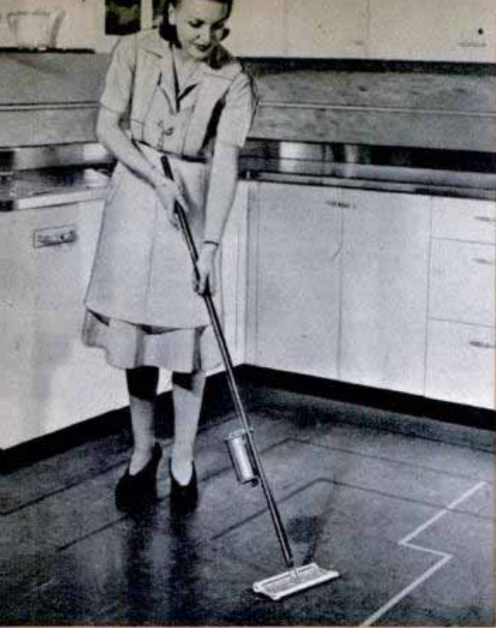
FLOOR WAXER automatically applies liquid wax as the operator pulls a trigger attached to the handle. The liquid flows from a container to a plush applicator
