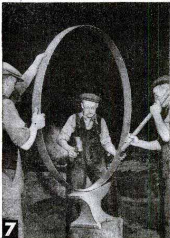
When spoke is "driven home," Sibley uses a straightedge to check alignment of each spoke With tire ends riveted together and made red-hot in fire, welding is completed on the anvil
