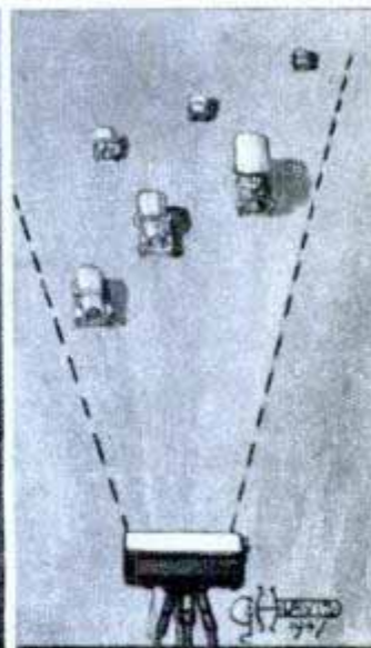
Instantaneous stereoscopic pictures are taken by this unusual camera equipped with 26 prisms instead of a conventional lens. Action of moving vehicles is stopped by camera
