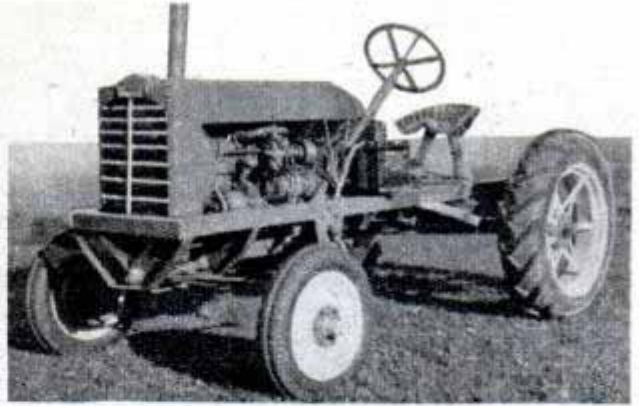
Snowplow attached to homemade tractor saves builder many backaches. With two transmissions, it has 13 speeds forward
