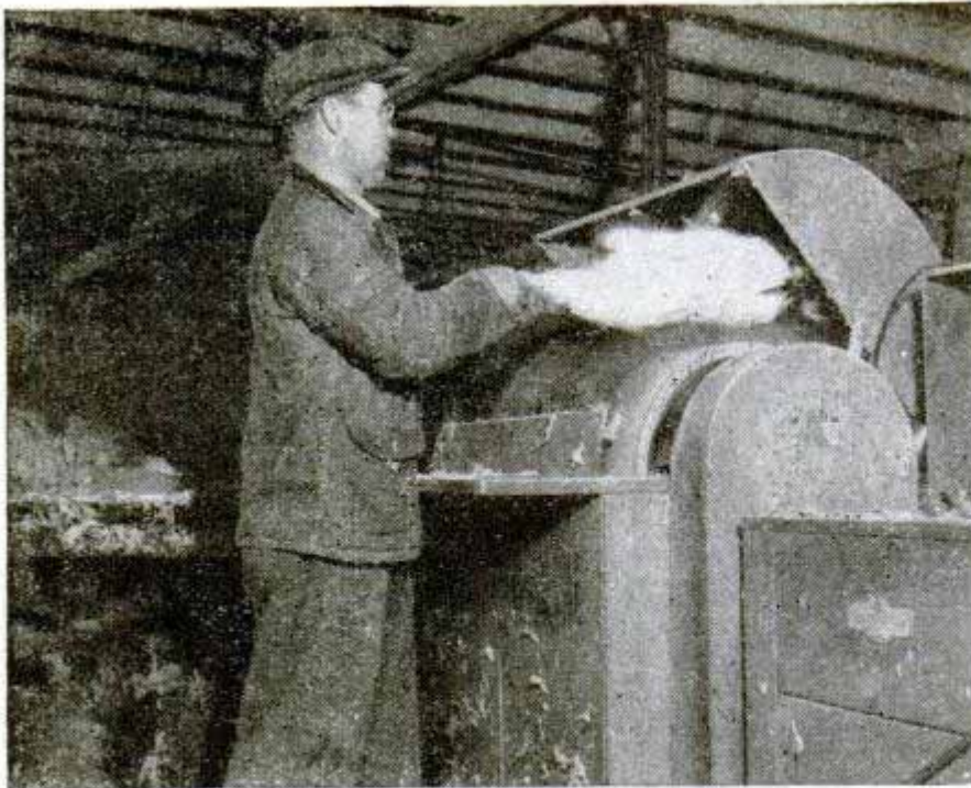
Metal spokes on a revolving wheel of mechanical plucker remove feathers
