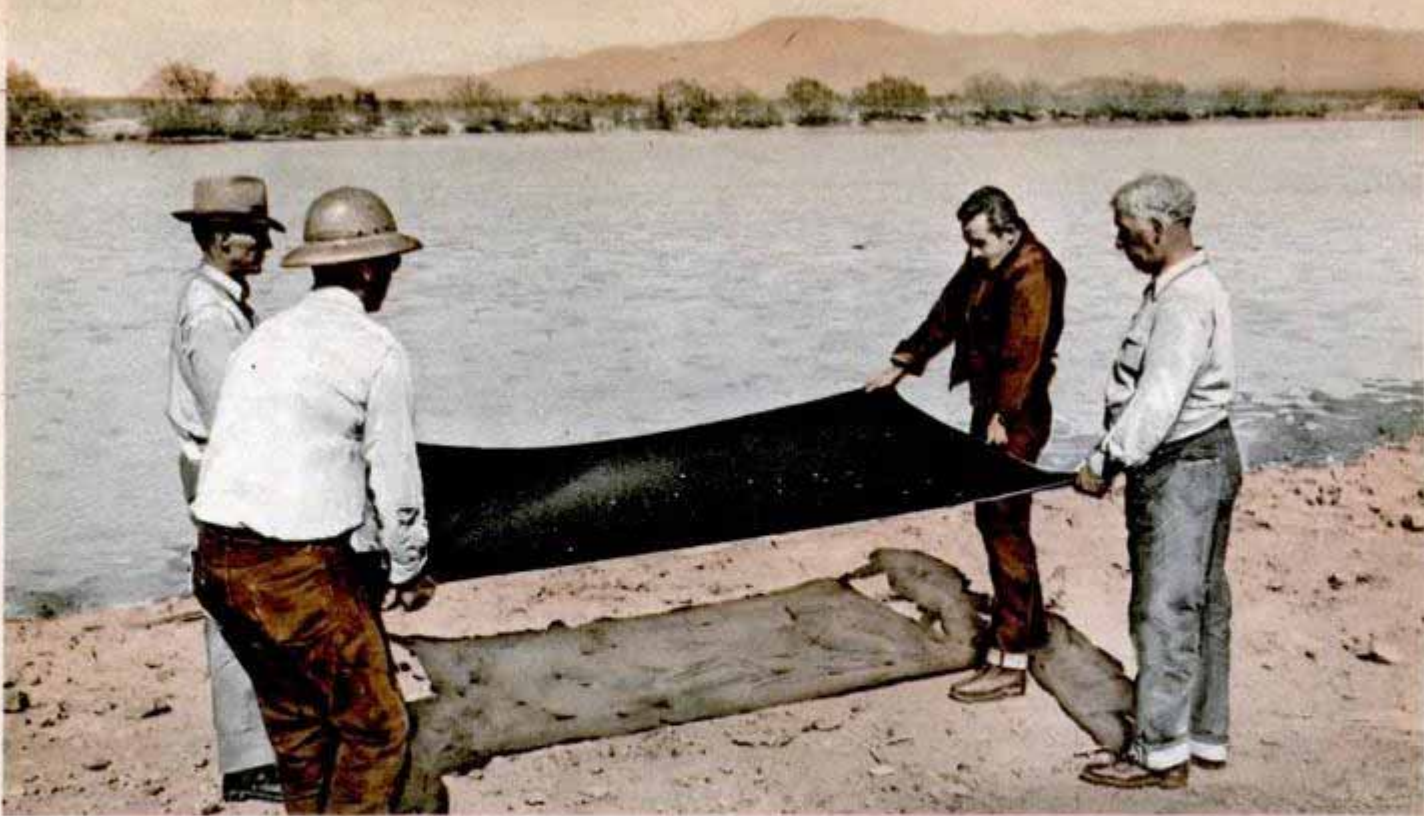
Blanket catches grass-seed pellets dropped from plane to check ability to plant one pellet for every square foot
