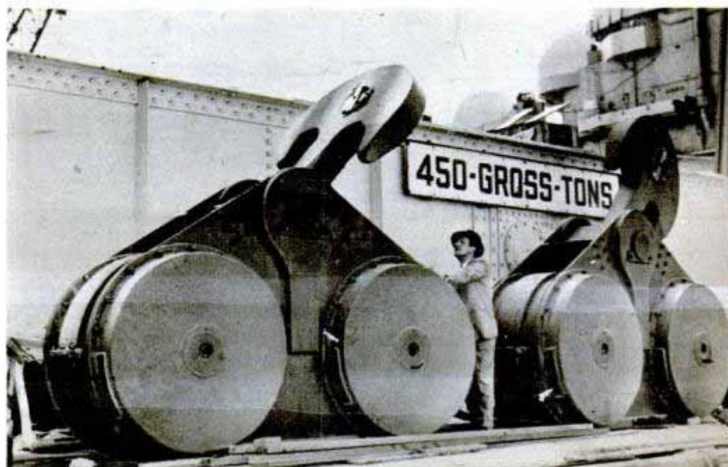
At left is the biggest hook of all, a 5-ton casting that will hang from the equalizer beam when weights near 400 tons are being handled. Right, 245-ton capacity hooks that will be suspended from each of the cranes
