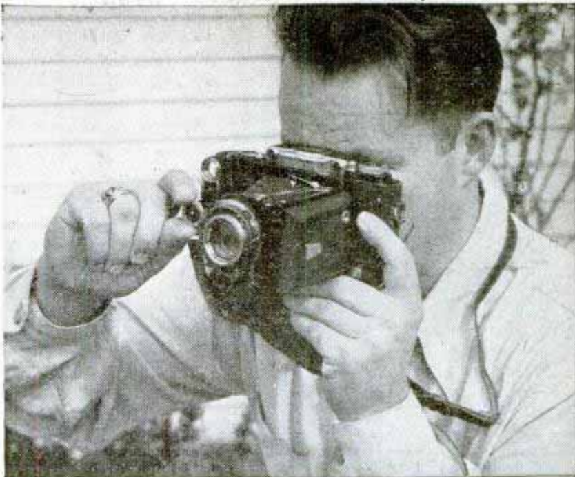
Reflex-type cameras (above) employ a ground glass for focusing, while cameras with coupled range finders are focused by super-imposing split image
