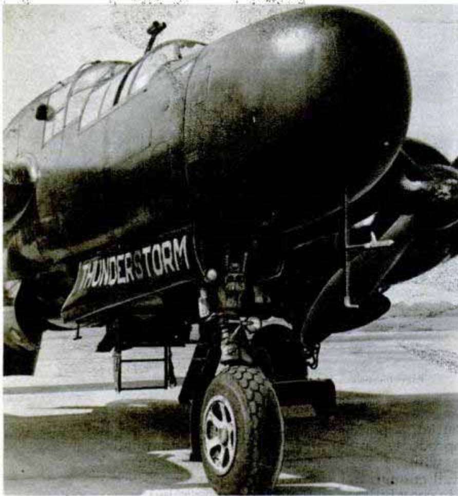
Another view of an instrumented P-61 in which AAF pilots and radar observers battle through thunderstorms to learn more about rocky weather to make flying safer. Below, analytical chart of a plane's flight through a storm
