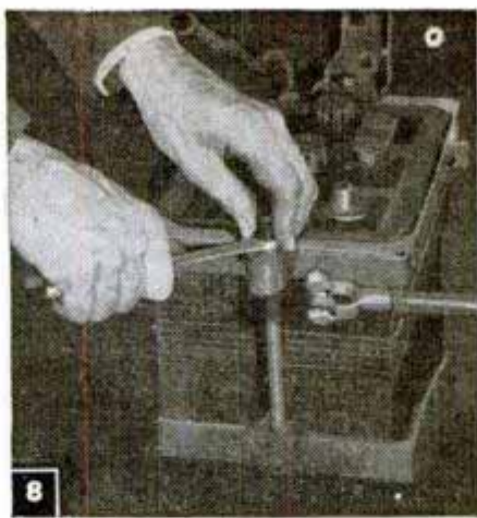
8 When replacing battery, tighten bolts uniformly. Renew rubber washers. Don't draw nuts too tightly
