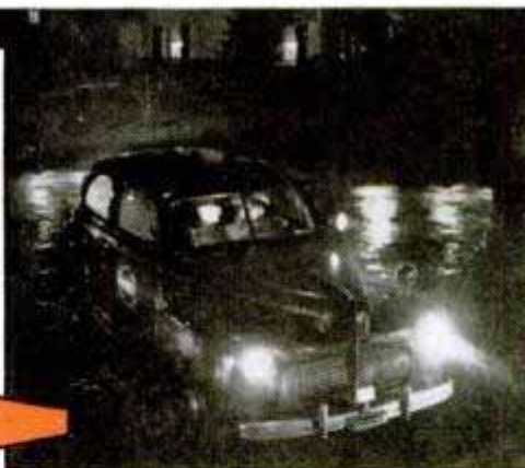
STOP-AND-CREEP DRIVING —Police cars, hearses, door-to-door delivery vehicles, etc. that have long periods of idling usually require a hot plug to prevent fouling.
