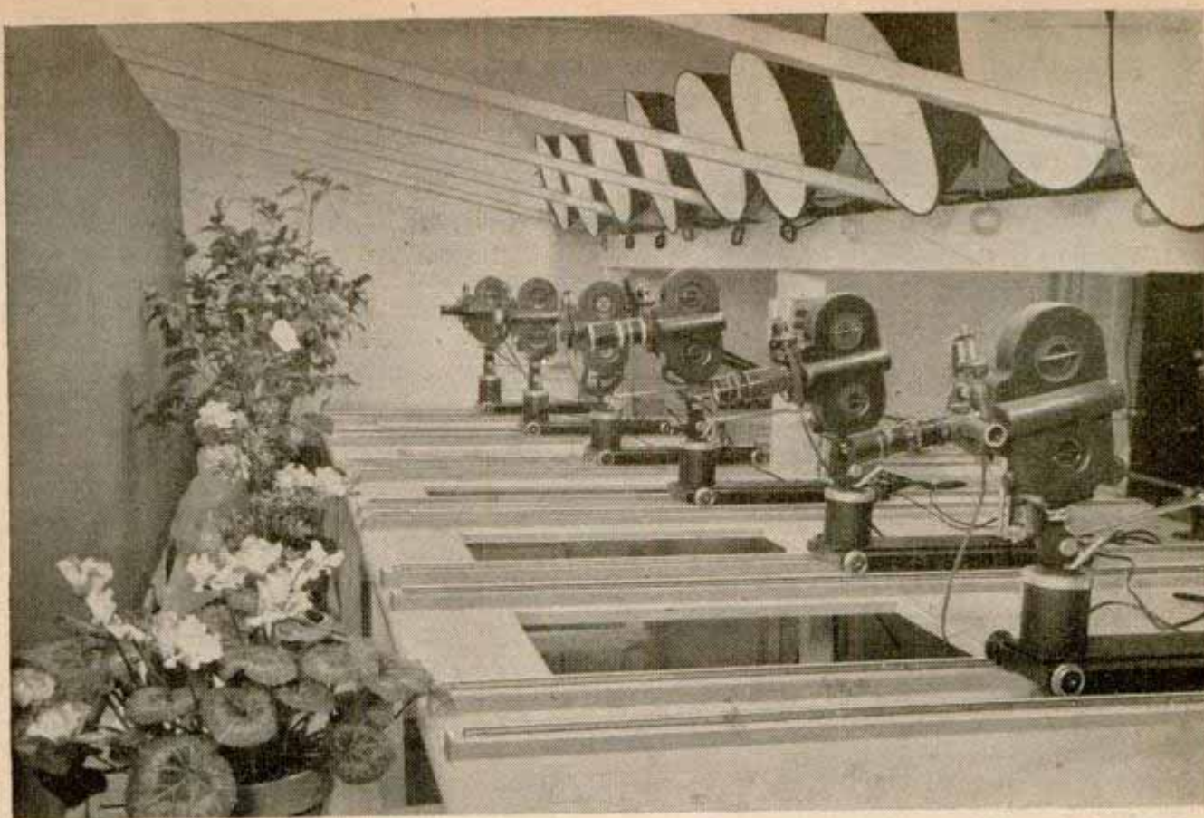
Six robot-operated cameras are lined up on six different subjects. Note variations in lens elevations
