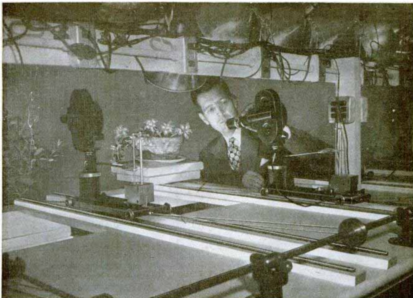
After Ott makes a final adjustment on the lens, the robots will expose a 16-mm. frame every five minutes
