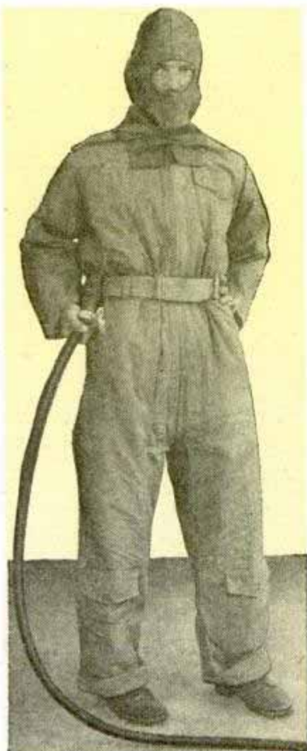
Pressured air entering "tail" of cooling suit at left, finally billowing out at the face and pants legs, forms protective layer over body for work at 165 above. Right, fur-lined cold-weather garb with face protector
