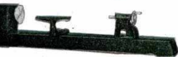
Master Model 31-Inch Lathe—with 10-inch swing, rigidly built with 4-step-pulley for wide range of speeds.
