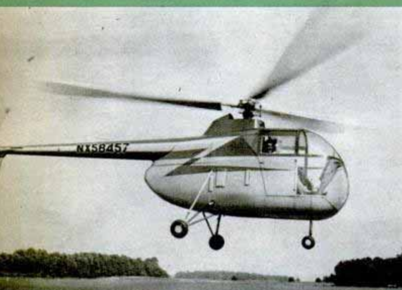
Firestone's two-seater can climb 1250 feet a minute and travel over 220 miles on 25 gallons of gasoline. This model has a 175-horsepower air-cooled engine
