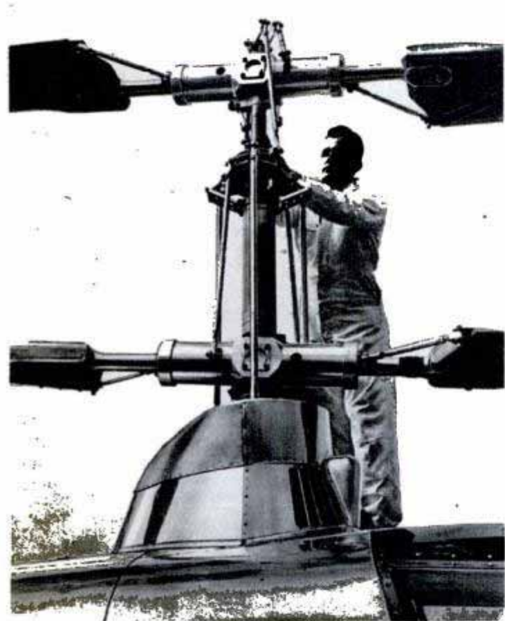
Helicopters at left and in the center counteract torque with a tail rotor and a tail jet, while coaxial type at right uses two overhead rotors for that purpose. Below left, checking mechanisms that change rotor blades' angle of attack. Right, with rotors and aluminum skin removed, helicopter is a maze of controls
