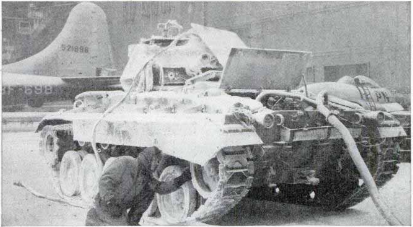
Mechanic examining effects of extreme cold on idler wheel of M-24 tank. Below, a P-47, mobile observation room and a Superfort occupy a small part of the huge hangar's 200 by 250 feet
