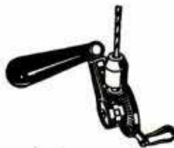
Turret locks chuck in seven different positions
