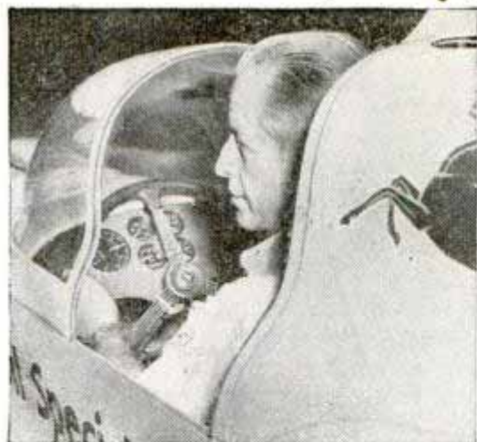
Gauges in Jenkins' car show oil temperatures at such crucial points as the connecting-rod bearings and gear box
