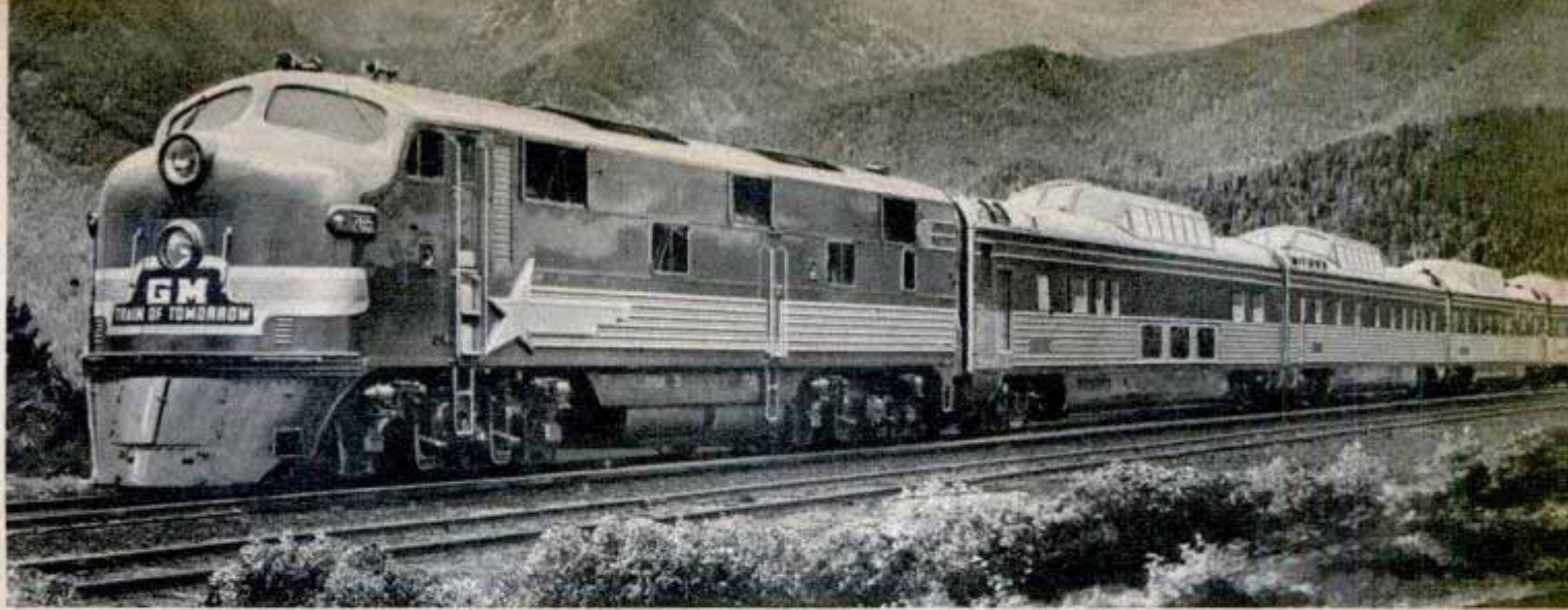
Four-car experimental train, pulled by a Diesel, has a glass-enclosed top deck on each car for all-around view
