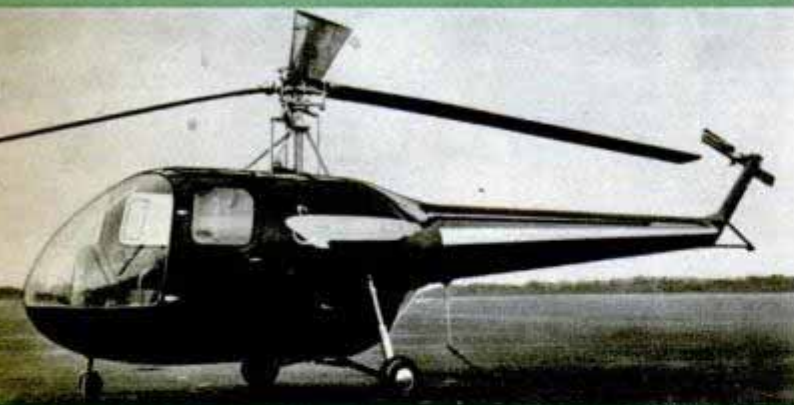
An old name in the rotary-wing-aircraft field, this Sikorsky carries loads up to 650 pounds. It weighs 1100 pounds empty. Below, a Bell model using pontoons. Many of these are used for rescue and patrol
