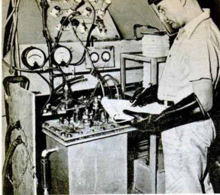
Recently developed electrolytic cell finally makes possible the separation of pure elemental fluorine
