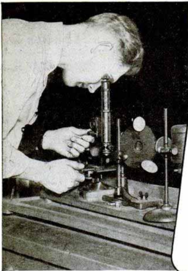
1200 magnifications reveal the structure of annealed forgings. Under the microscope, the laboratory technician can determine if the sample meets specifications.
