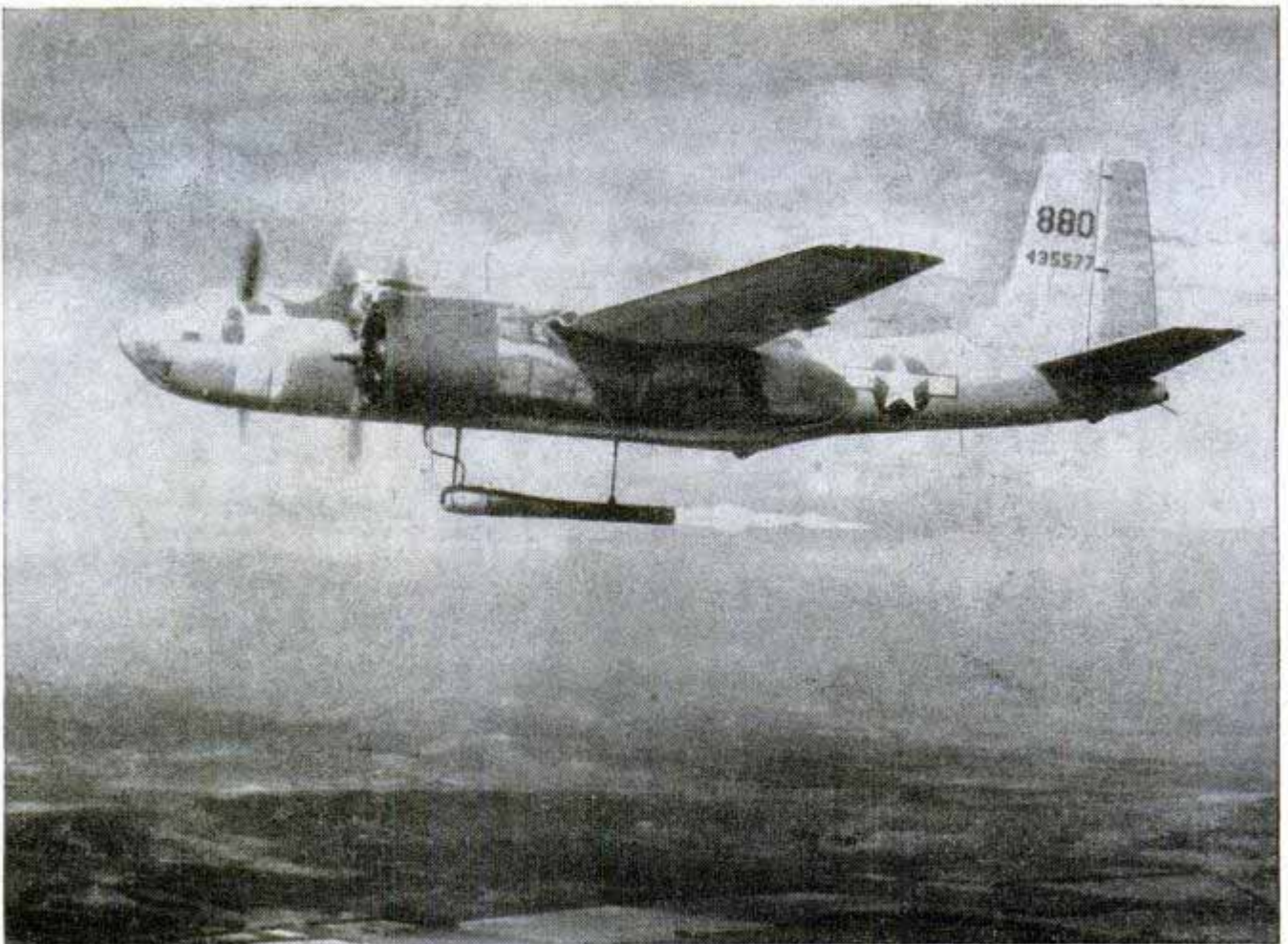
Gauges inside plane record results of flight test under power by nine-inch pulse jet engine below the fuselage
