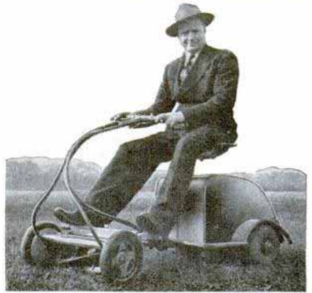
Top left, snow sweeper with brushes cleans sidewalks. Top, "scooter" pulls creeping-bent mower. Above, the front wheel can be replaced with a manual lawn mower for a quick job on ordinary grass
