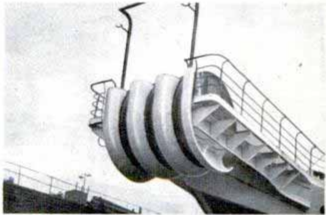
Tension on the grapnel rope is determined by the dynamometer to show when grapnel strikes cable. Below, all grapnel ropes are run through the bow sheaves
