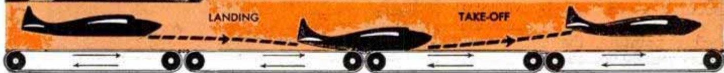
For ease of maintenance and repair, the speeding belts would be in sections. The surface would always be free of snow and ice in bad weather
