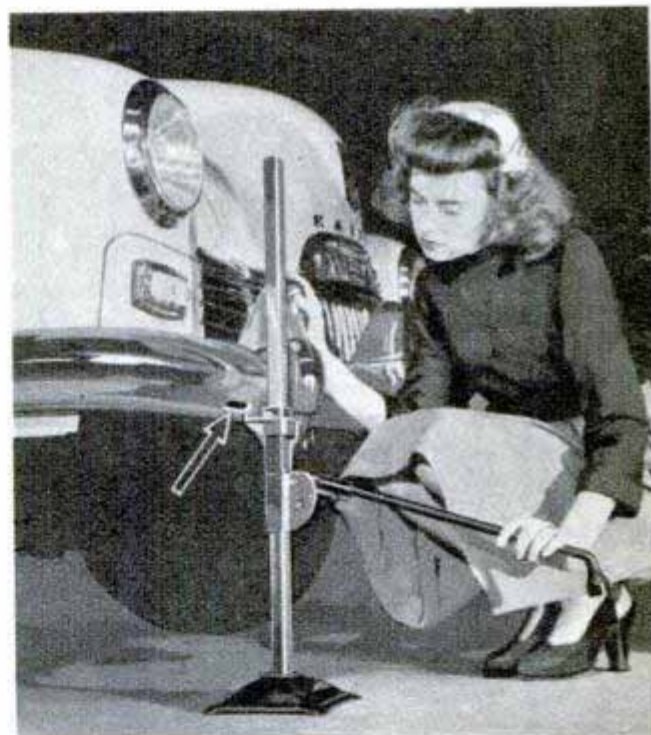
NAIL DETECTOR locates any metal object inside a tire casing that might work in and cause a puncture. A floating permanent magnet signals the presence of metal in the casing, yet its range is so limited it is not affected by metal rim or any wire reinforcement. A six-volt lamp provides signal flash
