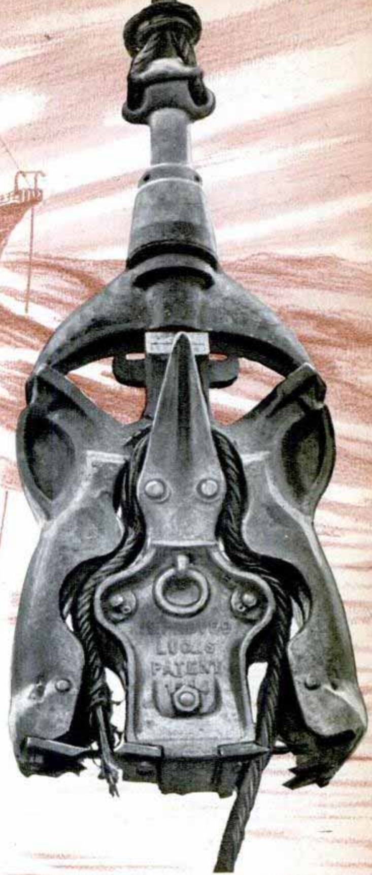
Lucas grapnel, used in deep water, cuts the cable in two. When the grapnel strikes the strand, huge jaws automatically bite the cable and hold one of the free ends so it can be lifted to the surface
