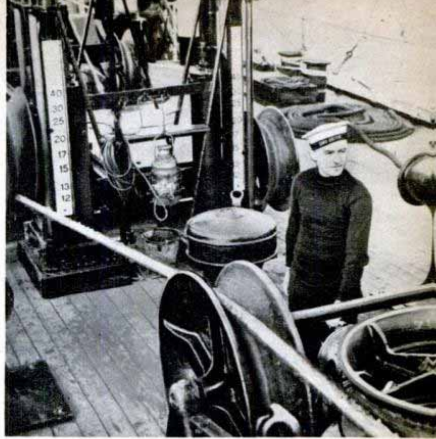
Tension on the grapnel rope is determined by the dynamometer to show when grapnel strikes cable. Below, all grapnel ropes are run through the bow sheaves
