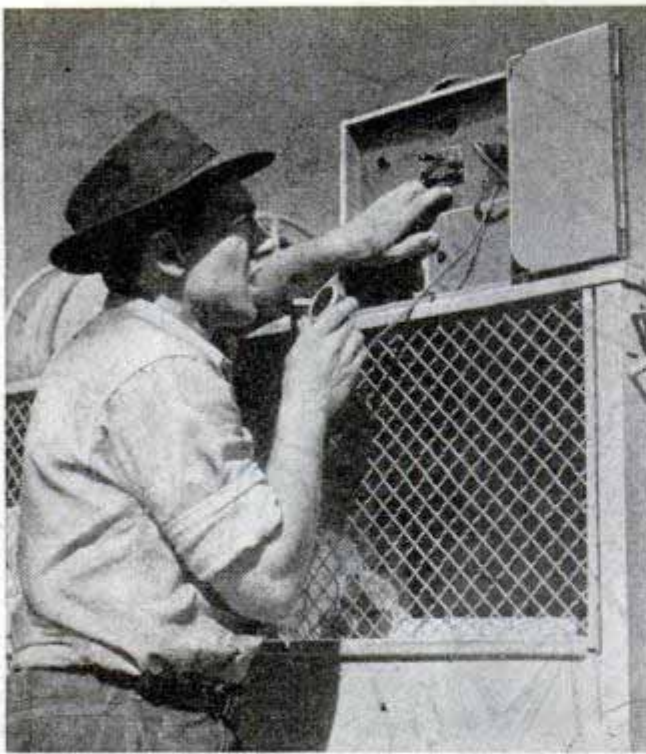
Crewman reports progress of a battle against flames over a shortwave radio mounted on a high-speed truck. Right, more than 170 miles of telephone wire thread the forest and patrolmen can tap in anywhere for reports
