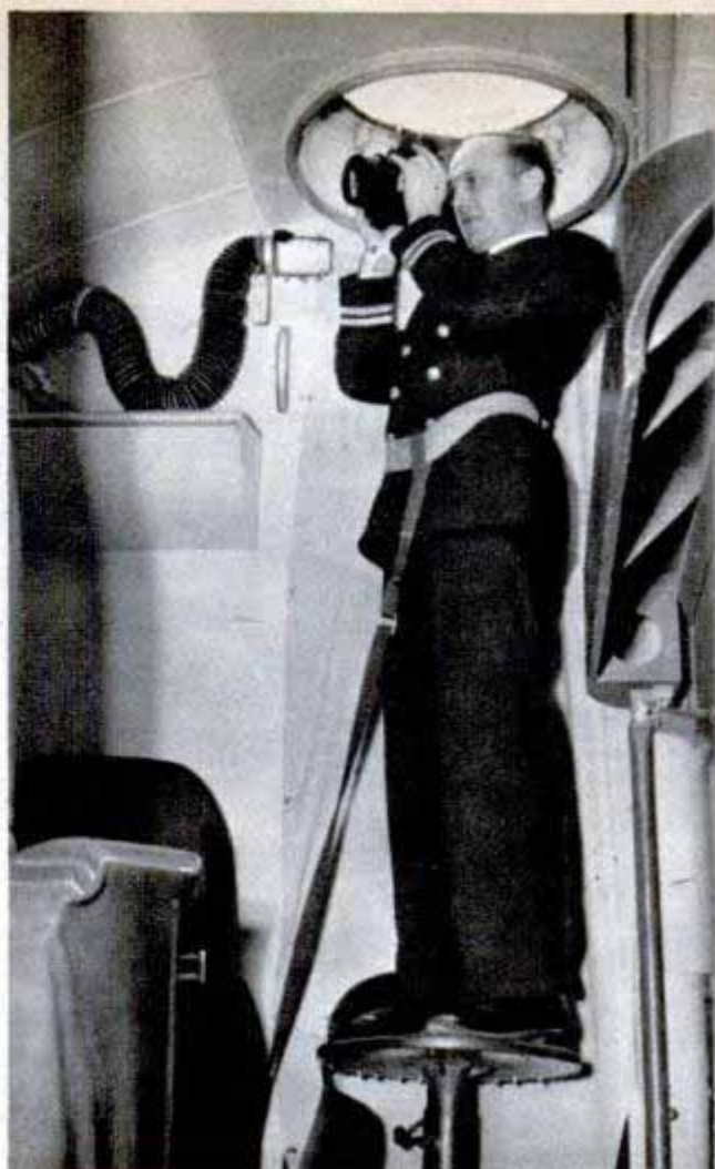
HELD BY a safety harness, a navigator takes a "fix" over the mid-Atlantic. The belt was rigged up after a pressurized transoceanic air liner blew its astrodome
