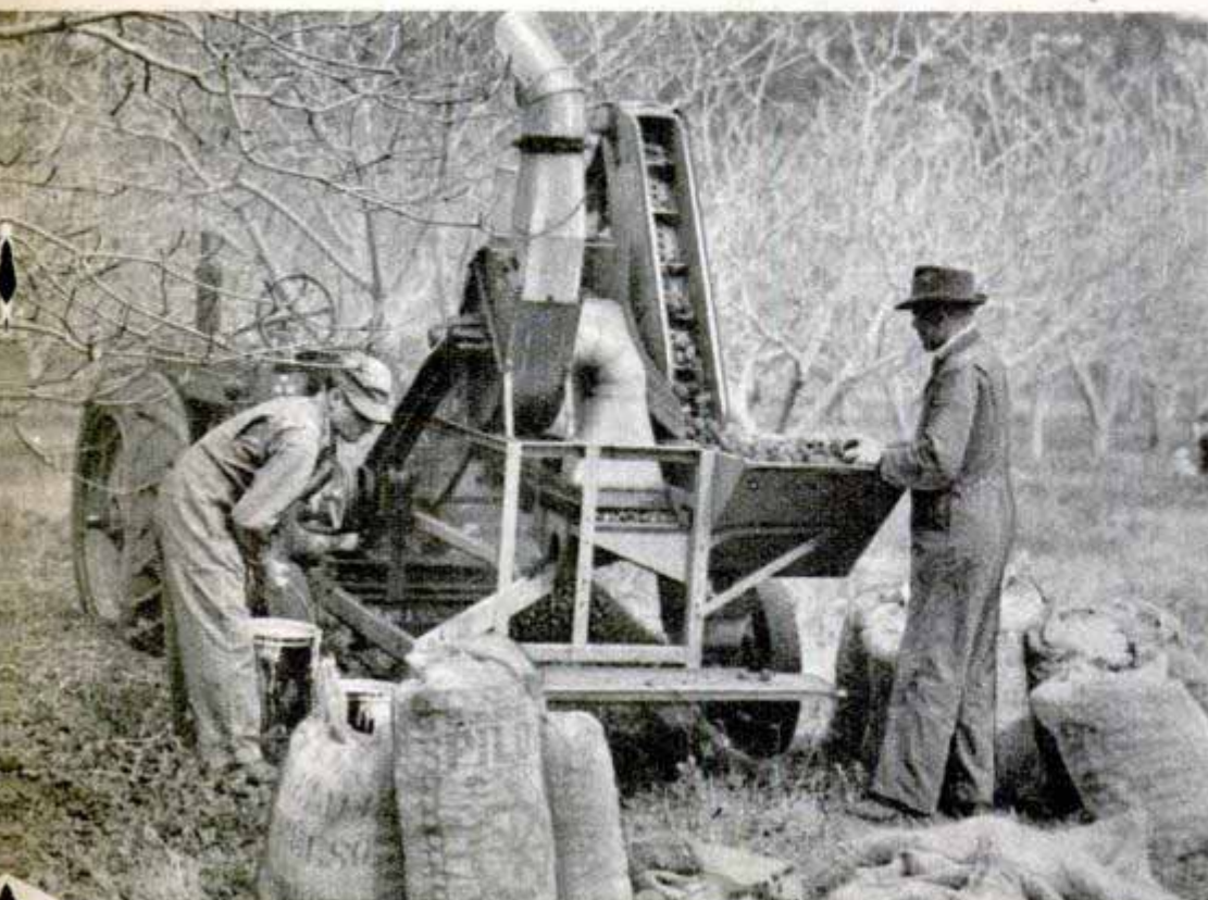
Portable tung nut huller operated in orchard saves trucking to distant hulling plant. This machine is a laboratory "baby"
