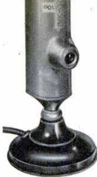
NAIL DETECTOR locates any metal object inside a tire casing that might work in and cause a puncture. A floating permanent magnet signals the presence of metal in the casing, yet its range is so limited it is not affected by metal rim or any wire reinforcement. A six-volt lamp provides signal flash
