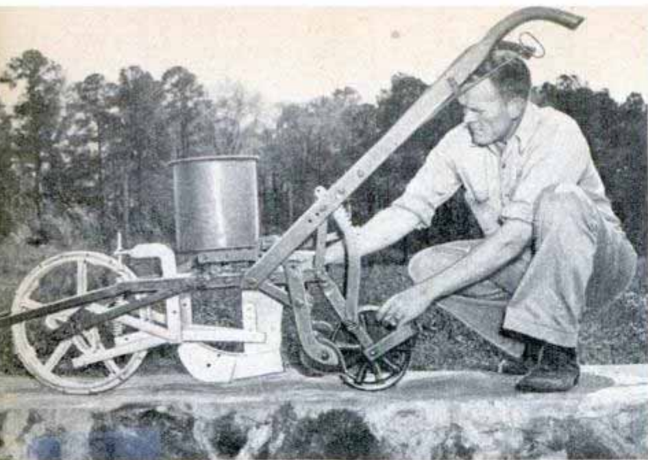
Experimental variable depth cotton seed planter assures good stand in a wet or dry season; planting depth varies 1½ inches
