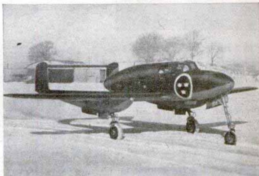
SWEDEN'S FIRST JET fighter plane, the J-21-R, has reached speeds in excess of 500 miles an hour at the air force base at Norrkoping. The plane is similar in appearance to the British De Havilland Vampire
