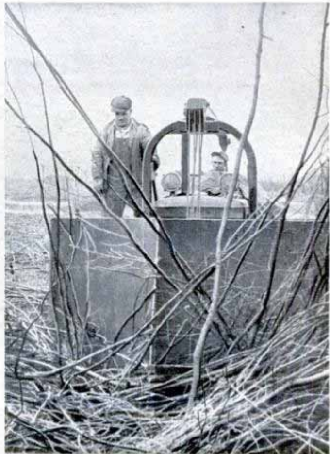
TREE "MOWER" operates like a snowplow to cut 14-foot willow saplings off river land. With the machine one man can clear 20 acres of overgrown land in one day
