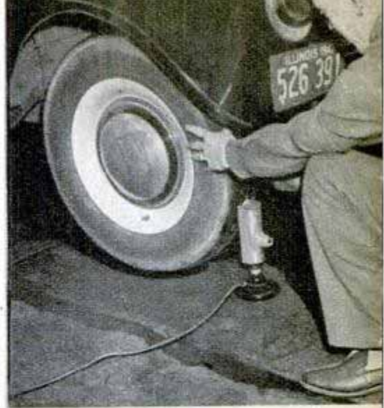
NAIL DETECTOR locates any metal object inside a tire casing that might work in and cause a puncture. A floating permanent magnet signals the presence of metal in the casing, yet its range is so limited it is not affected by metal rim or any wire reinforcement. A six-volt lamp provides signal flash
