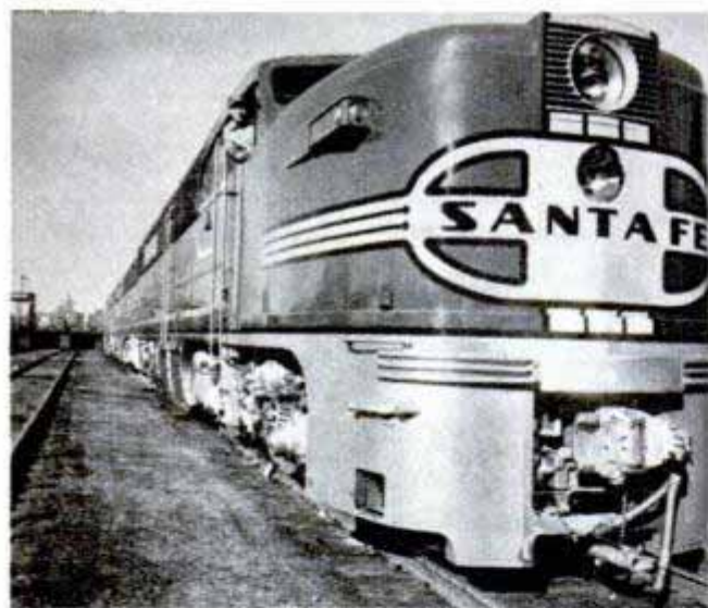
↑ Engineer's fingertips control 6000 horsepower in this new locomotive. Below, Diesel-electric engine can be geared for heavy freight or fast passenger run
