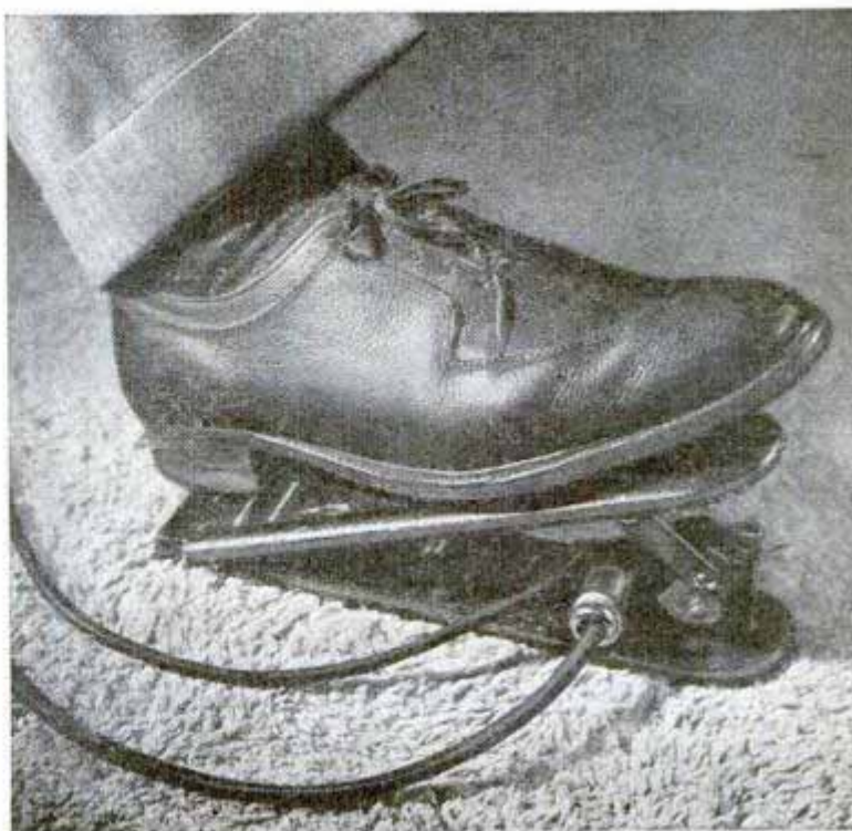
Lynn, the inventor of electronic instruments, plays his favorite, the vibrolynn, which mimics air raids and recites "Mary Had a Little Lamb." Below, foot control regulates volume by stepping up tone frequencies
