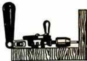
Drill's flat side holds bit parallel to surface.
