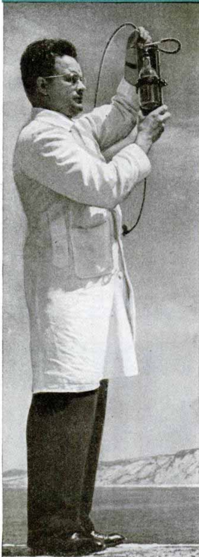
Dr. Claude E. ZoBell checks water sampler he designed. The bottle at right, above, shows oil scum from bacteria; bottle at left contains oil shale, no bacteria
