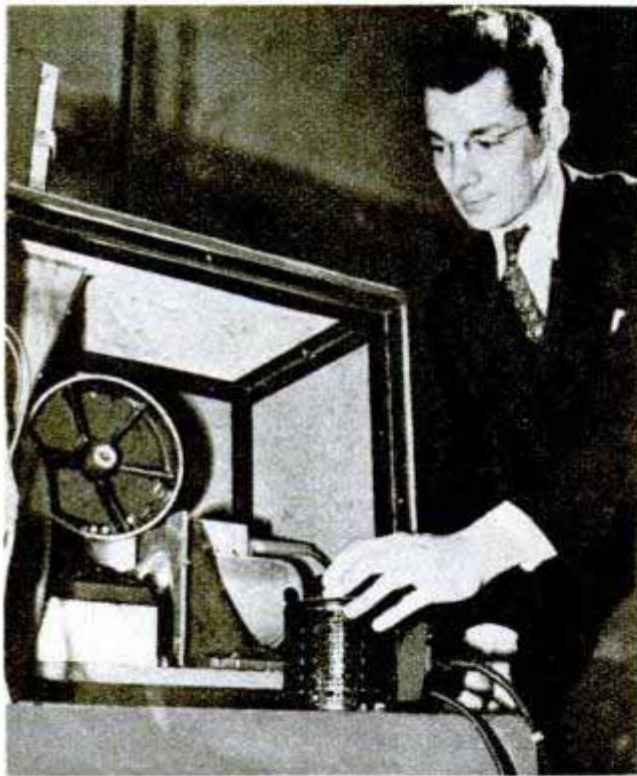
Top, a battery of small lenses snaps pictures. Top right, rifle is aimed preparatory to photographing bullet. Model above takes 70,000 pictures a second
