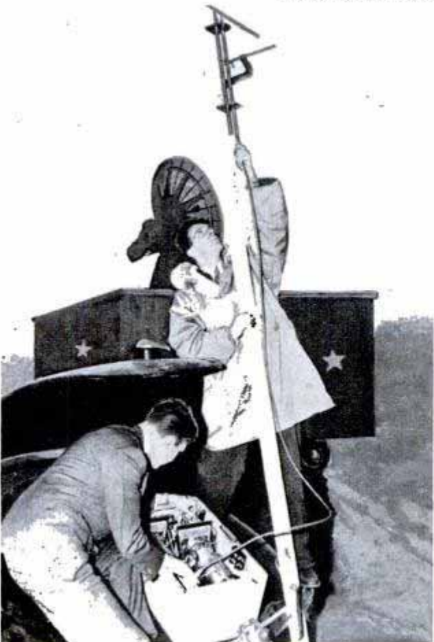
ROCKET RADIO installed in test-fired V-2 transmits 28 separate items of information each 1/35 second General Electric photo
