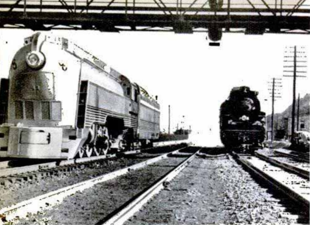
↑ Modernized by streamlined jacket, Chesapeake and Ohio locomotive actually began service in 1926. Drawing at right, reproduced from our cover, shows sky-view observation car of Milwaukee Road's Olympian Hiawatha
