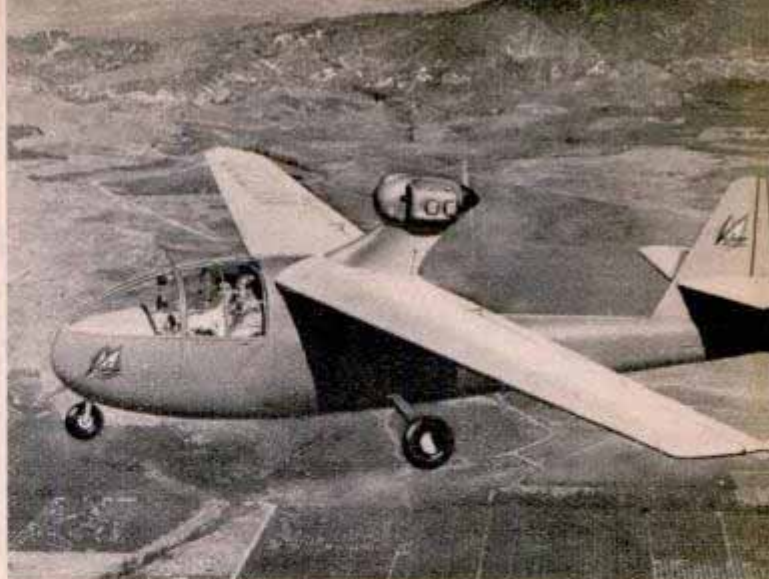
Verandalike visibility is a distinguishing feature of the new Volmer VJ-21. The three-place pusher has a top speed of 120 miles an hour and a 500-mile range. A low, auto-style door permits easy entry to the cabin
