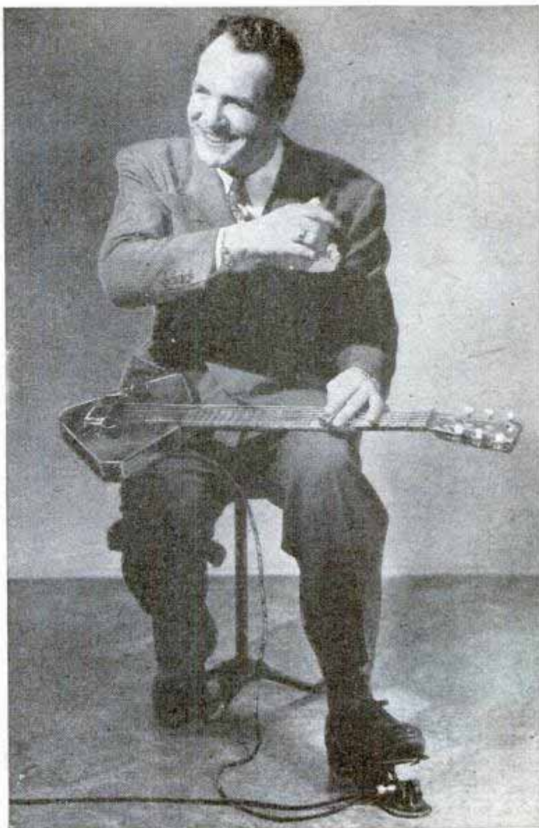
Lynn, the inventor of electronic instruments, plays his favorite, the vibrolynn, which mimics air raids and recites "Mary Had a Little Lamb." Below, foot control regulates volume by stepping up tone frequencies
