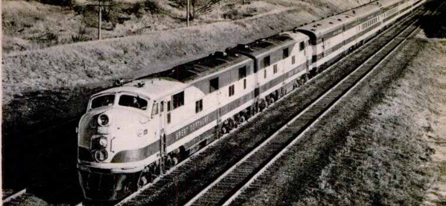
Postwar Empire Builders are pulled by two-unit 4000-horsepower locomotives with twin cabs
