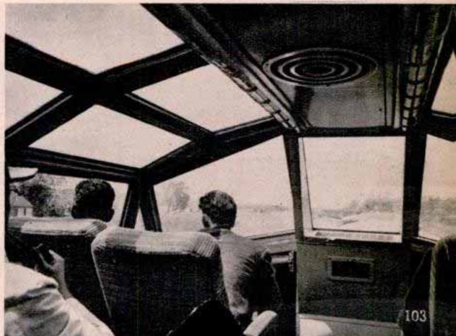
Left, designers have budgeted every inch of space in a single room that costs little more than an open section berth. Right, double-deck Vista Dome cars have glassed-in tops to give travelers a broad view of the scenery
