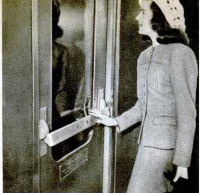
↑ Air conditioning-heating outlet is in the ceiling of Pennsylvania coach. After air is circulated it returns through tiny perforations in baggage rack. Right, door swings open automatically as soon as bar is touched
