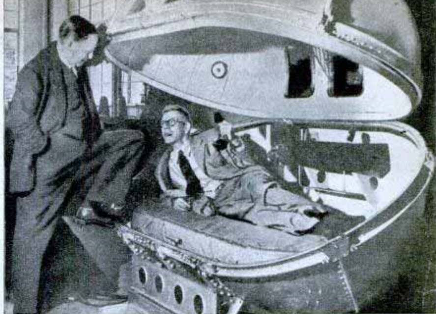
PRESSURE CHAMBER , designed on doctor's orders for Winston Churchill's flights, has a couch, telephone, ash tray, shelf
