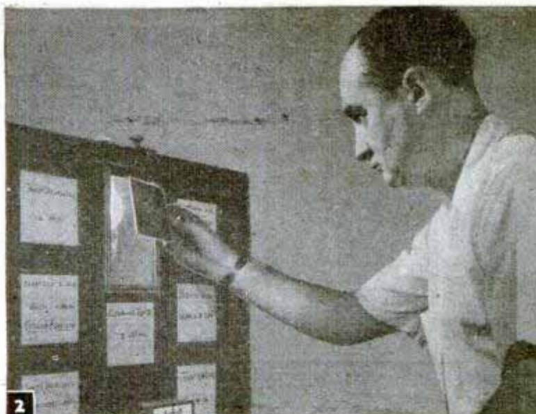
2 Second exposure requires only a few seconds because light from photoflood lamp is heat-filtered by absorbing glass in window
