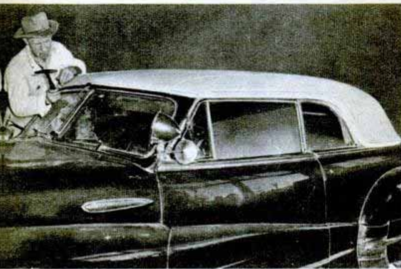
↑ Cloth is tacked to welded frame to complete a hand-tailored convertible top that will eliminate drafts
