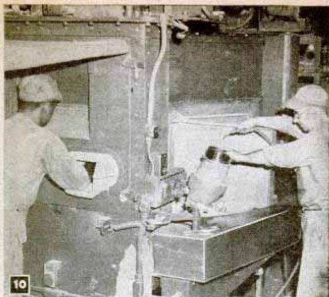
Sandblasting cylinders. Worker at left puts hands into rubber gloves and sleeves to handle the parts
