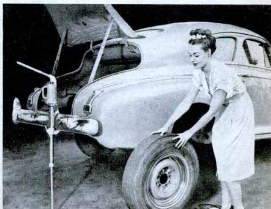
HYDRAULIC JACK fastens to bumper, can be installed without stooping. Handle is on top and requires only slight pressure
