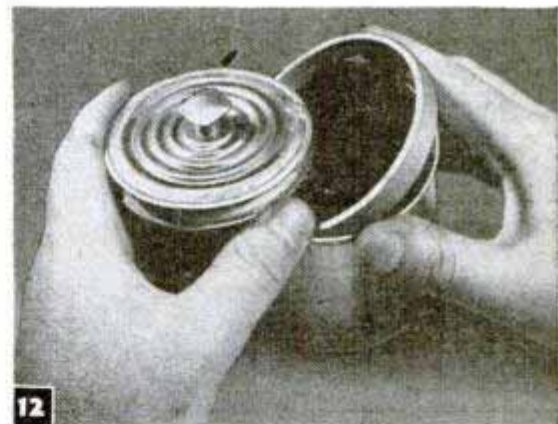
12 Section of embroidery hoop serves as a fitting for thermostat, which is covered with heavy oil
