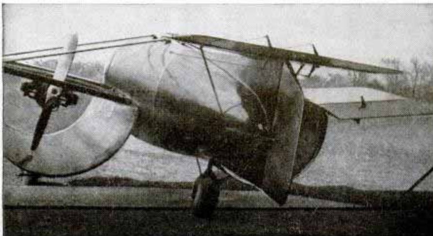
Readying six-foot channel for plywood skin prior to full-scale laboratory trials to determine lift, drag, thrust and pitching moment. Below, rear view of test model flown during Maryland trials. Despite its unusual appearance, the plane's controls are conventional and it is easy to fly
