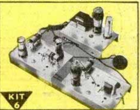
KIT 6 You build this Superheterodyne Receiver which brings in local and distant stations—and gives you more experience to help you win success in Radio.
