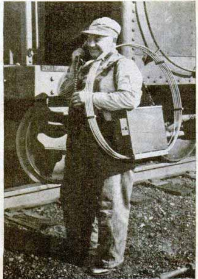
PORTABLE TELEPHONE for Pennsylvania Railroad picks up messages 15 miles away, receiving through air by induction with tracks as communication channels
