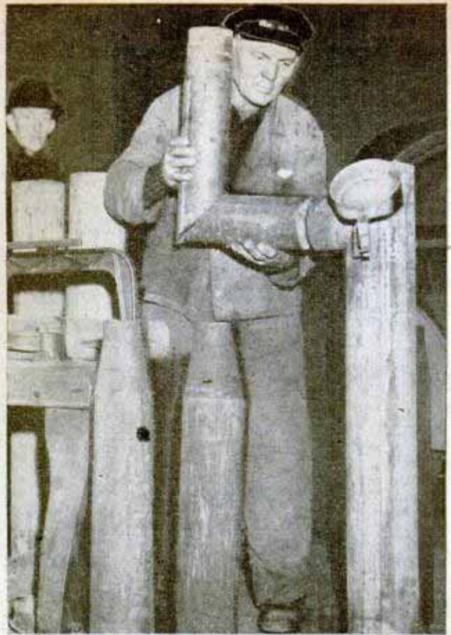
STOVEPIPES are made from German artillery and anti-aircraft shells by Wilhelm Kersten, a blacksmith who converts Nazi war scrap into essential products
