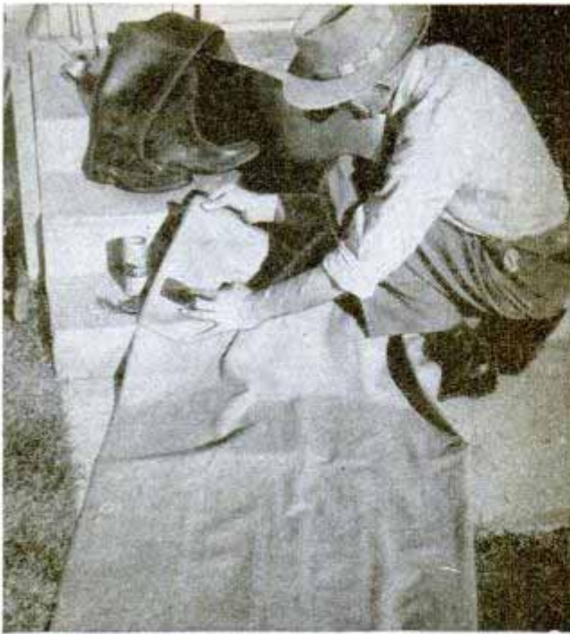
Air mattresses should be inspected or you may be in for a big letdown. Repair the leaks with a tire kit ↓ Bubbles from mattress immersed in water show leaks
