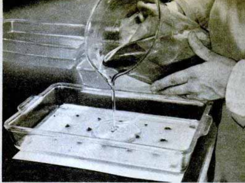
Next step in the process, developed by Ward's Natural Science Establishment, is adding a second layer of plastic
