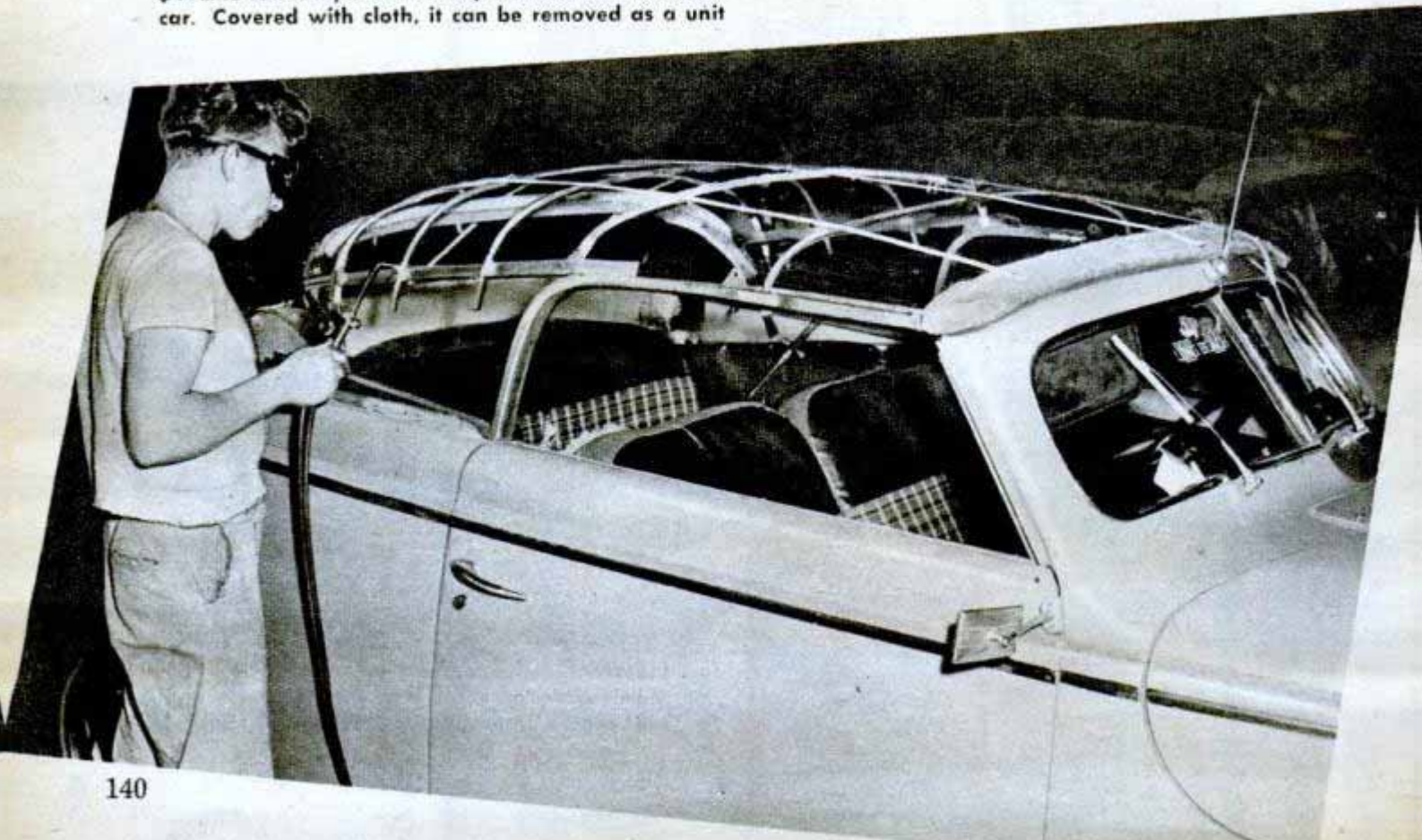
↓ Frame for semipermanent top is fitted to a cut-down car. Covered with cloth, it can be removed as a unit
