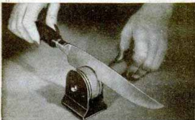
↓ KNIFE SHARPENER holds the blade at proper angle
