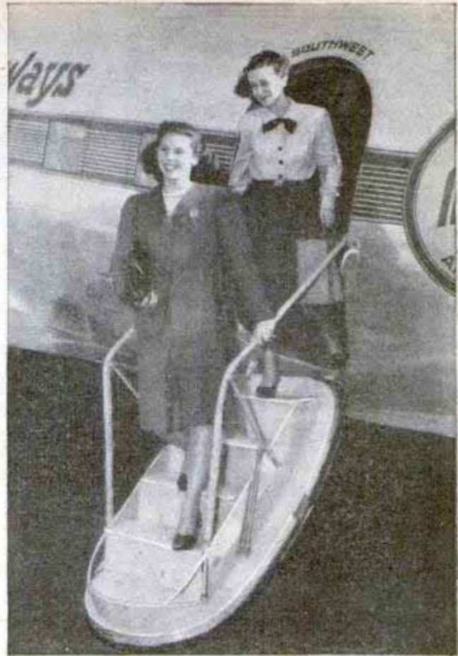
DOOR RAMPS are being tested by Southwest Airways to save time, labor and ground equipment at airports. They hinge at the bottom, have built-in steps to the ground and open from either the inside or outside
