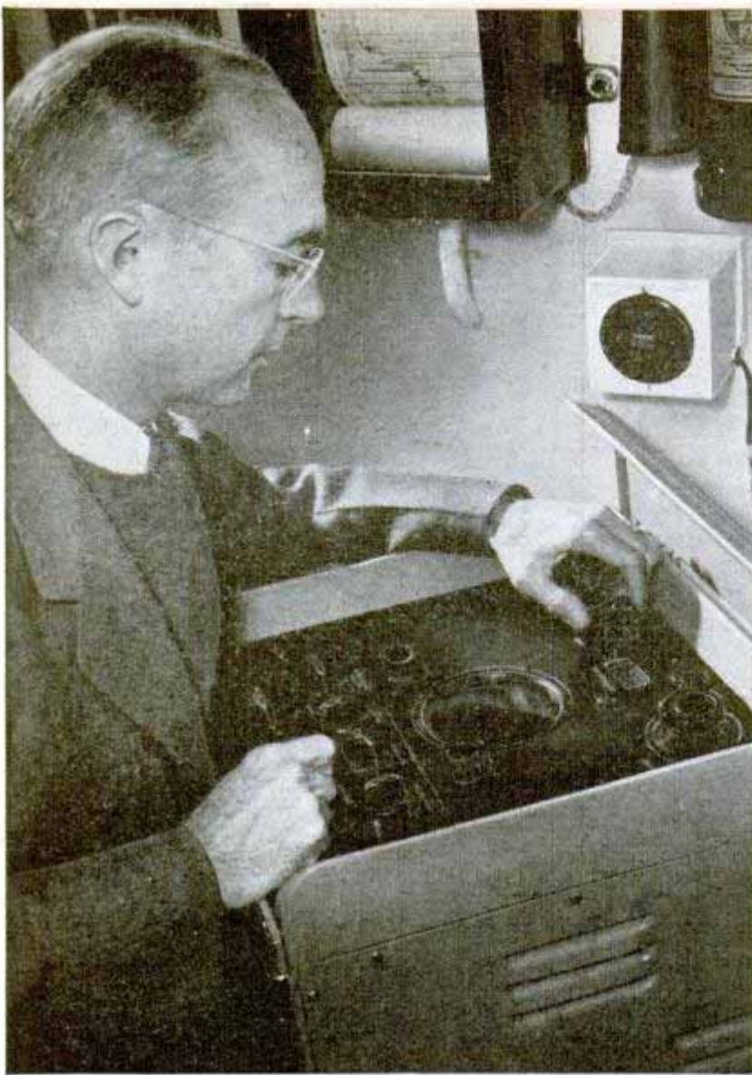
A ship's exact position is determined in two to six minutes by an electronic device called loran—an abbreviation for long range navigation
