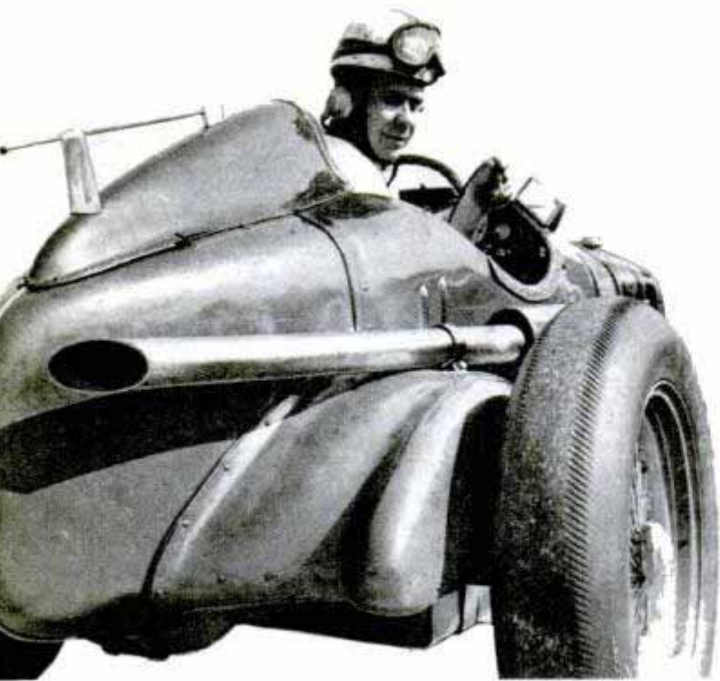
Rod on rear of car is the antenna of a two-way radio. Pit crew can warn driver at the first sign of trouble
