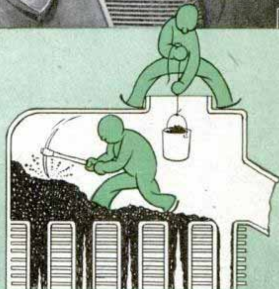
Here's how rust, boiled out of water jacket, can build up to obstruct the radiator tubes
