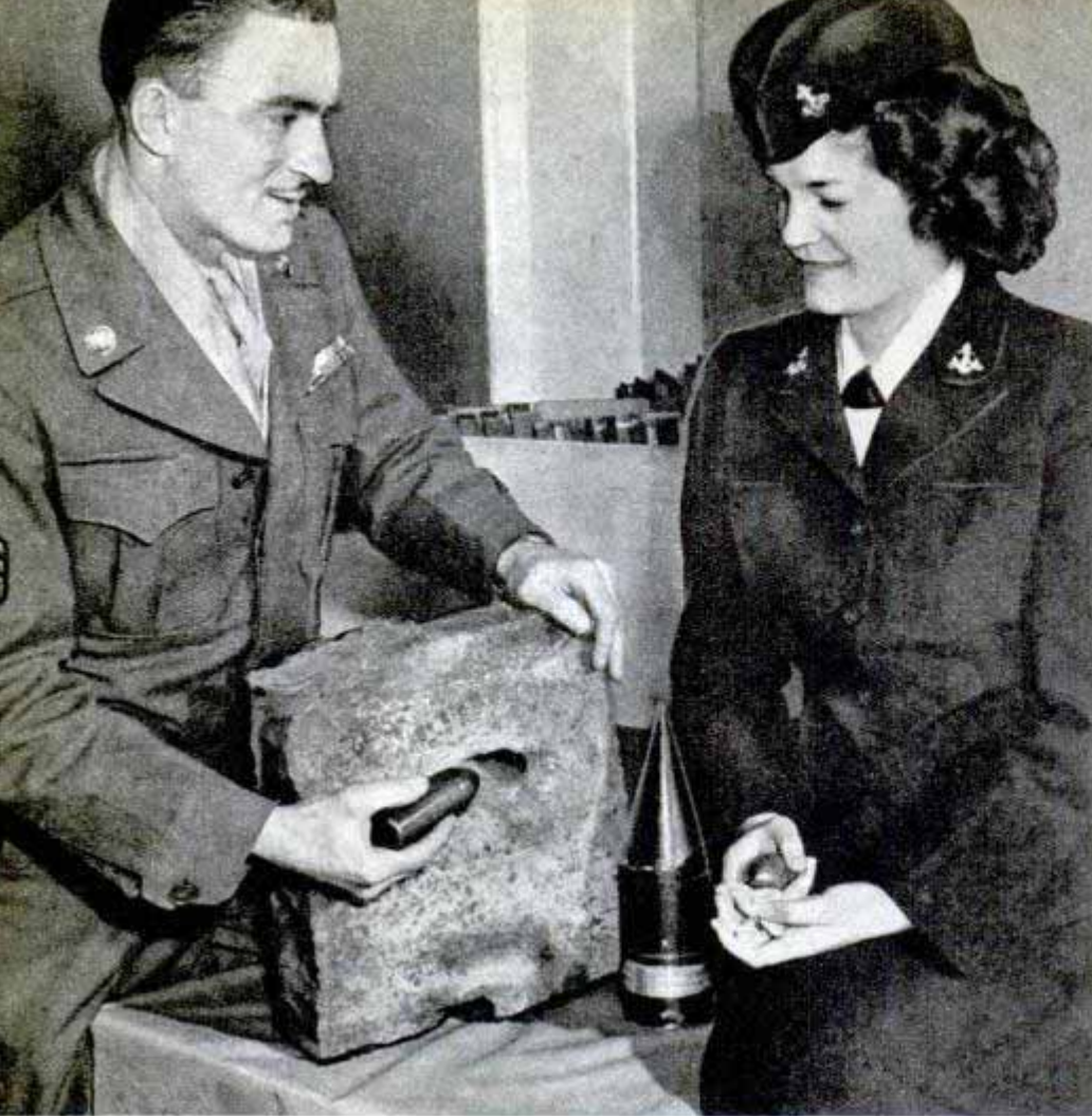
Section of heavy armor plate from German tank was pierced by hard carbide projectile. Carbide shell core shown below is centered in an aluminum housing
