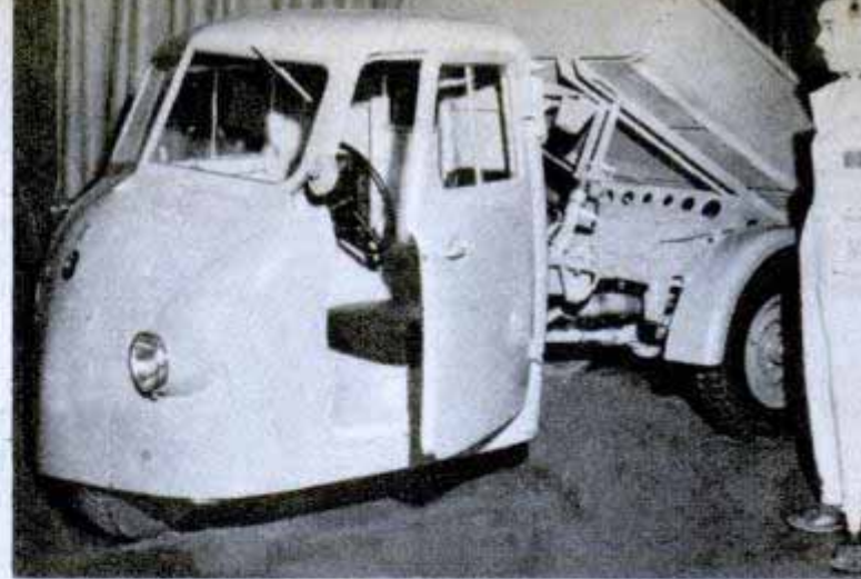
MIDGET VEHICLES are becoming popular in Italy because of their extremely low fuel consumption. The tiny car at the left covers 120 miles per gallon of gas under steady driving conditions and can be lifted by two men. The three-wheel dump truck at right carries as much as 1½ tons of cargo, yet goes 30 miles per gallon
