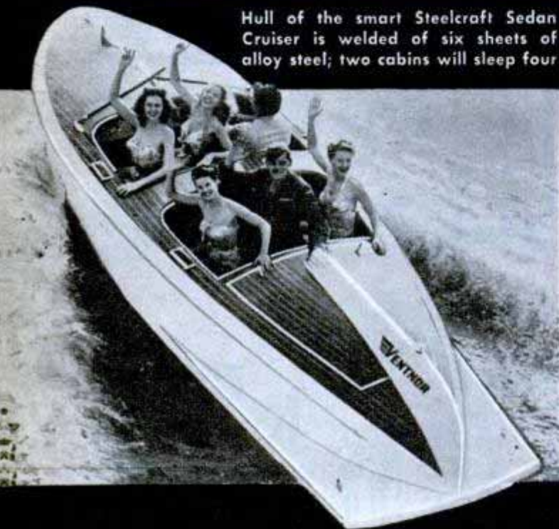
This 20-foot Ventnor De Luxe Runabout can go 40 miles an hour; it has 150-horsepower engine
