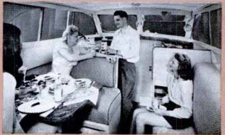
Screened sliding windows around the cabin of Chris-Craft's 27-foot cruiser make it open sport or closed family boat. Dinette in 26-footer, below, converts into double bed, and lounge seat at right makes up into upper and lower berths
