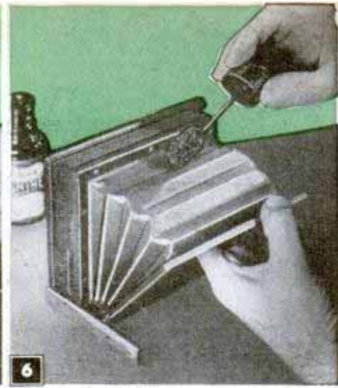
Shoe polish or leather dye is used to touch up the bellows
