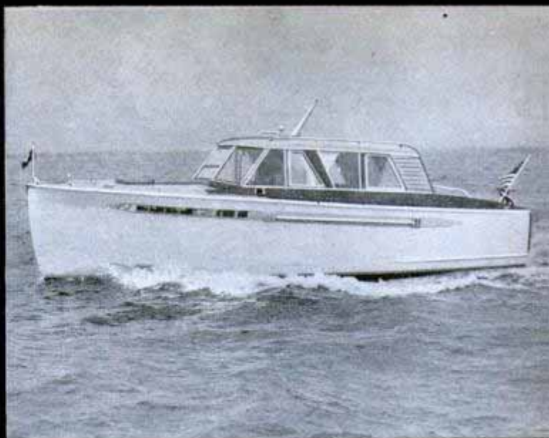
Plexiglas strip along hull of 33-foot craft provides something new in portholes. The square ports swing open on hinges to ventilate the cabin of the Sunlounge
