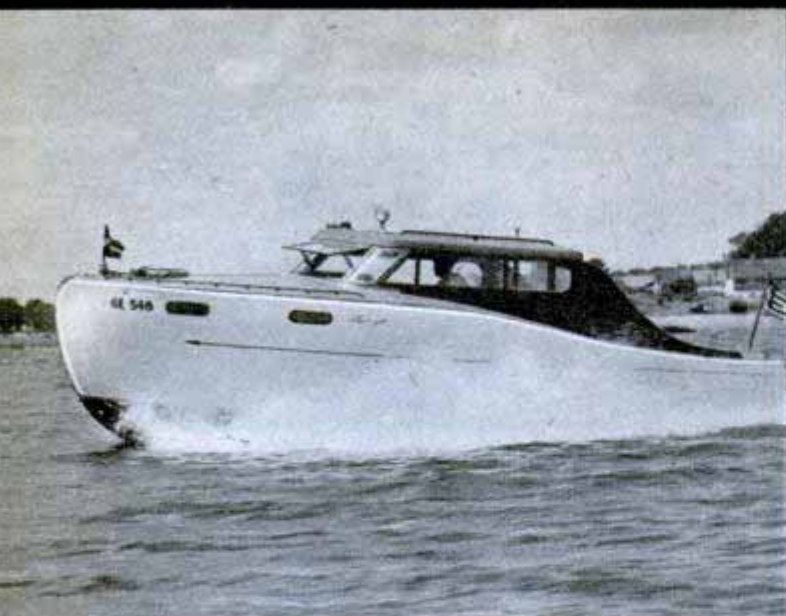
Hull of the smart Steelcraft Sedan Cruiser is welded of six sheets of alloy steel; two cabins will sleep four
