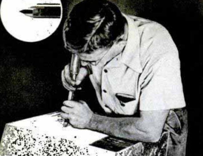
Steel chisel tipped with carbide is used in sculptor's air hammer. Right, magnified particles of Carboloy
