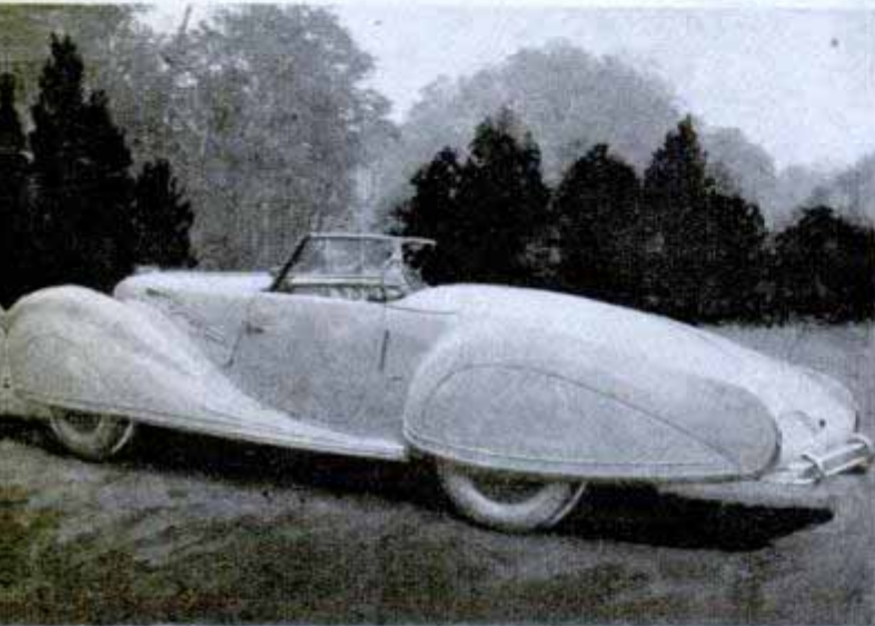
SLEEK CAR for the French buyer is the Delahaye Competition, a low-slung six-cylinder auto with super streamlining. Available in the models shown above, it has built-in headlights, an electromechanical gearbox and a special oil system. Cars built by this manufacturer have won several international races in the past
