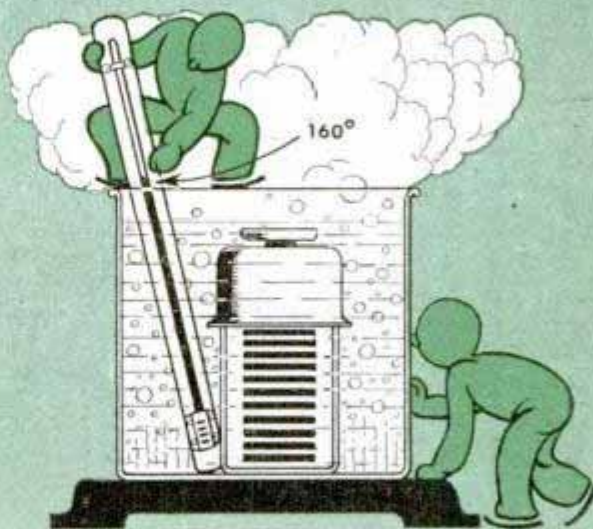
Test thermostat's working order. Gummy one that fails to open causes overheating
