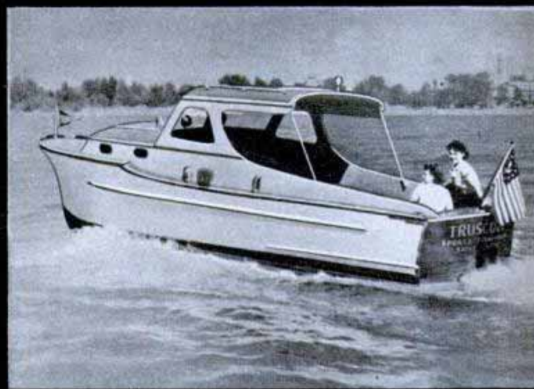
The Sport Fisherman has seats for six but bunks only two. Maximum speed is about 27 miles an hour with a choice of Chrysler, Gray or Kermath engines. Below, Elco Sports Cruiser — see plan view on opposite page
