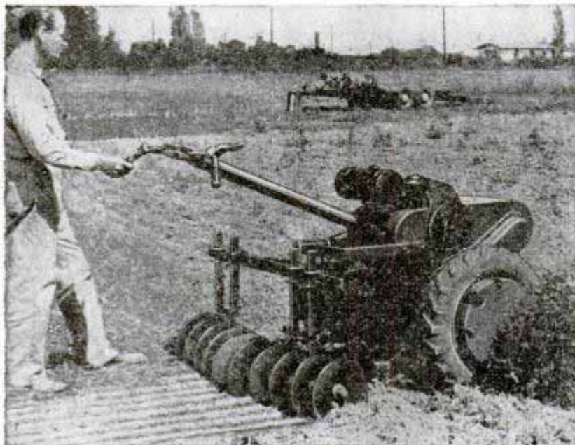
Handlebar controls on two-wheel tractor allow operator to walk to one side when plowing or cultivating
