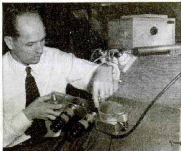
Photos of cosmic rays, showing trails of ionized water vapor particles left behind as they speed through the cloud chamber, are made with stereoscopic camera at left. Dr. Carl Anderson, right, at chamber's control panel
