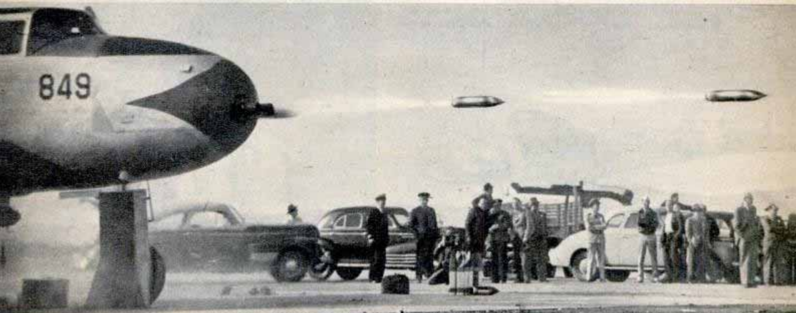
↑ Searing flame jets out through exhaust stack of the test ship just before rocket emerges from its tube ↓ Two rockets streak from the plane's nose in the first ground test of new weapon designed for air combat
