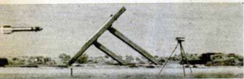
↑ Double motors give an 11.75-inch rocket airplane speed when it's launched from the 1500-foot test track ↓ Strip photos show the same rocket penetrating a 2½-inch armor-plate target and exploding just beyond
