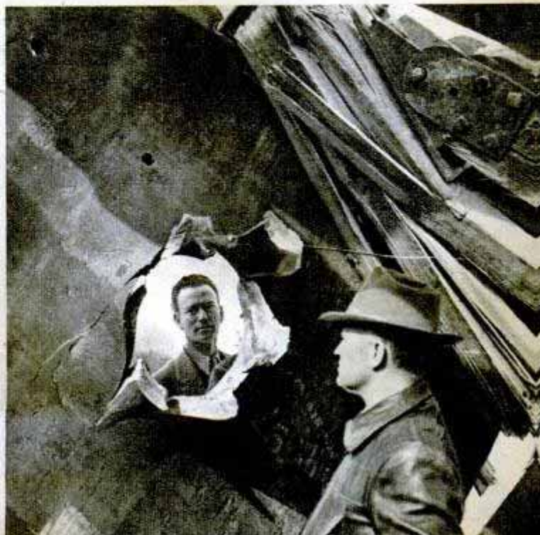
↑ Note marks left by fins when rocket penetrates target ↓ Ordnance experts examine opposite side of the armor
