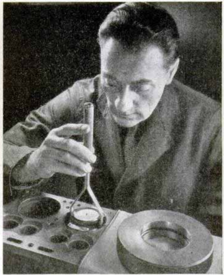
Gauge shows wear to nearest 0.0001 inch in cylinders
