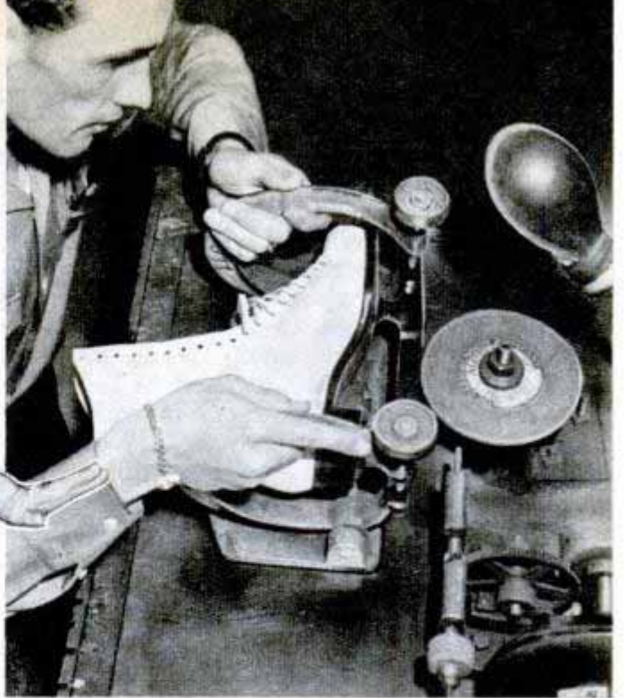
Evelyn Chandler performs difficult butterfly leap. Right, skate is sharpened against edge of grinding wheel cut to convex shape
