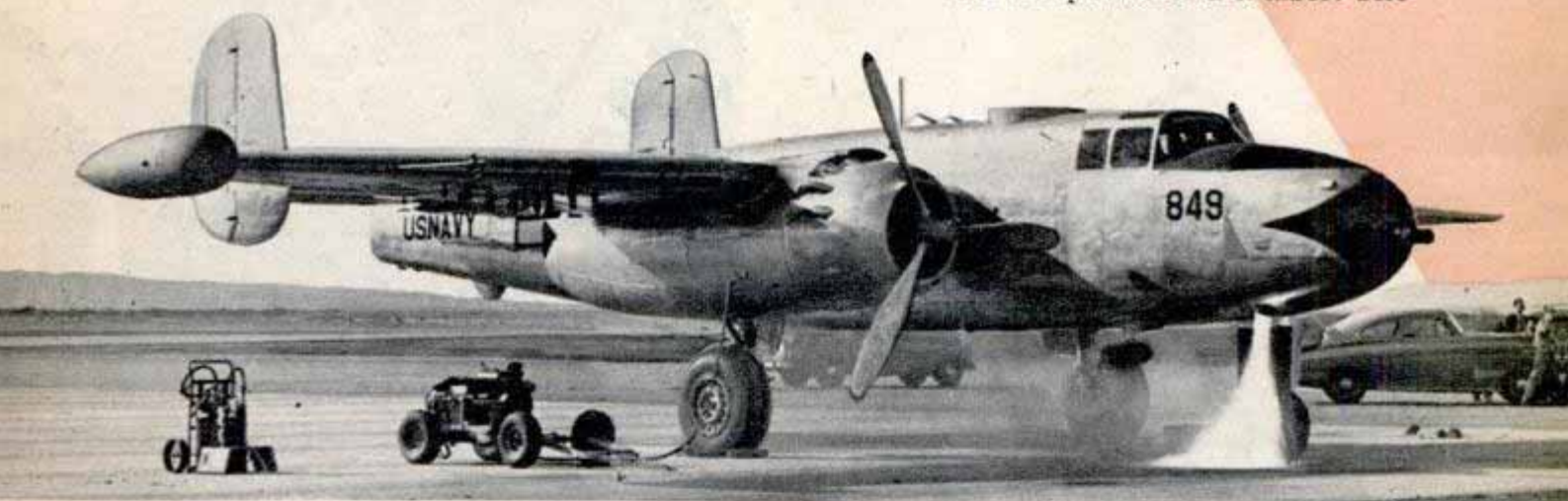
↑ Searing flame jets out through exhaust stack of the test ship just before rocket emerges from its tube ↓ Two rockets streak from the plane's nose in the first ground test of new weapon designed for air combat
