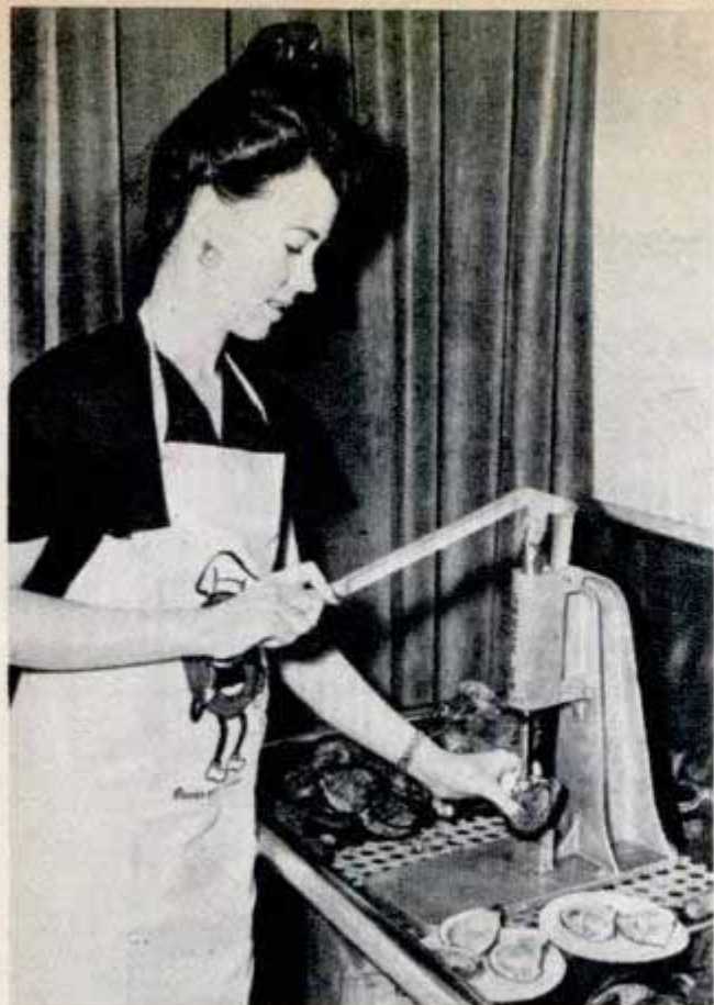
OPENING OYSTERS is no longer a struggle. By placing pressure on the center of the oyster, new shucking device opens the shell without damaging the oyster
