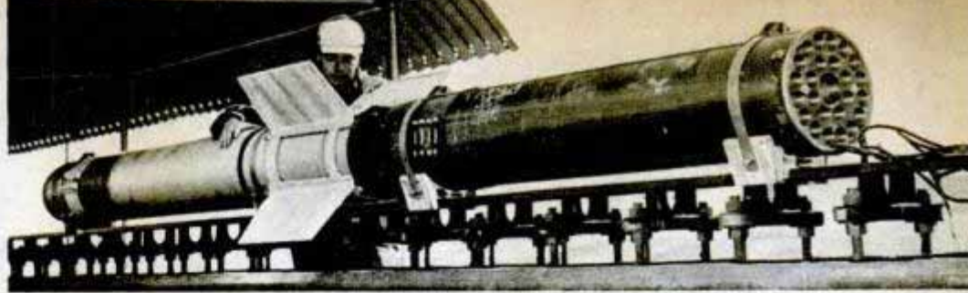
↑ Double motors give an 11.75-inch rocket airplane speed when it's launched from the 1500-foot test track ↓ Strip photos show the same rocket penetrating a 2½-inch armor-plate target and exploding just beyond
