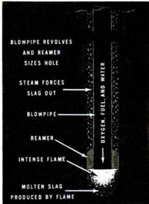
Above left, experimental rig is set up for a fusion-piercing test. Left, diagram shows how an intense flame melts hole through rock. Above, rig expels slag during test. Right, six-inch blast hole was drilled 30 feet by fusion piercing
