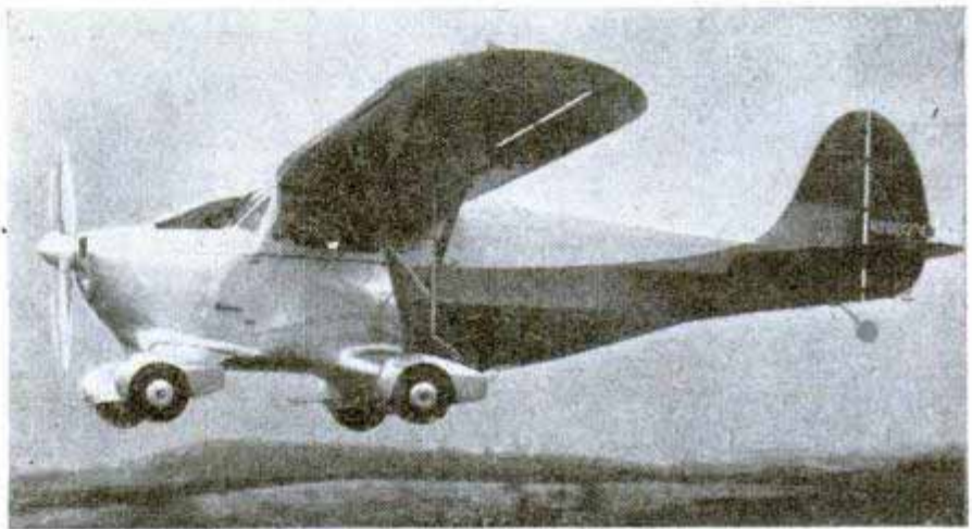
As a two-passenger automobile, left, the Airphibian can go 750 miles on a tank filled with 30 gallons of gasoline. Converting it from air to road use requires disconnecting two locks and takes five minutes. The silver colored, aluminum bodied coupe has a roll-back canvas top
