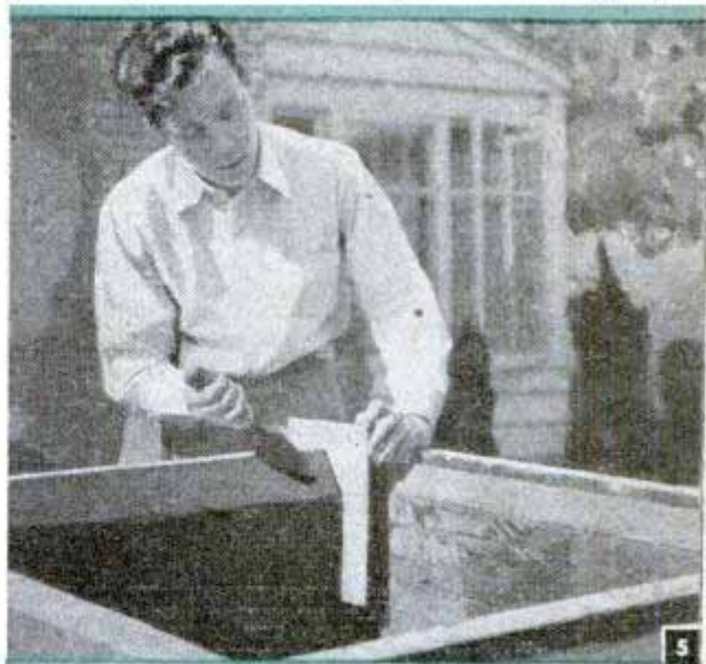
A template must be used to gauge the correct bevel between the sides and lid of the unit
