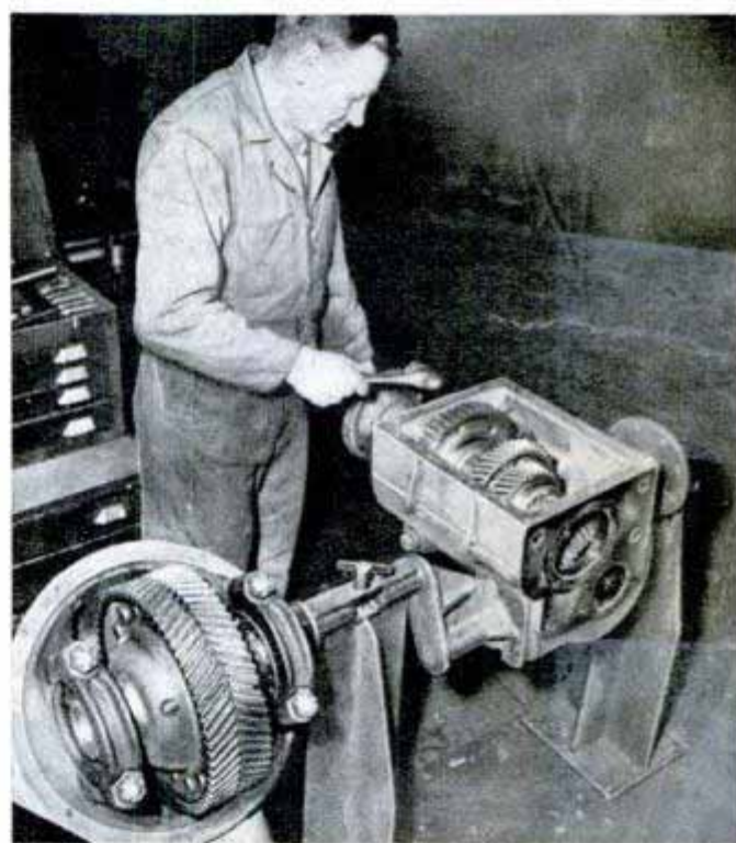
Gearboxes and rear-end gear assemblies mounted on test stand for complete teardown and overhaul. Below, a special device for testing and adjusting fuel pumps
