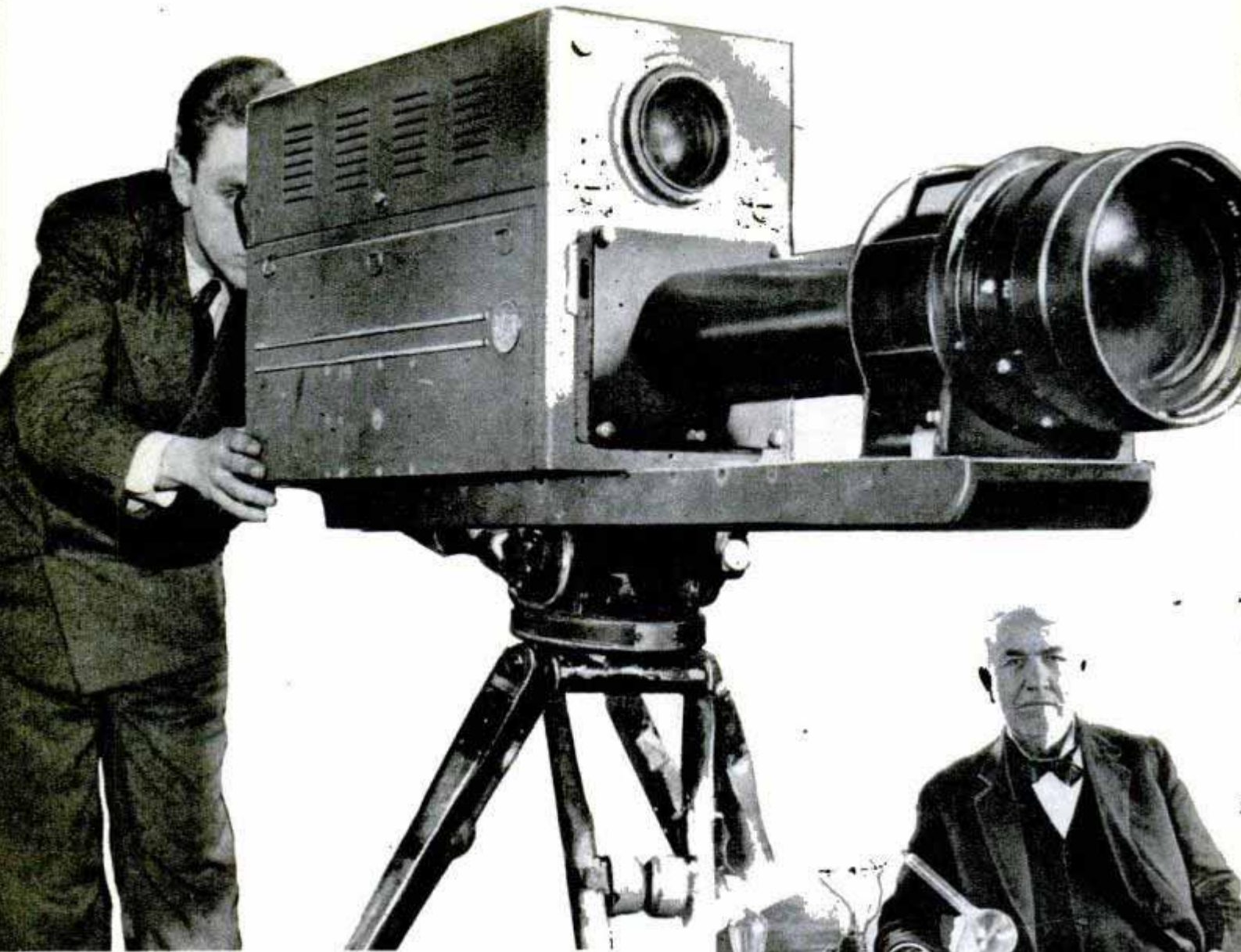
Outdoor sports events are televised by NBC with a 40-inch focal length lens, the longest ever used. Television and other electronic miracles stem from Edison's discovery of the Edison Effect which he found while working with externally wired lamps, right
