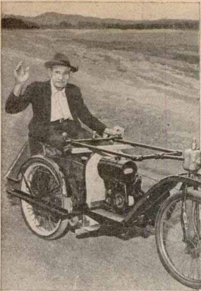
Since building a 1½-horsepower tricycle from scrap, 87-year-old Marshall Pressley finds it easier to get around. The machine is driven by a belt transmission
