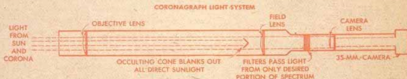
The coronagraph resembles a long-barrel field gun. Its photoelectric guider keeps it pointed toward the sun
