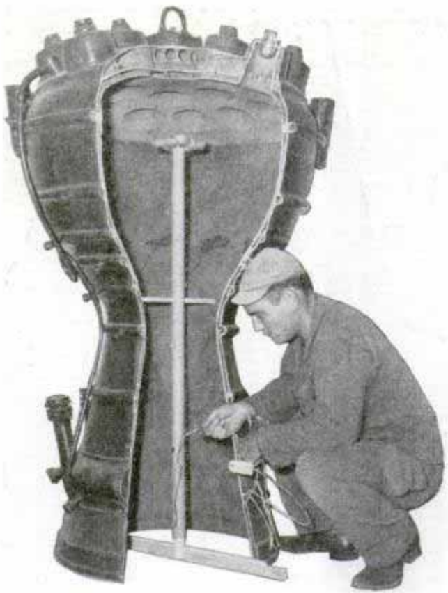
Cutaway V-2 motor shows double skin in which the fuel is preheated before entering the blast chamber
