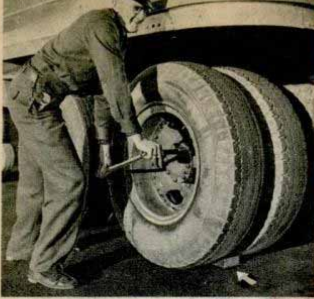
Easiest change is an outside tire. Driver can run inside wheel up on a wooden block and avoid using his 10-ton jack. At right, bumping each of the 19 giant tires with a steel bar to detect any sign of softness
