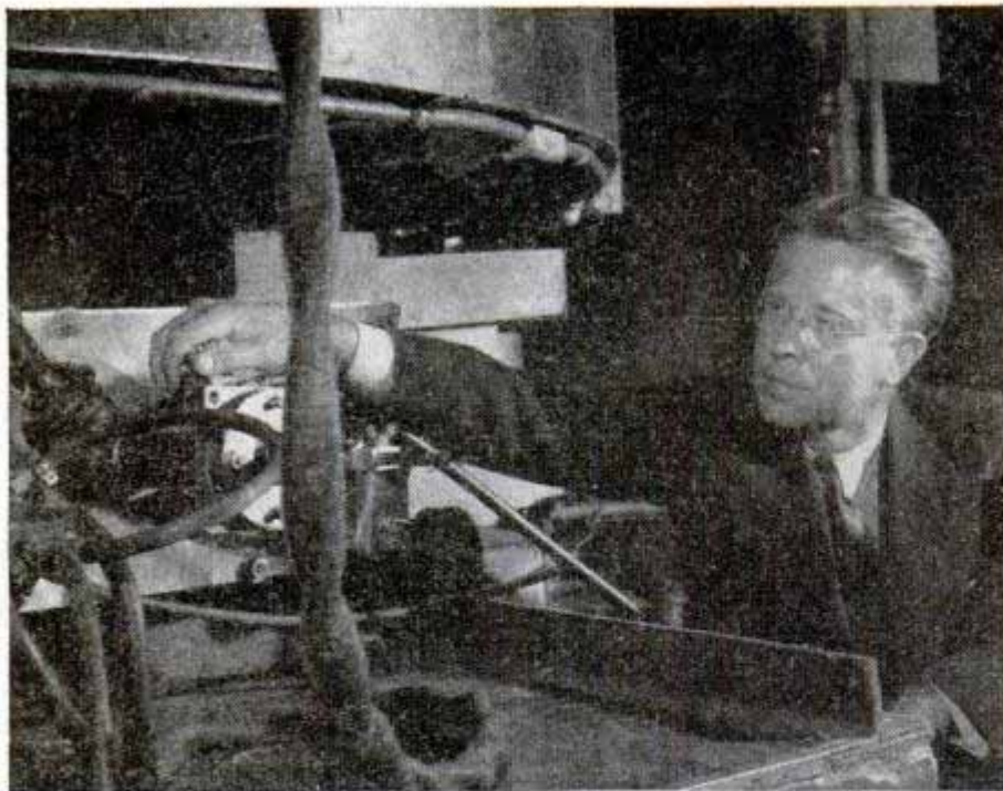
Professor Ernest O. Lawrence, noted University of California physicist, adjusts the target area of a pilot model for the giant 184-inch cyclotron
