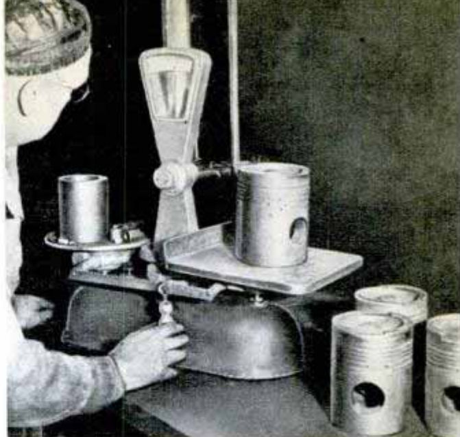
Maintenance is an around-the-clock affair. Mechanic balances pistons to match weight of six in full set
