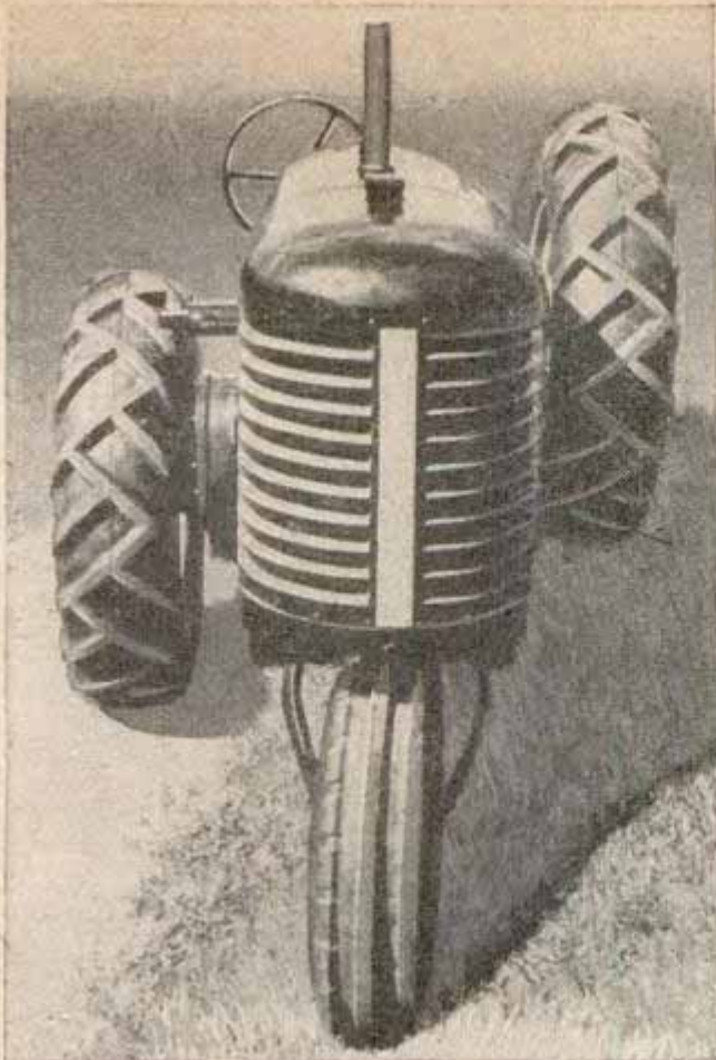
TRACTOR has rear wheels which automatically adjust their height to contour of land to keep machine level
