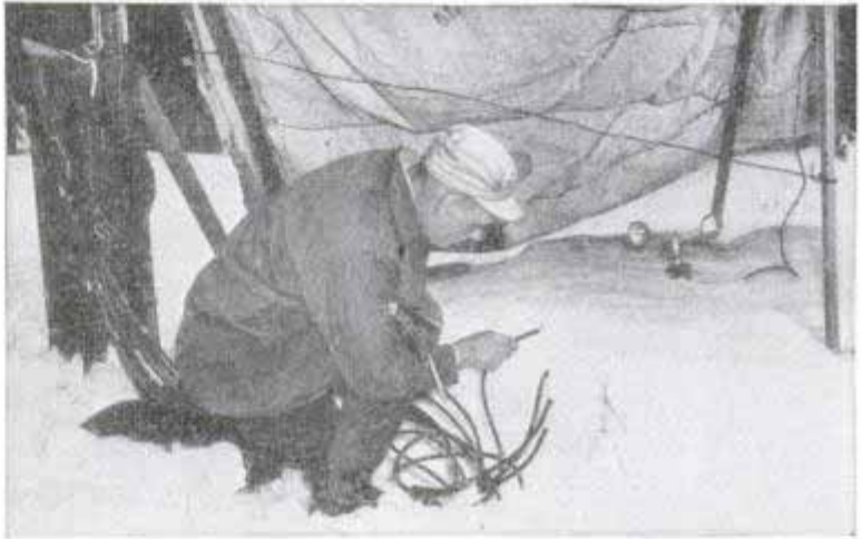
Snowfall is measured in terms of precipitation in tank at upper left and the volume of melted run-off from test basin is recorded at station above. Below, electric wires are plunged into the snow to measure its temperature. Ground and air temperature at 28 points register at one minute intervals on meters shown at bottom
