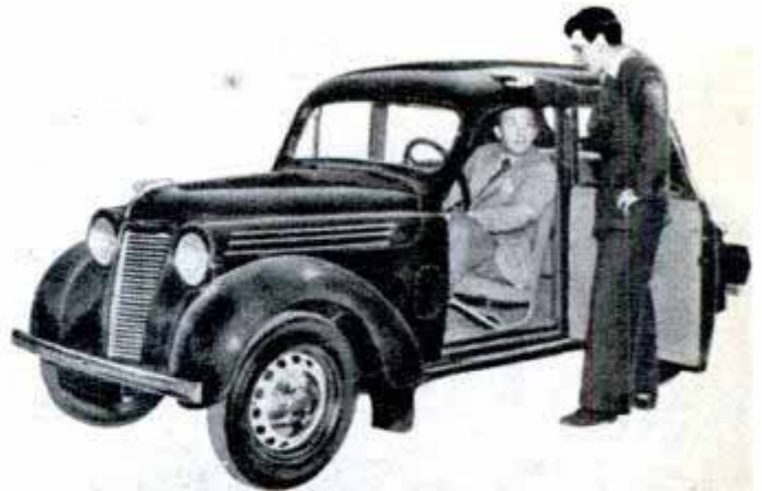
Renault Eight, a popular French model, has a detachable aluminum cylinder head, will go about 50 miles per gallon
