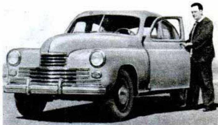
Victory car with four-cylinder engine follows American trends. Headlamps are built into long sweeping fenders
