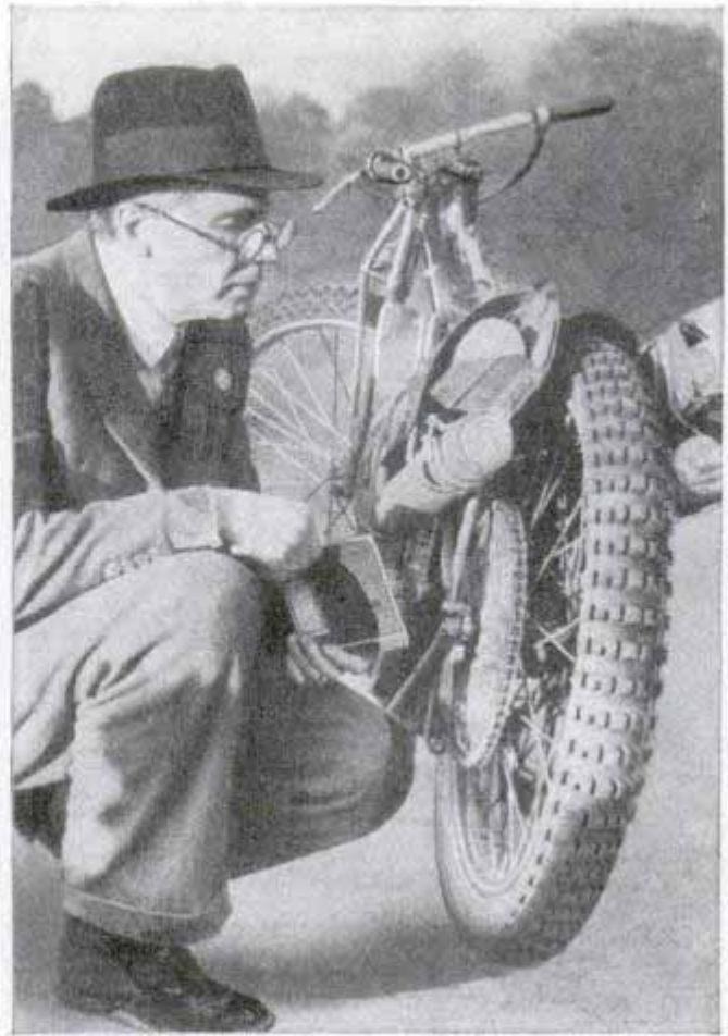
FOUR ROCKETS controlled by switches on handlebars give an added boost to a speedy English motorcycle
