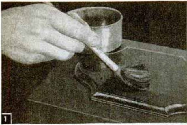
1 Only small areas at a time should be treated and a brush should be used to keep the solvent active
