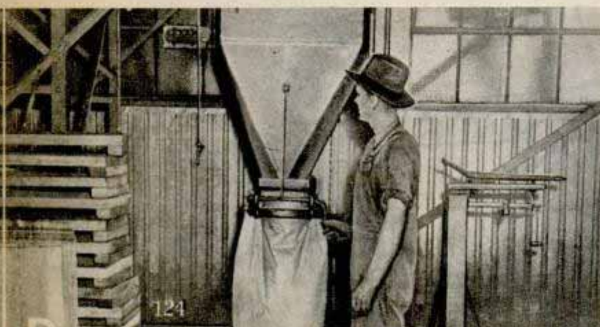
A—Conveyor belt takes ore from truck to plant B—Crusher pulverizes biggest chunks of ore C—Ore is separated from rock by air pressure D—Processed gilsonite is sacked for market
