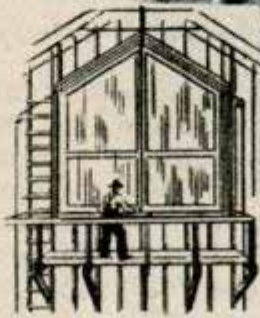
If the doors should open suddenly this farmer would disappear. The walkway should be three feet beneath door level with a handrail
