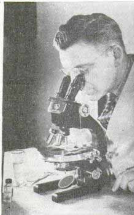
↓ Bottom, phase microscope equipped with light-controlling diffraction plate (upper inset) clearly reveals mold fragments (white objects below)
