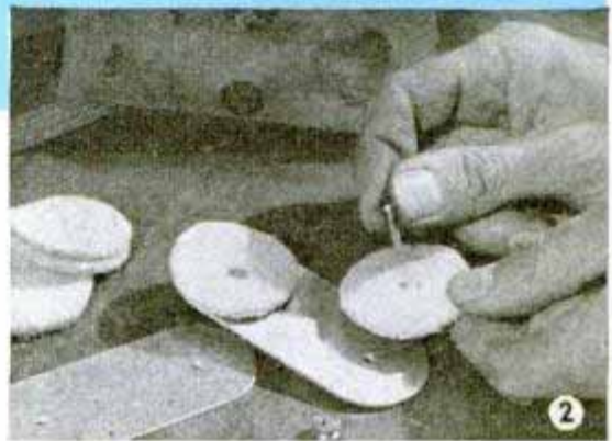
Four miniature powder puffs are used as cleaning pads. Small bolts hold them in place
