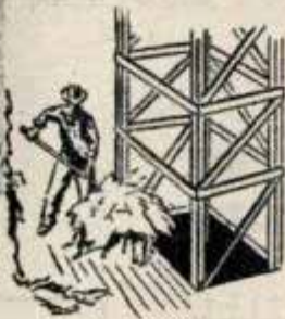
Open hay chutes can mean a quick, unexpected trip to ground level. A framework like the one drawn at right will protect the farmer
