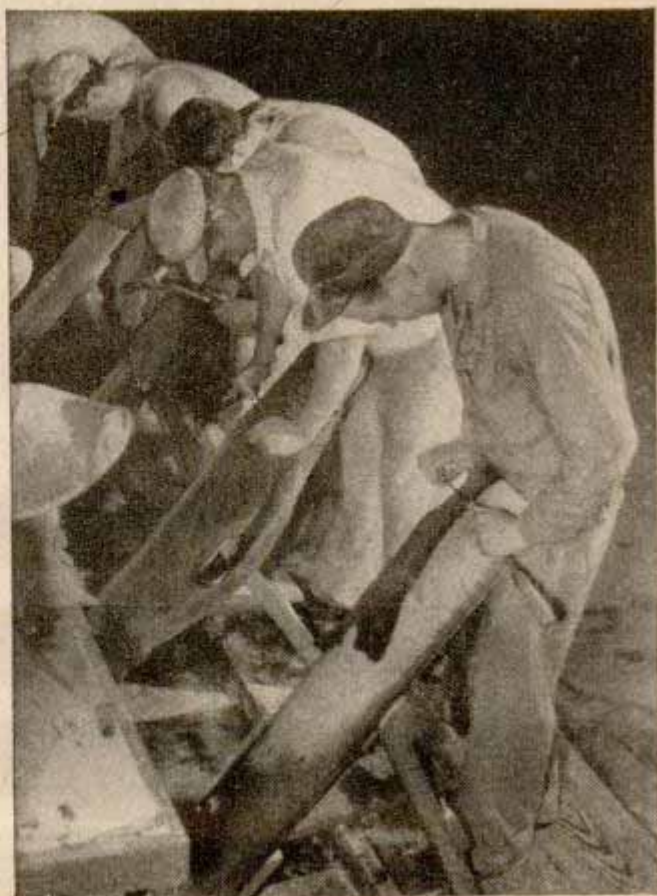
↓ Coarse guard hair is removed from sealskins by a two-handed knife deftly moved across the surface. The blade is kept dull so that no fine fur will be cut
