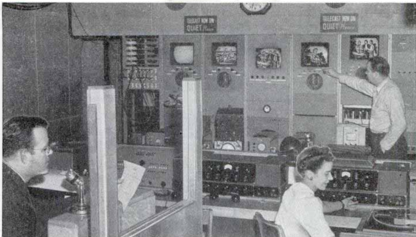
Director supervises broadcast from booth at left. Screen at far left is reserved for remote pickups, the second is a movie film, the two at right show what studio cameras see, and center screen shows what's on the air
