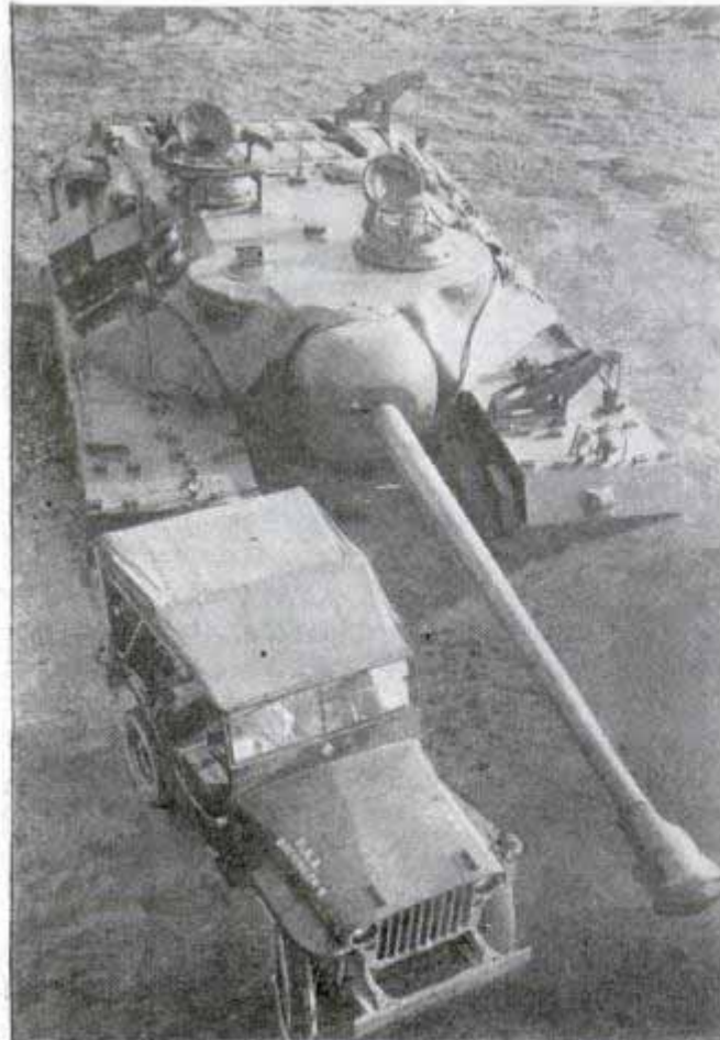
SUPERTANK for the Army weighs nearly 100 tons and carries a 105-mm. gun that dwarfs a jeep in length. The Army says it's the heaviest vehicle ever built
