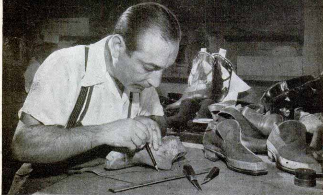
Wooden lasts shaped exactly like the feet of film stars guide Joe Napoli in making movie boots and shoes
