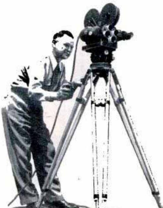
Mitchell professional "16," small version of 35-mm. studio camera, operates on 110 volts
