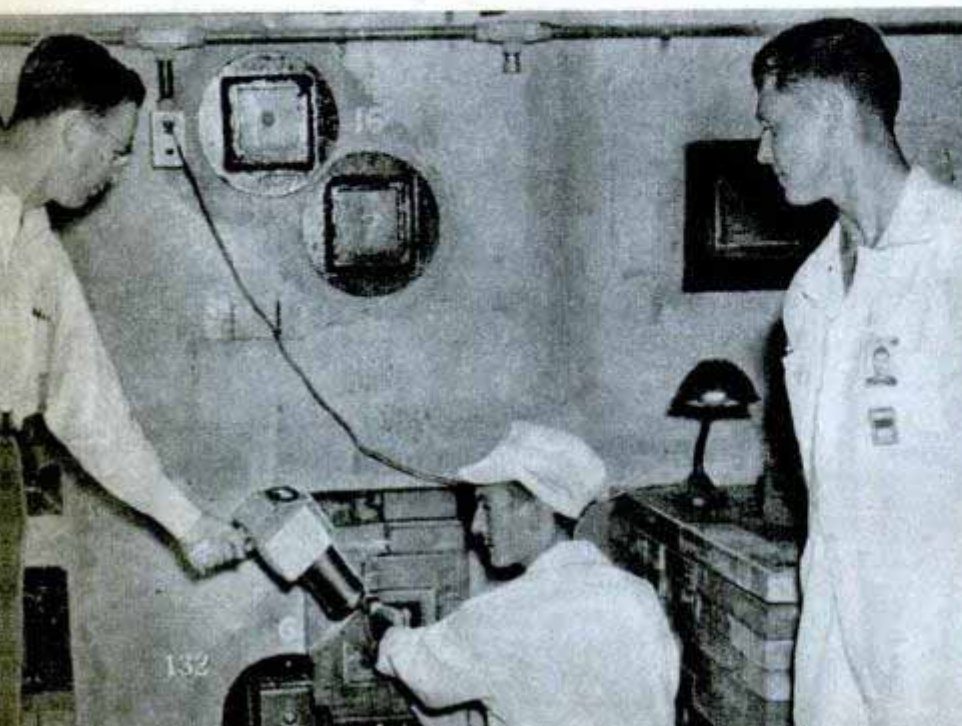
Isotope can is sealed prior to being inserted in atomic pile. Below, removing shielding plugs from uranium pile before freeing isotope. Uranium is bombarded behind protective walls of concrete
