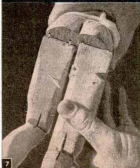
7 Toothpick holds end of cord, and notches are made to receive knots
