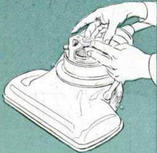
7 EXAMINE THE COMMUTATOR AND CLEAN WITH FINE (8-0) SANDPAPER
