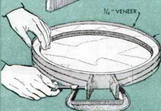
THEN, VENEER BAND COVERS EDGE TO CONCEAL PLYS...
