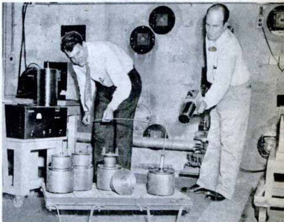
Can of radio-isotopes (above) removed from the pile is placed in a lead shipping container. Below, physicist (right) uses radiation-measuring device to be sure no dangerous rays are emitted
