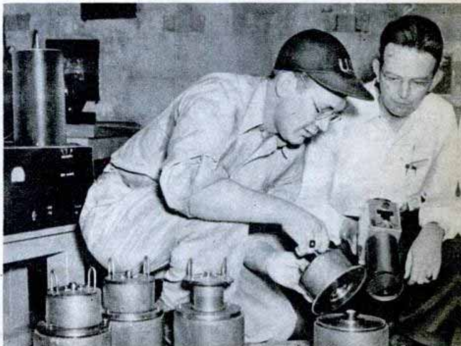
Can of radio-isotopes (above) removed from the pile is placed in a lead shipping container. Below, physicist (right) uses radiation-measuring device to be sure no dangerous rays are emitted
