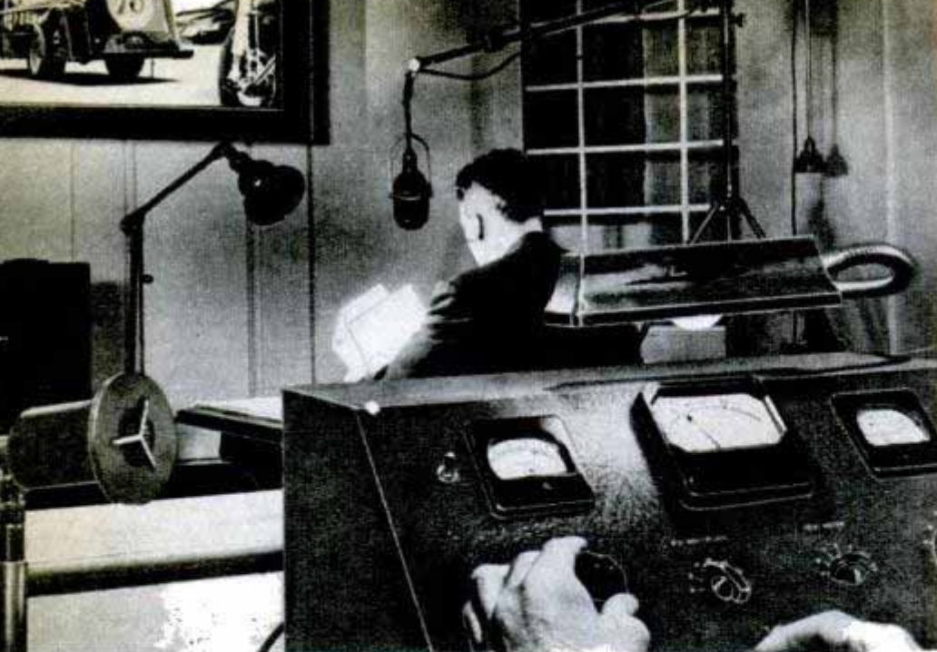
Narrator supplies voice accompaniment to the film as he watches screening in the studio. Mixer handles the controls that record voice on film
