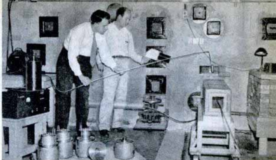
Remote control device—out of range of dangerous radiation—is used to remove atomic energy (radio-isotopes) from uranium pile
