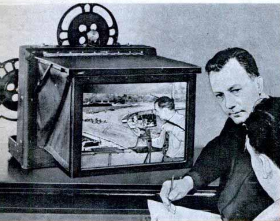
When equipped with a hood, 16-mm. projector can show clear movies in ordinary light. Top of the hood is one side of the projector carrying case
