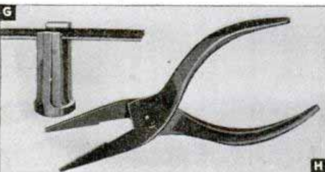
(G) Plastic stand-off insulator for 300-ohm twin-lead transmission line keeps line at fixed distance from any surface. (H) Shockproof plastic radio pliers. (J) Absorption wave meters available in many ranges. These handy frequency meters can be poked into small shield compartments, coil stages and corners to check harmonics and for similar applications, thus enabling the experimenter to find out exactly what is "going on" in the circuit
