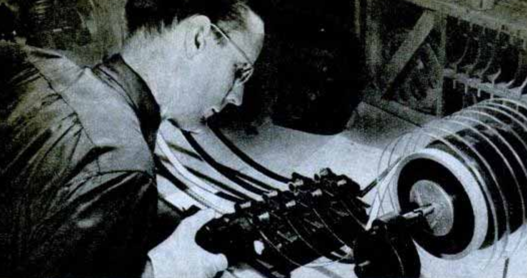
↑ In preliminary step to making 16-mm. sound-on-film master prints, picture reels must be matched and synchronized with three sound-track reels
