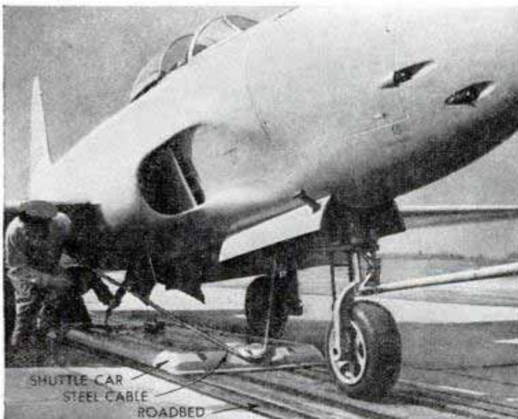
Hitching the "bridle" to shuttle car for takeoff and a view of the 1382-foot track on which plane is pulled
