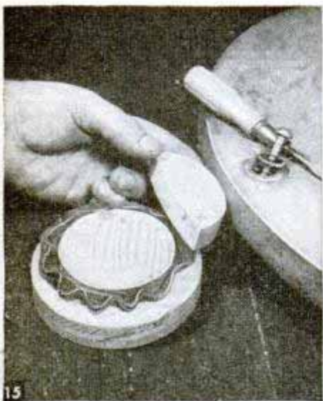
15 If the insulators are used under a drill-press base an additional semicircular block is provided for a bearing
