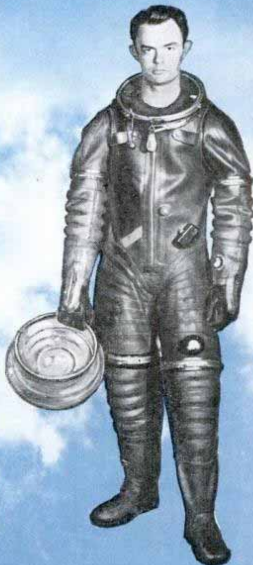
Resembling a deep-sea diver, the pilot in a high-altitude pressure suit is holding his transparent fishbowl helmet
