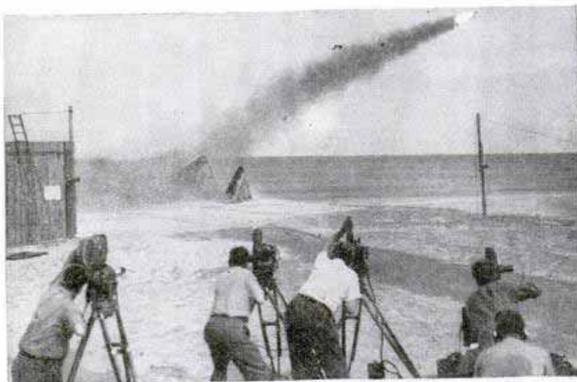
Above and below, launching 70-pound ramjet engine capable of speeds over 1500 miles an hour. Bottom, close-up view of the propulsion unit
