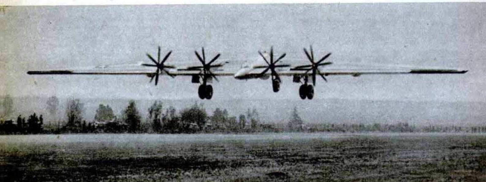
FLYING WING BOMBER , the first of 15 that Northrop Aircraft is building for the Army Air Forces, rises into the air on its initial test flight. The high-speed camera momentarily "stops" the pusher-type eight-blade coaxial propellers. Performance figures are still secret but it has been revealed that the plane has a 10,000-mile range
