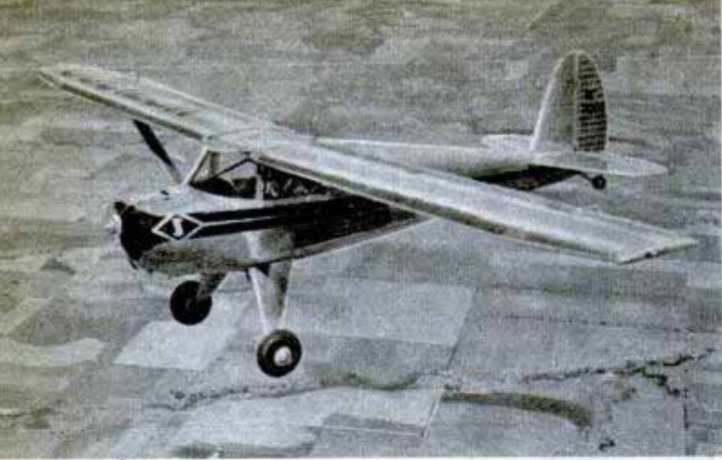
ALL-METAL WINGS replacing fabric-covered type boost speed of Luscombe Silvaire five to eight miles an hour. They're also more durable and easier to inspect
