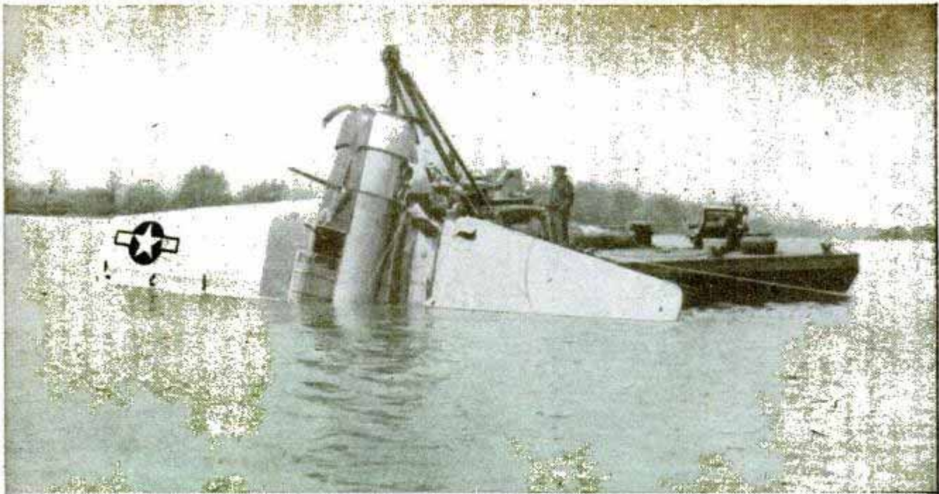
Trapped victims must be removed first. Then diver fastens salvage lines and wreckage is hauled to surface
