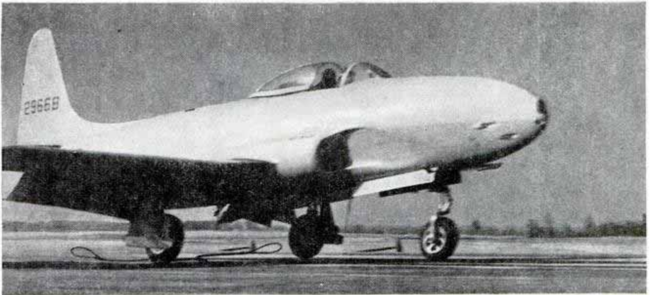
Jet fighter releasing steel cable "bridle" and taking to the air at 116 miles an hour after 340-foot run
