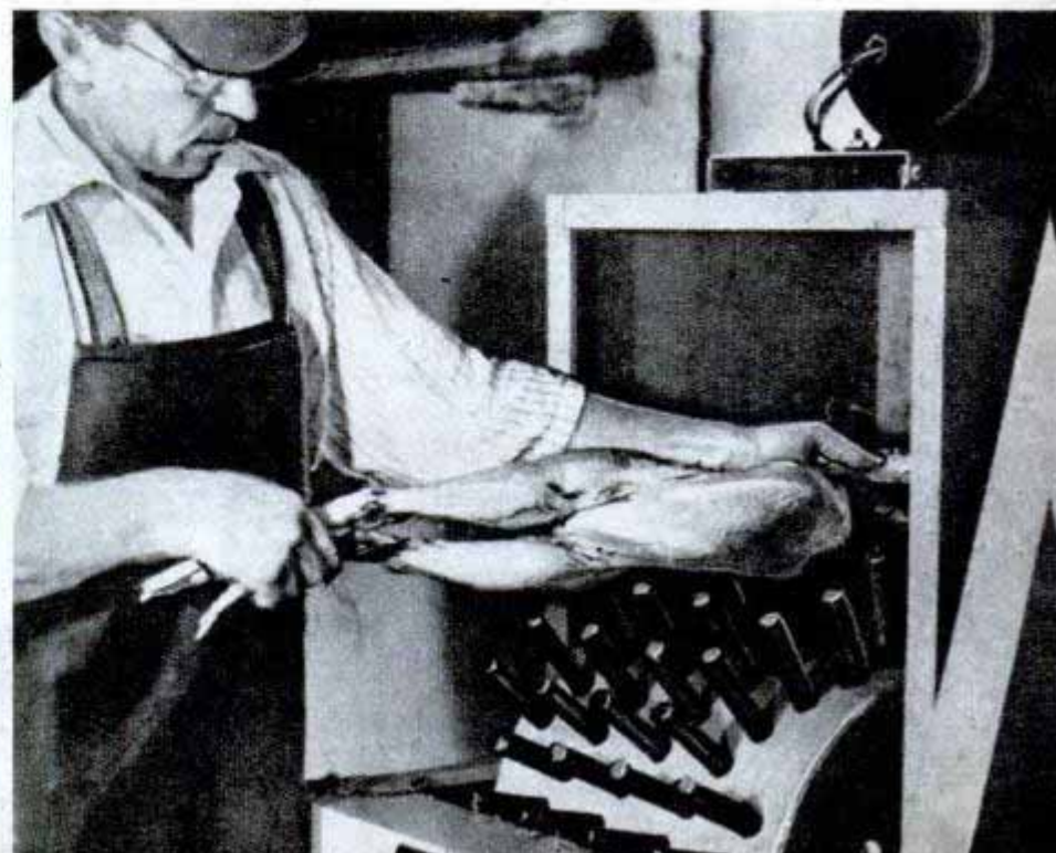
Float valves automatically regulate flow of water to troughs. Right, rubber-fingered mechanical feather picker
