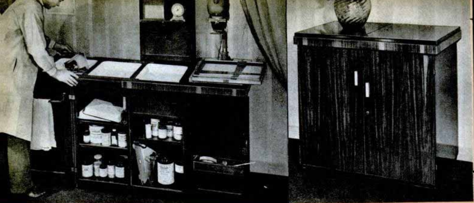
Photo darkroom becomes the decorative walnut cabinet shown at right when it's not in use. Doors and lid swing open to reveal shelves, enlarger, drain, timer, safelight and space for three trays
