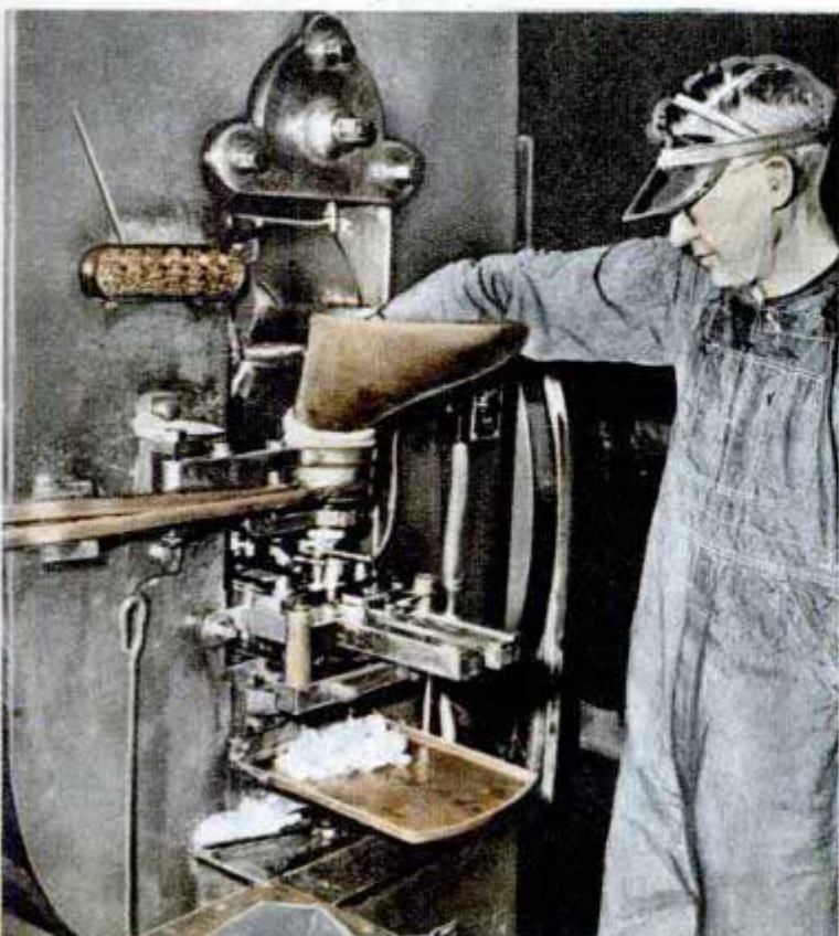
Weighing 5700 ounces of pure copper to be used in making one-cent pieces. Below, hopper in front of each press stacks coins and feeds them into place between dies, where designations are struck upon them
