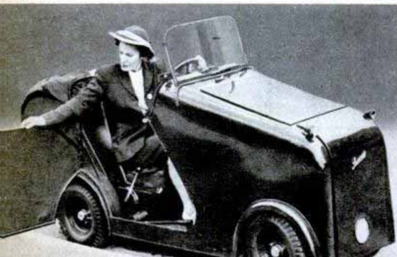
Runabout designed in London for disabled persons has interchangeable hand or foot controls. It gets 65 miles per gallon from 2½-hp. motor at speeds up to 40 m.p.h.
