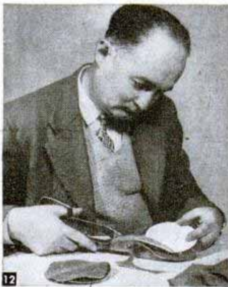
12 Using a cardboard template, disks are cut from "live" inner tube. Two rubber disks are required for each insulator
