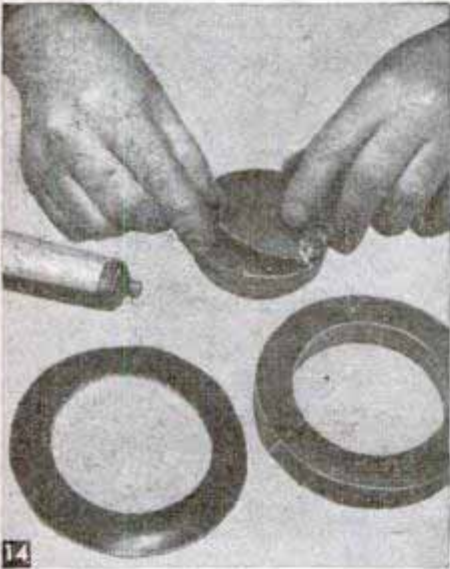
Where insulators are not bolted to machine bases rubber facings are cemented to both the disk and the ring
