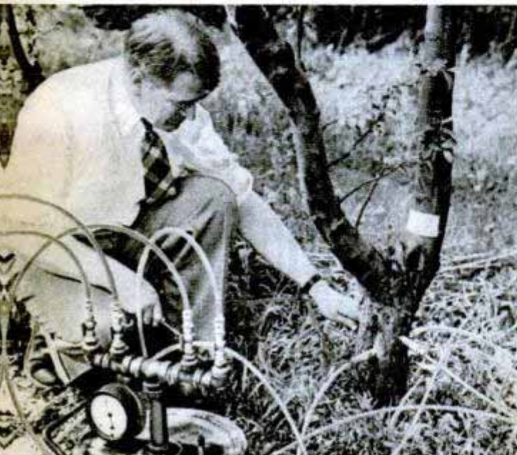
NEEDLES on this machine, developed by a Michigan State College horticulture expert, inject chemical nutrients and dissolved fertilizers into sick fruit trees
