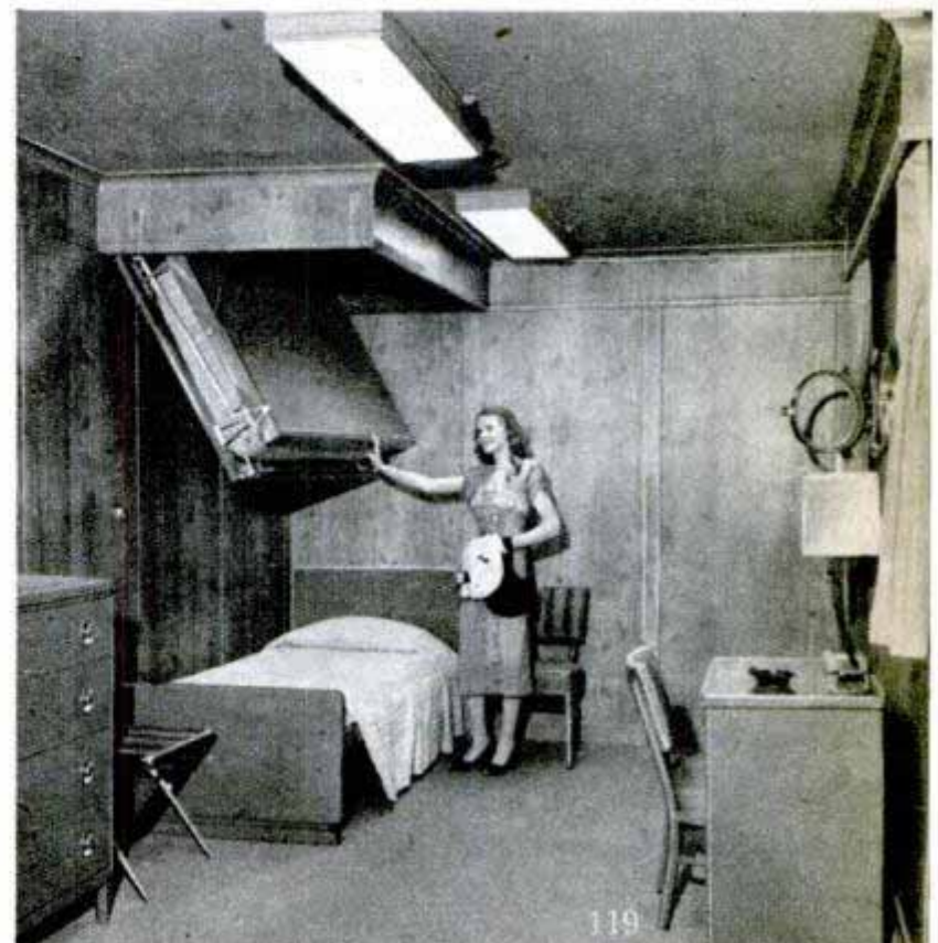
Upper berths in cabins of SS Amerita fold into ceiling, right. In another design, below, they fold into wall. During daytime, lower berths serve as sofas
