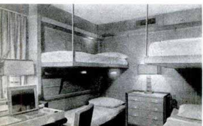
Upper berths in cabins of SS Amerita fold into ceiling, right. In another design, below, they fold into wall. During daytime, lower berths serve as sofas
