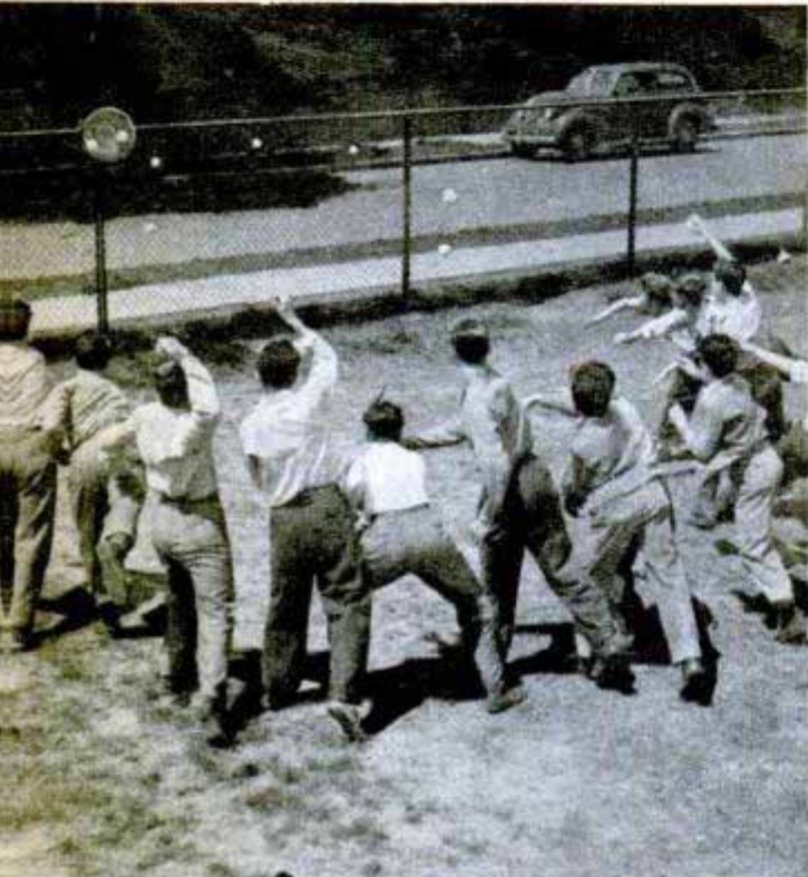
SANDLOTTERS try unsuccessfully to break the glass in one of the new GE floodlights at New York's Yankee Stadium. The "ballproof" glass is only \frac{1}{4} inch thick
