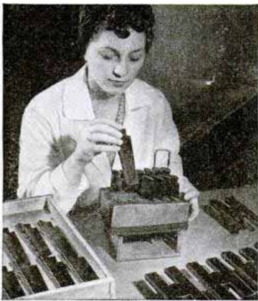
Model blades are cast in wax and mounted in holder. Below, assembly is surface-treated and covered with flask. Above right, flask filled with hardened cement is baked in oven to melt wax, leaving mold
