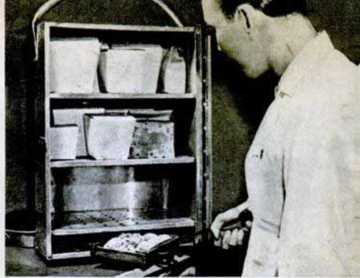
HOT BOX heated by charcoal in a pan at the bottom keeps food hot for three hours and is useful for delivering meals from restaurants or for picnics. Holes in the shelves permit heat to reach all the dishes
