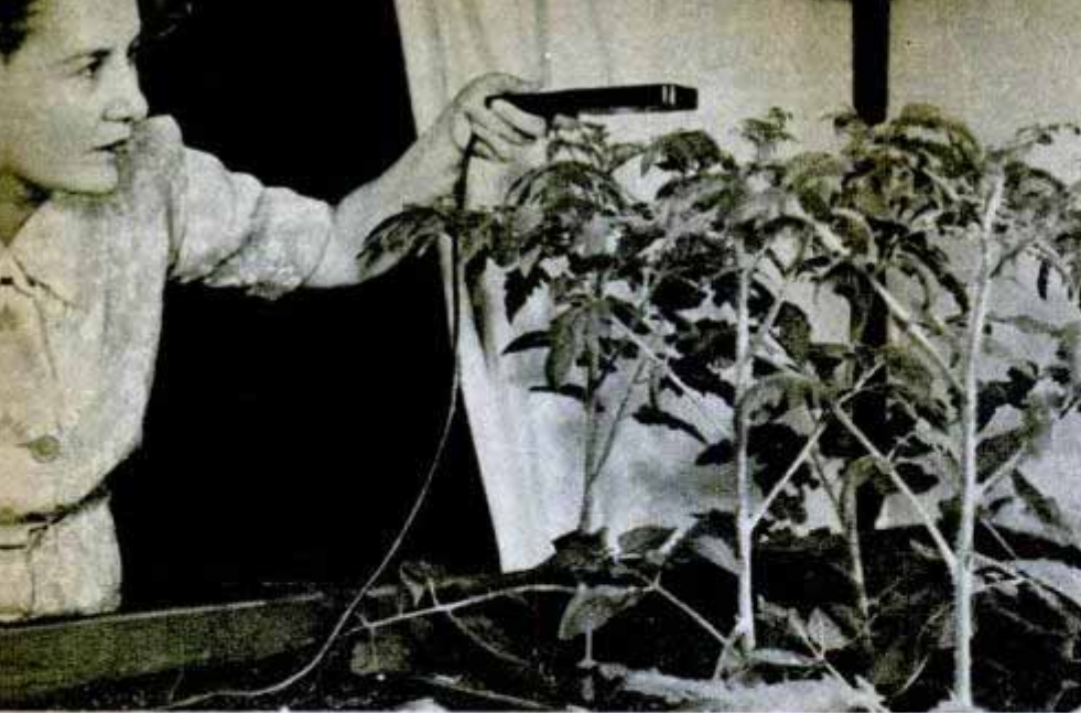
↑ Studies made by Mrs. Alice P. Withrow, research assistant at Purdue Agricultural Experiment Station, have revealed growing secrets. With meter she measures intensity of fluorescent light over test bed
