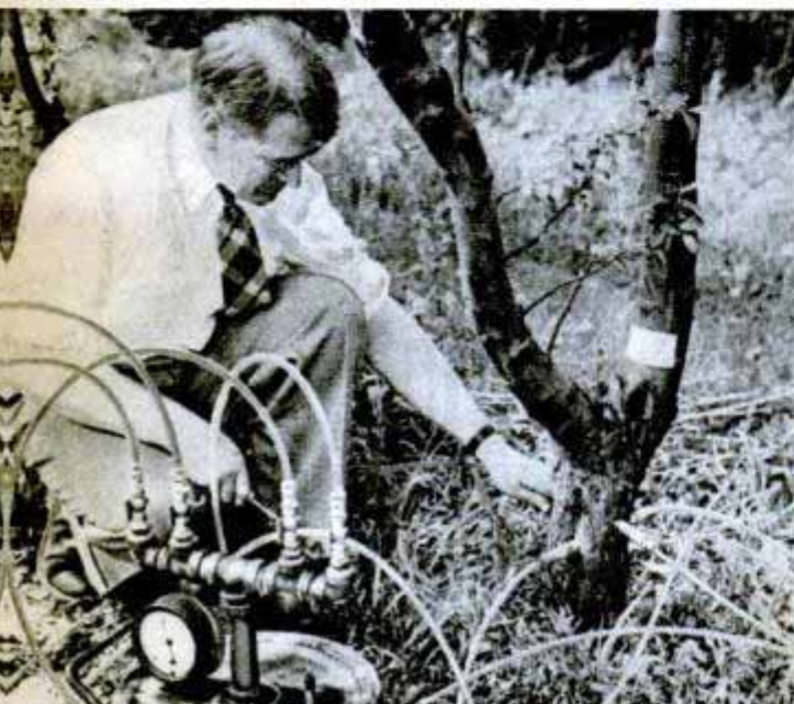
NEEDLES on this machine, developed by a Michigan State College horticulture expert, inject chemical nutrients and dissolved fertilizers into sick fruit trees
