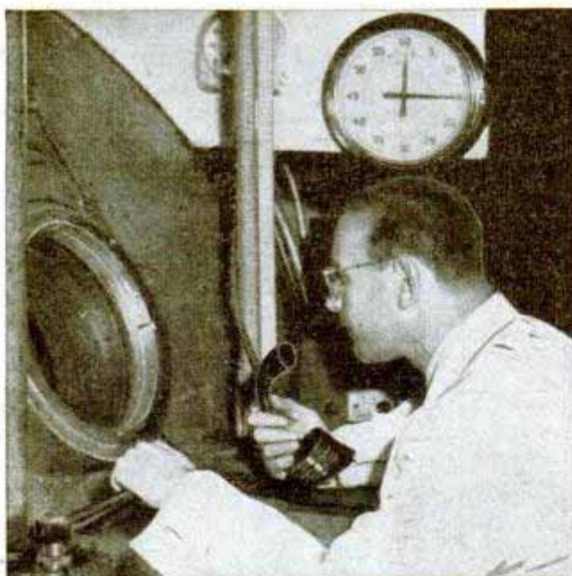
In this test an electric wire punctures a hole in paper panel to let air enter decompression chamber. Contact with the subject in the chamber is maintained by means of an intercommunication system.
