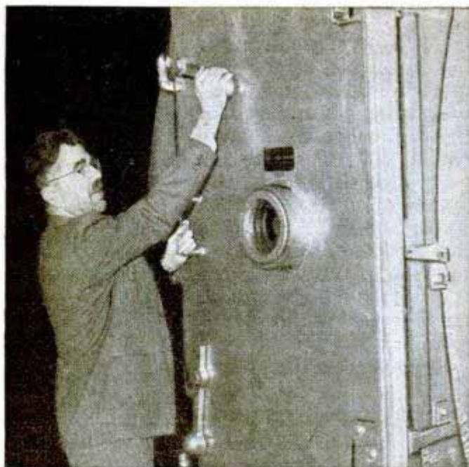
Dr. Fred Hitchcock of Ohio State University locks the heavy steel door of the decompression tank for a test. With a loud report, the panel is blown out and pressure in the two chambers rapidly becomes equalized.
