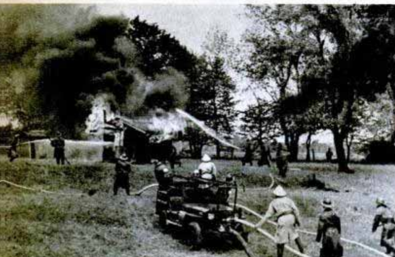
JEEP FIRE ENGINE , a dwarf compared to a regular size machine, is ideal for hurdling ditches and speeding across bumpy fields to combat fires in rural communities. Some industrial plants also use the modified war jeep to scoot through production aisles and hurriedly reach the scene of a fire or explosion. The fire jeep costs $2800
