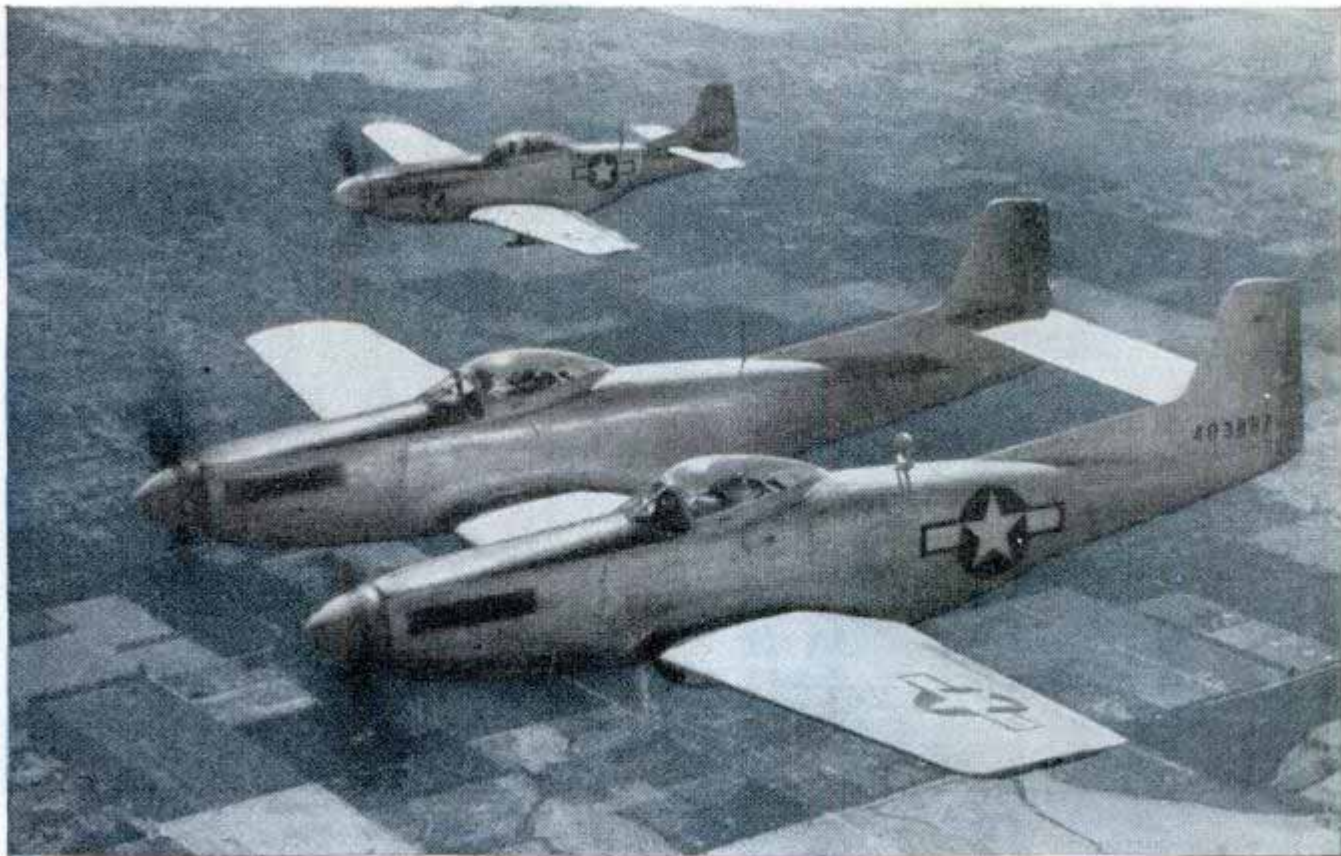
When AAF added P-51 to P-51 it came up with faster, more powerful twin, the P-82, above, In 500-m.p.h. twin-jet flying wing XP-79, below, pilot lies prone to avoid "blackout"
