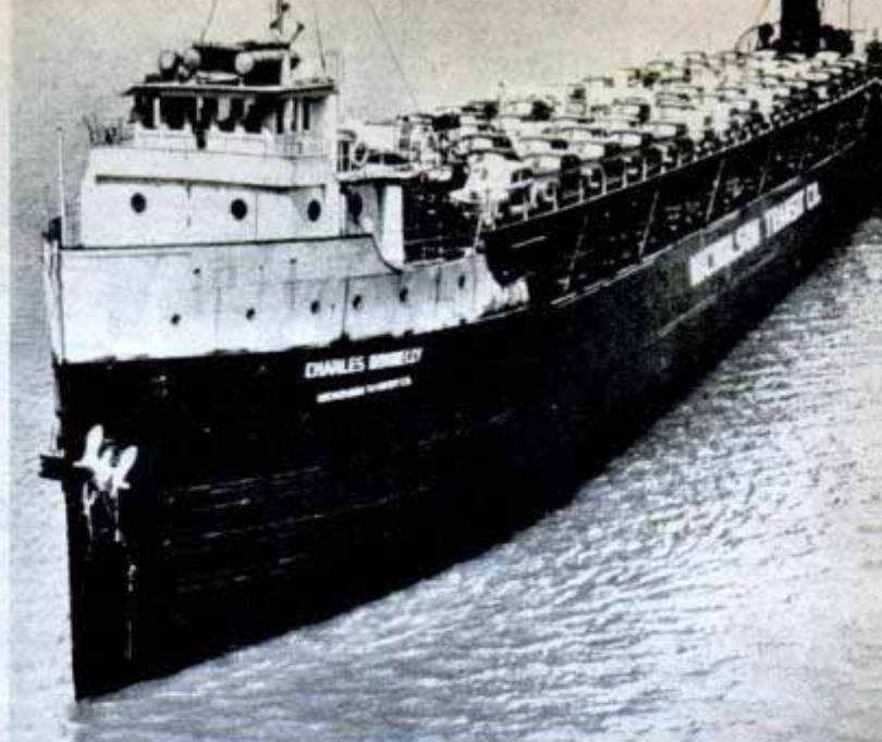
THIRD DECK installed on Great Lakes Steamer Charles Donnelly increases ship's auto-carrying capacity by 90 cars. Now 432 cars are transported on three decks
