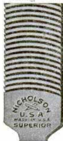
SUPER-SHEAR FILE with wide-spaced short-angle teeth at right for fast cutting; narrow-spaced, long-angle teeth at left for smoothing.
