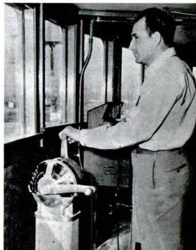
Portable switchbox in fisherman's hand controls a rugged electric motor on cargo boom. Right, wheelhouse governor permits remote control of main engine
