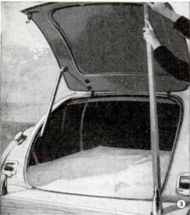
As a safety precaution, a wooden brace supports the rear-deck door. The base of the support is wedged tightly into the bumper guard
