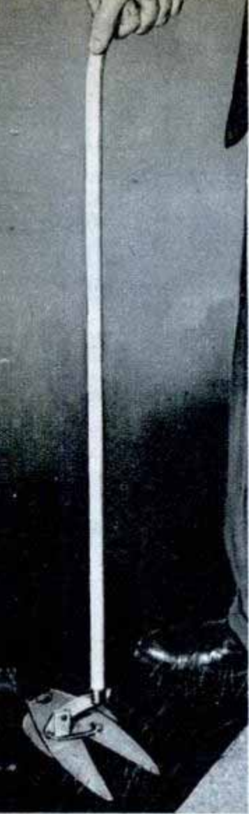
GRASS TRIMMER for tufts missed by mower operates by pushing down handle
