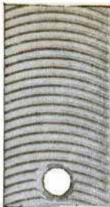
FLEXIBLE CURVED TOOTH FILE design — for use in special holder shown in picture at left.
