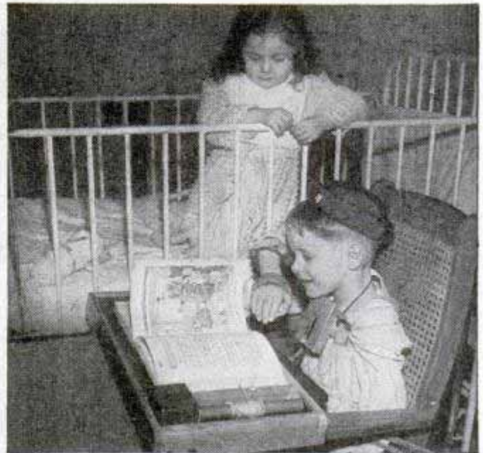
After nurse attaches thread to book pages, an automatic page turner enables incapacitated boy and woman in iron lung to read the books
