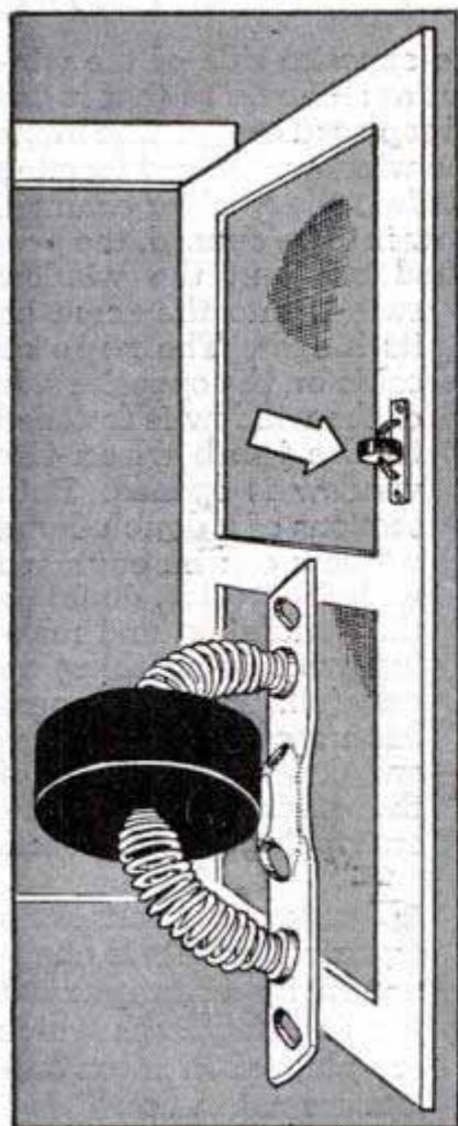
Snap-fasteners are "sewed" in place with hammer and U-shaped tool with hole for punch. Below, steel spring and rubber wheel muffle closing of a screen door
