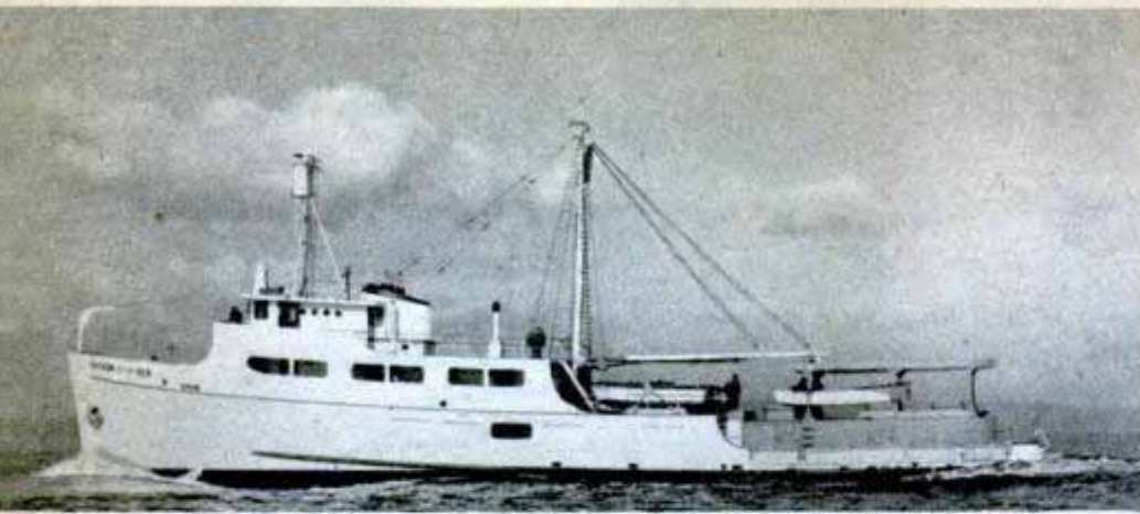
Complex tuna clippers like this modern ship can range far from home port and quick-freeze as much as 500 tons of fish during each trip Courtesy Van Camp Sea Food Co.
