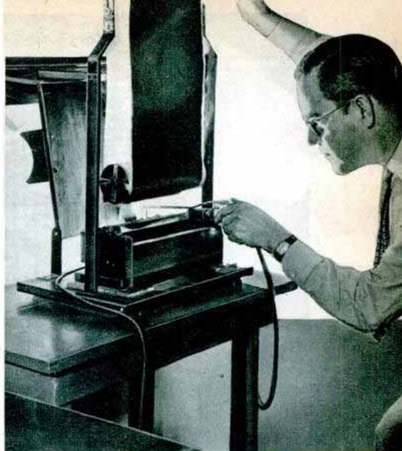
Applying lamp black (above) to paper roll for use in a seismograph. Below, essential parts of a home-made seismograph which will trace earthquakes
