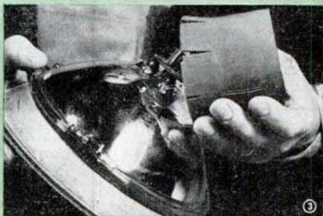
Slitted piece of radiator hose provides pressure to keep the sealed-beam unit in place
