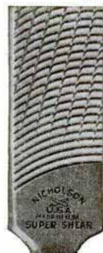
SUPER-SHEAR FILE with wide-spaced short-angle teeth at right for fast cutting; narrow-spaced, long-angle teeth at left for smoothing.
