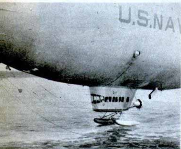
SEAGOING NAVY BLIMP is equipped with rubber pontoons for water landings. After coming to rest, the craft can be moored by throwing out a sea anchor
