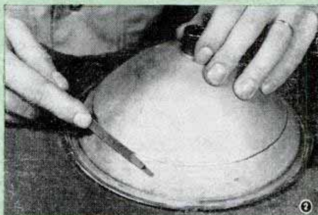
After rechecking diameter marked, reflector is cut through with a three-cornered file
