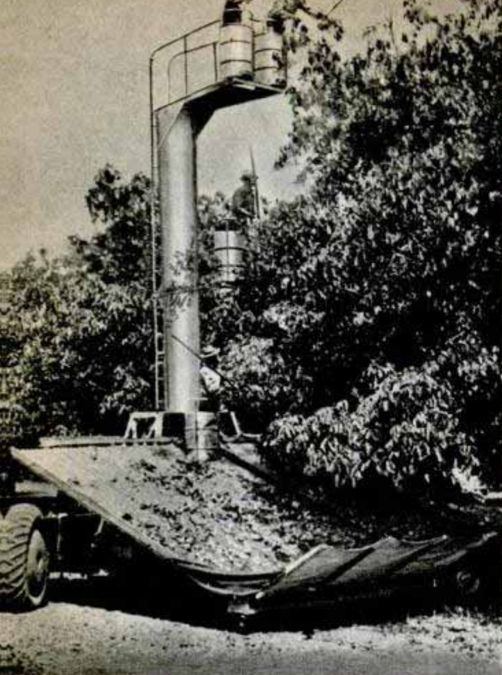
WALNUT HARVESTER has steel and canvas apron which catches nuts knocked down by men on attached towers
