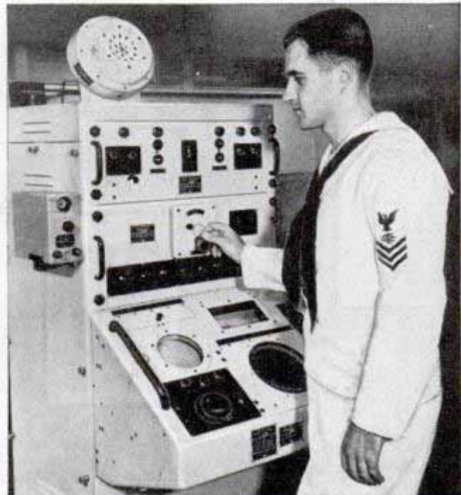
Sonar control “stack” guides beam, listens for echo
