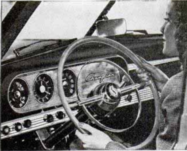
Nonglare black light illuminates jumbo-sized dials on dash of new Studebaker. Below, arrow points to plug on self-adjusting brake shoe described in text
