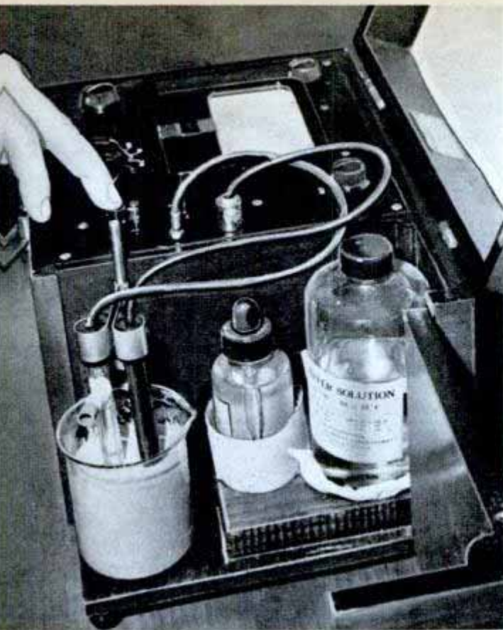
Left, testing for acidity or alkalinity of the fluid. Right, tank drips chemicals into the mud circulation system
