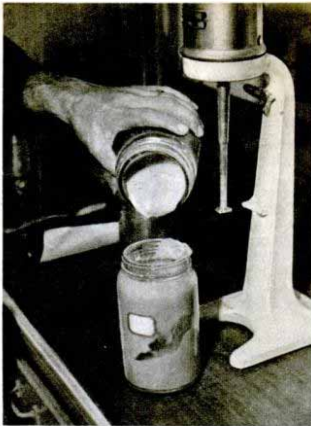
Colloidal material picked up in the underground bore has thickened this mud (left). The mud engineer can reduce its viscosity by adding a few drops of complex or poly phosphates to the sample as shown at right
