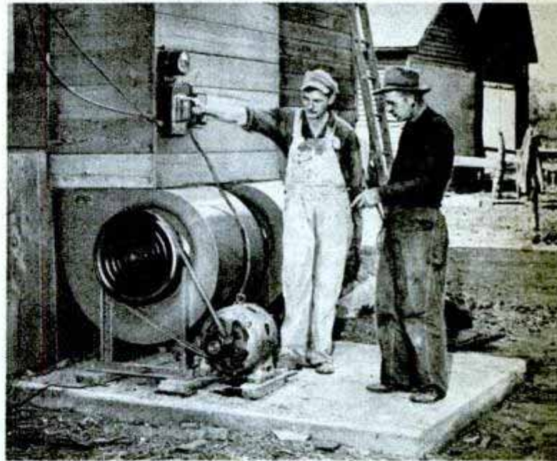
Electric blower forces air through ducts to cure hay in mow. Below, electric clippers shear sheep
