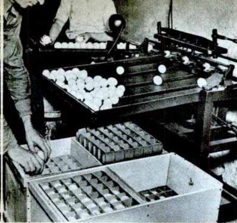
Eight cases of eggs per hour are graded by machine
