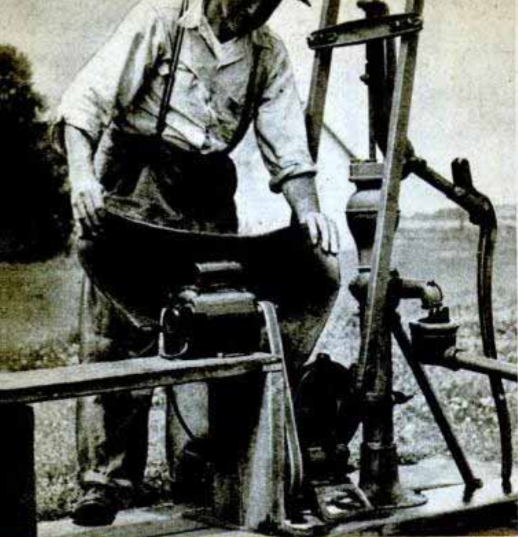
Public Service Co. of Northern Illinois photo Unlike a windmill which works only when the wind is blowing, electric motor pumps water at any time
