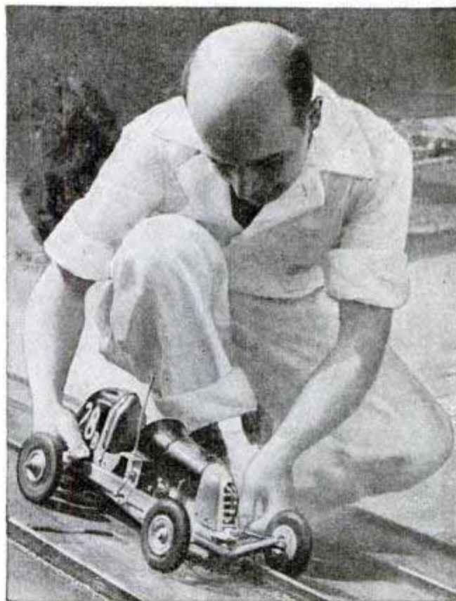
↑ An impatient car is fastened securely to the rail ↓ Note ball bearing locking studs on the front axle
