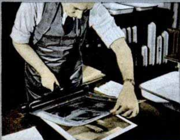
5—Dyes are transferred to the paper with a special roller
