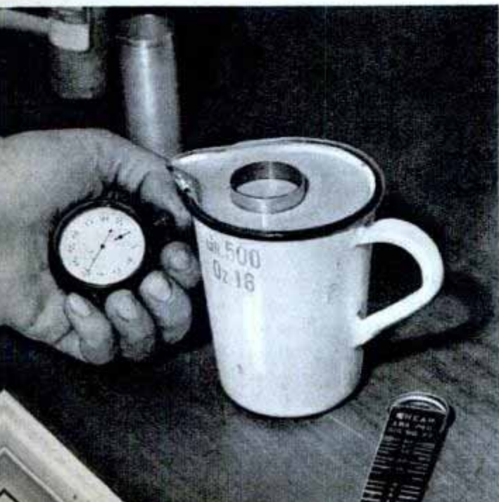
Left, mud's “gel” strength is checked by timing the sinking of an aluminum tube in a sample. Right, mud engineer tests under pressure the water-retaining property and cake-building rate of four samples of fluid
