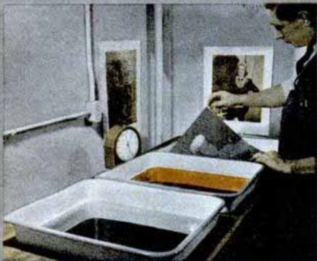
3—Inherent colors are added to the films in pans of dye
