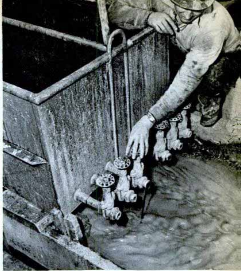
Left, testing for acidity or alkalinity of the fluid. Right, tank drips chemicals into the mud circulation system
