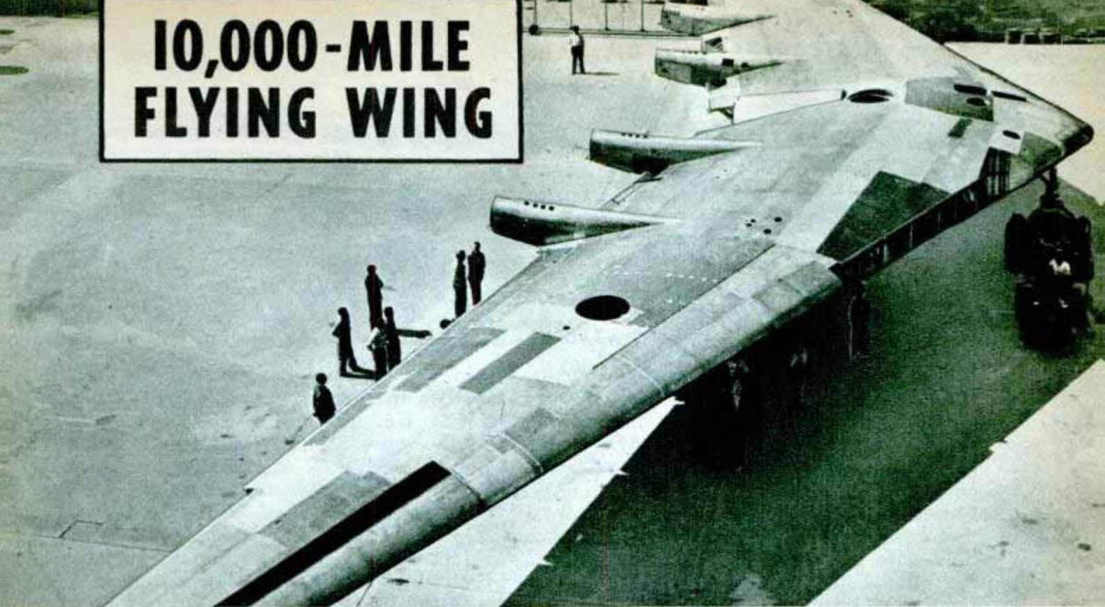
Side and rear views of 104½-ton XB-35. Diameter of the contrarotating propeller is 15 feet four inches
