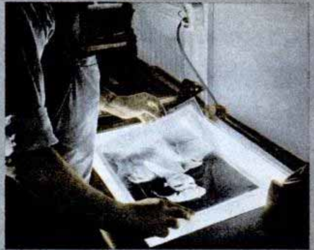
2—The matrices are registered in position, then trimmed
