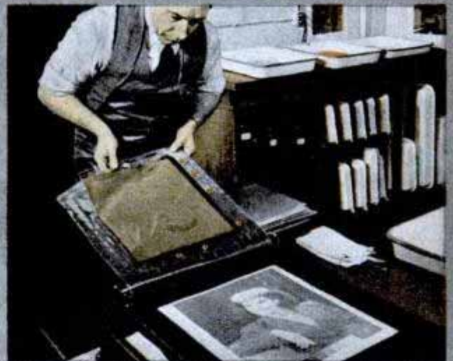
4—"Buttons" on the blanket re-register films for printing
