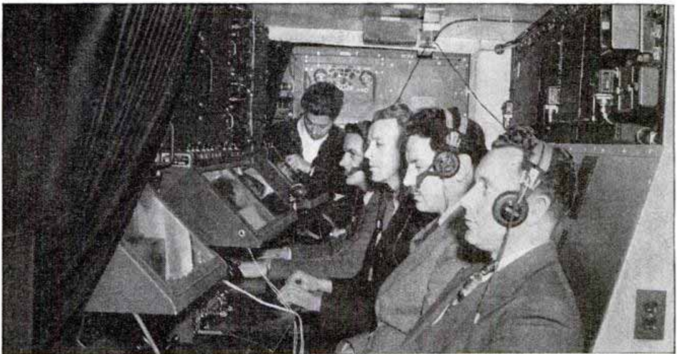
Interior of a GCA trailer, showing positions of five operators. Elevation indicator station is in foreground, final controller next, then the azimuth indicator post, with the two search scope watchers farthest from the camera
