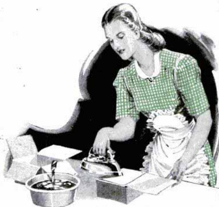
A moderately hot household iron, applied for a few seconds, will seal "bag-in-carton" containers. Cellophane bags may be sealed with a curling iron, taking care not to burn them
