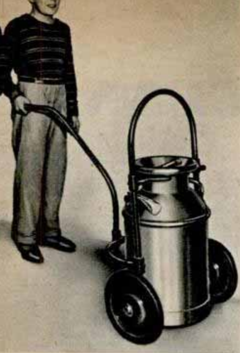
Rubber tired cart, above left, is equipped with hooks which fit under the collar of a milk can for easy handling of the heavy containers. Adjustable collar hooks fit any can, holding it in an upright position. At right, a home-built, labor and time-saving walnut tree shaker built by a California rancher is powered by a Diesel tractor
