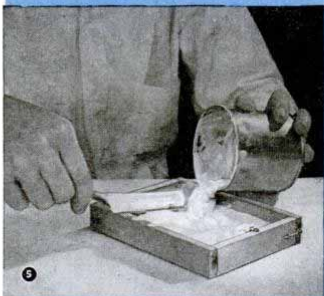
5 Place the mold back in the frame, oil the surface and once again pour the mold full of plaster of paris
