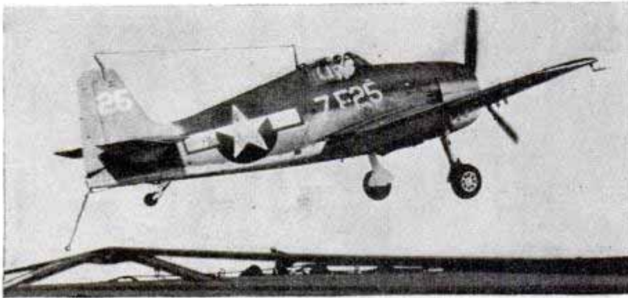
An F6F-3 is about to hook arresting gear cable five inches above deck
