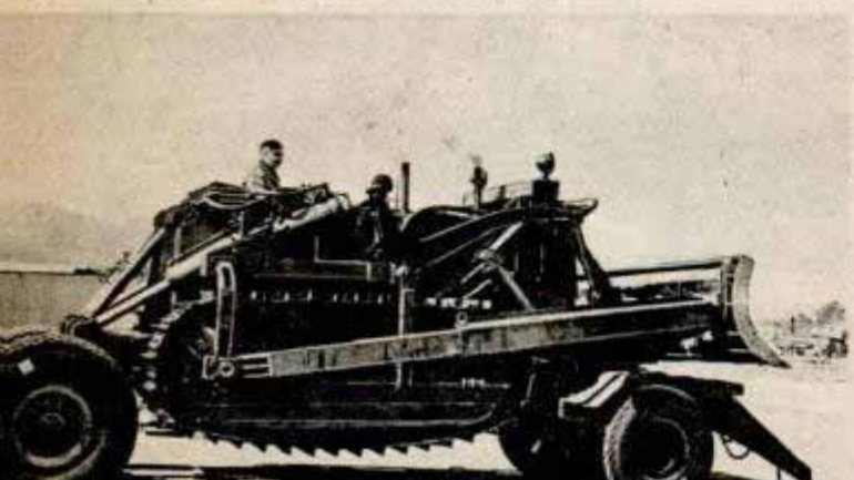
Below left, built-in hydraulic jacks lift this combination tractor and bulldozer on to its own rubber tired wheels for high-speed transportation. Right, Hollanders make rafts of biscuit cans that were dropped from planes by the Allies to relieve the food shortage. The rafts are used to navigate the canals of Rotterdam
