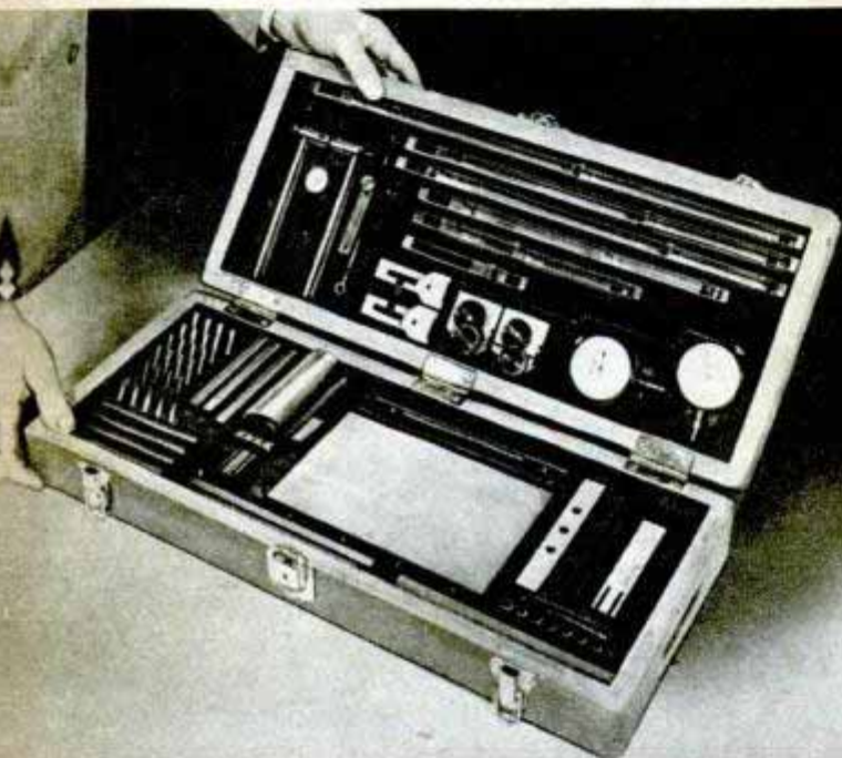
GAUGES for a thousand precision checking jobs are made up from instruments packed in case 20 inches long. They are used in conjunction with gauge blocks
