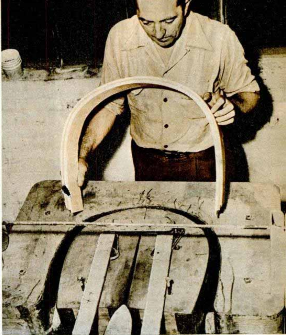
This plywood shape for an article of furniture was molded in only two minutes by high-frequency heat. Below, engineer inspects machine that generates heat in dielectric substances by beaming waves of energy in the radio spectrum
