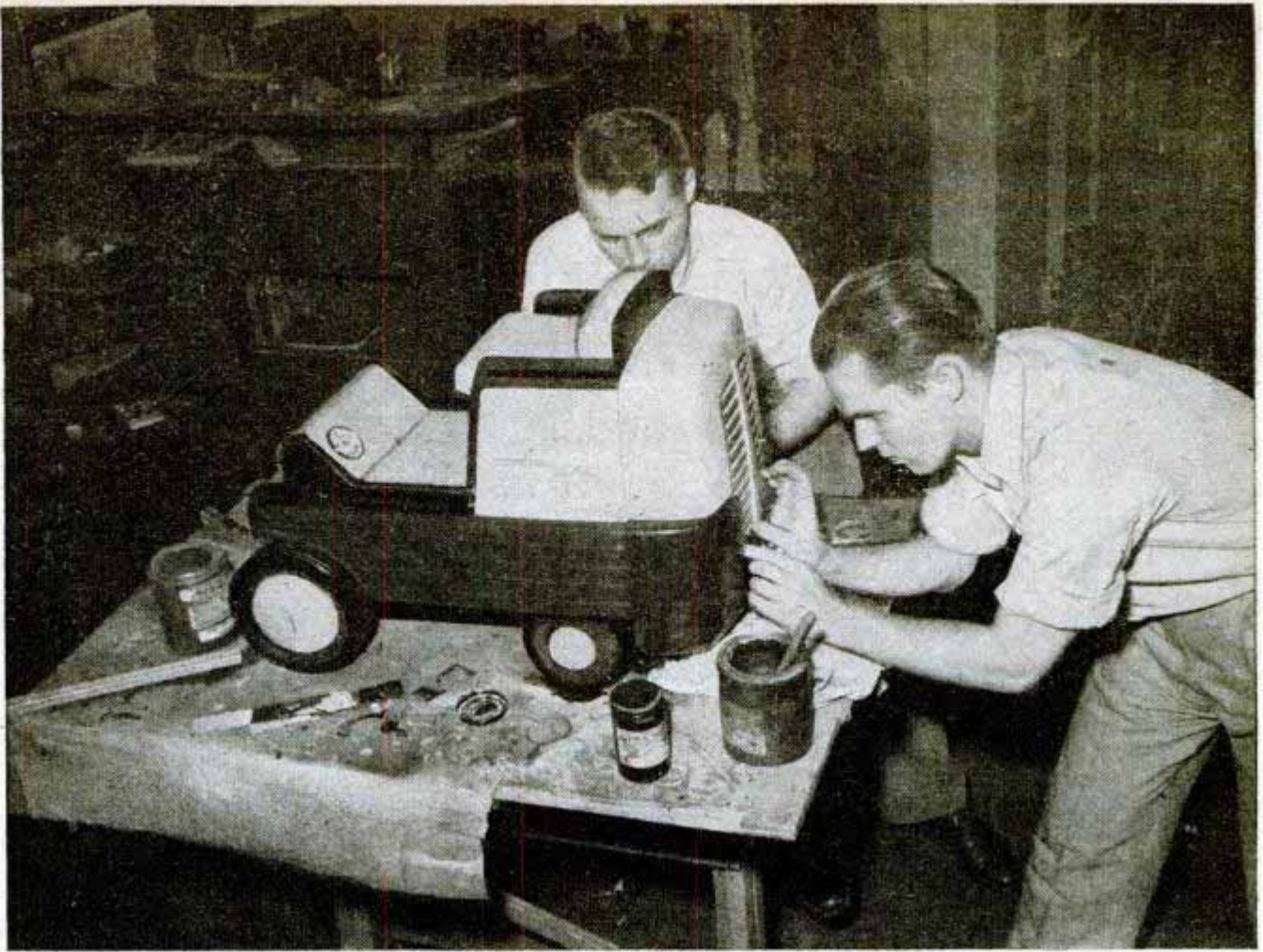
Wooden model (above) receives final touches from associates of Dave Chapman, Chicago designer, as guide for industrial truck below
