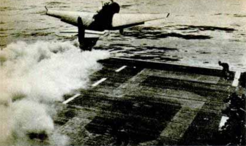
Catapulted by JATO (Jet Assisted Takeoff), Avenger wings its way from a carrier deck out over the Pacific
