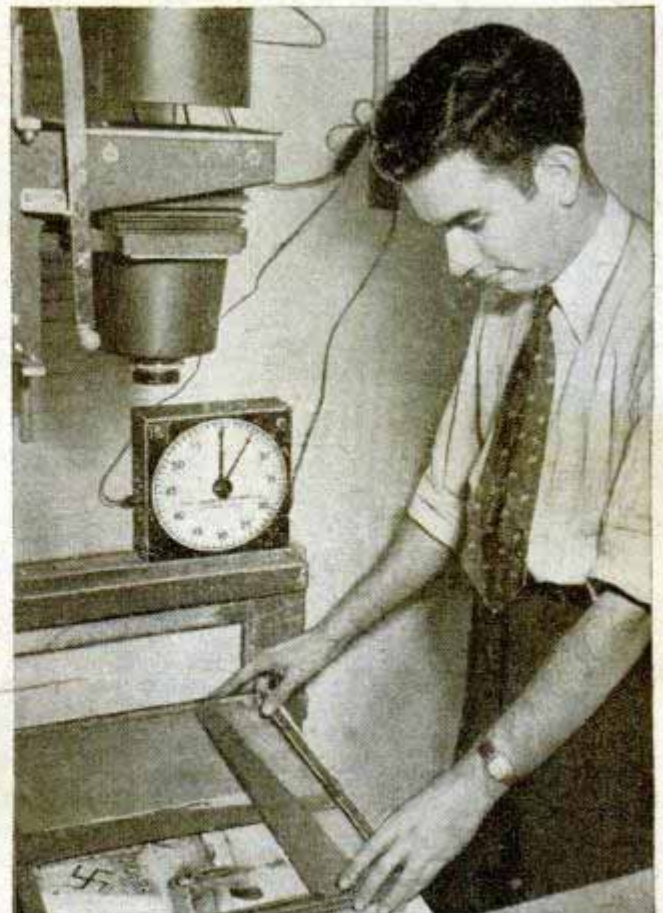
NEW TIMER automatically controls "on" and "off" timing when plugged into developing, printing, enlarging or photoengraving equipment. It has eight-inch dial and operates on 110-volt, 60-cycle current
