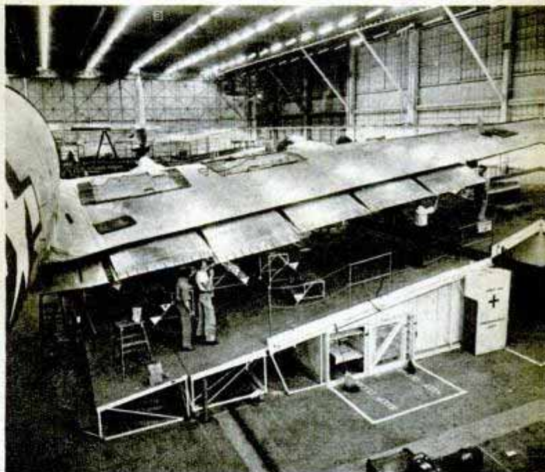
INCLINED FLOORS provide workers with plenty of room to install ailerons, wing flaps and other subassemblies in the wings of giant Lockheed Constellations
