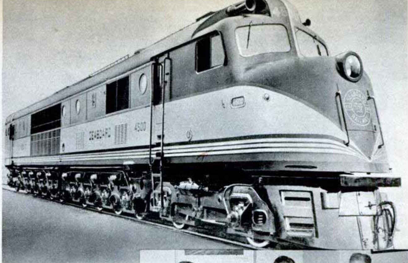
Most powerful single-unit Diesel engine built by Baldwin Locomotive Works for Seaboard Air Line Railway develops 3000 horsepower
