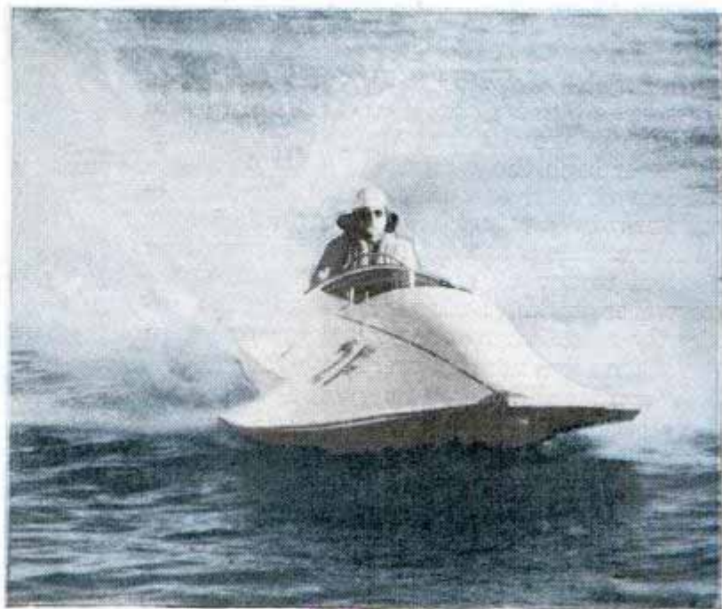
The radical hull of this hydroplane was designed to lift boat almost free of water. The boat below broke record with speed of 77 plus m.p.h.
