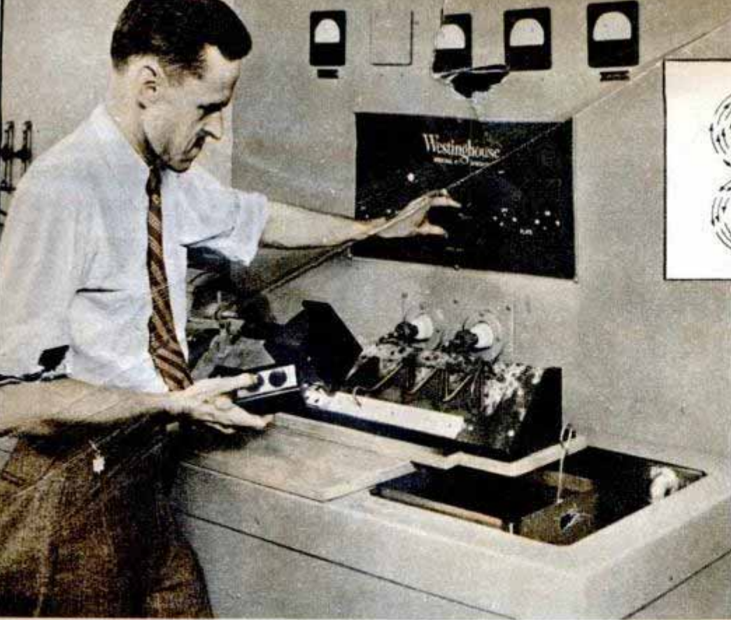
INDUCTION HEATING: Agricultural mower blades are hardened electronically. The sketch shows work in the magnetic field that is created by current in an induction coil
