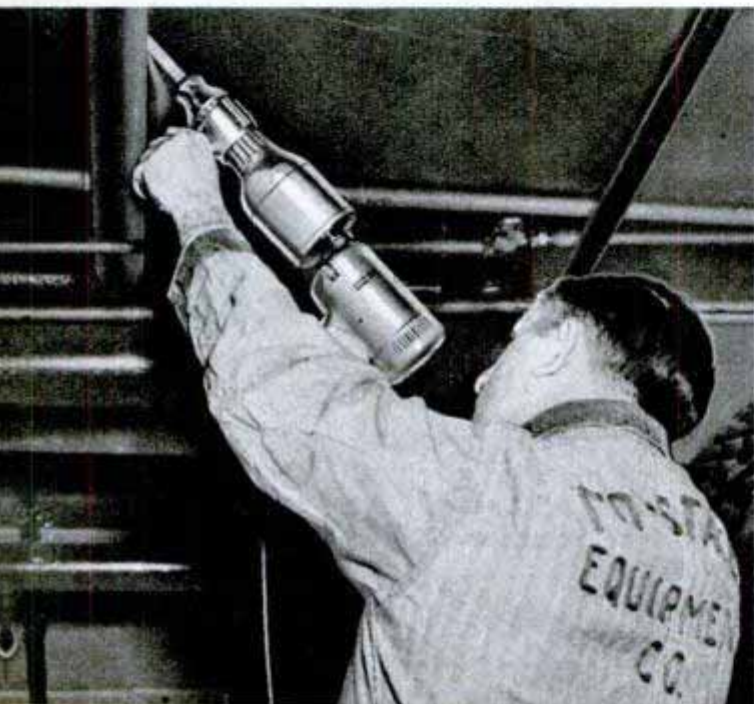
THREE KINDS OF POWER , electricity, compressed air or a flexible shaft, will drive a handy tool for sawing and filing that will reach into awkward corners
