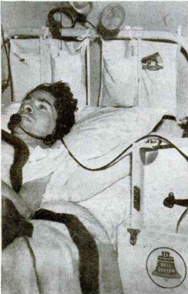
UNIQUE BED TELEPHONE was developed for use of Army veterans unable to use their arms. Both receiver and mouthpiece are supported without manual aid
