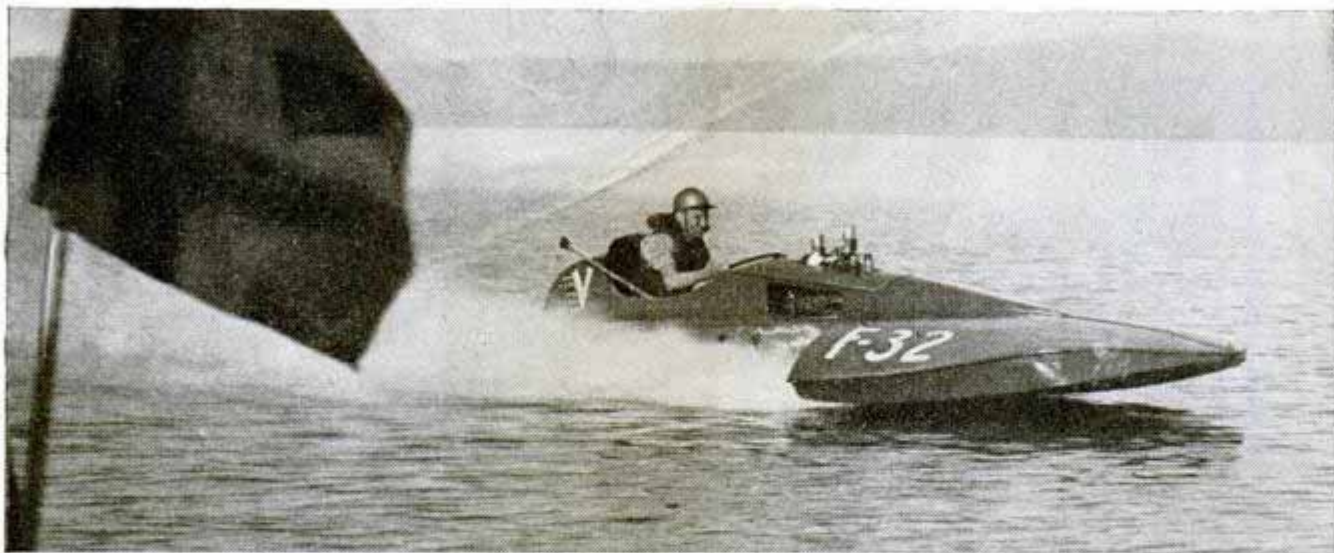
Three-point hydroplane teeters between bow sponsons on either side as speed lifts the craft from the water
