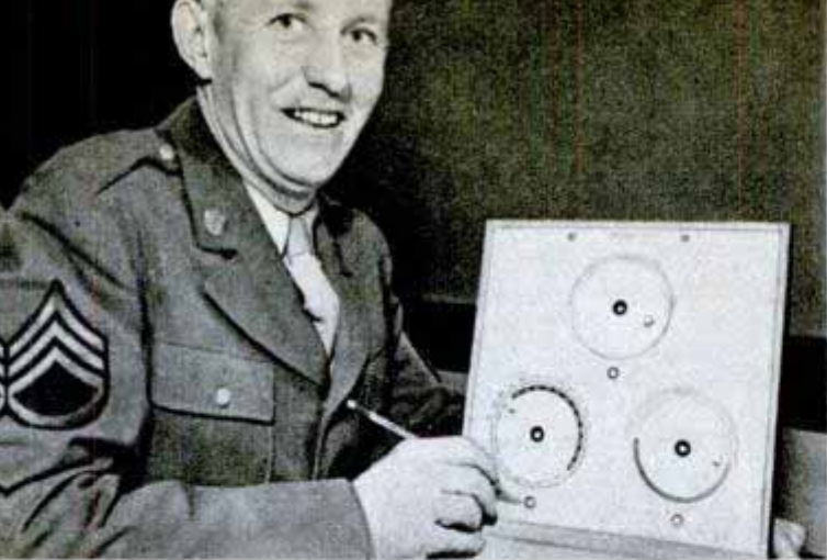
COMPUTING MACHINE invented by Sgt. James T. Patterson figures years, months and days of service to aid soldiers in totaling up their "points" for discharge
