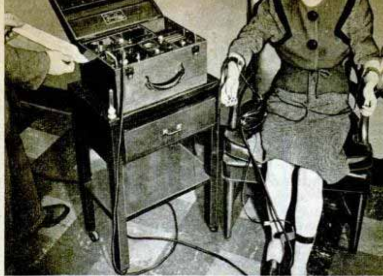
DIRECT-WRITING ELECTROCARDIOGRAPH records patient's heart action as it "listens," eliminating photographic procedure required with former machines. New instrument magnifies heart action about 14,000 times
