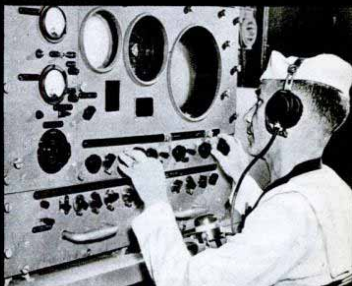
PPI at right shows objects picked up; beam rises in A-scope at left to a peak when the echo comes back
