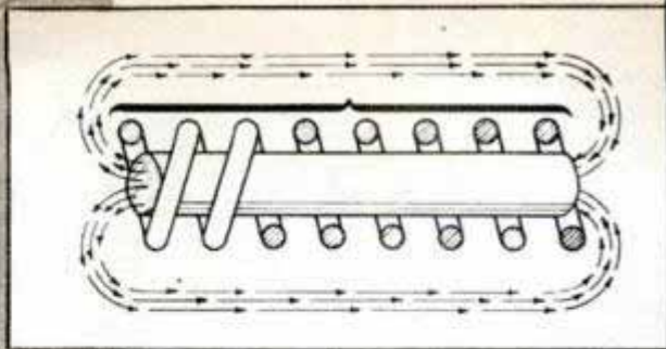
INDUCTION HEATING: Agricultural mower blades are hardened electronically. The sketch shows work in the magnetic field that is created by current in an induction coil
