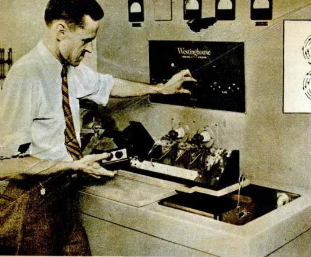
INDUCTION HEATING: Agricultural mower blades are hardened electronically. The sketch shows work in the magnetic field that is created by current in an induction coil
