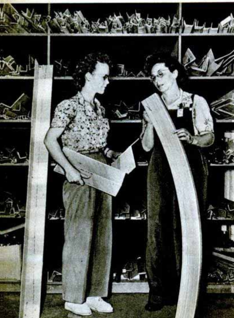
Glue in wood table top is cured in two minutes in a high-frequency heating jig. Below, these curved plywood beams were bonded by radio heat for use in building the giant Hughes flying boat
