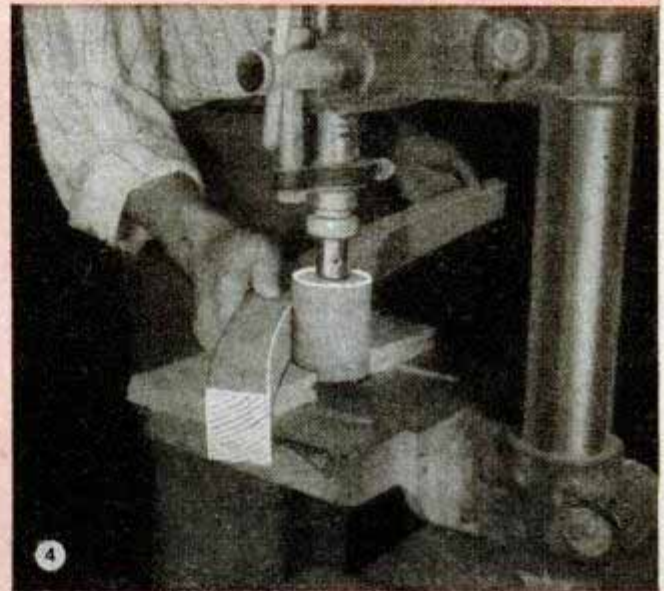
4 A small sanding drum mounted in the drill press is just the thing for smoothing the curved surfaces of the rough-sawed legs and rails to finish size
