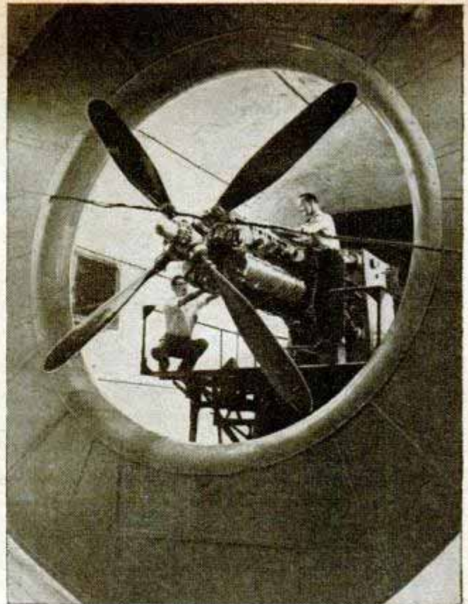
MORE POWER than from other engines of similar displacement is reported developed by this 16-cylinder inverted V-type engine built by Chrysler for the AAF. Liquid cooled, the engine develops 2500 horsepower
