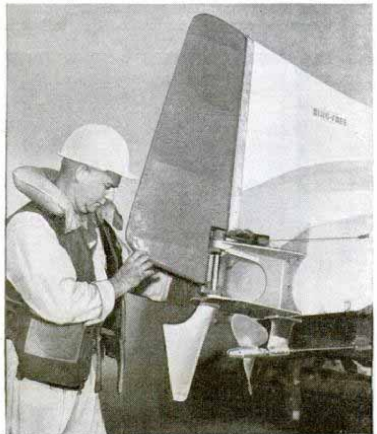
Racers watch the flag as they cross the starting line. Inside the long tube below the starter is an electric eye for timing the race. Below, an aircraft-type rudder works with the water rudder in controlling the boat
