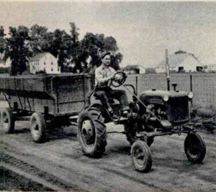
"CUB" TRACTOR weighing 1050 pounds (two thirds weight of previous small tractors) is capable of plowing three acres in 10 hours. Driven by a four-cylinder, 10-horsepower engine, it has three speeds forward
