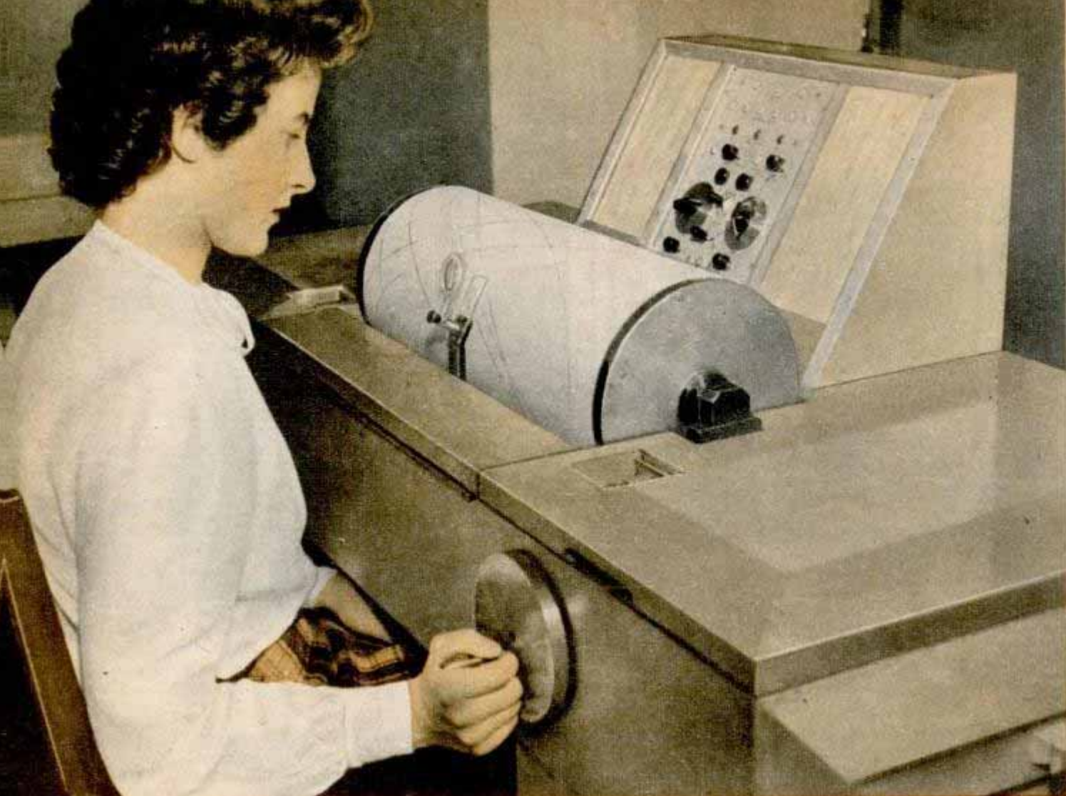
Input table of the electromechanical differential analyzer where the operator "presents" the problem in graphic form to the machine. Below, maze of more than 200 miles of wiring connects machine's 150 motors
