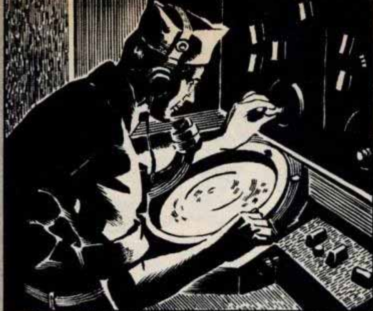
3 Small blob of light appearing on PPI scope gives interceptor officer warning of bogey
