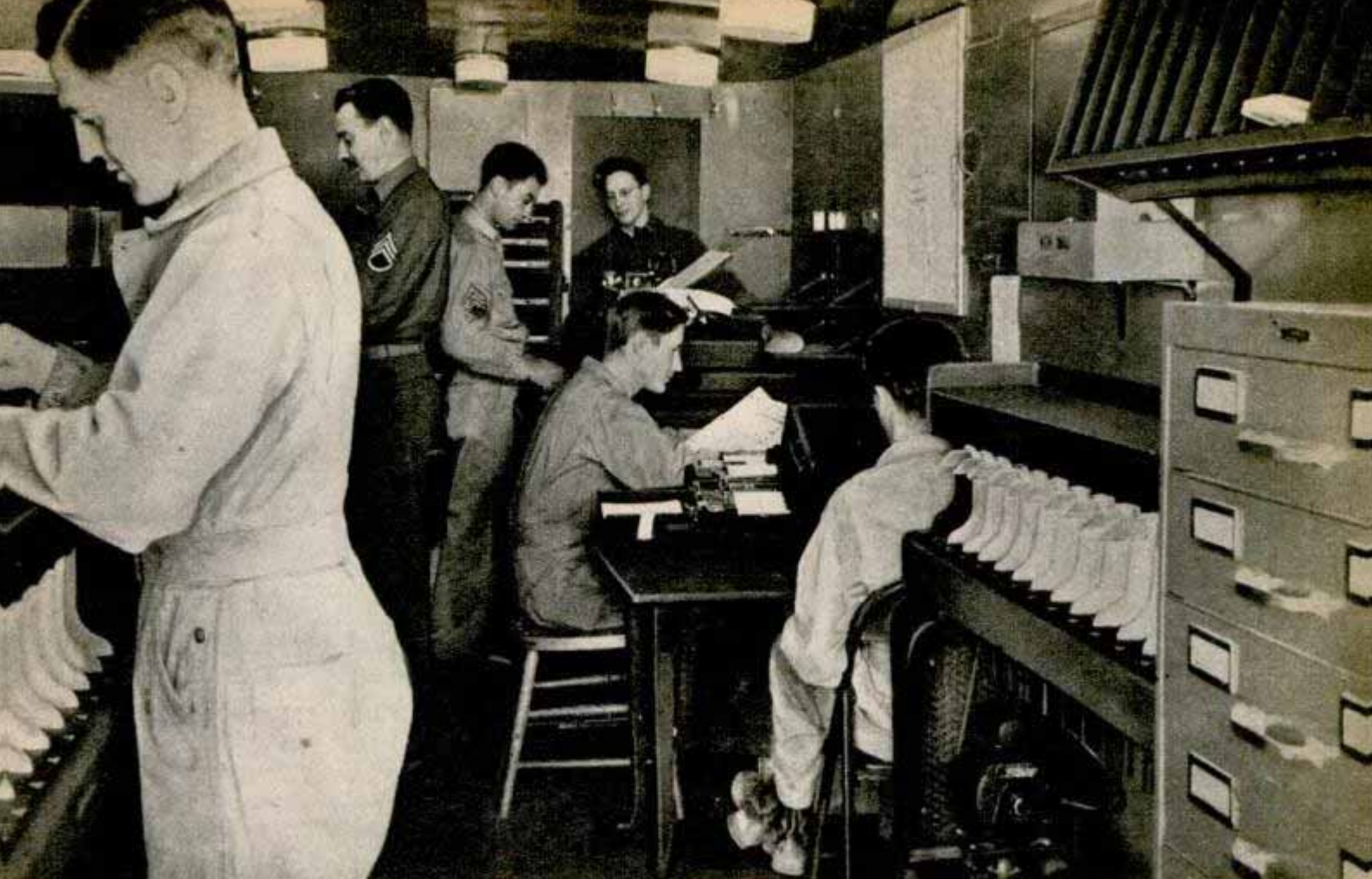
Interior of an Army machine records unit trailer showing two sorters, printing punch and reproducing machine
