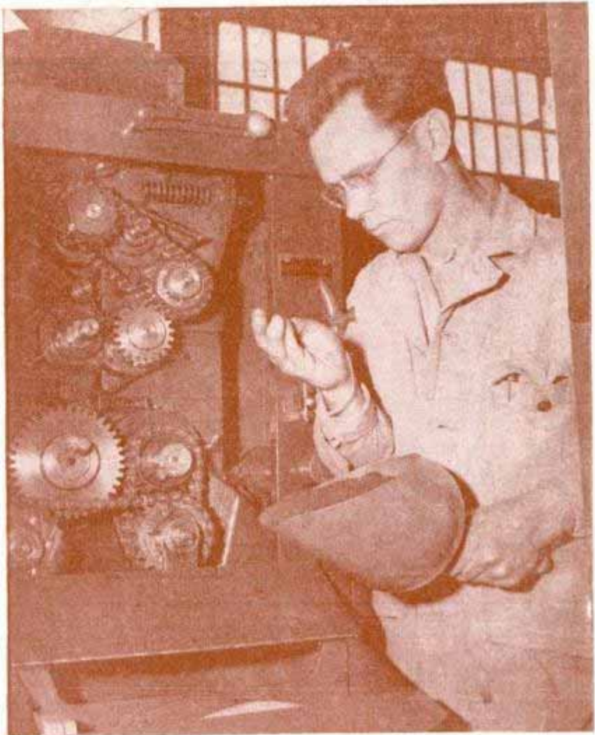
Inspecting the "grind" of coffee coming from an Army roller mill. Below, roaster's heating unit was improvised from gasoline drum Signal Corps photo
