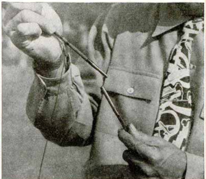
↑ Screw reel seat with duralumin fittings holds reel securely. ↓ Ferrules should fit snugly with sufficient length for long wear
