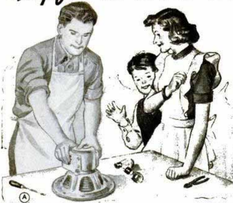
(C) Voice coil centering is checked easily by pressing on the cone rim as illustrated and listening for rubbing sounds; often scraping on the pole pieces is felt through the fingers. This is a common cause of distortion and indicates a recentering operation
