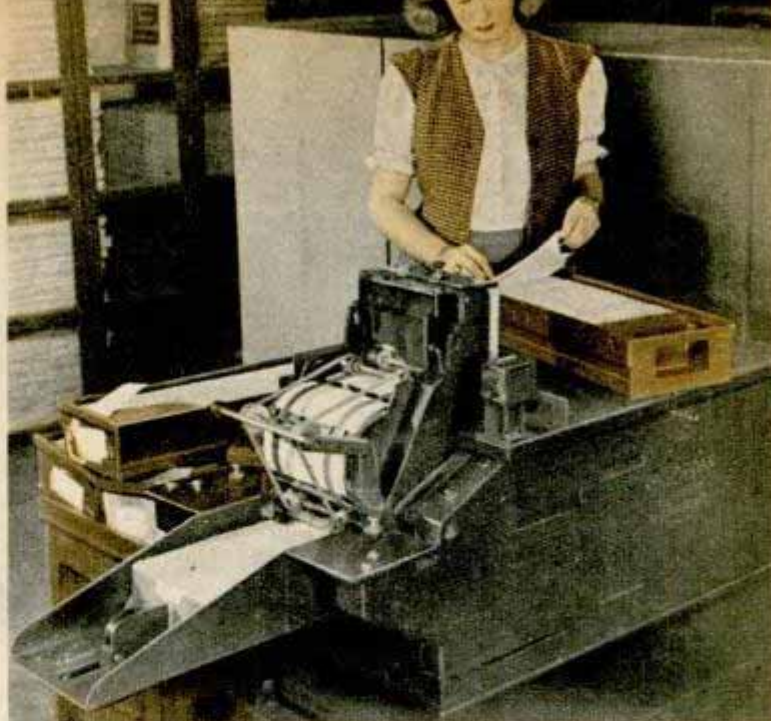
Above, microfilm camera photographs 400 cards per minute. Below, automatic punch reproducing machine
