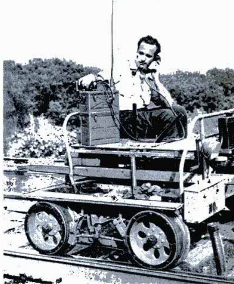
When lines are down, radio "patching" solves communication problem. Left, operator of portable transmitter-receiver spans gap in telephone line by putting signals on the air. At other end of gap similar unit receives message which is put back on wire. Right, testing walkie-talkie for use on handcar to keep repairmen informed of approaching trains. Below, cutaway drawing shows layout of Rock Island's rolling radio laboratory
