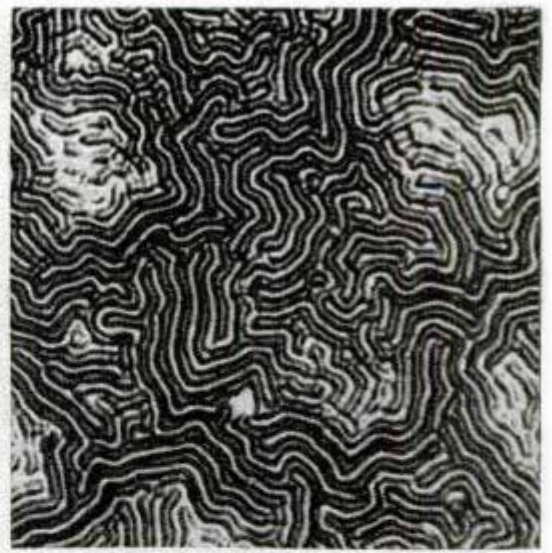
Resembling ripples in water, these circles are tool marks on metal faced on a lathe. Right, wrinkled enamel
