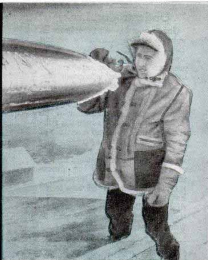
Inspector braves icy gale atop Mt. Washington, N. H., to get valuable data on rime formation on test wing. White rime ice forms rough deposits upsetting aerodynamics. It also plays havoc with radio towers (below) and forms "beads" which rotate on the cables
