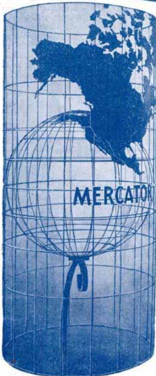
Relationship between azimuthal equidistant projection and a globe made to the same scale is demonstrated above. Similar comparison (left) between Mercator projection and a wire globe
