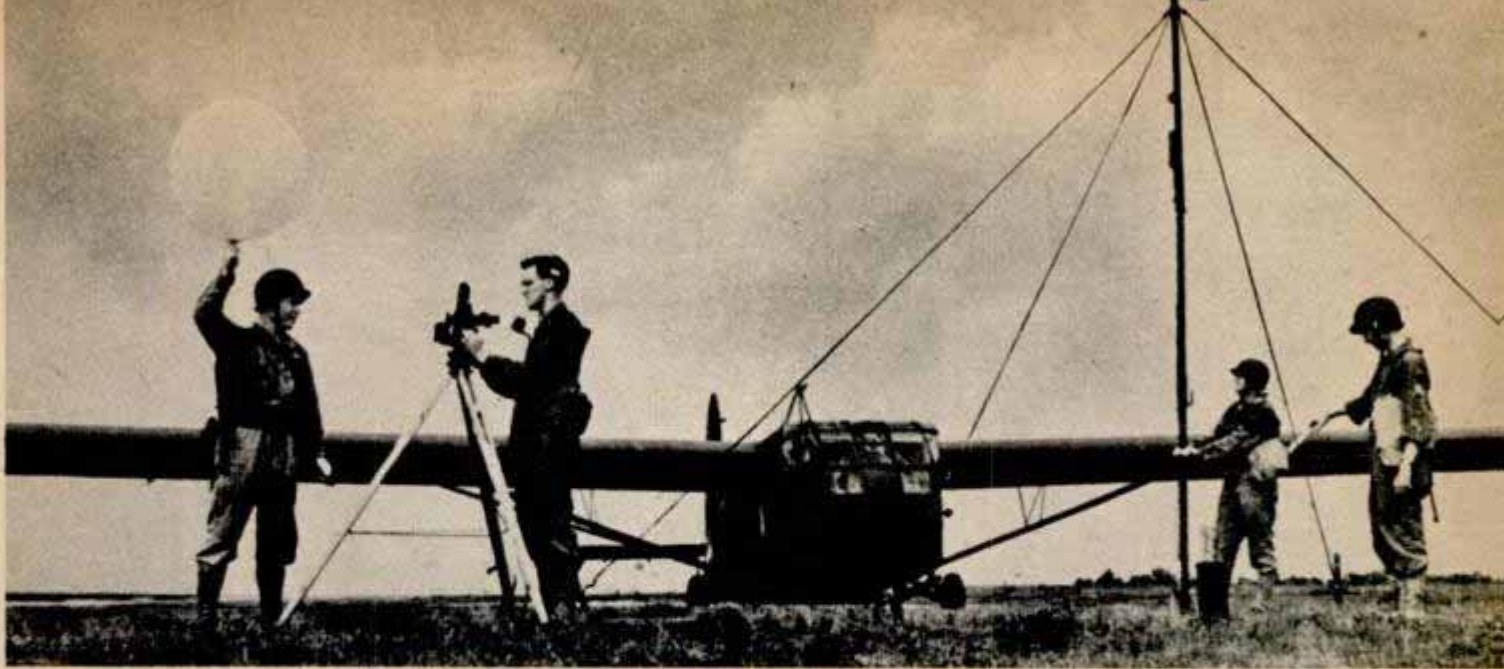
Army glider unit sets up airborne weather station; wind vane is at right, theodolite and balloon at left
