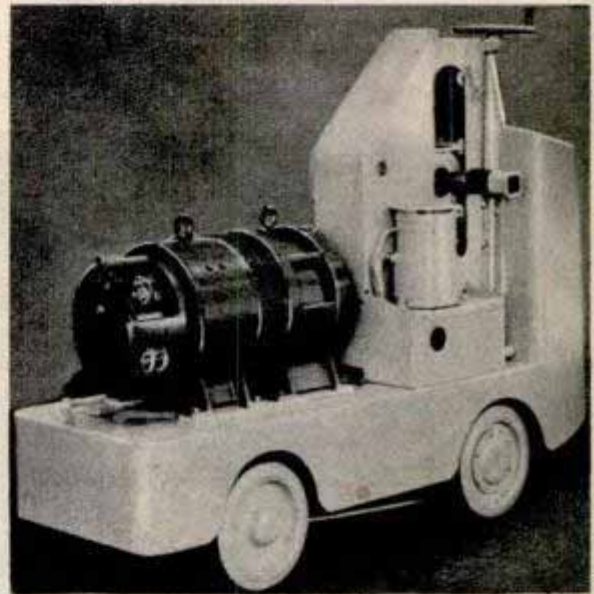
PLUG-IN ELECTRIC TRUCKS speed up the job of unloading hopper cars filled with iron ore. Powered by electricity from outlets along railroad docks, the trucks' motors turn four-foot-long wrenches which open and close bottom gates of hopper cars. One operator can do the job now in a fraction of the time previously required for two men to wield a 55-pound wrench. The truck has three-phase, 220-volt AC motor connected with a generator
