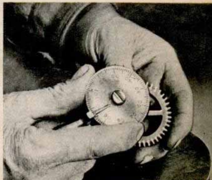
Shaping a commando knife blade on a grinder. Right, measuring an ivory-toothed gear wheel for a locomotive
