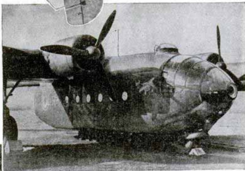
Above: Twin General Electric engines power the XP-83, built by Bell for the AAF and reported to be the longest ranged of the jet-propelled craft. Its top speed is "in excess of 500 miles an hour"
