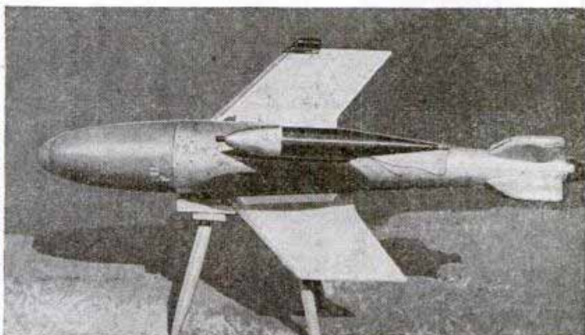
Wing model on new launching sled that cuts takeoff from 300 feet to 50. Below, the Nazi X-4 missile, equipped with a proximity fuse
