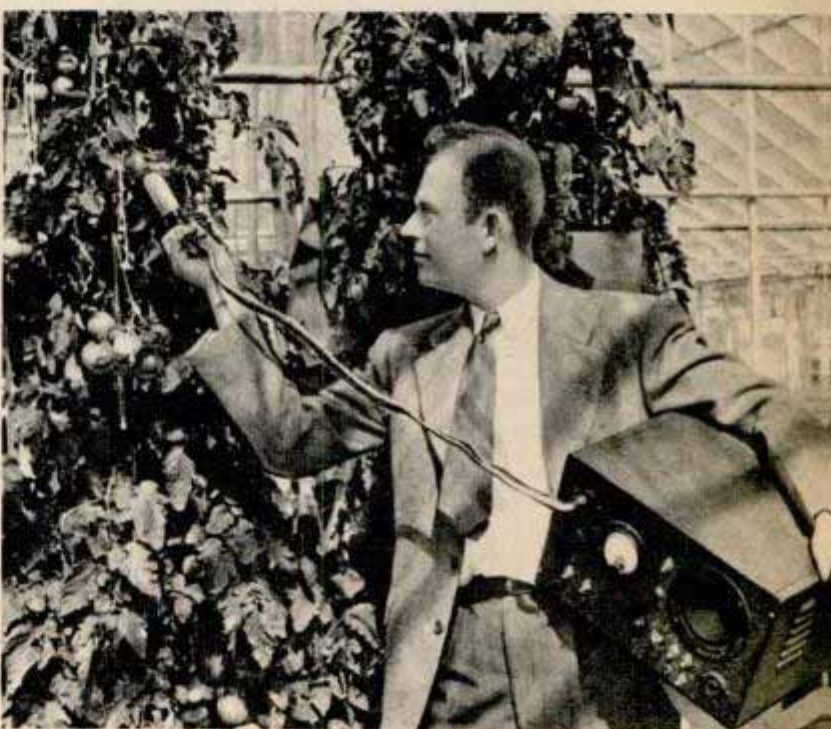
Measuring radioactive "trace elements" fed to tomato plant to learn rate of food absorption. Below, cyclotron control is insulated by water and concrete
