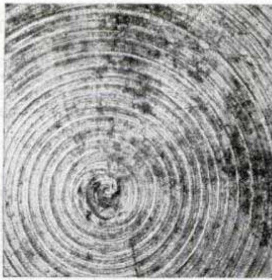
Resembling ripples in water, these circles are tool marks on metal faced on a lathe. Right, wrinkled enamel
