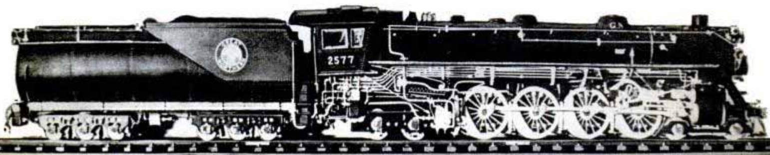
Great Northern mountain type locomotive Designed and built by the Baldwin Locomotive works 1930
