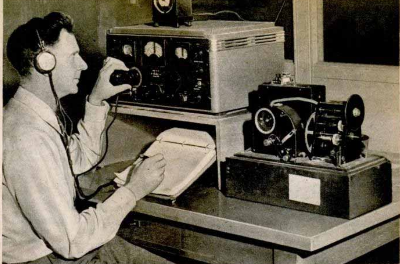
Radioman at Sacramento records high water reports flashed by automatic measurers and radio transmitters
