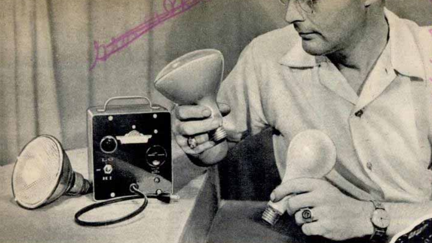
Ordinary light bulbs are stepped up to photoflood intensity by special transformer. Spiral tube (below) replaces flash lamp in reflector for fast shots Megard Corp. photo
