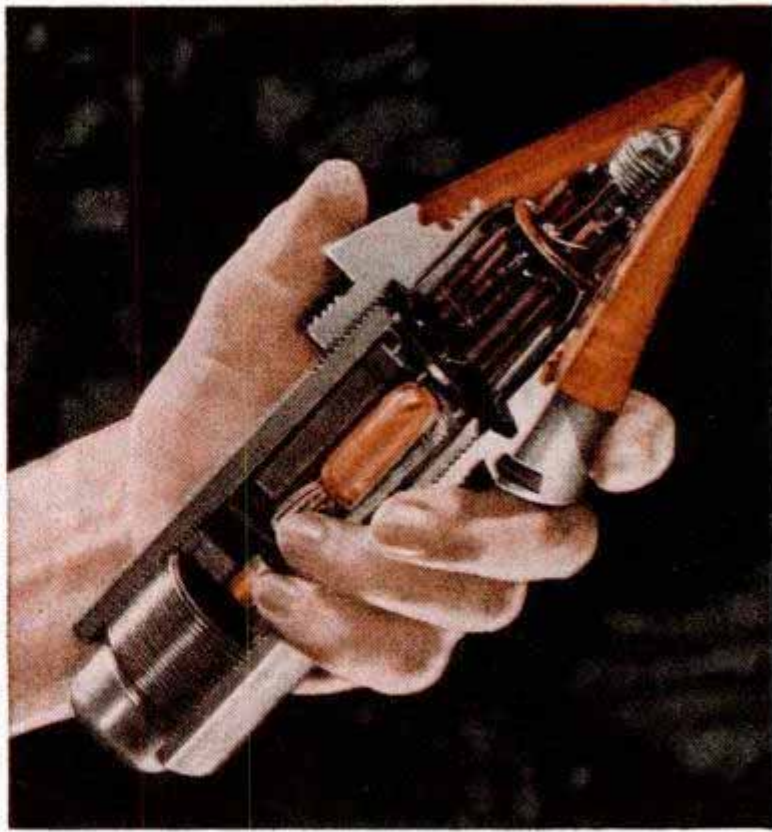
FIVE-TUBE RADIO transmitter and receiver, in the fuse of the shell, is the brain of the secret weapon. In flight, the transmitter broadcasts a continuous radio wave. Reflected back from the target, this wave explodes the shell at exactly the right moment!
