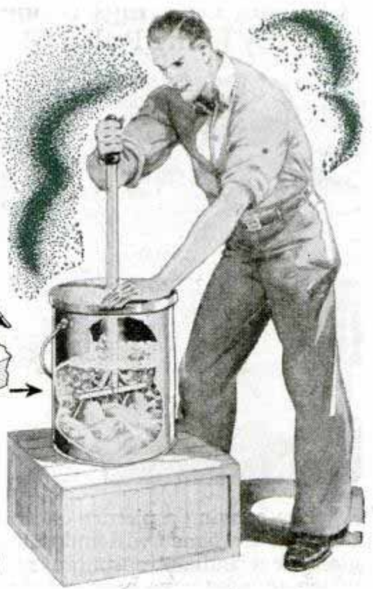
7. To help in locating a toggle switch on the wall in the dark, drill a series of holes in the switch plate and tape a luminous chain pull to it directly in line with the holes. 8. A hand-operated clothes washer, suitable for a baby's garments or for other light laundering, can be made from a large covered can or pail and a T-shaped plunger reinforced with flat iron as shown. Funnels with the necks shortened are bolted to the plunger arm
