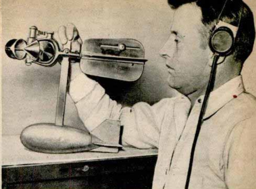
Meteorologist inspects a current flow meter used to measure the rate at which rivers discharge water during big floods
