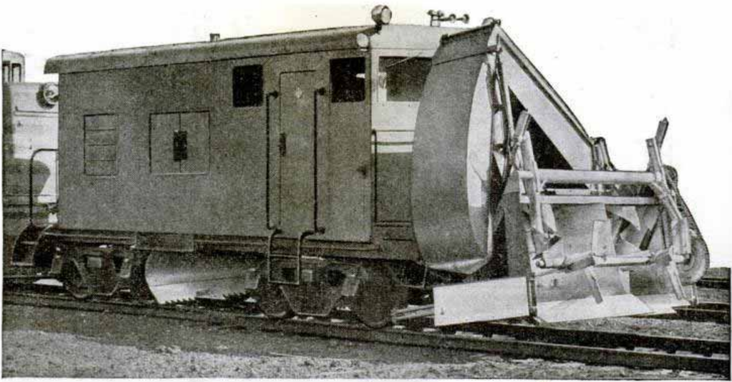
Beneath the cab of the snowplow is an ice scarifier (seen in closeup below) which is lowered to the rail to cut away ice and snow on either side.
