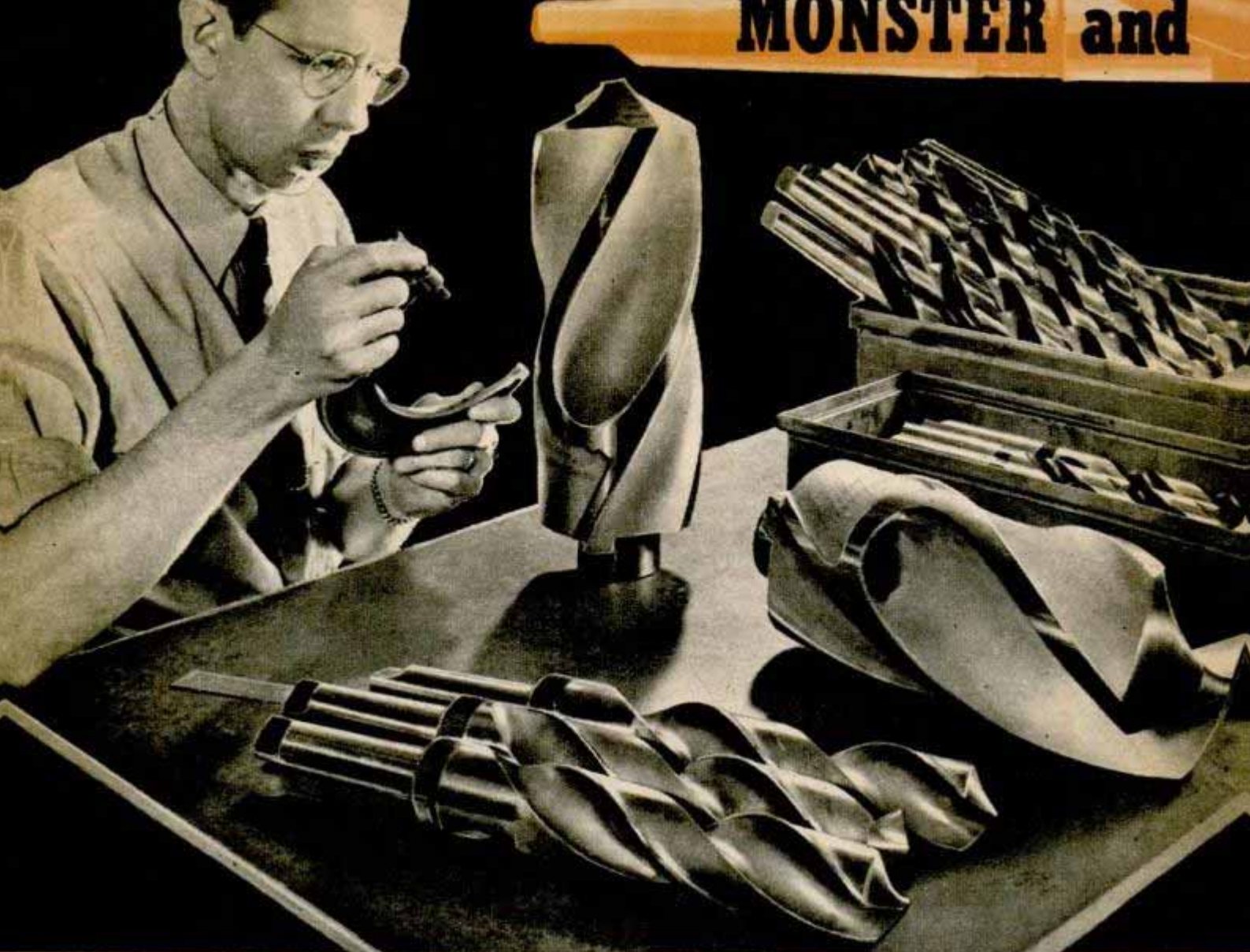
Mesta Machine Co. photo Drill being inspected makes gun bores in 155-millimeter cannon. Below, shankless and conventional drills compared
