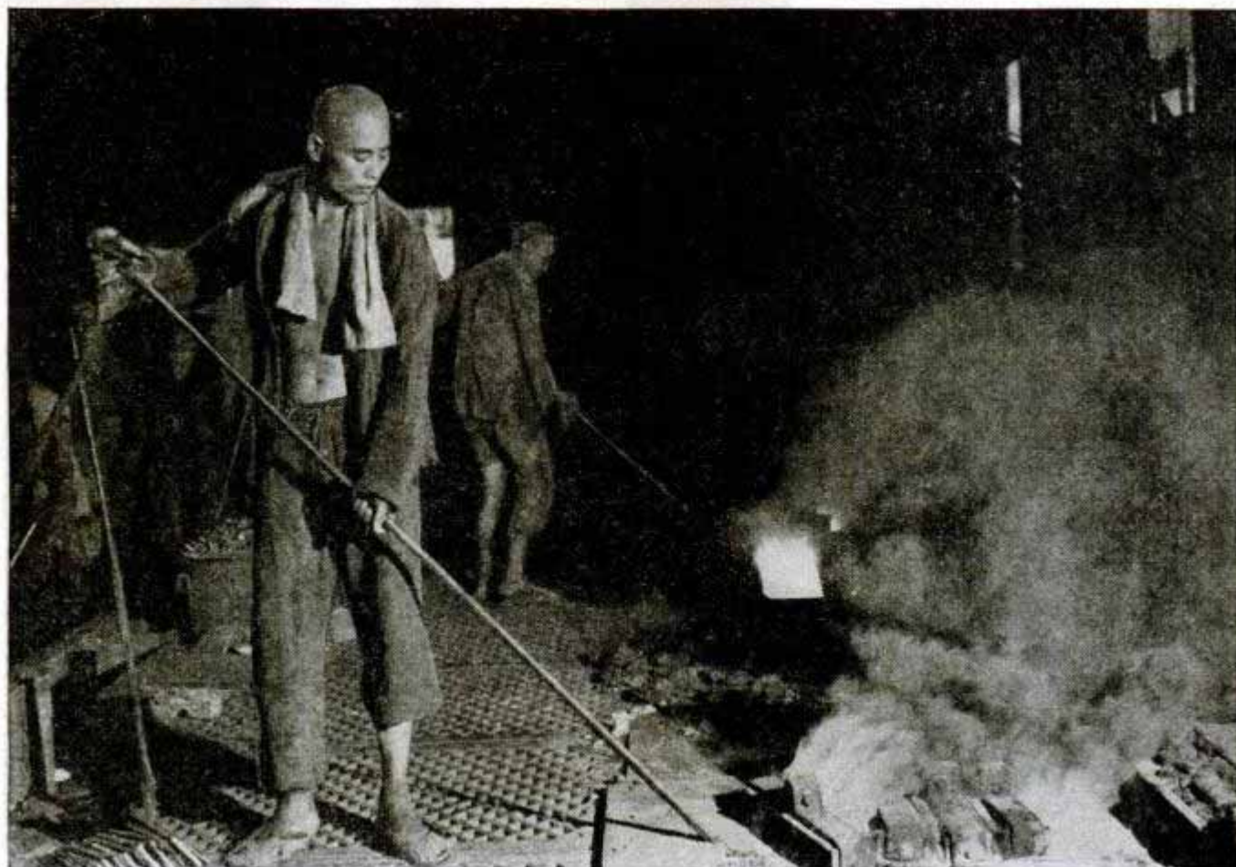
In foundry at hidden arsenal deep in China, workmen prepare to melt brass in one of the many furnaces
