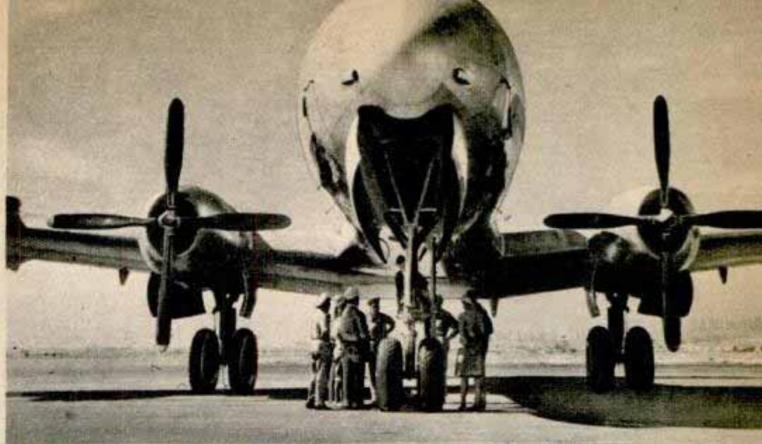
"Bug eyes" of C-74 Globemaster provide pilots with unobstructed vision
