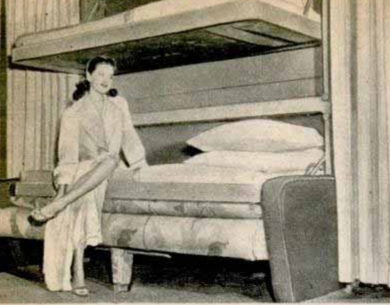
Just push a button and this luxurious club divan for railroad cars is converted into a sleeping unit. Designed by Nathaniel D. Arnot of Baltimore, Md., the sleeper will make bed-making easier for the porters
