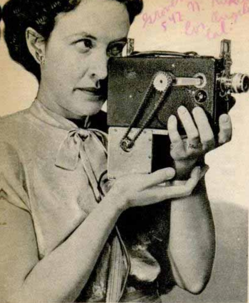
Motion picture camera powered by a battery-driven motor with chain and sprocket wheel. Below, photo printer places wording on the margin of photographs
