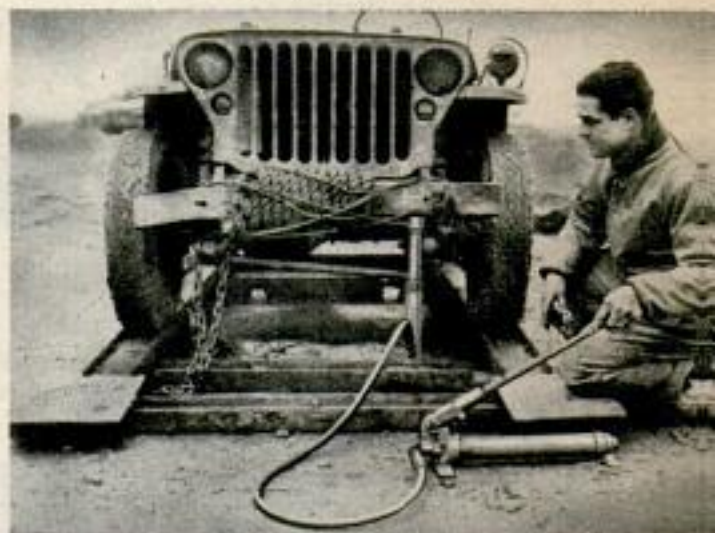
HYDRAULIC PUMP for straightening bent frames is demonstrated by Sgt. Joseph Ferrara, Montclair, N. J.
