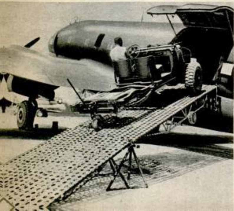
INGENIOUS Army Air Force mechanics used a section of metal landing strip as a ramp to load equipment—even war vehicles—aboard huge cargo planes
