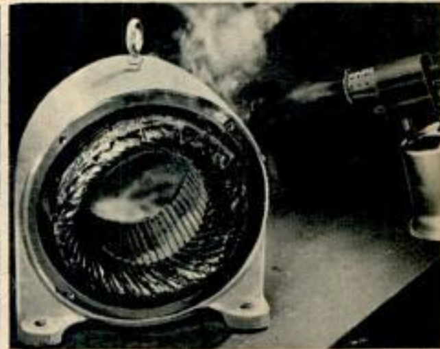
Left, torch ignites silicone-varnished insulation; right, flame goes out seven seconds after torch is turned off
