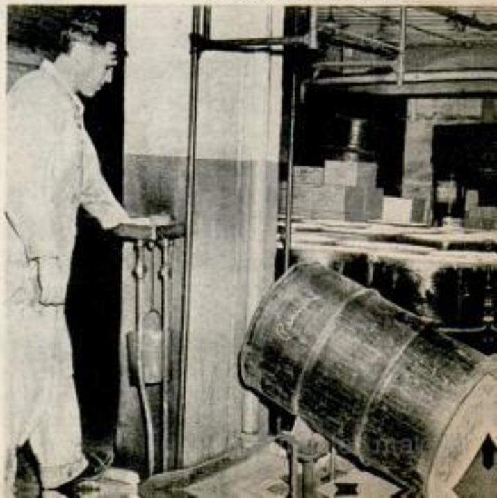
LIFTING 1000-pound drums—a back breaking job—is performed by an air lift. The equipment consists of a double-acting cylinder hoist and three-way valve Compressed Air Institute photo
