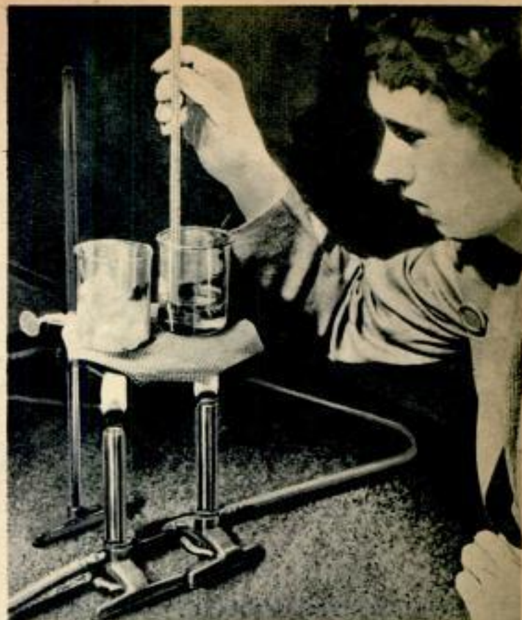
These pictures demonstrate that silicone lubricant withstands higher temperature than petroleum jelly. Left, silicone lubricant is in the left-hand vessel; petroleum jelly in the other. Right, flame melts the jelly
