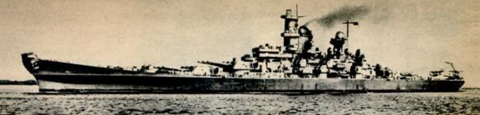
One of Uncle Sam's new $100,000,000 battleships is the USS Wisconsin, 45,000-ton giant of the Iowa class; its overall length is 860 feet. Armament includes nine 16-inch guns, 20 five-inchers and 128 others
