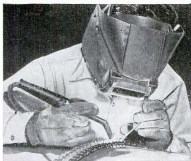
Helium prevents magnesium from bursting into flame during welding operation. Chain holds sheet of magnesium in place. Right, helium tank at air station
