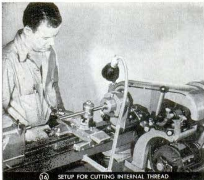
16 SETUP FOR CUTTING INTERNAL THREAD
