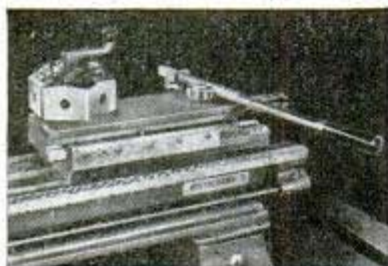
Handlever Bed Turret for 9" or 10" lathes multiplies their versatility through multiple tooling for repetitive operations.
