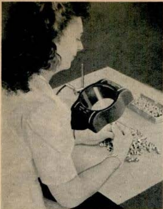
ILLUMINATED WIDE-FIELD MAGNIFIER , equipped with two 110-volt bulbs and a two or three-inch lens, throws a scientifically correct light on the object in the magnification field. The device may be turned to any angle by a universal clamping attachment, and may be raised and lowered quickly for numerous purposes such as machine parts inspections, examination of currency and signatures, or virtually any fine work requiring visual examination.
