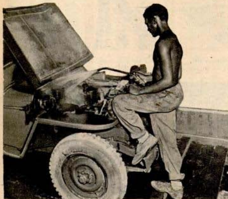
Veteran jeep from Guam is sprayed with preservative after repair job. Below, setting lathe to make jig for fuse setter on shells
