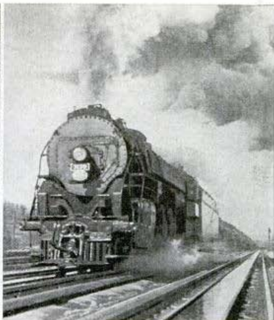
Roaring over track pans, locomotives refill their boilers with scoops lowered from the tender by air
