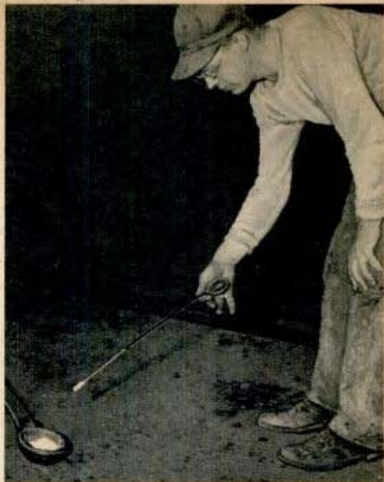
WHITE HOT STEEL is sucked up like lemonade in a straw with a glass tube fitted with a rubber bulb on one end. This procedure is used to obtain a sample of slag-free metal for carbon analysis. When the steel cools, the glass is broken and the test piece is weighed and placed in a high temperature furnace to determine carbon content. Before this method was introduced at U. S. Steel Corporation plants, samples were secured by drilling into slugs of cooled metal.
