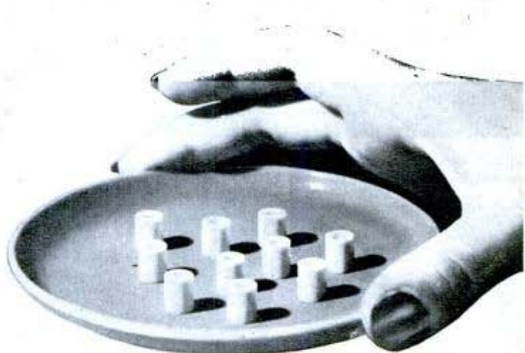
Cylinders made of steatite test penicillin. Below, hand-painting a design
