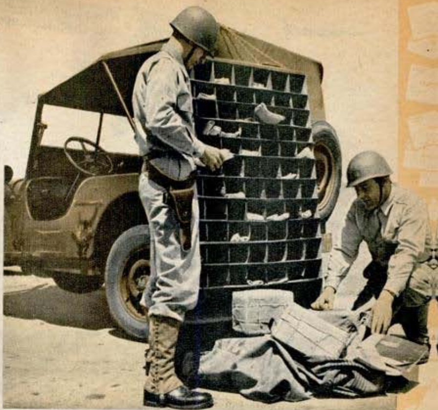
Portable distribution case of canvas and plywood used for field sorting
