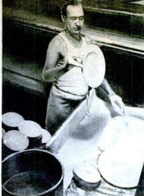
Glazing, or dipping in liquid glass, must be done deftly. Translucence over light discloses glazing flaws
