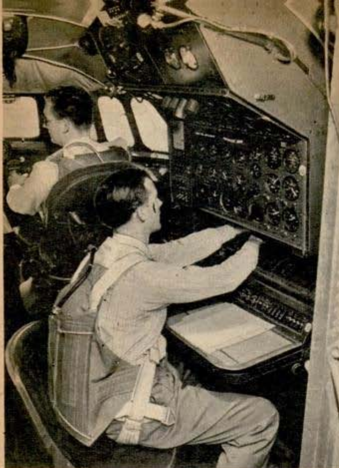
Tiny autosyn motors back of panel operate engine instruments on Constellation. Below, checking hydraulic cylinder that retracts the Constellation's landing gear
