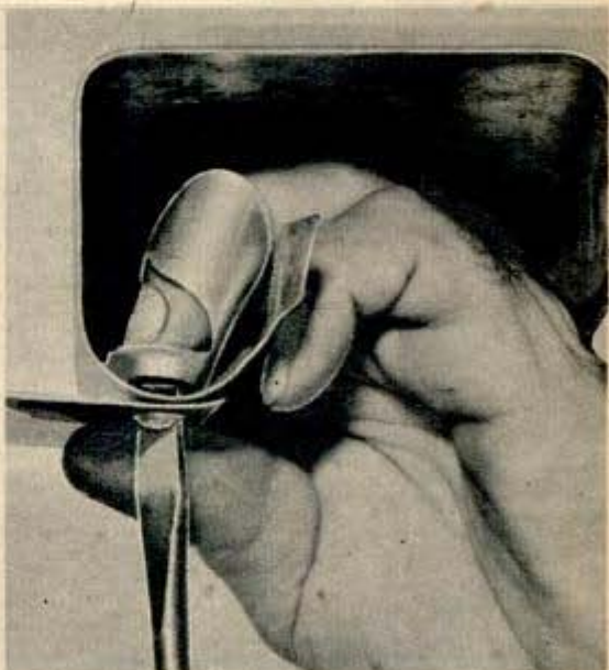
SENSE-OF-TOUCH TOOL locates nuts, bolts or screws which must be fixed in invisible or remote positions. This compact tool, which is worn like a ring on the finger tip, also grips the nut or bolt to hold it in position, and enables a mechanic to use his sense of touch, which is almost impossible with a wrench or screwdriver. When not in use the tool is turned around out of the way, leaving the hand free.
