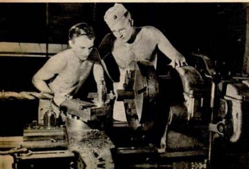
Veteran jeep from Guam is sprayed with preservative after repair job. Below, setting lathe to make jig for fuse setter on shells
