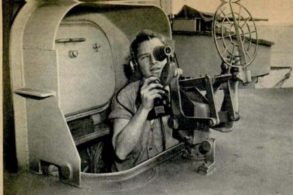
If fire control instruments are knocked out, five-inch turret guns are pointed by this manually operated sighting device mounted on top of the turret
