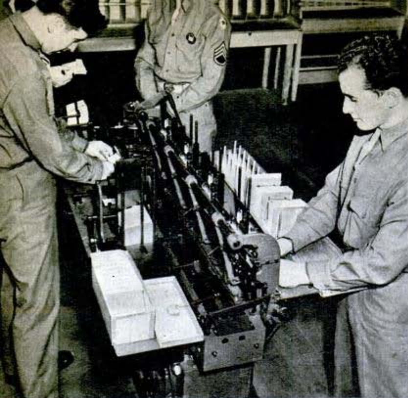
Machine at San Francisco APO puts V-mail in envelope, seals it. B-25 is loaded with mail to drop by chute
