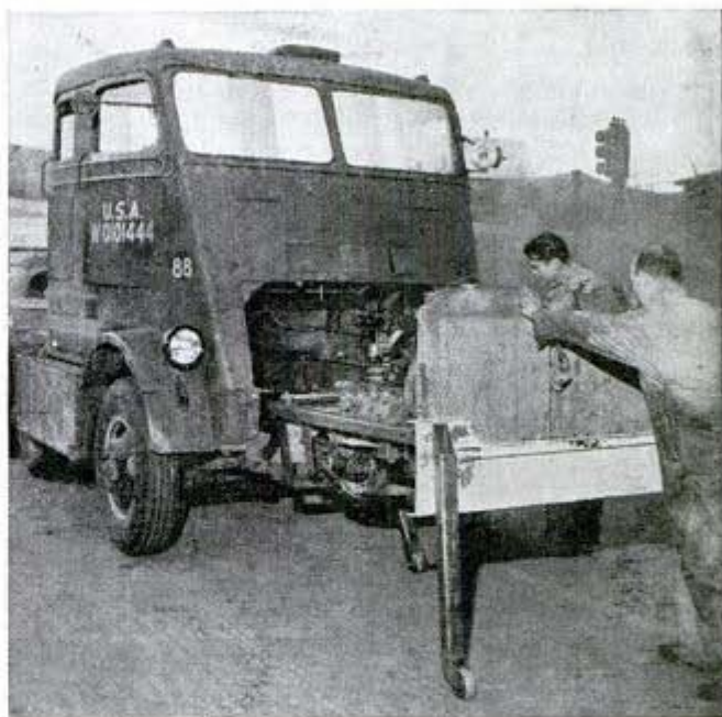
Twin V-8 engines on removable mount which pulls out from beneath hood can be replaced quickly in supertrailer operation
