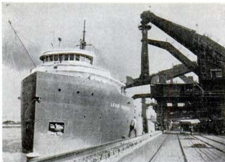
Pittsburgh Steamship Co. photo Unloading new 639-foot ore boat which carried to Conneaut, Ohio, one of largest iron ore cargoes—16,383 tons. Hulett unloader is at work
