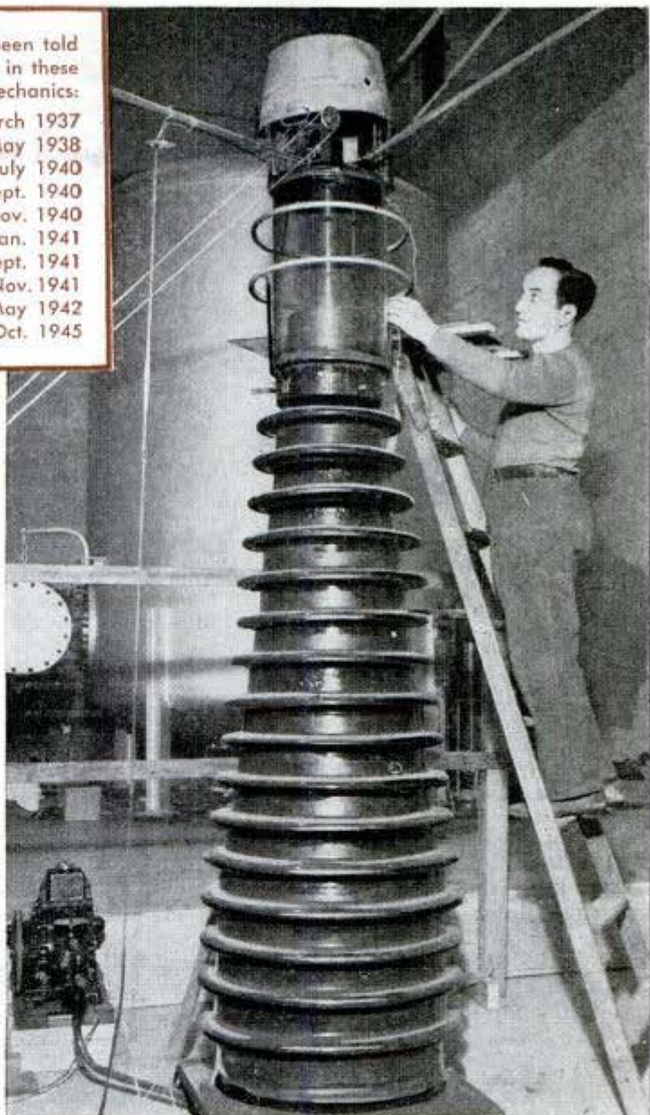
Electrostatic generator of California Institute of Technology performs same work as cyclotron in atom-smashing experiments. Below, scientists in New Mexico used tanks coated with lead inside to guard against radioactivity in studying first A-bomb explosion
