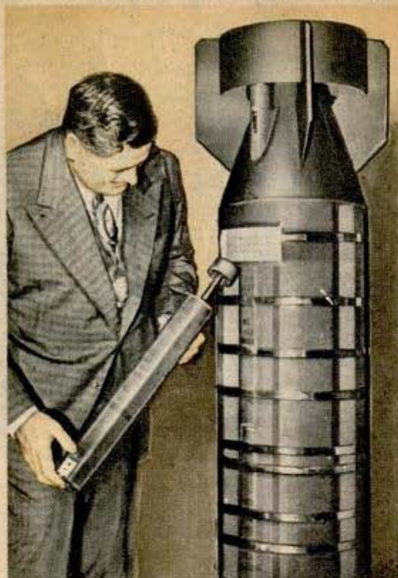
Thirty-eight "Tokyo Fireflies," small incendiary bombs, fit into a big 500-pound missile, shown beside K. T. Keller, president of Chrysler Corporation
