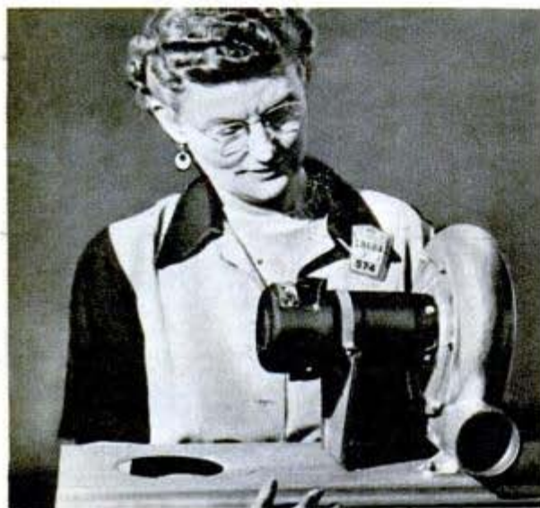
Waterproof motor fits in nose of Douglas Skymaster to operate blower that ventilates the pilots' compartment
