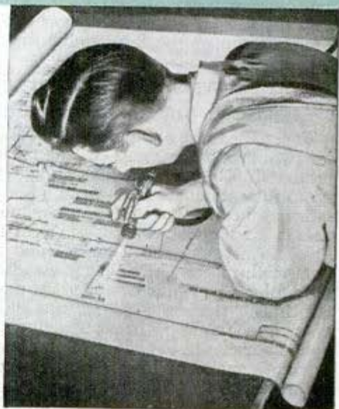
Stayflat frame at back of camera interior is loaded with film, below left. Strong light is focused on frame holding subject matter and correct exposure given. Airbrushing corrects the cloth positive
