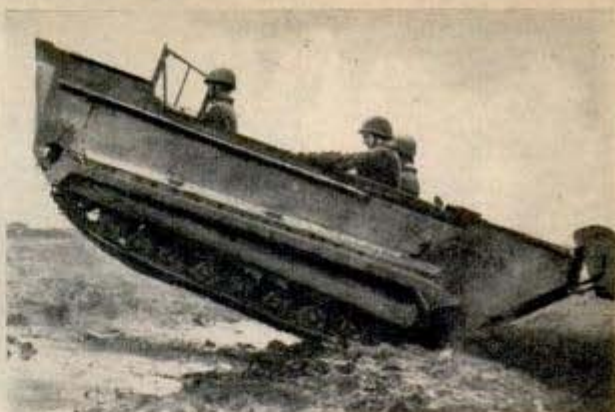
Rugged descendant of Sea Turtle is the Weasel which can climb steep bank; it's powered by Studebaker engine
