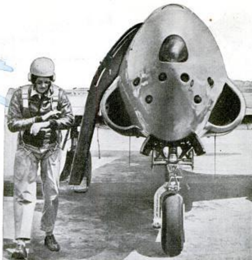
"Ears" of the clean-lined "Shooting Star," seen in head-on view, are air intake ducts. Below, engine of P-59 jet plane with ring of combustion chambers
