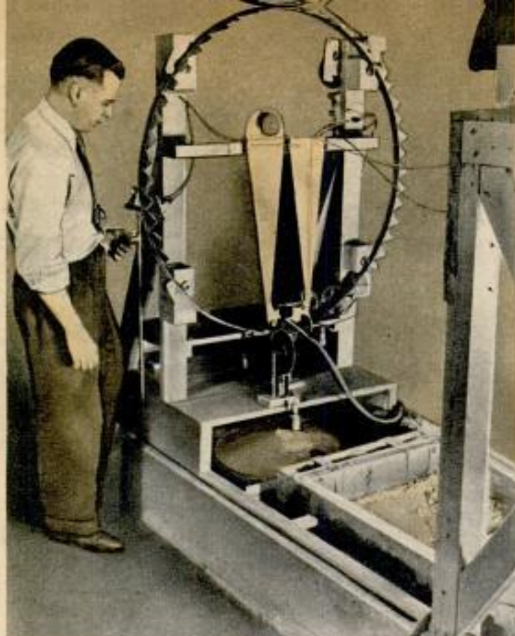
Saw-toothed wheel above in tide machine forms profile of tides in San Joaquin Delta and enabled engineers to learn if fresh water could be transferred across delta model at right. Wheel controls lifting and lowering of sandfilled box in trough of water, simulating tides. Below, 8000-ft. belt conveyor for earth-fill dam
