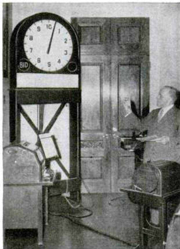
SELEVISION , a device embodying television principles and used for commodity buying and selling, reflects bids made by buyers or sellers in many cities on its white panel from "Quojector," machine at right
