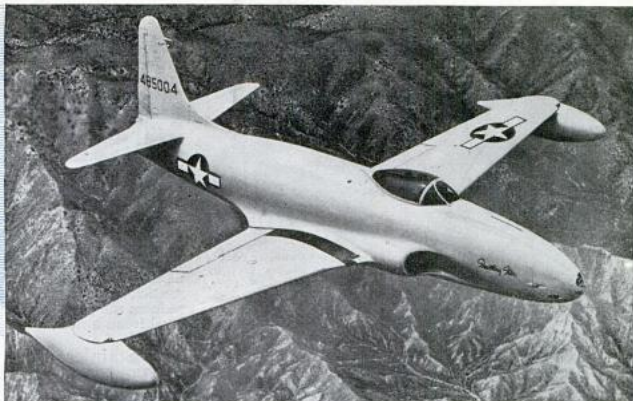
Air ducts hug the fuselage without marring aerodynamic lines; the cockpit is supercharged
