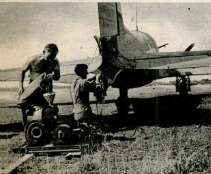
Starting up power plant, which was connected to tail of plane
