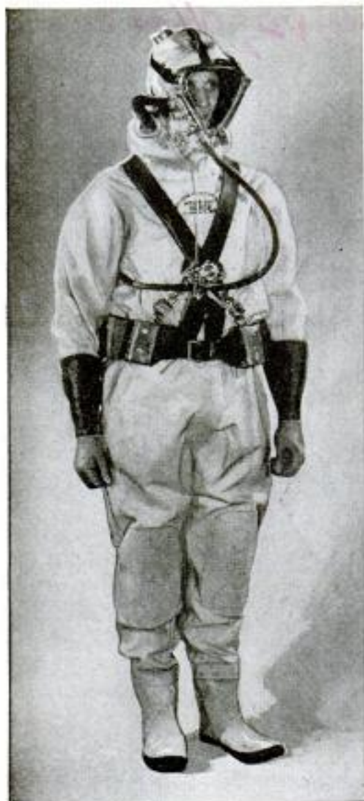
This is the revolutionary 50-pound diving suit. Below, clamp closes the back entrance
