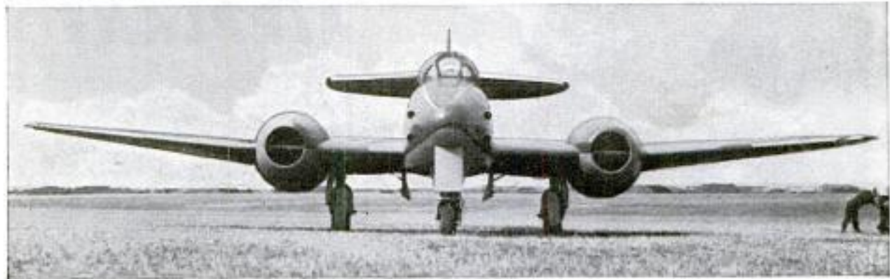
Twin jet British Meteor has high tail and four cannon in nose
