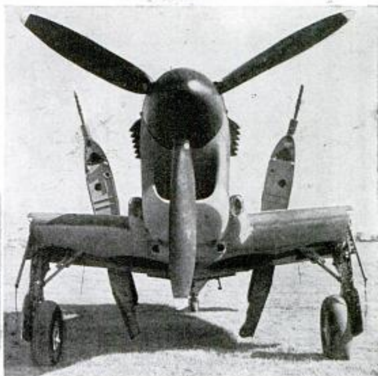
Rocket-carrying Firefly also has four cannon. It can fold wings back (below) to occupy small deck space
