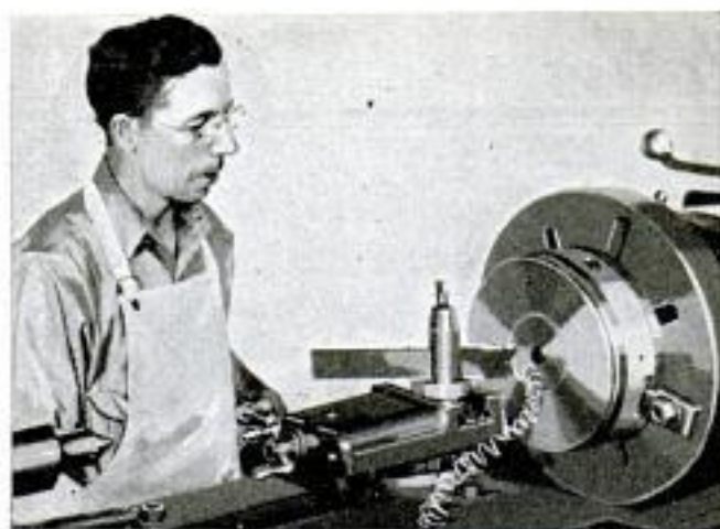
9 WORK HELD ON MAGNETIC CHUCK
