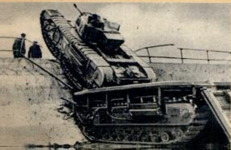
Still another type of bridge-tank, The Ark is a Churchill tank equipped with two trackways made of hornbeam sections of a small box girder bridge. These are fixed together to form a bridge projecting in front of the tank and held in place by wire rope. Ark at top left forms a ramp against a seawall, and another Churchill tank then scales the wall successfully by climbing over The Ark's ramp, left
