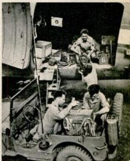
Mercury operators install a set in a jeep for local use, above. Below, working on plane aerial and ground
