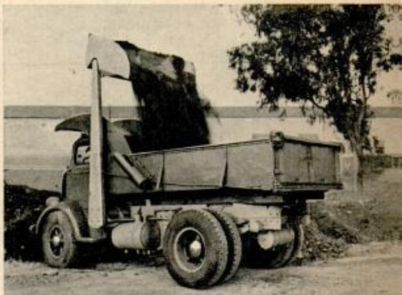
TRUCK SCOOP anchored to frame tosses loads over top of cab into open body. This one-man hydraulic unit is operated from cab by manipulating one lever
