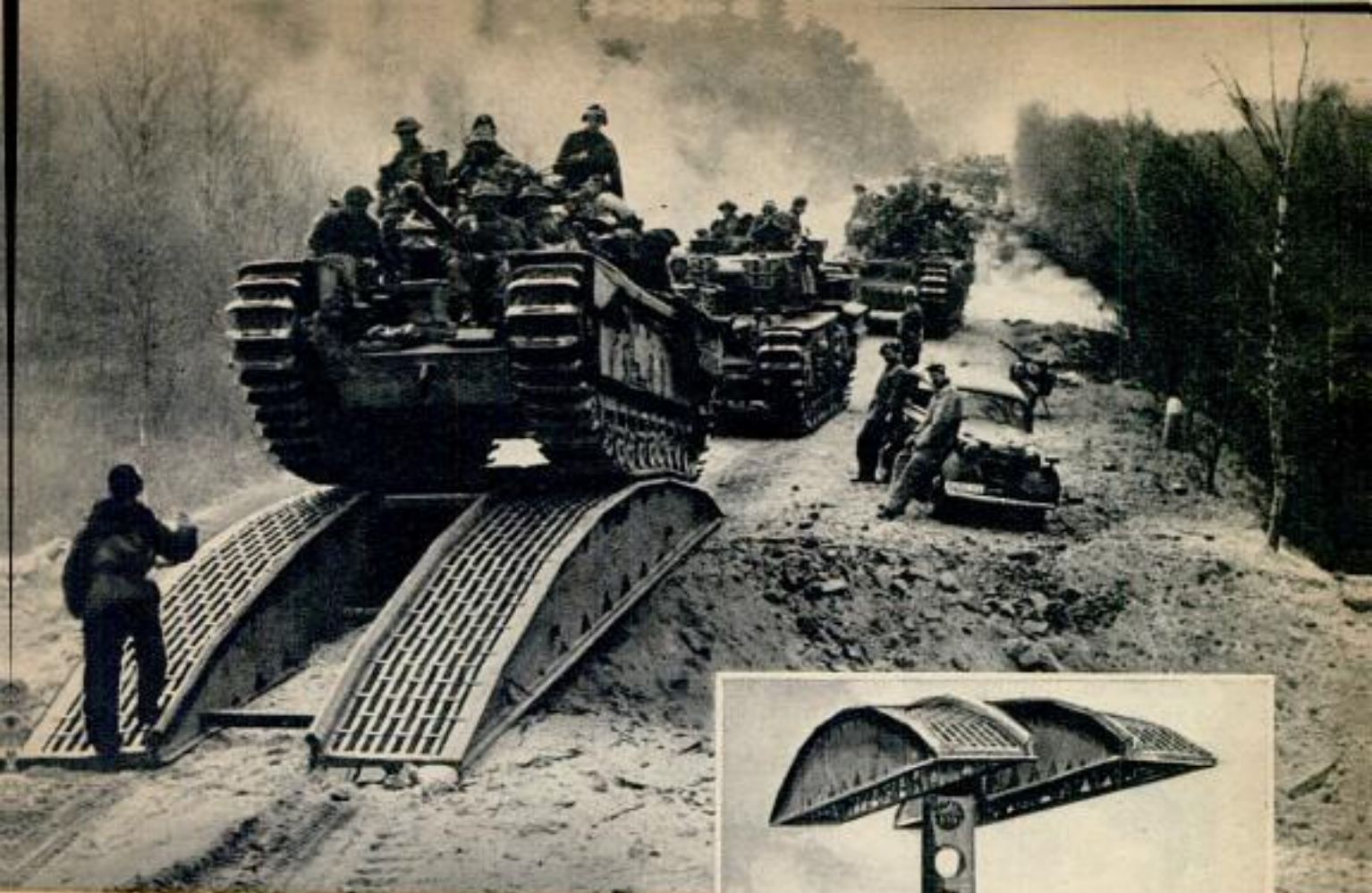
Churchill Bridgelayer is a 30-foot steel span trackway mounted on a Churchill tank. The tanks above are crossing a crater on span laid by the bridgelayer. Hydraulic arm of bridgelayer lifts the span, as at right, then moves it forward and lowers it across gap to be bridged
