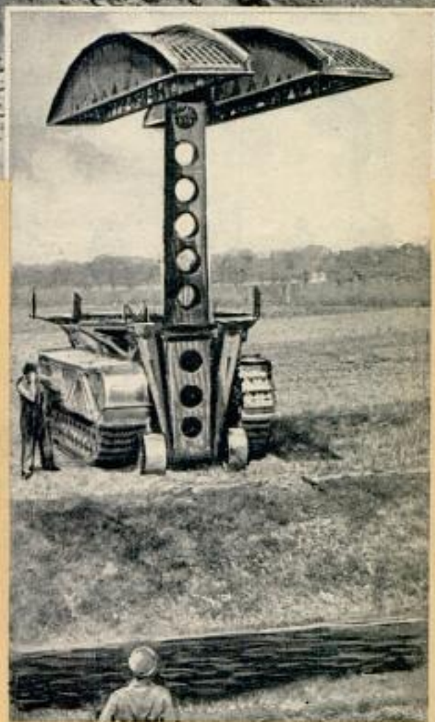
Still another type of bridge-tank, The Ark is a Churchill tank equipped with two trackways made of hornbeam sections of a small box girder bridge. These are fixed together to form a bridge projecting in front of the tank and held in place by wire rope. Ark at top left forms a ramp against a seawall, and another Churchill tank then scales the wall successfully by climbing over The Ark's ramp, left
