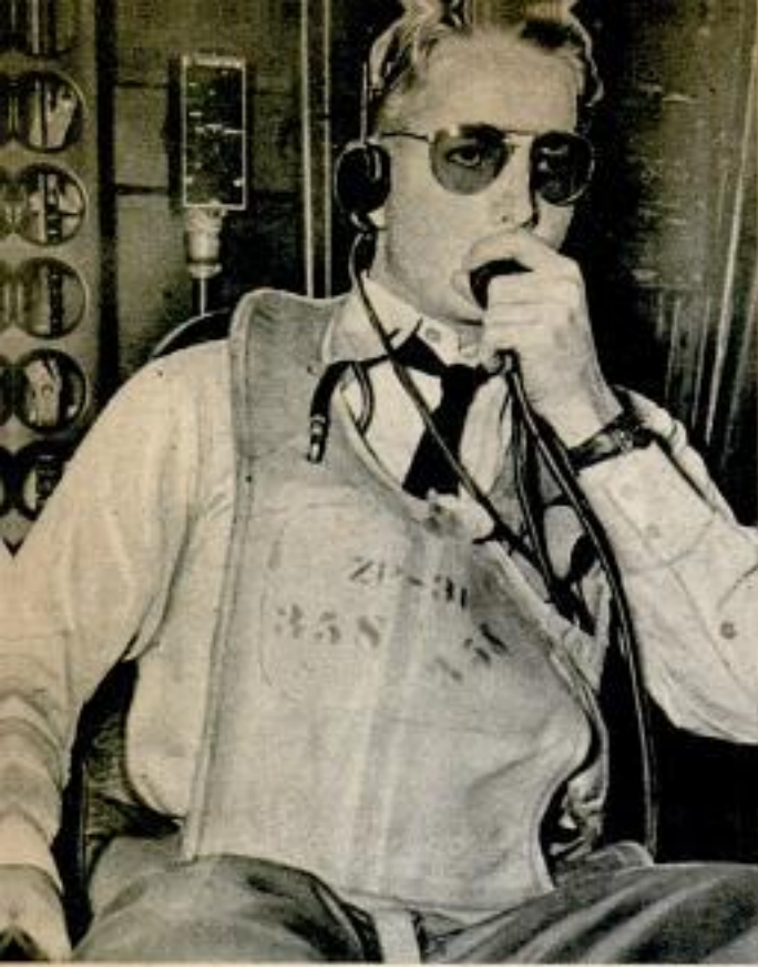
Wearing Mae West life preserver, airship's pilot grasps rudder control wheel while getting a report by intercom phone from aft lookout in cabin
