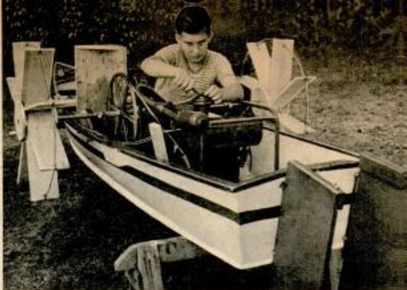
MIDGET SIDEWHEELER is powered by a two-horse-power gasoline engine and is only 14 feet long. Two 30-inch paddle wheels propel craft. It was built by 14-year-old David Bucher at Lake Mohawk, N. J.
