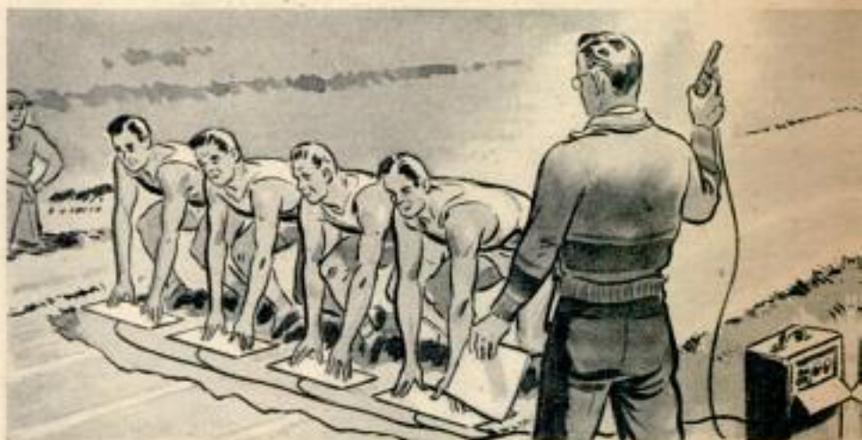
False starts are avoided by metal plates before runner; if hands are taken off, gun cannot be fired. Below, science records a close finish
