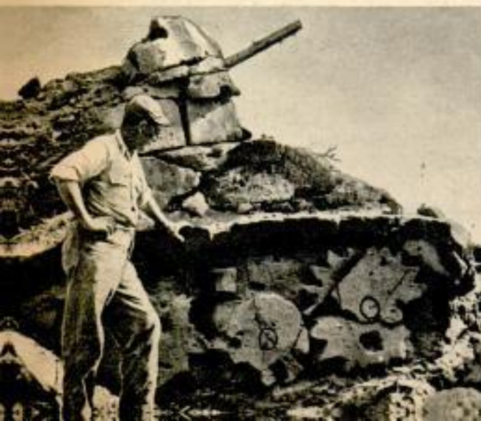
DUMMY TANK made by the Japs was constructed of volcanic ash. They cut cogs in the wheels and used a tree limb as cannon. Yanks found dummy on Iwo Jima
