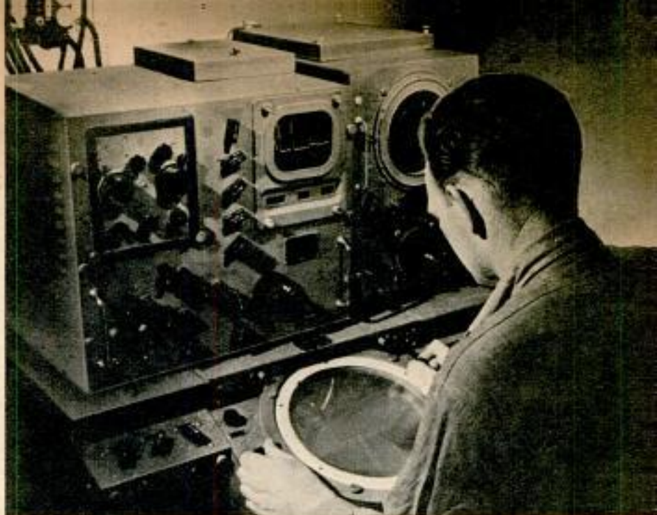
U. S. Navy photo Radar operator is guided by scope in center of set showing graphlike line and by large disk into which he is peering showing actual scene
