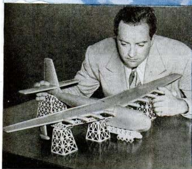
Hughes Aircraft photos Engineer studies model of 225-ton "Hercules," mounted on supports on which hull will float into water. Below, mockup of the control cabin, pilot's seat at left and copilot's at right
