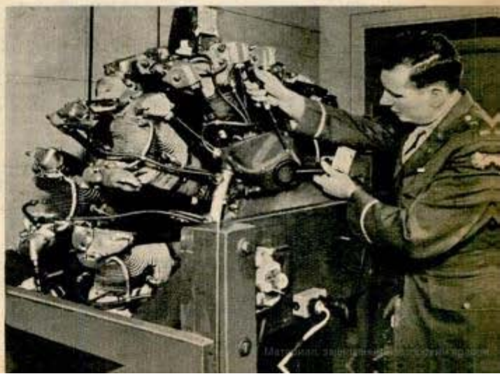
Static discharge tube, above, reduces interference in plane radio. Probe antenna in lieutenant's left hand, below, spots electrical leaks affecting radio
