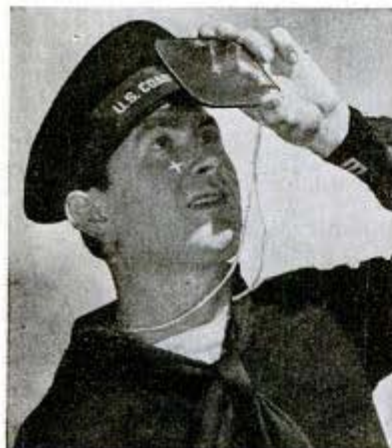
Solar searchlight designed by General Electric, in cooperation with National Bureau of Standards, gives flyers and sailors adrift at sea a way to signal rescuers as far away as ten miles. Most important problem was to find a method of aiming mirror so pilot of plane would catch reflection of the sun.
