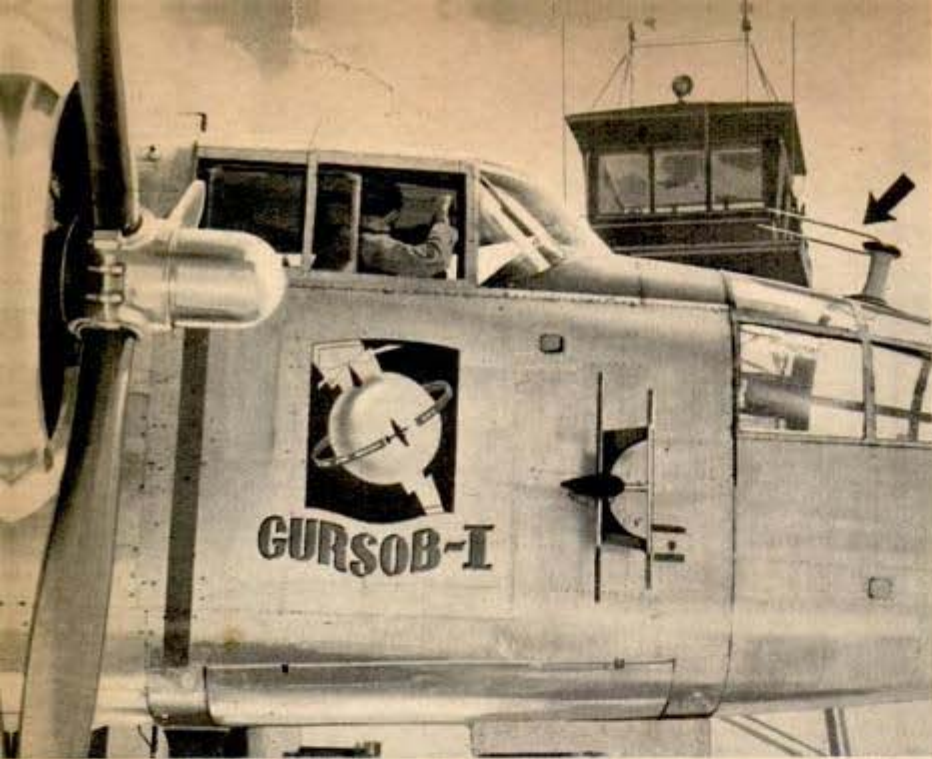
Arrow points to fork-type antenna which receives localizer landing beam
