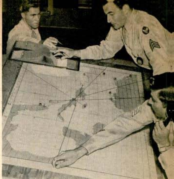
With metal pegs for direction finder stations and cords showing bearings, board charts plane position
