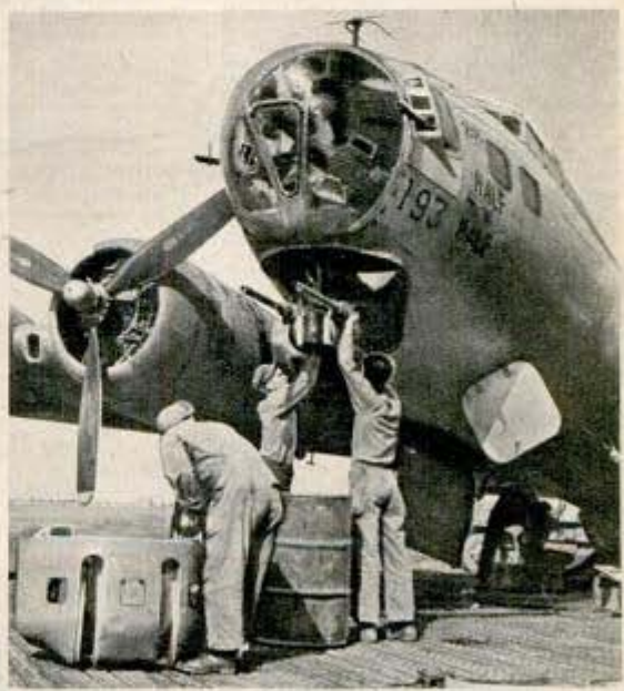
Mechanics remove top turret, above. Engineer-gunner who had station becomes airline "hostess," serving food to returning GIs. Right, out come the chin turret and its twin machine guns. New surface skin will patch up the openings. Fort carries 15 men and crew of five in speed and comfort of any modern passenger airliner. With load, it now weighs in at a mere 57,000 pounds
