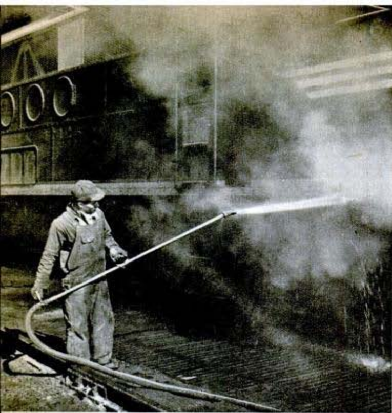
On the wash rack at Winslow a high-pressure steam-operated jet washes grease and dirt from a Diesel engine's trucks
