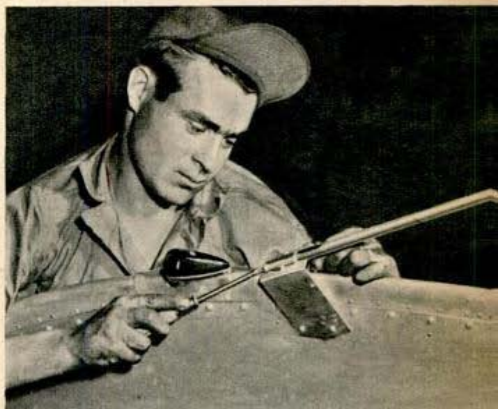
Static discharge tube, above, reduces interference in plane radio. Probe antenna in lieutenant's left hand, below, spots electrical leaks affecting radio
