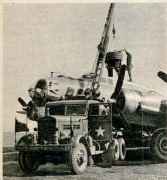
Mechanics remove top turret, above. Engineer-gunner who had station becomes airline "hostess," serving food to returning GIs. Right, out come the chin turret and its twin machine guns. New surface skin will patch up the openings. Fort carries 15 men and crew of five in speed and comfort of any modern passenger airliner. With load, it now weighs in at a mere 57,000 pounds
