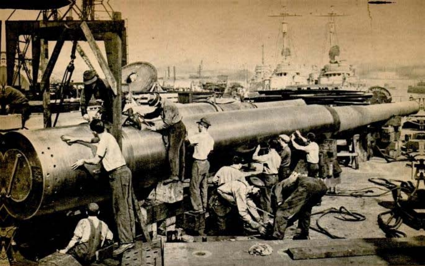
Workmen polish up a 16-inch rifle before 175-ton crane hoists it aboard the 45,000-ton battleship Iowa
