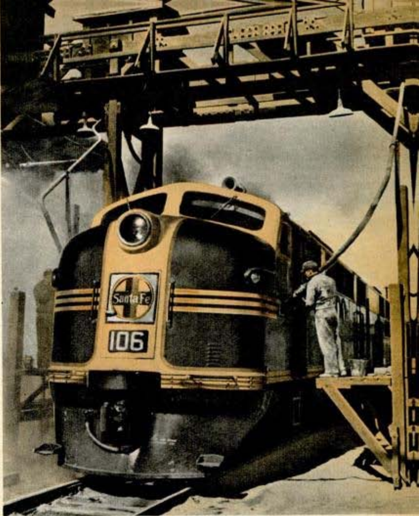
At the Winslow sanding tower the four sand boxes on each engine unit are filled. Below, a new truck is rolled on transfer table under Diesel locomotive. Substitution of a new truck is accomplished in 1½ to 2 hours
