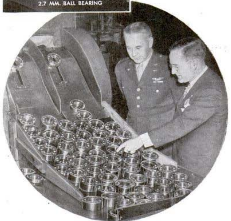
Bombsight bearing, left, is world's smallest. Magnified, it's tiny beside navy beans. Aircraft engine bearings below get final washing in oil
