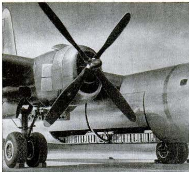
Twin bomb bays of the B-32, arranged in tandem, are shown here with doors open. The tail rises 32 feet high in taxiing position
