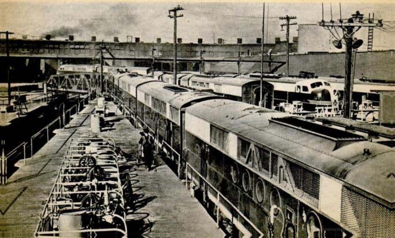
Three of the outdoor service tracks have lighted pits. The 200-foot platforms just fit a four-unit Diesel
