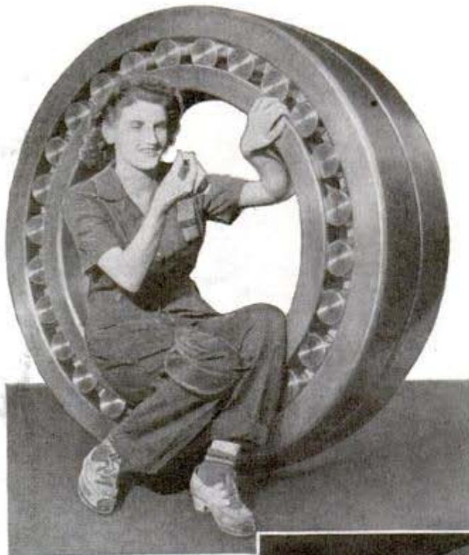
Girl in 10-ton bearing for gun turrets holds a \frac{3}{8} -inch ball
