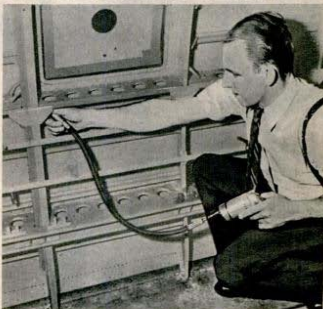
Offset spindles and straight, 45-degree and 90-degree angle heads permit drilling around corners and in hard-to-get-at spots
