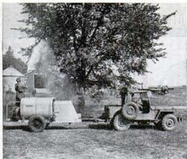
Power takeoff on postwar jeep operates tree spray
