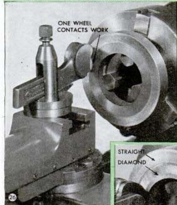
Face knurling: One wheel contacts work for straight pattern, both wheels for diamond pattern
