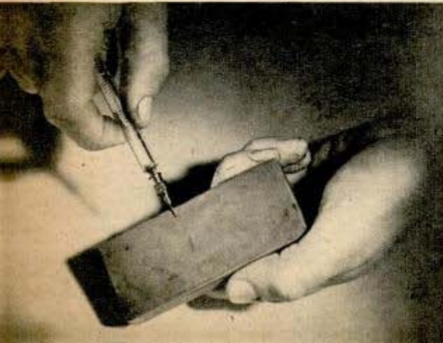
Pictures above show first steps in converting needle to pen. After nicking with file, needle is broken off short. Needle stub is then rotated across whetstone (below) until smooth and small enough to make line of desired thickness. Below right, special attachment for making arcs or large circles in varied colors Consolidated Vultee Aircraft Corp. photos
