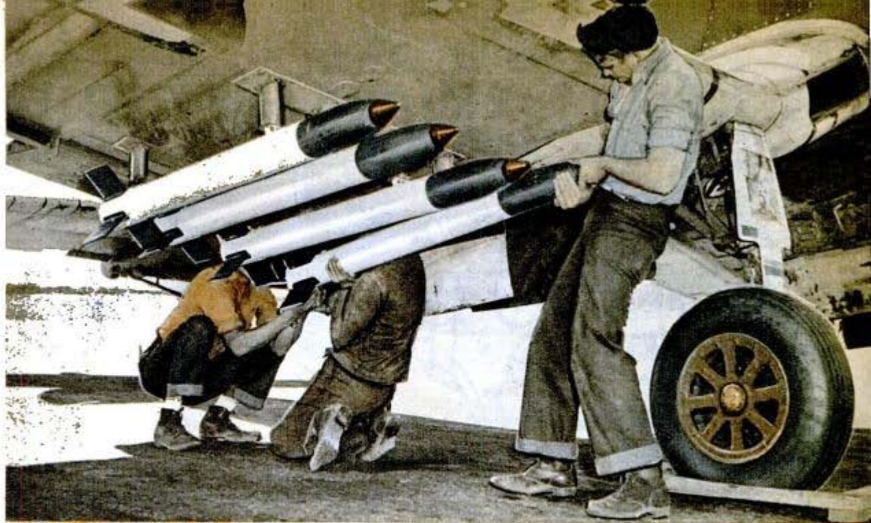
Naval ordnance men fit high-velocity rockets to rack of rocket-carrying plane for test run at desert range
