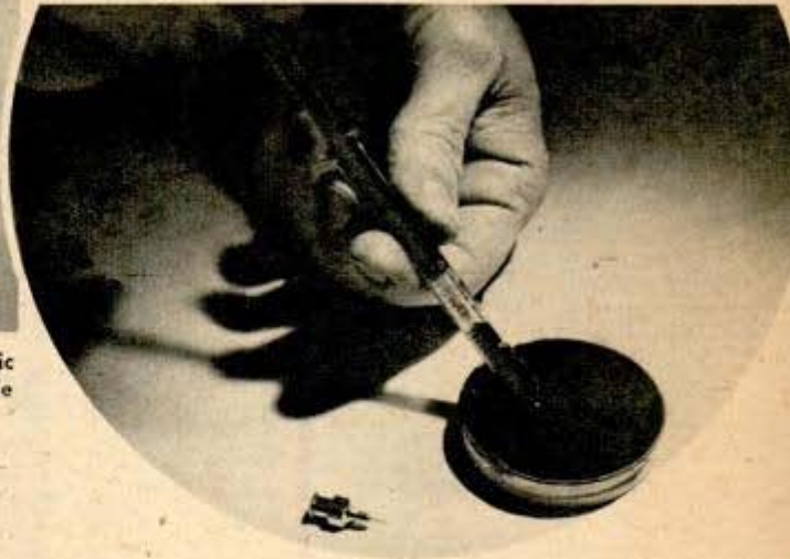
"Hypo" pen made by engineer in aircraft plant is filled with lacquer-type ink, hard to smear but easy to erase. Below, pen makes a sharp line which dries quickly
