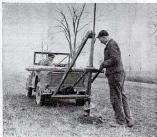
Postwar post holes—power takeoff operates auger. Below, jeep helps paint barn by powering a sprayer
