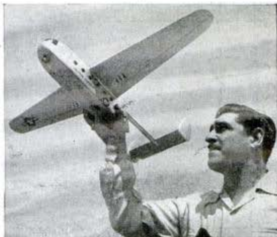
Model of J-19 shows rear loading doors. At right it is held at angle at which it will be towed into the air assisted by six rocket units held under the wings
