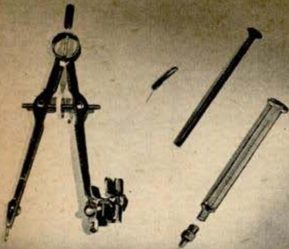
Equipment for drafting pen made from hypodermic needle includes compass, syringe and the needle
