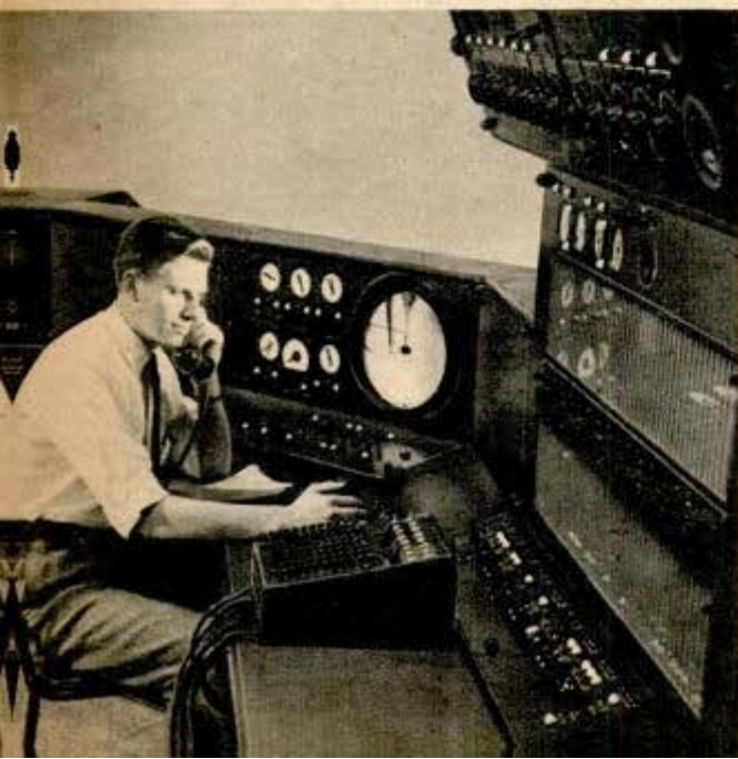
Dr. Clark B. Millikan, director of Pasadena wind tunnel, adjusts model for test. Below, "console" of twin tunnel in Buffalo, N. Y., has 587 signal lights Curtiss-Wright Corp. photo
