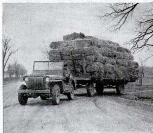
Postwar jeep pulls trailer loads up to 5500 pounds. Below, power takeoff delivers 30 h.p. to buzz saw
