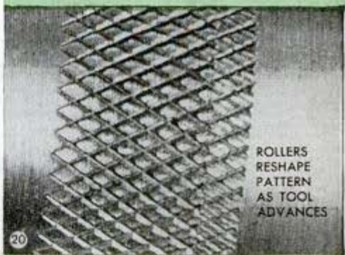
Knurling rollers will reshape the pattern after a good track is established
