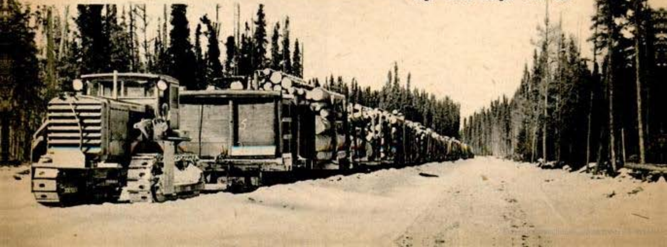
Left, Diesel engines are ideal power units for tugboats. Below, Caterpillar pulling sled train of logs — total weight 1192 tons
