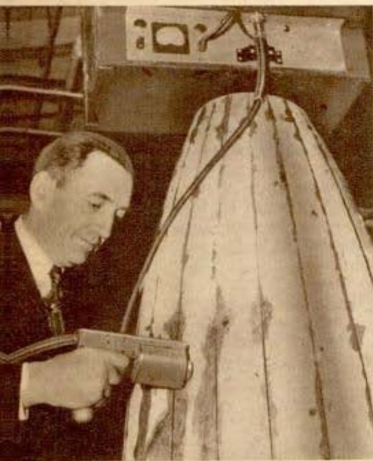
Brushing glue onto wood that will form sturdy spar for wood airplane. Below, short-wave "spot welder" joins strips for airplane drop tank
