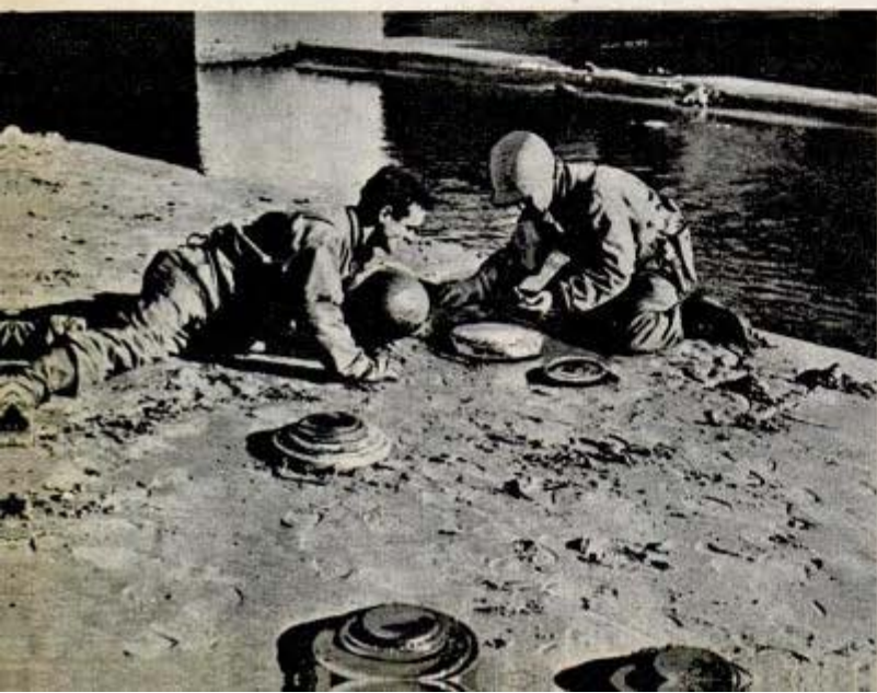
Mine at left above is connected to electric fuse. Center, with double fuse, and right, three-prong fuse. Below, engineer removes detonator of antitank mine
