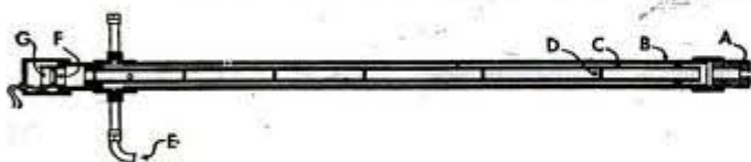
A, nose of pyrometer; B, outer case; C, inner tube; D, antireflection diaphragm; E, air line; F, window; G, photronic cell
