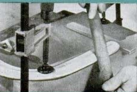
Round the top surface with a wood rasp and sand smooth
