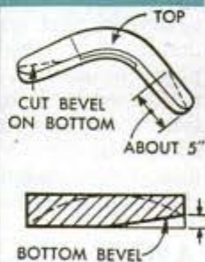
Sand or plane the bottom bevel—about \frac{1}{16} in. probably will be enough. You can increase it later if it is necessary
