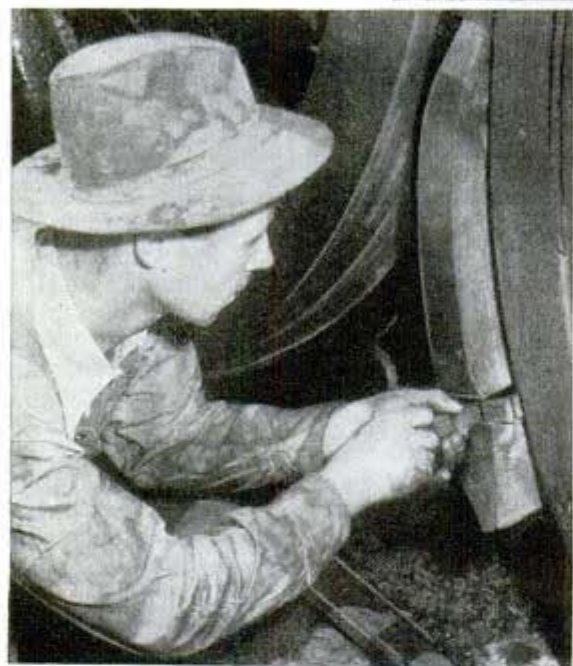
Above, tire cutting tool replaces the brake shoes. Cable tows engine on 800-foot siding, above right
