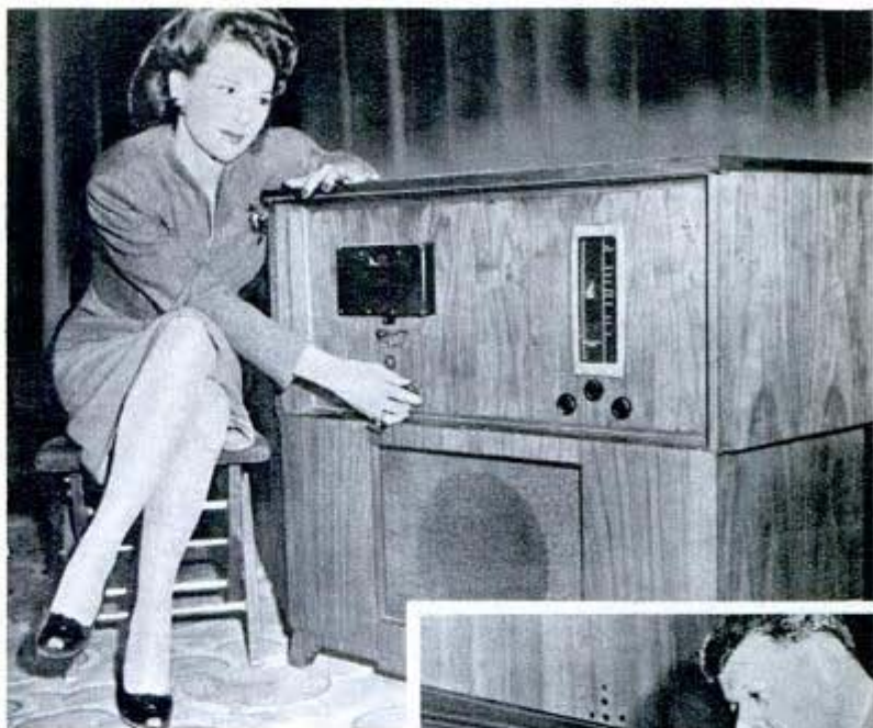
Above, girl "takes down" program on wire recorder magazine plugged into radio. Right, magazine unit is quickly detached
