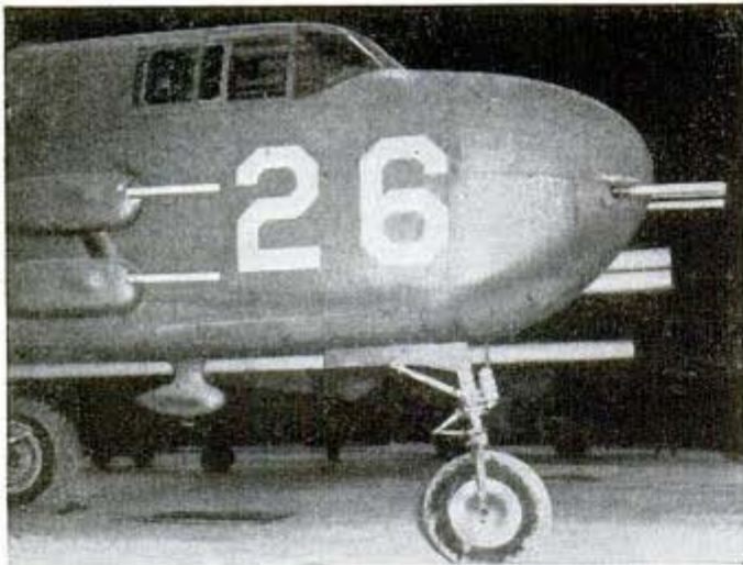
Hudson Motor Car Co. photo This B-25's wallop consists of six forward-firing machine guns (four in nose, two hugging fuselage) and three rocket launchers
