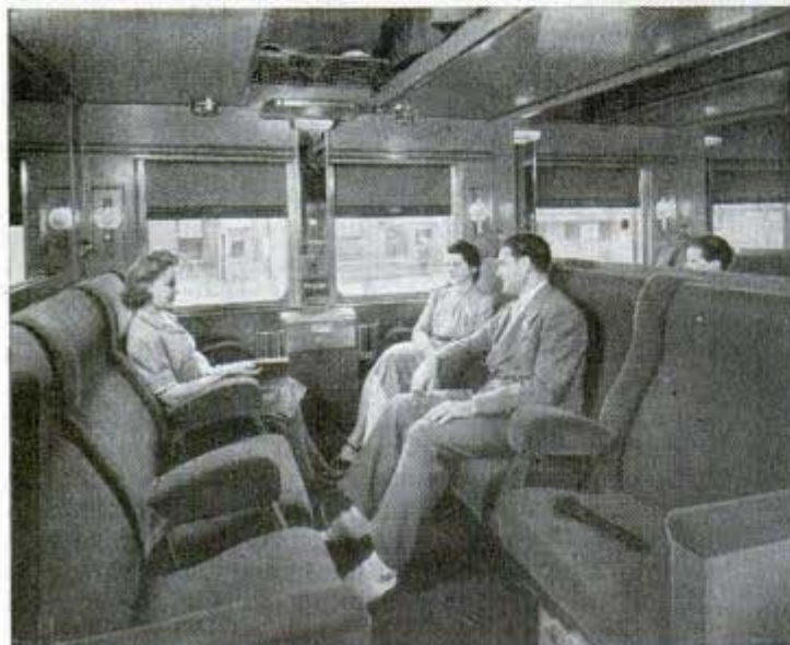
Seats of Triple-Deck sleeper are transformed at night into separate berth sections, each with own lavatory
