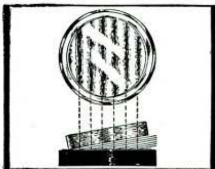
Optical Flat. Surface of Work. Interpretation of bands on truly flat surfaces.
