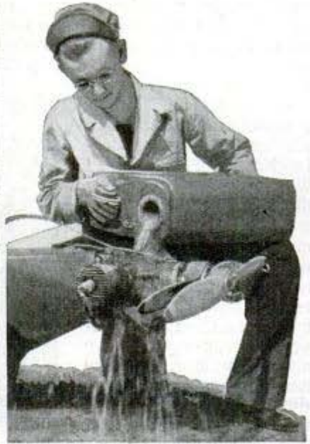
Upper left, robot plane's parachute must be detached swiftly by rescue squad. Plane is lifted tail up, as below, to shed salt water quickly. Gasoline bath, above, saves engine
