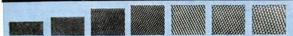
13 COARSENESS RANGE OF MACHINIST'S FLAT BASTARD FILE
