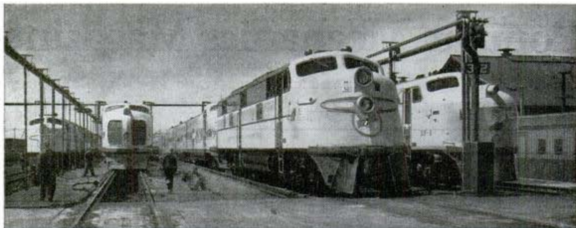
Standardized equipment of streamliners speeds their servicing in special yards built by the North Western
