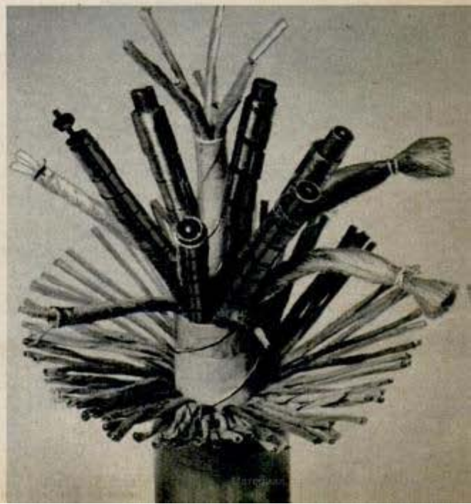
Splicing a coaxial cable, below left. At right, new cable carries six coaxials, many ordinary wire pairs
