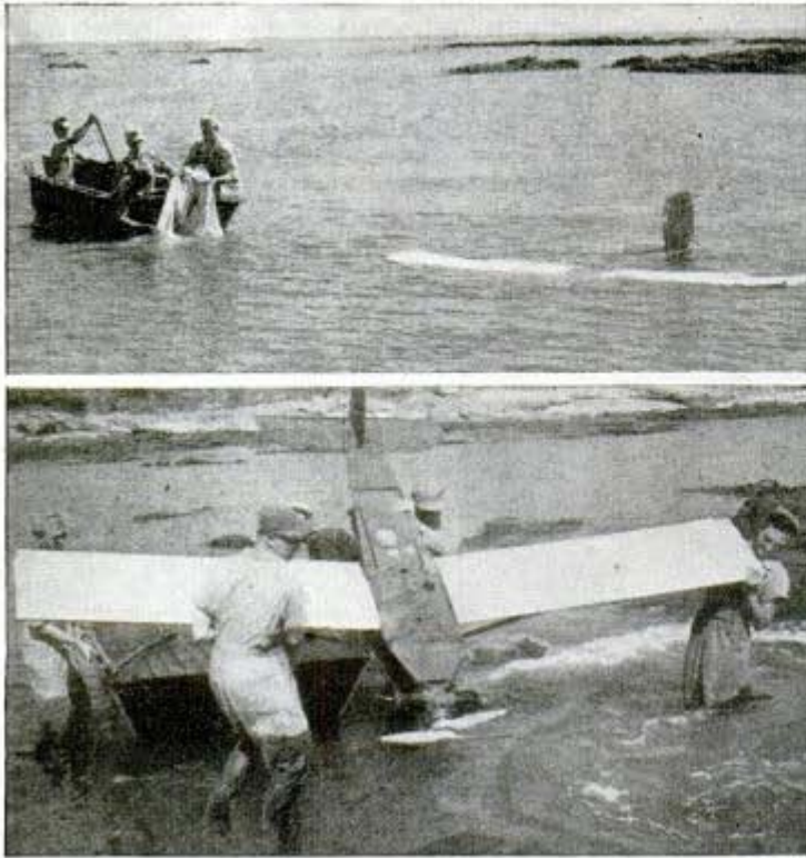
Upper left, robot plane's parachute must be detached swiftly by rescue squad. Plane is lifted tail up, as below, to shed salt water quickly. Gasoline bath, above, saves engine
