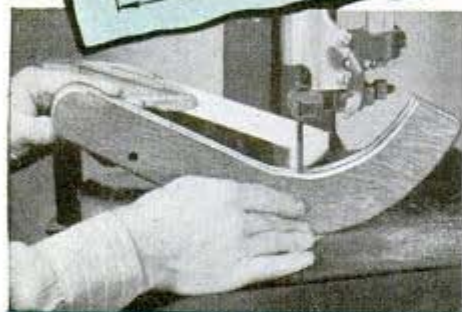
Cut outlined shape from \frac{7}{8} -in. stock, then rip to get two identical pieces
