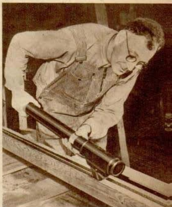
After arch is built up of plank laminates, clamps are used for shaping. Below, glue wheel takes guesswork out of applying correct amount to wood
