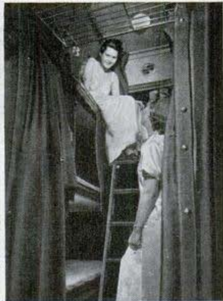
Seats of Triple-Deck sleeper are transformed at night into separate berth sections, each with own lavatory
