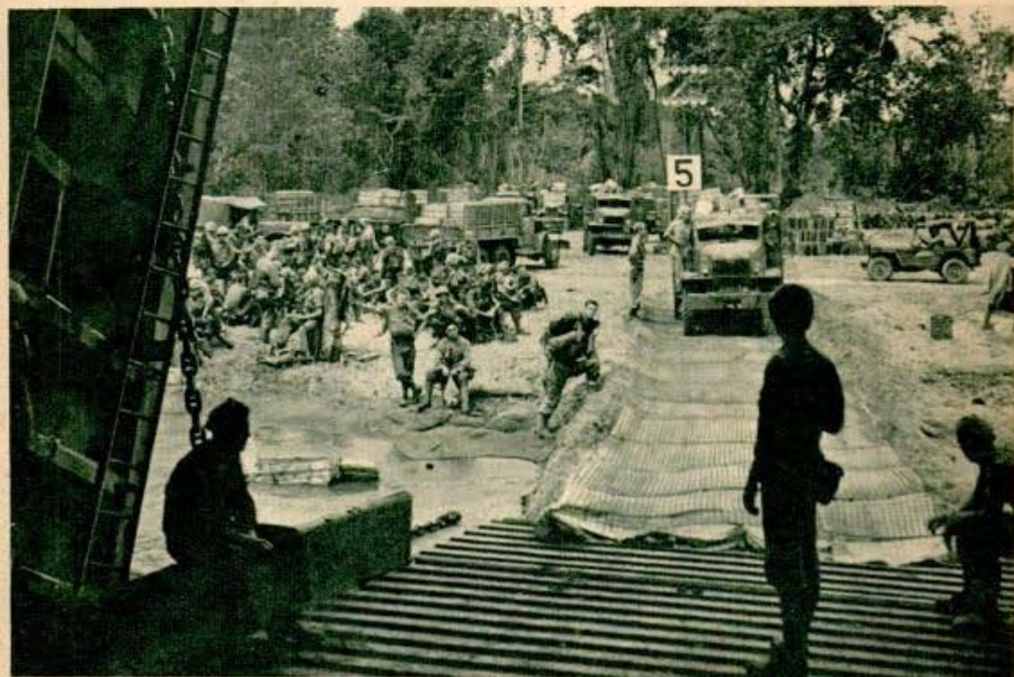
Loaded for combat, trucks roll over steel mat on sandy beach toward lowered ramp of Navy's sturdy LST
