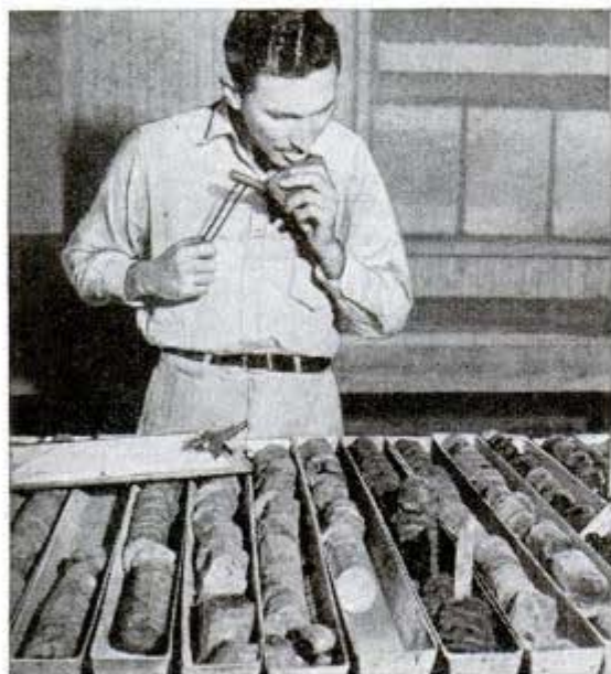
Above, 150-foot caisson pile being loaded on barge. Left, testing core samples in La Salina laboratory
