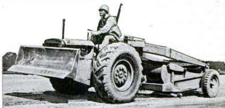
Courtesy R. G. Le Tourneau, Inc. Scraper and "tiltscraper" built for air shipment will do work of 50 men. Below, Yanks build road through jungles of Leyte
