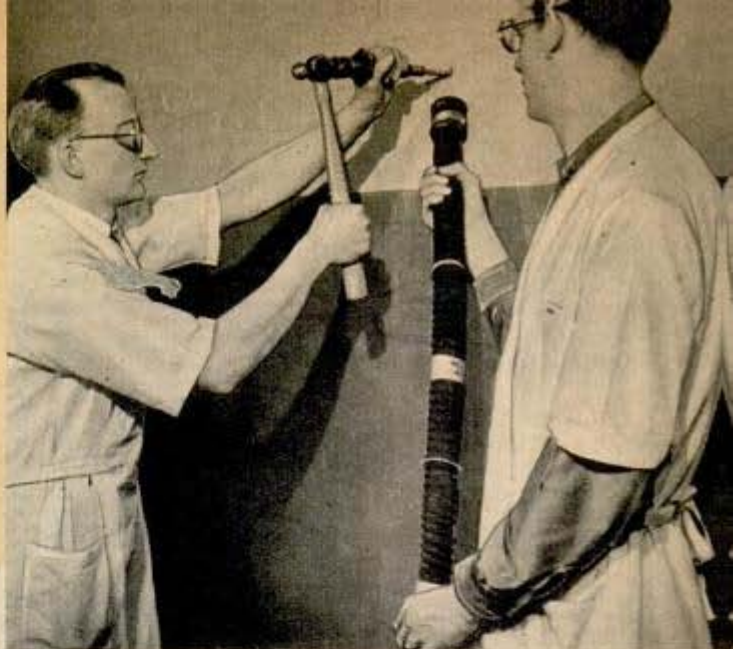
Courtesy Eastman Kodak Company The "D-Men" in a huge film manufacturing plant hunt down dust as G-Men hunt criminals. Vacuum hose (above) picks up particles of plaster as hole is made in wall. Below, dragging "dust detective" along floor. It is made of a two-pound weight with wrapping of cleansing tissue. Workmen wear special white uniforms which get "wind baths"
