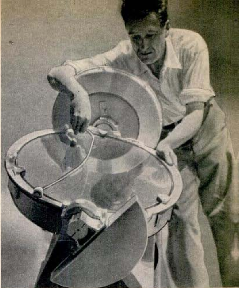
Centering beam on mirror at top of sun tower insures proper reflection down shaft. Below, "closeup" of moon shows craters
