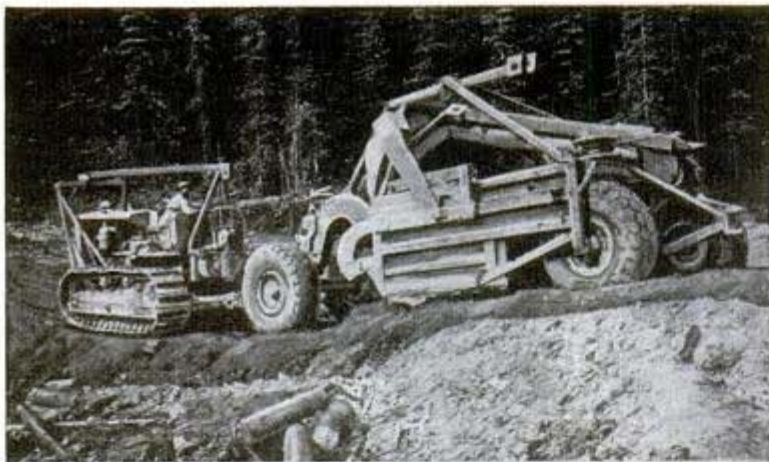
Cable-operated self-loading scraper used by Army is towed by tractor
