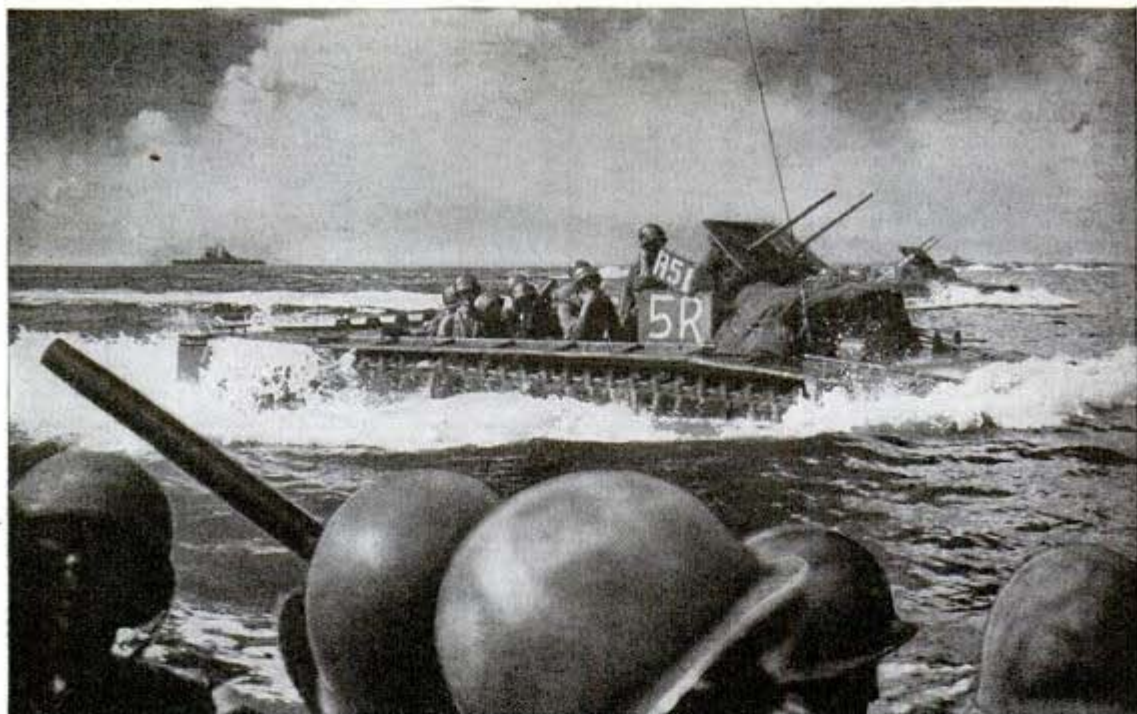
LVT(A) sweeps toward a beach in the Pacific. Tracks enable landing vehicle to creep over dangerous reefs
