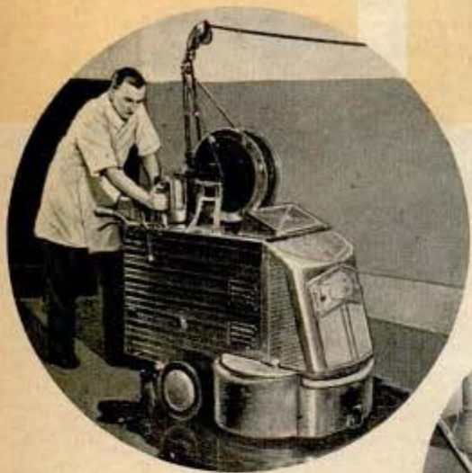
Above, hall floors and all main traffic routes in film plant are washed twice daily with electric suction scrubbing machine. Right, "gelatine" mats pick up dust
