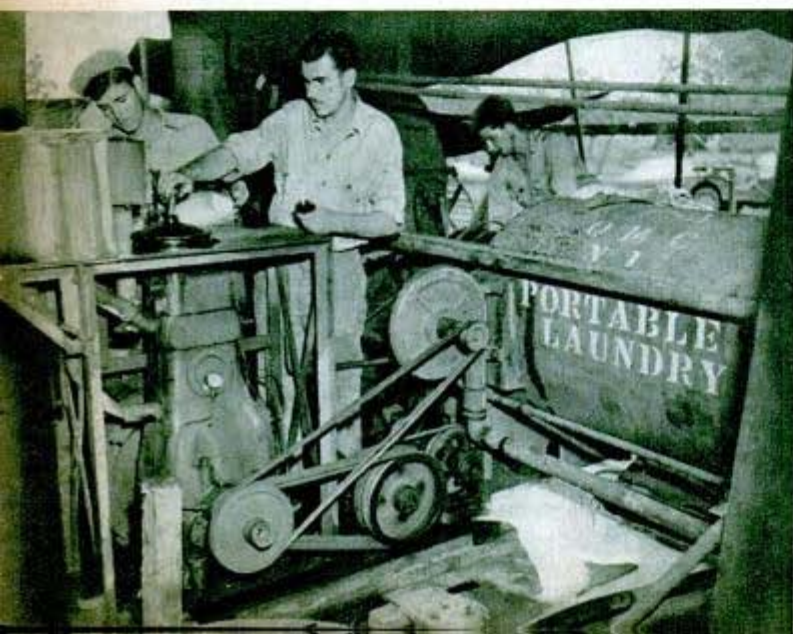
Portable Diesel engine furnishes the power for laundry operations in New Guinea
