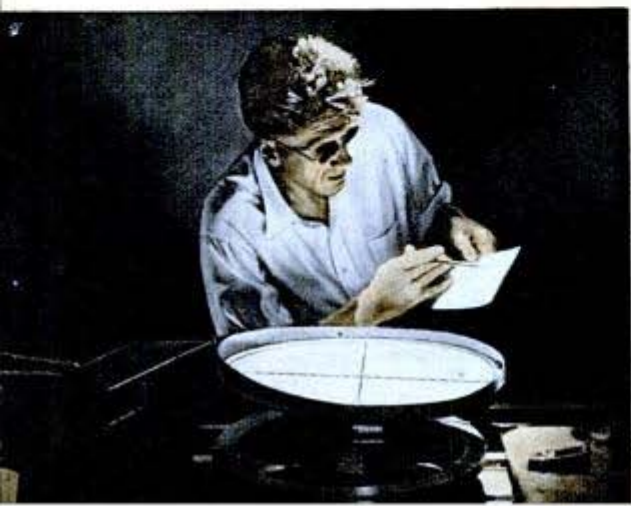
Diagram shows wide area from which eclipse can be viewed. Below, 17-inch disk captures image of sun projected from mirrors atop a high tower
