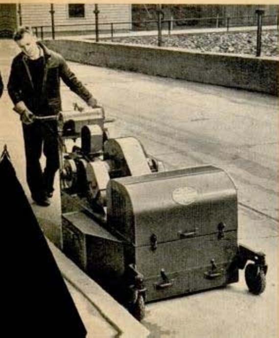
Giant vacuum cleaner (below) removes dust from streets adjacent to buildings. Right, these "pillows" are actually filter bags through which air passes and is cleaned at film plant
