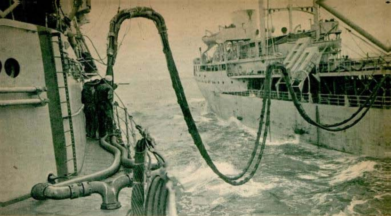
While helmsmen keep the two vessels at equal speeds, a British cruiser refuels from tanker far at sea
