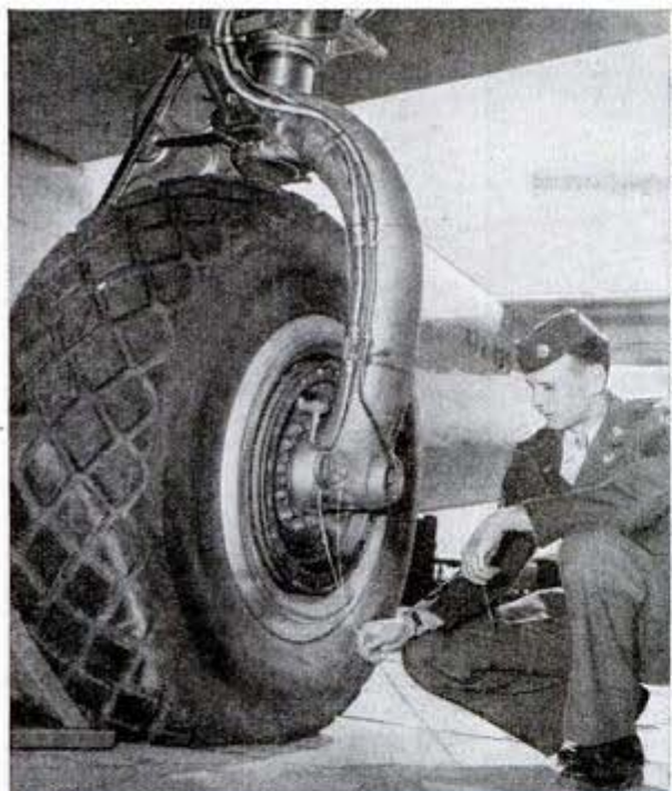
Catwhisker wire, above left, discharges static electricity as B-24 lands. Ferry crew member at right dons "Mae West" life preserver in a forced landing rehearsal. Below, CAA dispatchers in control tower
