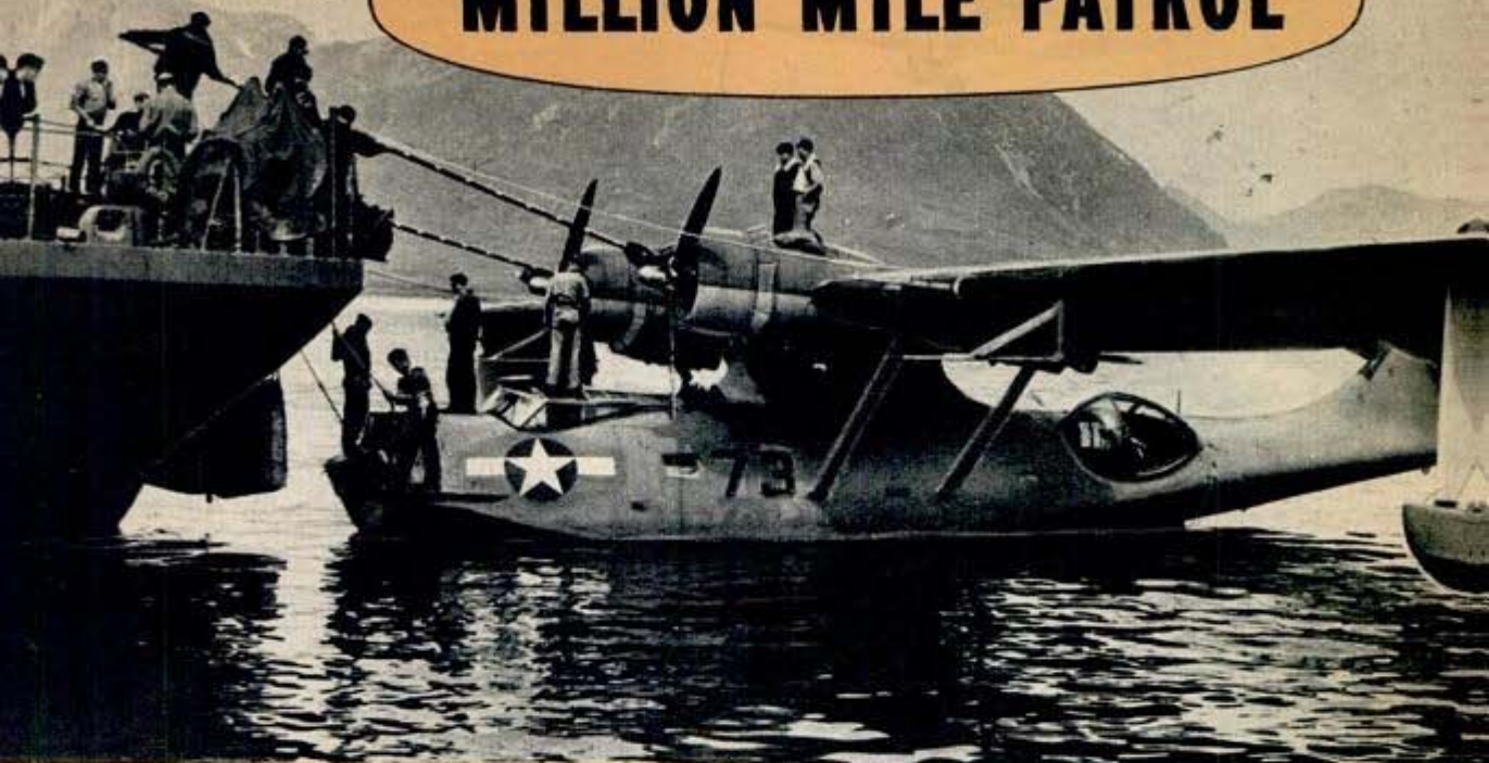
Catalina patrol bomber takes aboard gasoline from a seaplane tender in the frigid Aleutian waters. Bamboo poles are snubbed against the propellers to keep the plane from drifting into the ship's stern
