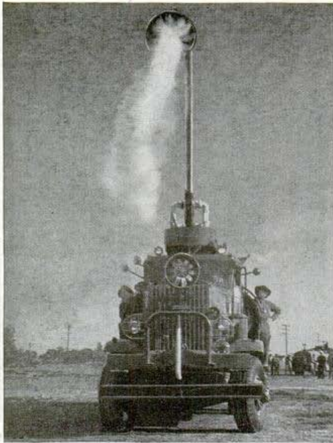
Stream of carbon dioxide and water begins to pour from the overhead boom nozzle of fire truck. Boom is moved from cab
