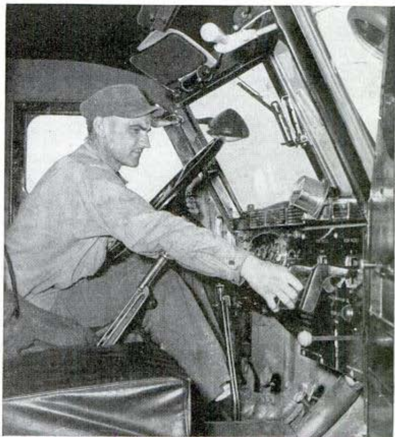
Walter Kidde & Co. photo 140 22 JAN 47 NY 6 NY Drawing shows built-in fire extinguishing system for plane engines. Pilot pulls handle and carbon dioxide from perforated ring kills blaze. Below, levers in cab of fire truck control overhead boom and nozzles
