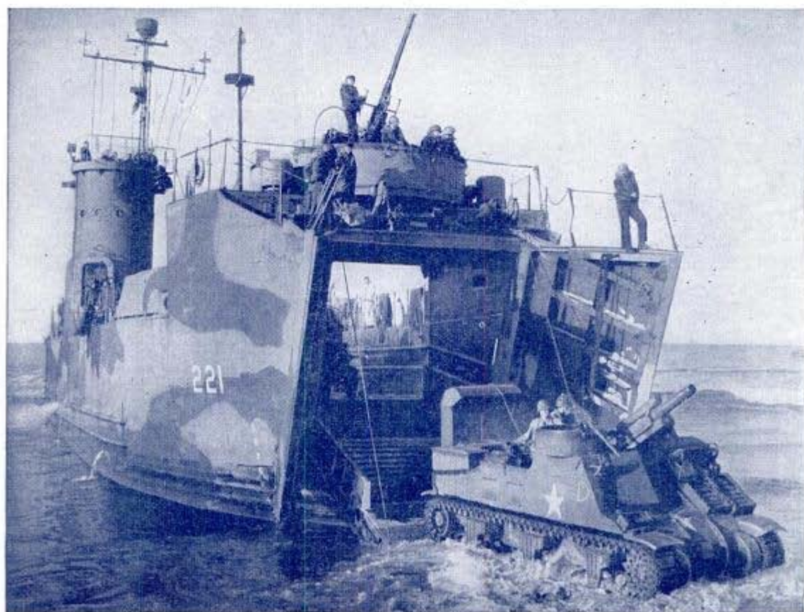
Barrage balloons hover above landing ships and beach storage points to help prevent attack by enemy aircraft. Below, a self-propelled howitzer on a tank chassis drives through the surf toward a beach from the ramp of an LSM. In an amphibious assault, each weapon moves toward the shore on a split-second schedule
