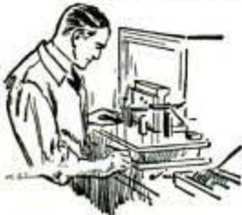
Checking a Fixture with Precision Gauges.
