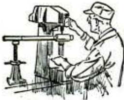
Testing the Hardness of a Carburized Headstock Spindle Bearing Surface.
