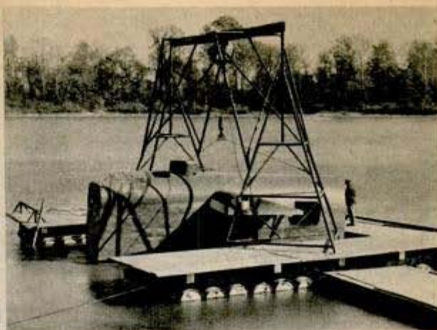
Mockup of B-24 bomber, above, is lowered into water for "walk-around" air unit test. Left, flyer emerges after several minutes under water and stands erect without showing any ill effects
