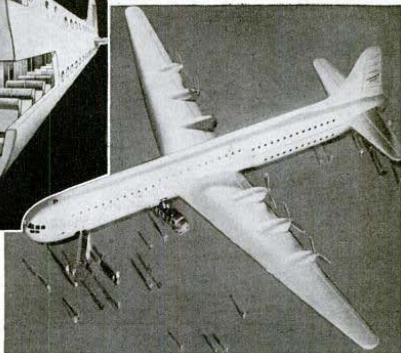
Upper deck of Clipper as shown in cutaway is divided into two passenger sections. Lower deck has rooms, seats. Right, model of plane
