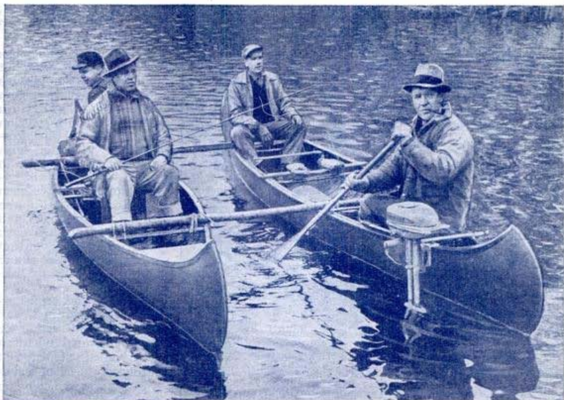
One outboard motor does work of two on these canoes. Left, flies dipped in solution of paraffin and gasoline will float like new
