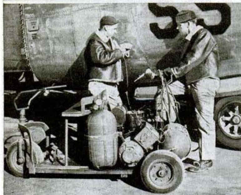
Tank track is welded with unit brought by "welder-jeep," top. GIs repair skin of B-24's nose, left, with mobile metal shop
