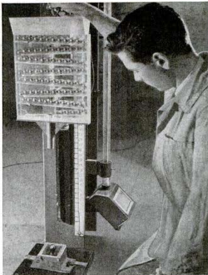
Steel balls are dropped repeatedly on Plexiglas panel to see if it is tough enough to be installed as a blister in bomber
