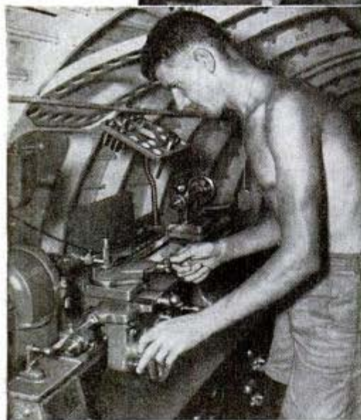
Interior views of a Commando Flying Machine Shop of the XX Bomber Command equipped with a South Bend Lathe. Official U. S. Army Photos.
