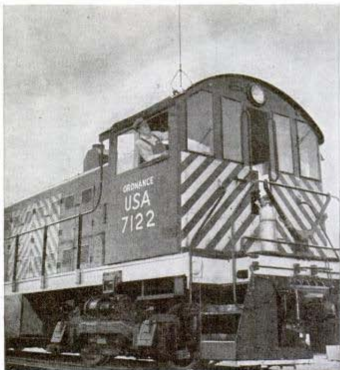
In case of fire, grab Mike. Note the aerial, above, on Diesel switcher cab in arms yard. Right, engineer tests his radio equipment
