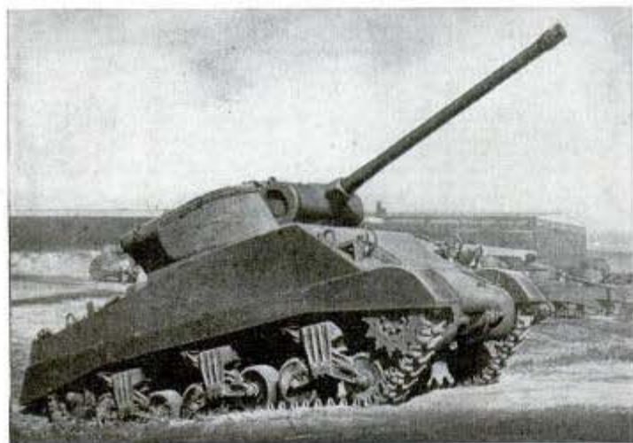
This 3,000-horsepower Allison engine is said to be the most powerful aircraft engine in the world. Below, the new M-36 tank destroyer mounts a 90-mm. cannon in heavy turret on the hull of an M-4
