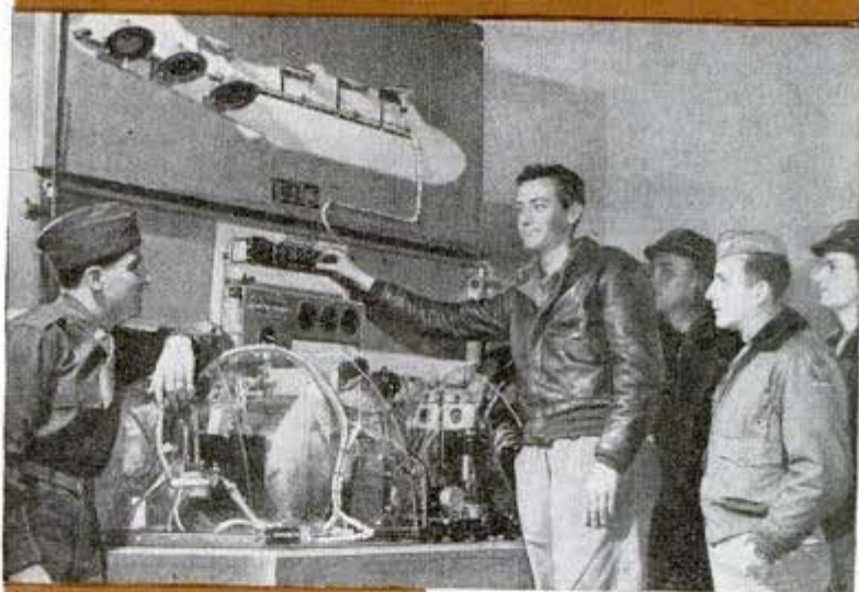
Below, in shadow of "Flak Alley Lil," crew chiefs get latest dope on servicing B-17 oxygen system
