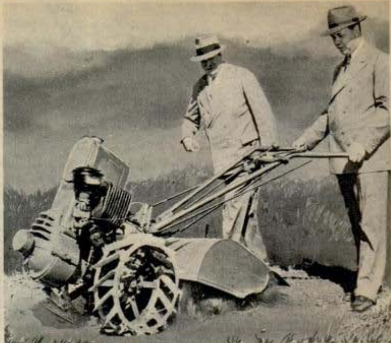
Left, Rototiller making soil "cement." Above, it churns earth into even seed bed
