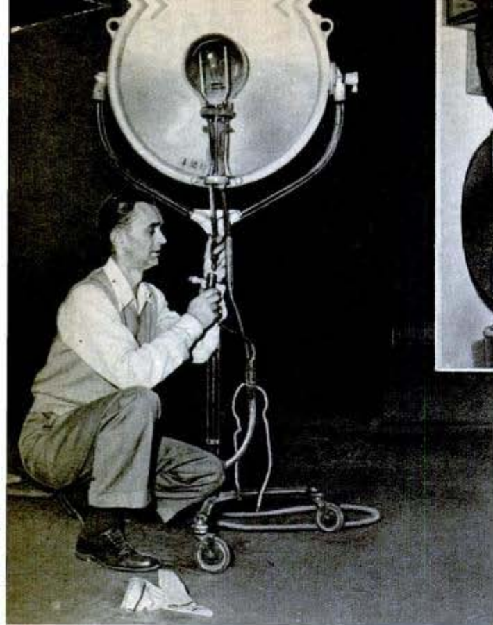
Hollywood technician uses 5,000-watt bulb in front of shallow reflecting surface to give soft lighting. Below, home movie screen is mounted behind draperies
