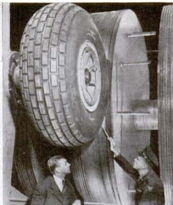
Airman (left) can quickly release steel and canvas flak vest by pulling strap attached to shoulder lacing. Right, inertia brake testing machine at Wright Field slams tire against spinning steel
