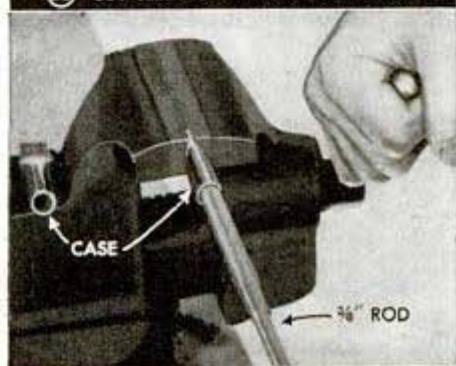
23 SQUEEZE 3/8" FLAT AT SMALL END
