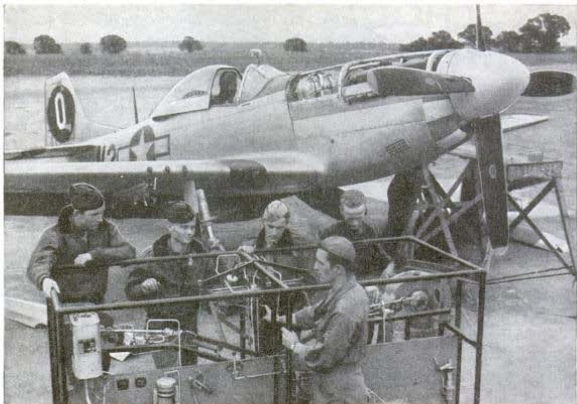
Unit hydraulics instructor uses mockup to explain the new emergency landing gear on Mustang to pilots
