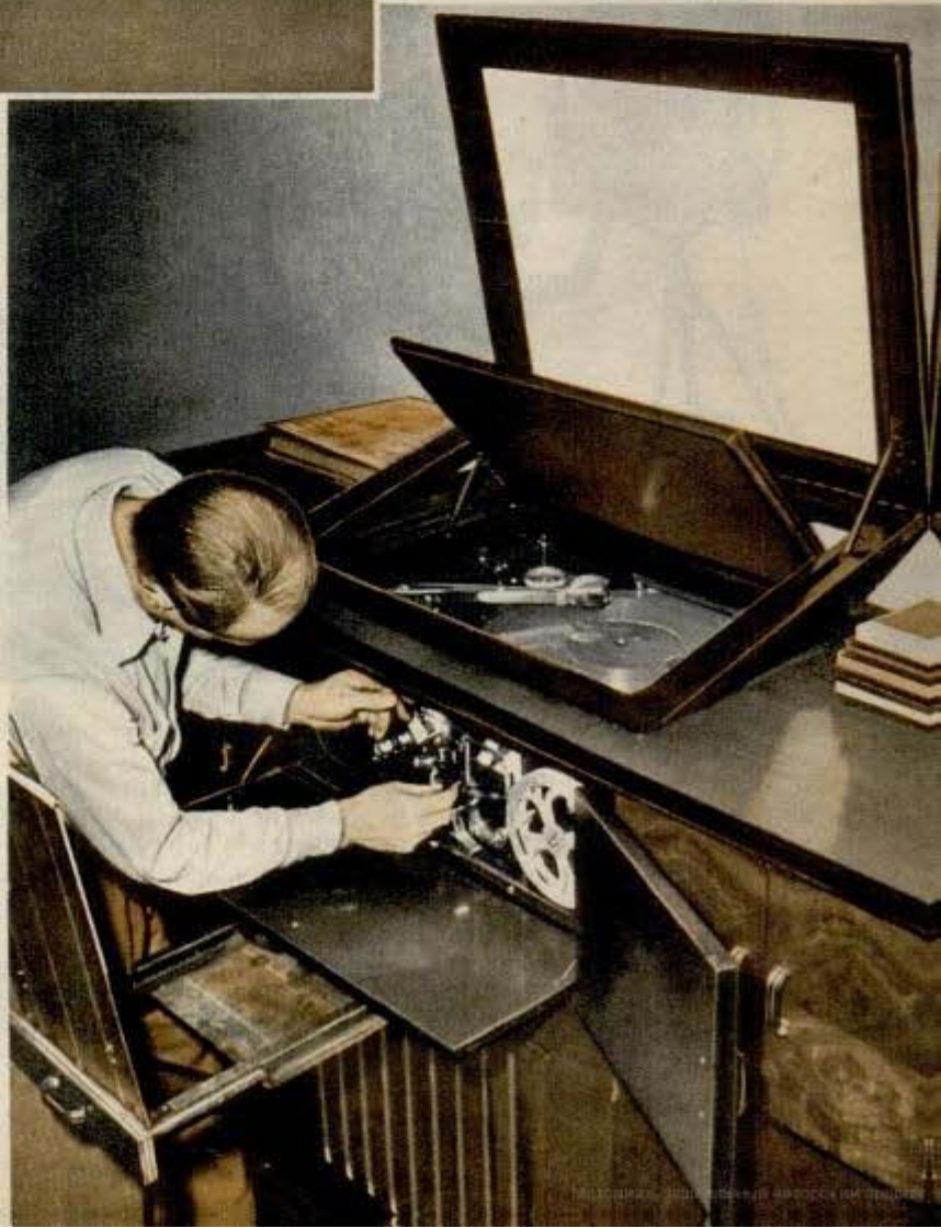
A 16-mm. camera contrasted with the huge $16,000 type used in Hollywood. At right, phonograph synchronizes with film which is projected to mirror (lower left) that reflects it to the screen above
