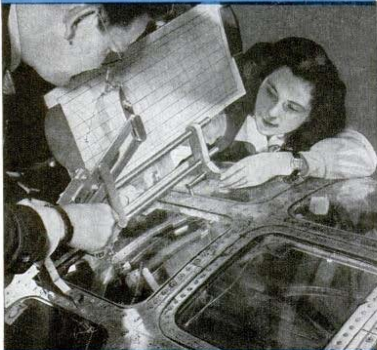
This instrument tells exactly how much pressure an airplane window can withstand in stratosphere. Below, Western Electric engineer tests a sample of brass sheet for tensile strength and elongation
