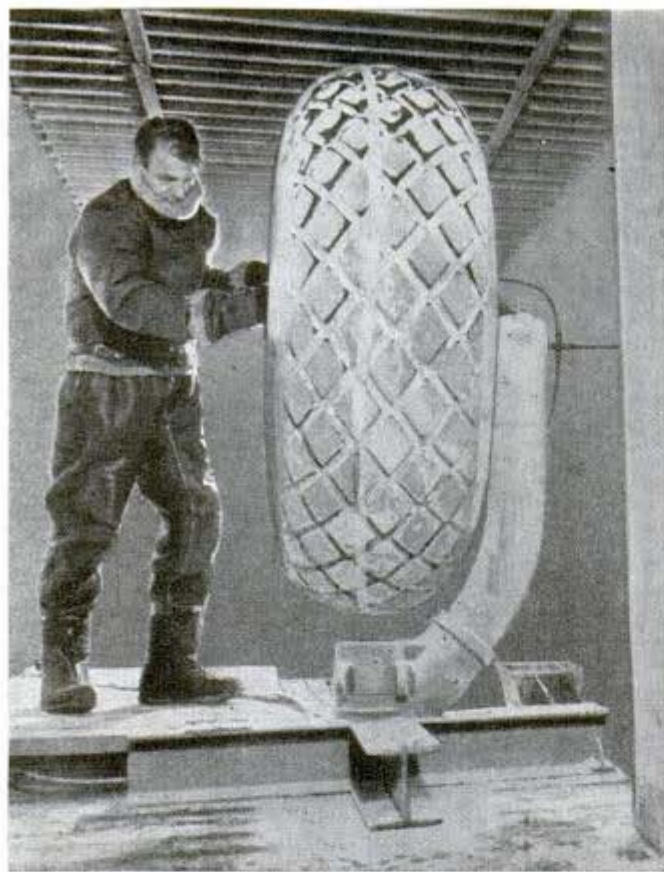
Liberator bomber's brakes are tested at 65 degrees below zero
