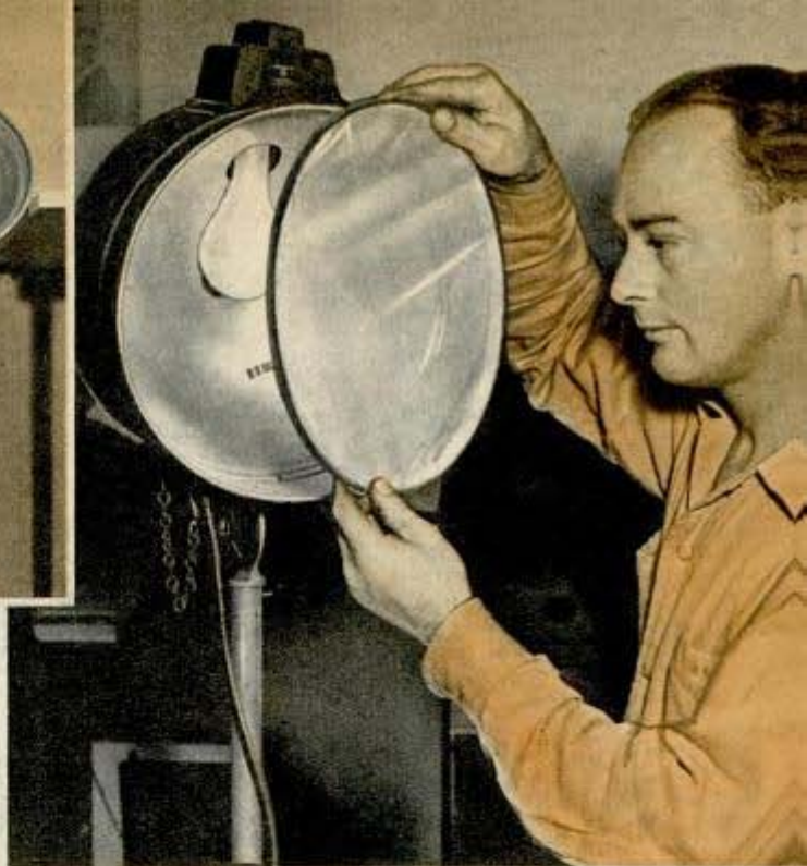
For indoor lighting amateur uses a specially wound transformer to double output of photo-floods. Right, scrim softens light for close-ups
