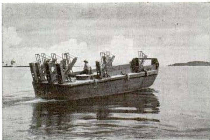
Little boats like the LCVP (above) pack the wallop of a much larger vessel, thanks to the installation of portable rocket-launching racks Official U. S. Navy photo
