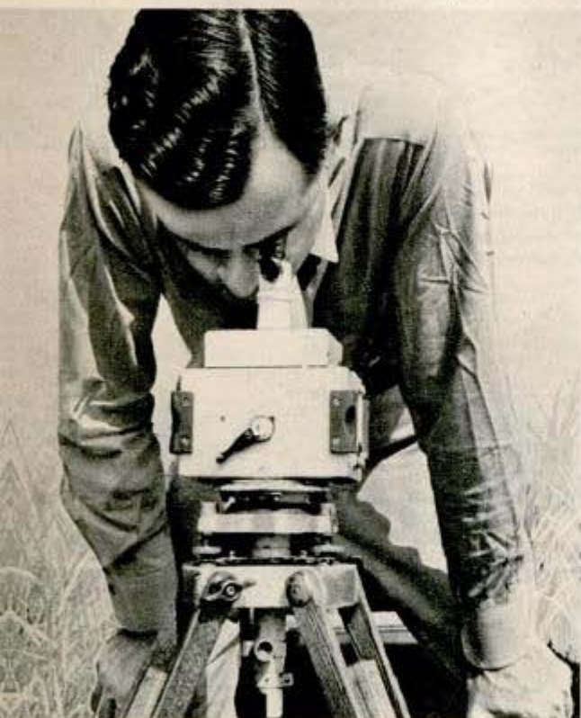
Above, preparing to run casing gun perforator into hole. Left, reading magnetometer which reveals mass of rock under ground that may form oil basin; gravity meters are used for the same purpose. Midway on derrick below, operator can be seen steadying pipe as rotary helpers on the floor below "stab" the pipe
