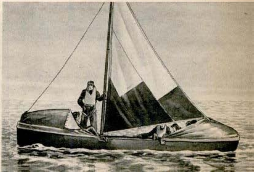
Top, motor sailboat is dropped from bomber by parachutes (inset), which carry it gently to water. As the boat hits the sea, two 150-yard buoyant lines (above) are shot out by rockets, enabling the castaways to pull themselves to the craft. Below, rescued airmen hoist sails of airborne lifeboat and head for shore
