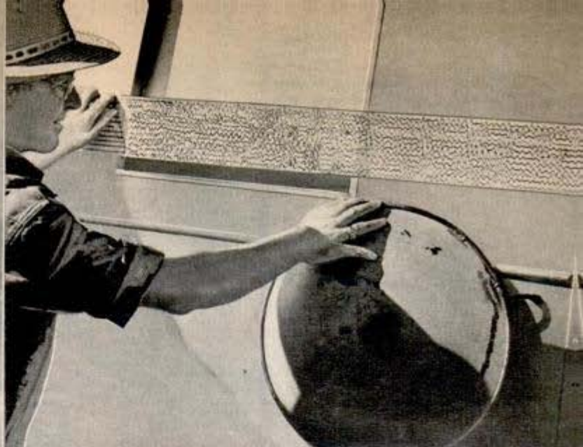
Man-made "earthquake" recorded by seismograph helps determine depth and angle of rock formations to reveal possible oil traps in earth
