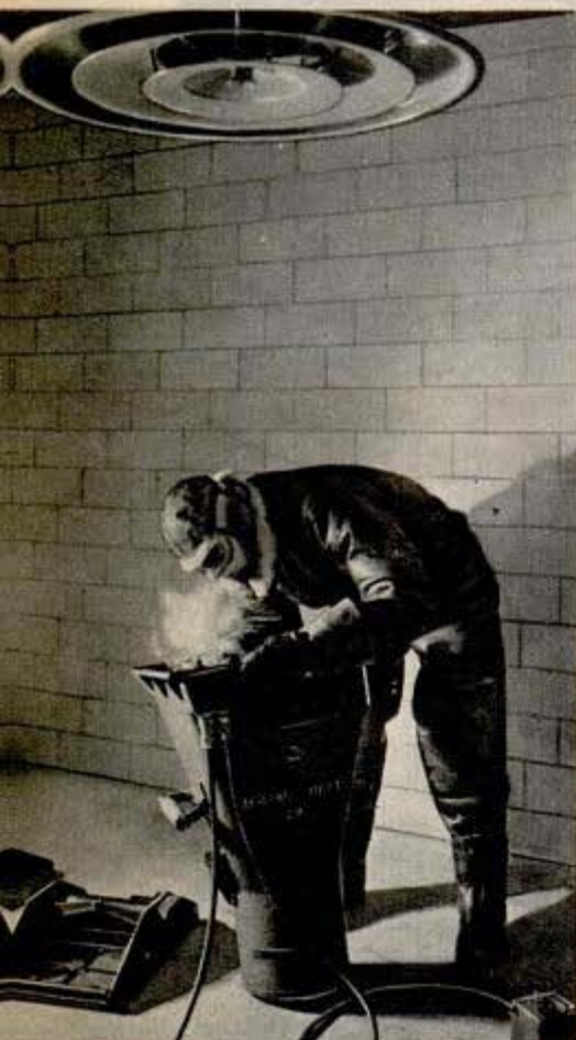
Above, testing aerial camera at 90 below zero in "Arctic" room guards against failure on operational flights. Right, drying cabinet on the "assembly line"
