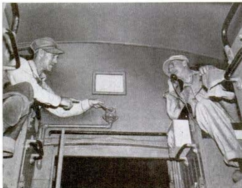
Trainman points to unneeded emergency valve for airbrake as conductor calls engineer Santa Fe photo
