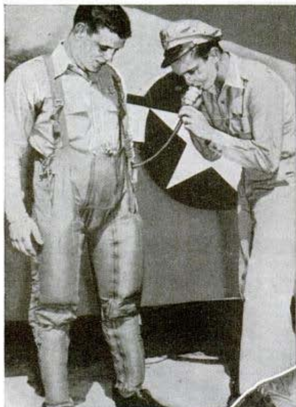
Top, left, pilot has his anti-gravity pants inflated. Top, right, RCAF officer with the accelerator which tested the suit
