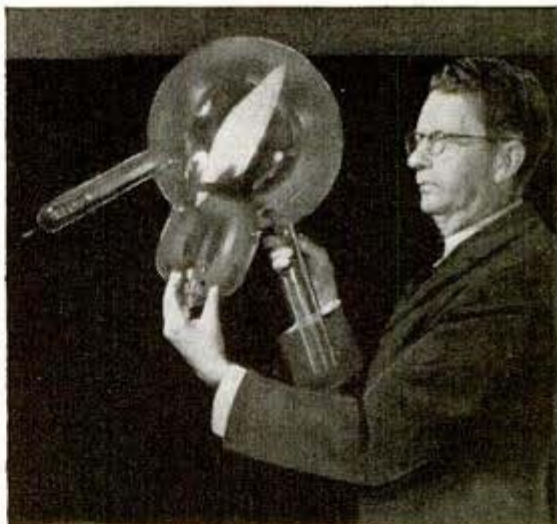
Above and at right, the cathode-ray tube which gives television in color. Below, Fig. 1 shows arrangement of phosphor coatings for two colors. Fig. 2 shows two surfaces on one side of the screen for a 3-color system
