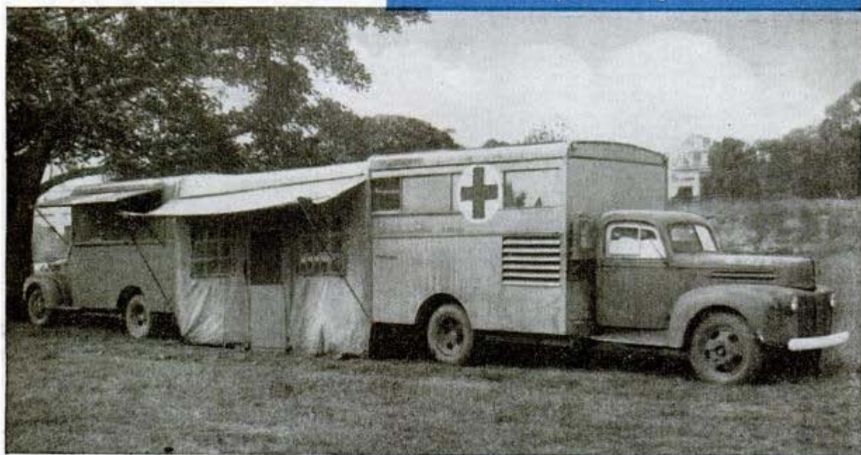
Courtesy William R. Warner & Co. Intravenous solutions of dextrose and of sodium chloride are sterilized in this autoclave at 240 degrees Fahrenheit. Below, kitchen and refrigerator unit of mobile hospital is formed by two vans back to back. Units like these kept pace during race across France
