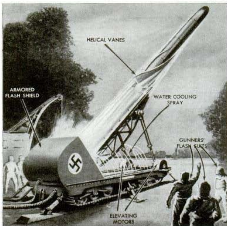
Artist's conception of portable launching ramp for V-2
