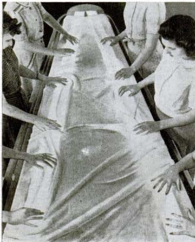
Above, world's record for low leap—82 feet by Carl Rupert in a theater. Below, modern chutes are repeatedly inspected. Here a completed chute is examined under fluorescent lights
