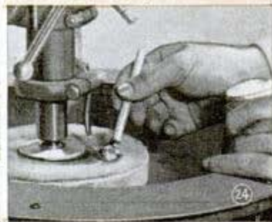
10—Polish on felt wheels. Keep wheel wet with tiny trickle of water. Speed 1200. Use moderate to heavy pressure (see text)
