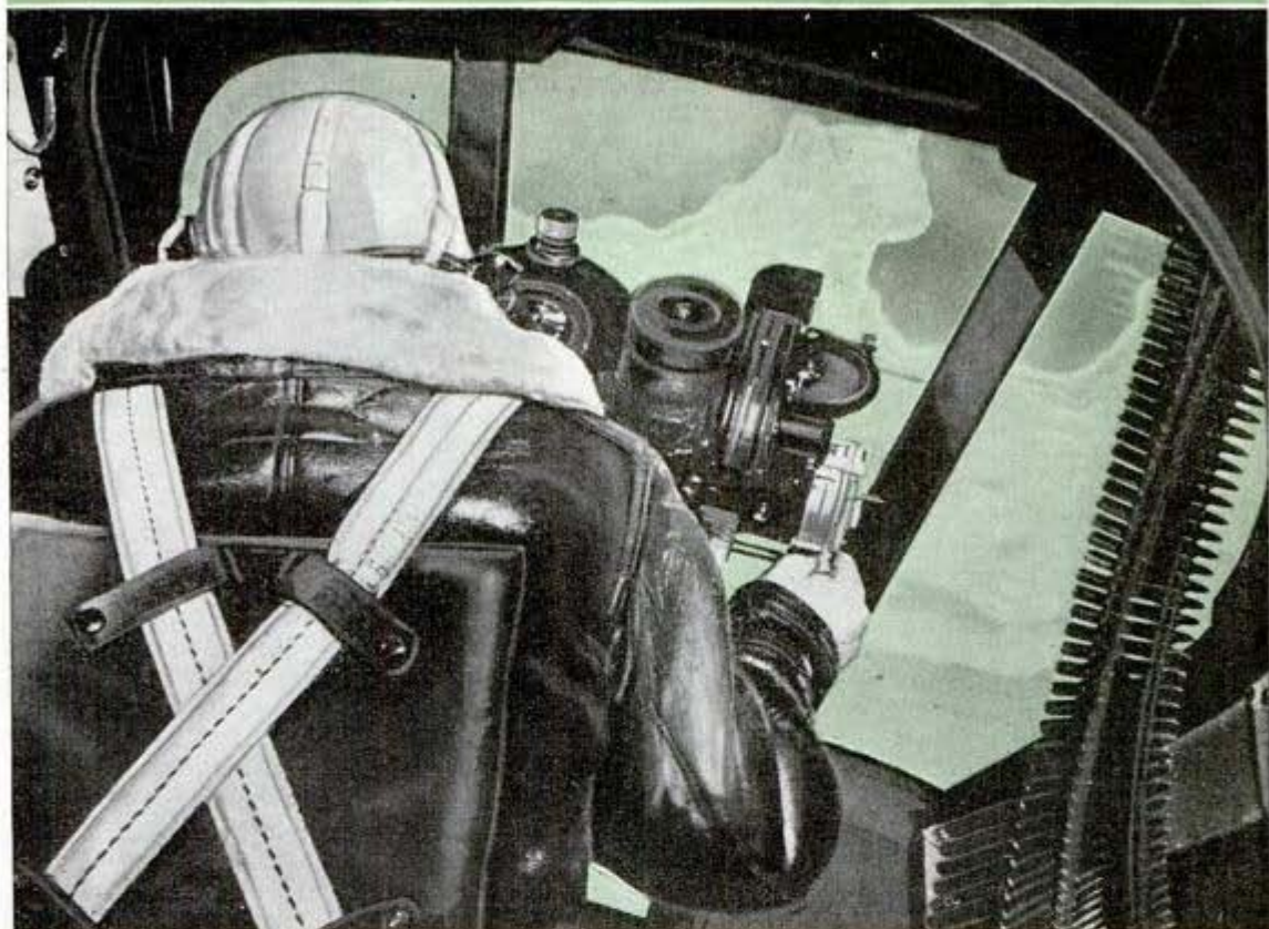
Nearing target, bombardier makes few simple adjustments—the Norden bombsight's "brain" does the rest
