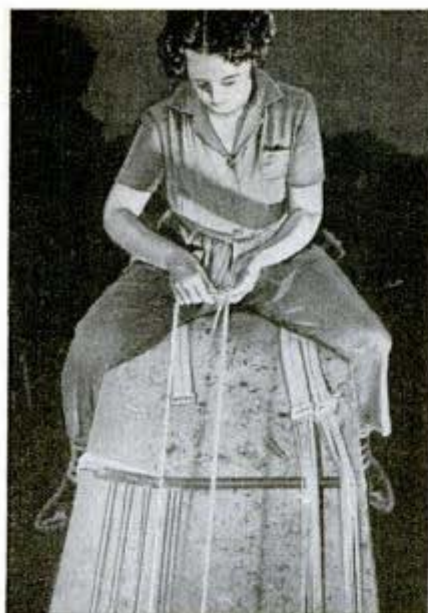
Above, attaching shroud cords to the straps of a parachute
