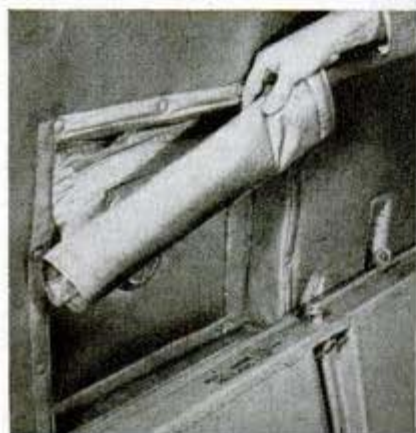
Top, right, pilot's seat in a C-46 next to quilted Fiberglas. Top, installing the cloth in a B-29 fuel cell. Above, insulating a window
