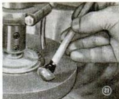
7—Further smooth the stone, using 100 and 220-grit wheels in succession. Keep wheel wet to avoid burning. Speed 1200-2400
