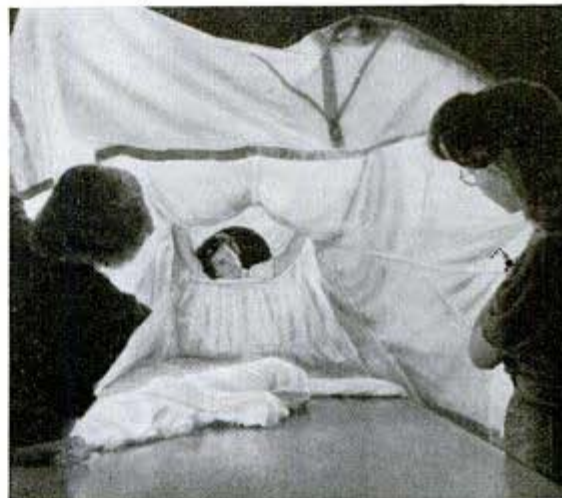
Above, life vest for stranded flyers. Below, examining vent through which air escapes as chute descends
