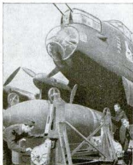
At top, one of the original six-ton "blockbusters" is readied for loading into a Lancaster bomber. The new six-tonner, lower right, has a sharply pointed nose and can pierce 12 feet of concrete before exploding
