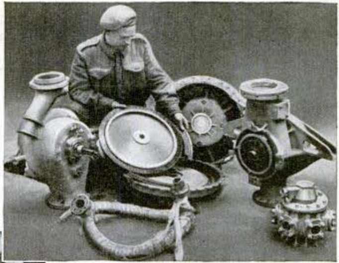
Inspecting turbo pumps of wrecked V-2; fuel pump is at left, liquid air pump right. Left, Allied soldiers remove parts of V-2 found in field in Belgium
