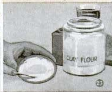
9—Mix polishing abrasives with clay flour and water to form a paste. Use F-grit silicon carbide for first polish; tripoli for final
