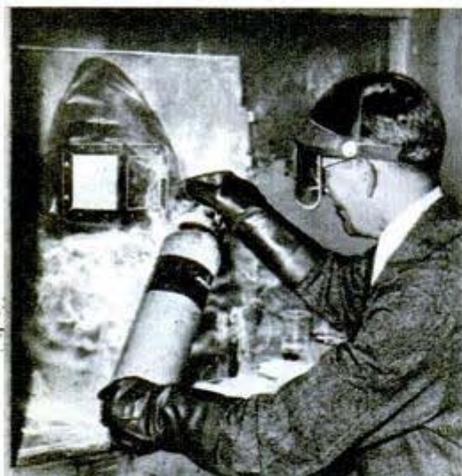
Left, top, sandless glass lens at right stays transparent after acid attack but other lens turns opaque. Left, chemist spraying acid against a protective hood
