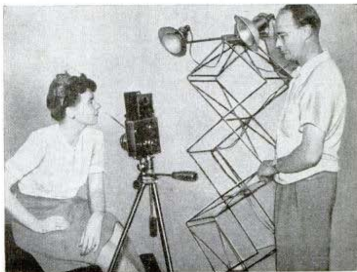
Above, installation of aerial cameras in nose of Lockheed P-38 Below, floodlamps on lazy tongs are raised and lowered easily
