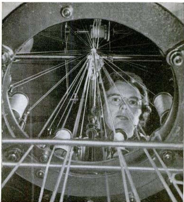
Above, nylon threads are woven into parachute shroud lines. Below, suspension rig determines how harness innovations fit under body weight
