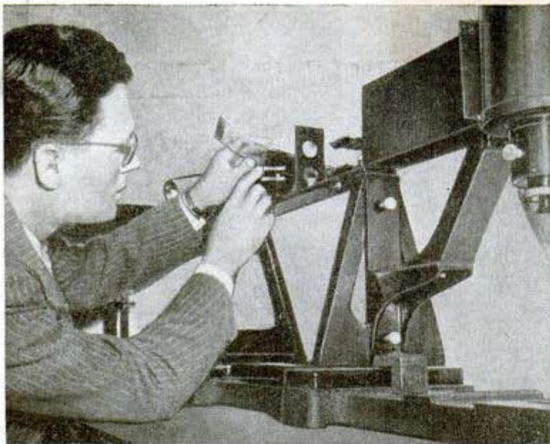
Placing test strip of filter emulsion in spectroscope to analyze color
