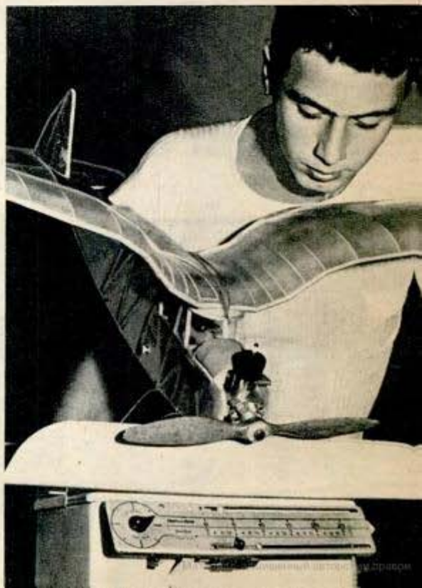
Twin boom endurance plane (above) similar to P-38 Lightning is ready for launching test. Below, weighing model plane. This one has a gross weight of just under fifteen ounces
