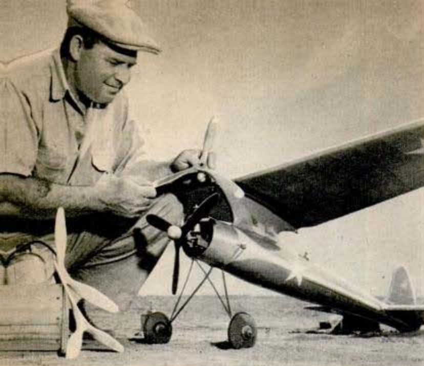
Above, substituting a propeller of a different pitch. Some propeller tip speeds reach 45,000 feet a minute
