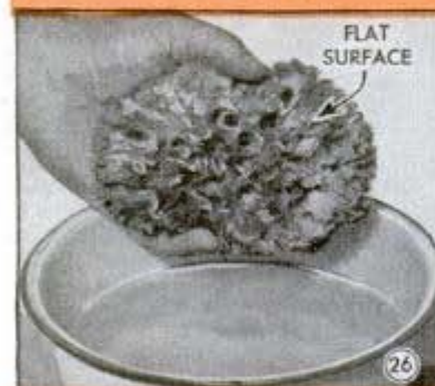
SPONGE MOTTLE —Trim sponge so that it has a flat side. Dip in water to soften, then wring dry. Press onto the color slab, Fig. 27, then transfer the paint to the wall. Two color mottles are very effective
