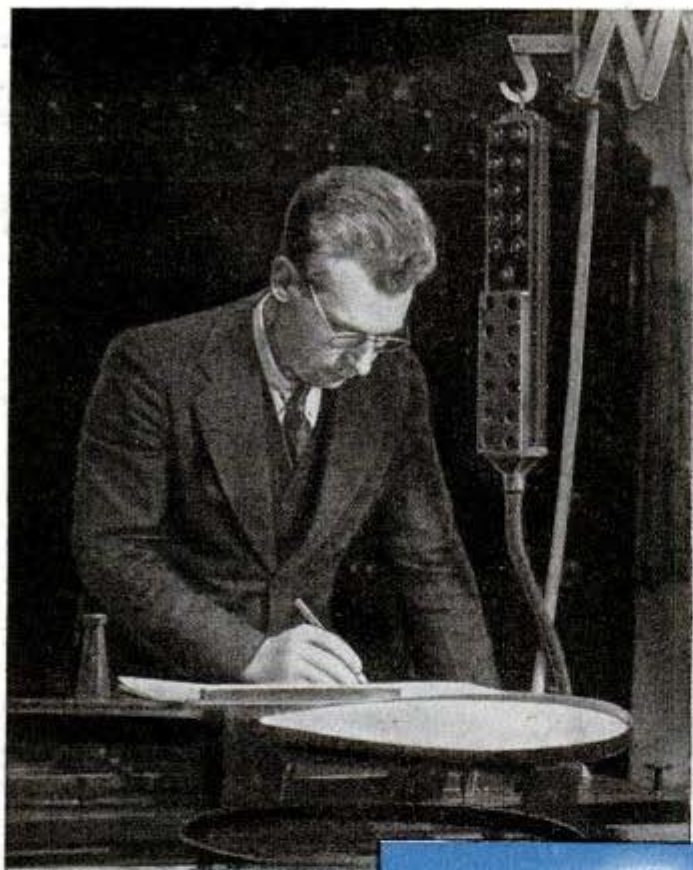
Image of sun is projected from high tower to disk in the foreground. Right, a total eclipse
