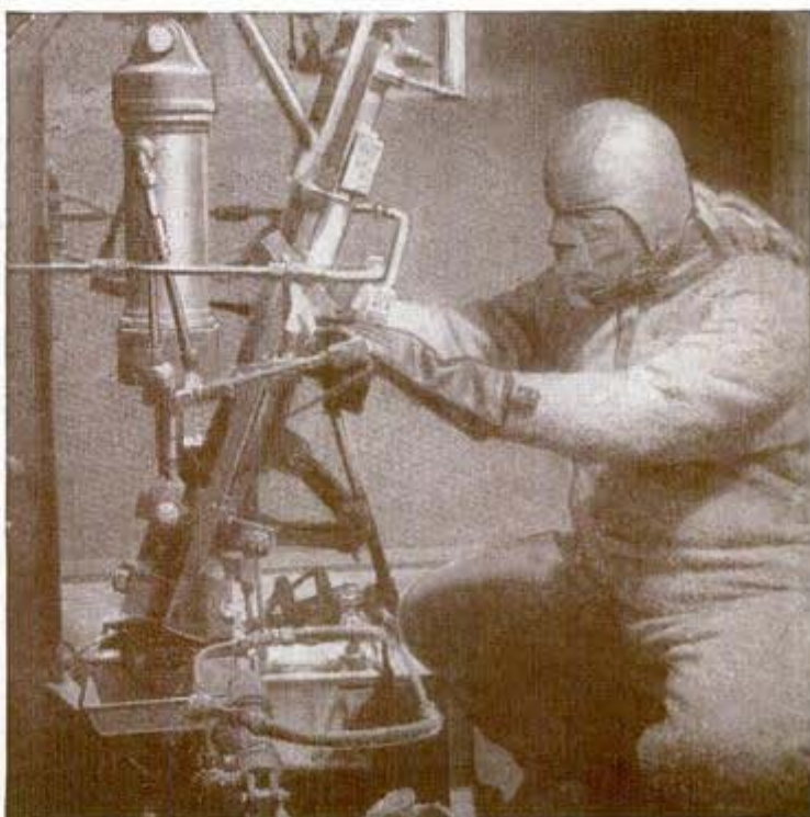
Above, engine is adjusted before being tested on a horizontal engine stand. Below, oleo strut is tested at 65 degrees below zero
