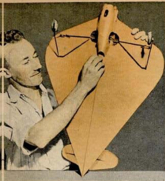
Above, flying wing's landing gear retracts into hull due to centrifugal pull when it is flown on a control wire. Right, interior of tiny motor
