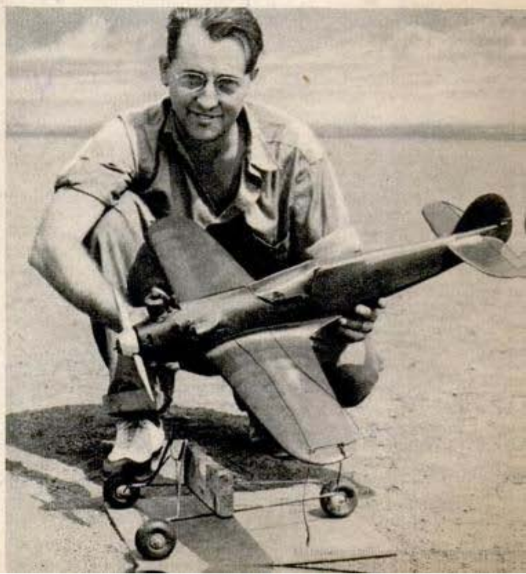
Below, high speed scale model of Messerschmitt that does 106 miles per hour, held above its takeoff dolly from which it rises into the air
