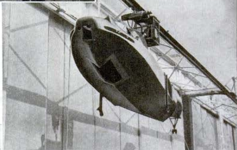
Overhead crane (above) lowers a nose machine gun turret into a B-24. Right, monorail crane takes sub-assembled hull of a Catalina PBY-5A flying boat to a final assembly line at Consolidated. Below, a small "lifting dolly" picks up a huge Pratt & Whitney engine for transfer to the Consolidated plant's final assembly line for installation in a Liberator. The company's intricate and efficient transportation system allows it to operate at full speed without stock piles
