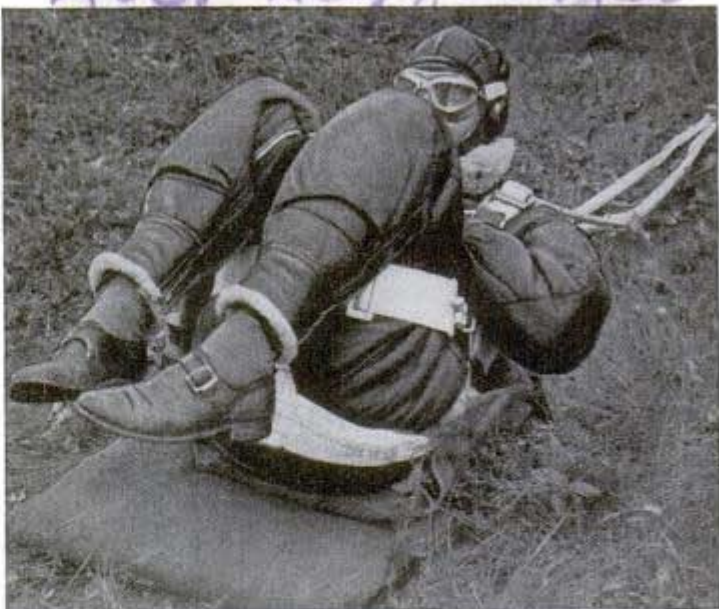
Sgt. Harry C. Conway, second man to demonstrate human pickup, is ready for takeoff in special harness which holds his knees against his chest. He wears a winter flying suit
