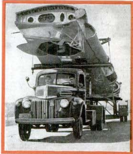
Trays full of small parts are moved from station to station by a "lifting dolly" (above) at Consolidated Vultee Aircraft. Below, a truck hauls wing center section of a Liberator bomber from a sub-assembly plant
