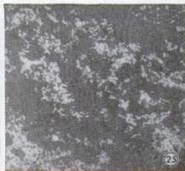
ROLLER MOTTLE —Pick up color on roller, Fig. 23, then apply roller to wall, being careful not to overlap. Two times over makes a heavier mottle, as shown in Fig. 25. Use a stippling roller, not a roller coater
