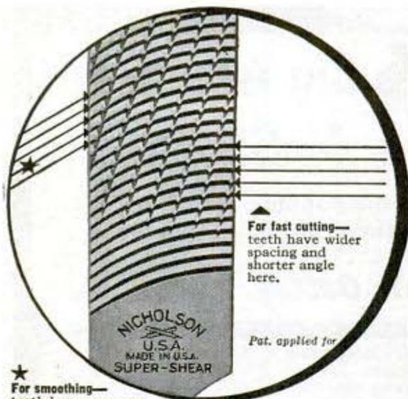
For fast cutting—teeth have wider spacing and shorter angle here.
