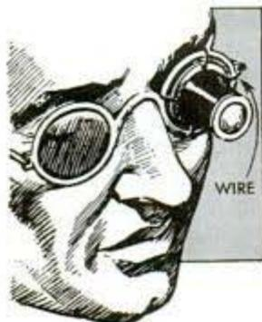
A magnifying eye-piece used in reading fine print or in close-inspection work can be held in place comfortably and securely by attaching it to an old pair of sun glasses from which one of the lenses has been removed.
