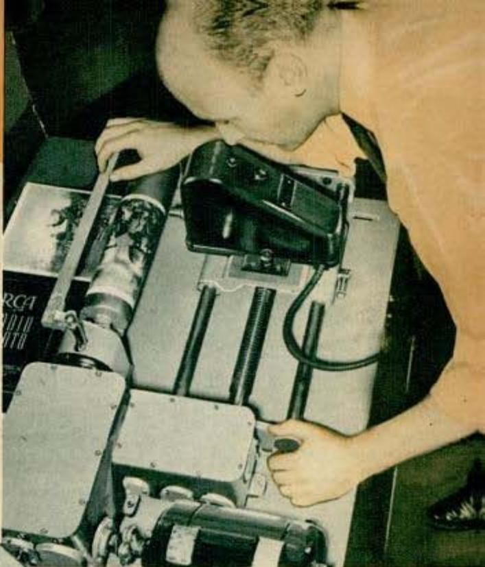
Upper left, monitor receiver which makes pictures constantly visible by means of ink spray as they are being received. Above, RCA operator adjusts radiophoto receiving machine before tuning in a distant transmitter. Below, engineers in control room of a television studio
