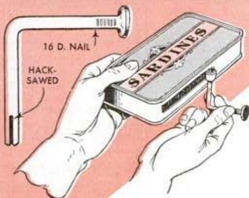
If a key to open sardine cans and similar containers is not at hand, you can make one from a large nail. Bend it at right angles in the center, cut off the point and slot the end. This can be done easily with a fine hacksaw blade if the nail is gripped firmly in a vise
