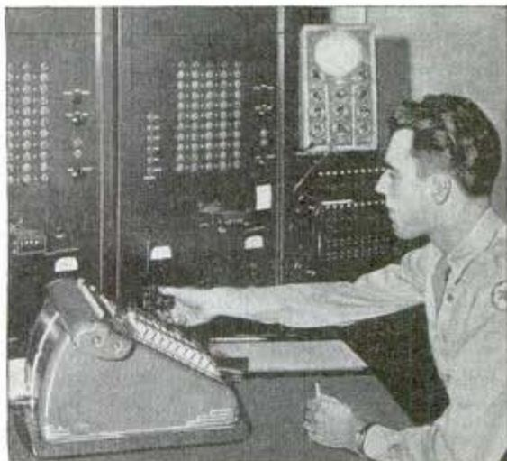
Taking readings of velocity of projectiles at arsenal. Below, gun and test towers
