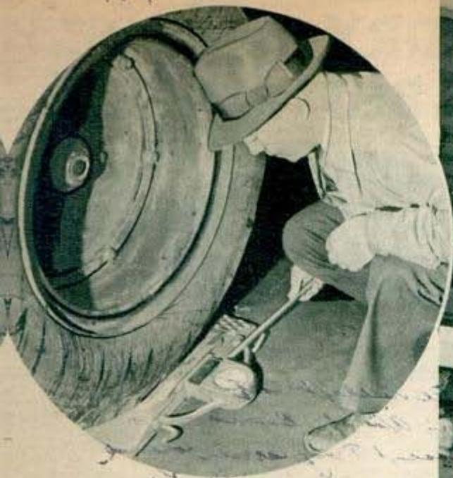
**B. F. Goodrich Co.** uses this scale to detect mismatched, misaligned, wrongly inflated tires
