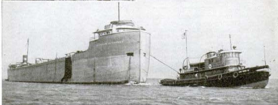
divers in bags, was applied to make the tank seams airtight. After being emptied, the tanks were to be partly filled to assist in the raising job. Theoretically, the Humphrey could have been raised by blowing enough air into her repaired tanks, but that probably would have resulted in her turning over.
