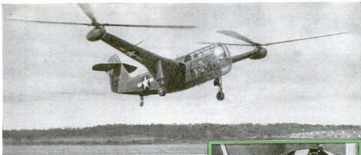
Hovering over Wright Field is the Platt-LePage XR-1, a dual-rotor helicopter undergoing tests for the Air Forces
