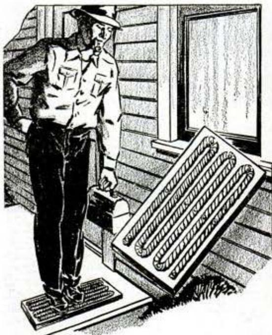
If you want a door mat that will last indefinitely under severe use, just nail some  $\frac{3}{4}$  or 1-in. rope to a wide board as indicated. This mat is especially suitable around a cabin during rainy weather.
