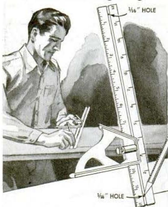
To convert an adjustable square into a marking gauge, drill a  $\frac{1}{16}$ -in. hole  $\frac{1}{2}$  in. from each end as shown. In use, set the gauge at the required distance, insert the tip of a pencil through the hole and slide the square along the edge of the work to mark off the line.
