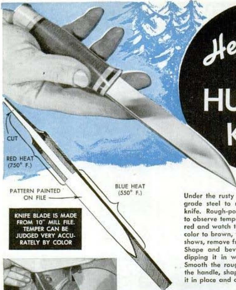
KNIFE BLADE IS MADE FROM 10" MILL FILE. TEMPER CAN BE JUDGED VERY ACCURATELY BY COLOR
