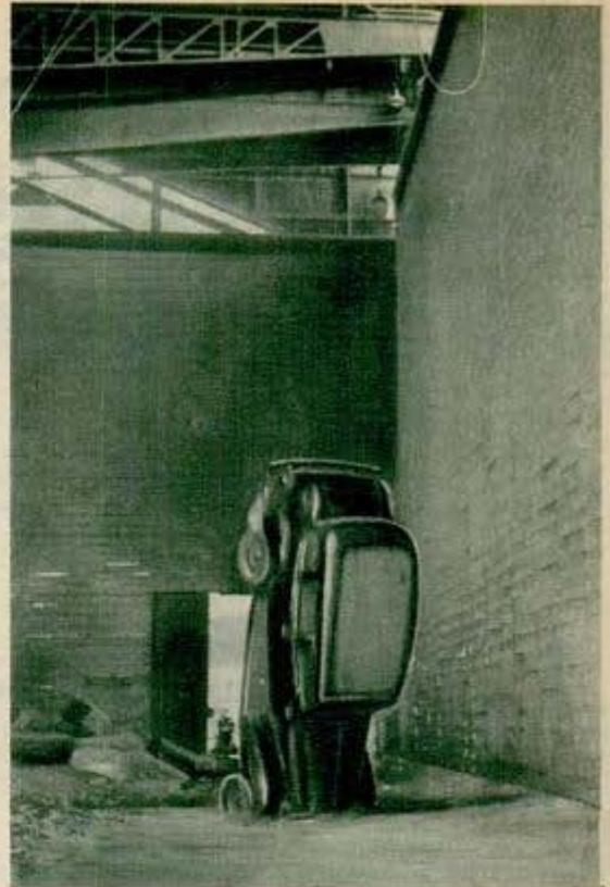
Left, sedan is hoisted by 40-foot crane and dropped on nose (above) to simulate collision at 35 m.p.h.
