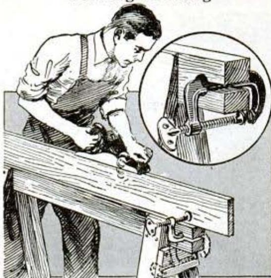
When you wish to edge-plane short boards on a sawhorse, you can hold them with a C-clamp which is kept handy in a keyhole slot cut in one end of the horse as indicated. The clamp may be raised, dropped out of the way or removed from the sawhorse easily when desired.
