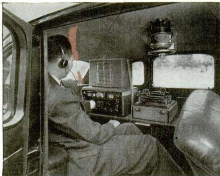
Taking close range bearing from mobile unit; note wax cylinder recorder. Right, terminus at primary station for the feeders from eight antennas
