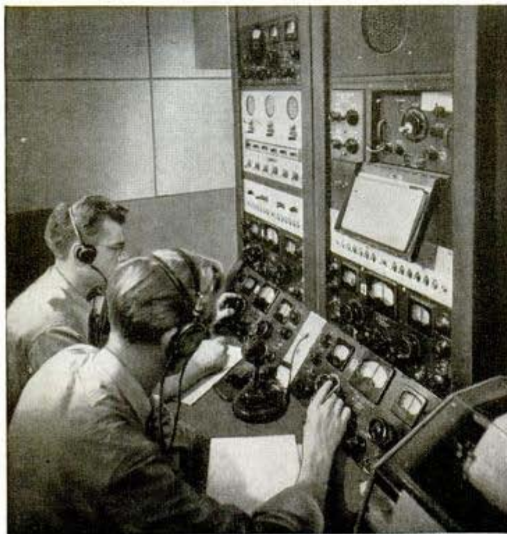
Hunting clandestine radio transmitter, operator rotates direction finder; calibrated scale indicates bearings of hunted signal. Above at right, huge direction finder has H-shaped antenna to locate signal within one or two degrees. Below, monitoring officer exchanges data over microphone with operator at direction finder
