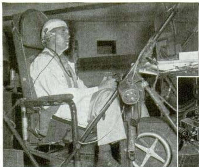
Left, Air Force corporal, wearing a molded brain-wave recorder, prepares for a test blackout run. Below, a technician sits next to centrifuge pivot shaft as an observer. She talks to control room
