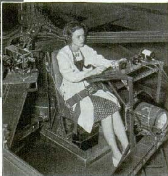
Left, Air Force corporal, wearing a molded brain-wave recorder, prepares for a test blackout run. Below, a technician sits next to centrifuge pivot shaft as an observer. She talks to control room
