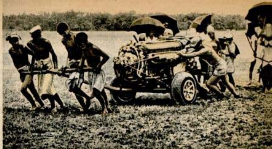
The engine removed from the P-40 is trundled over two miles of mud on a cart constructed from landing wheels of a salvaged airplane
