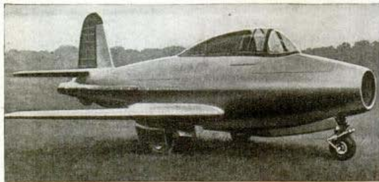
Above, the P59A Airacomet, first American jet plane. Below, the British Gloucester jet plane with intake vent in nose, propulsion vent in tail
