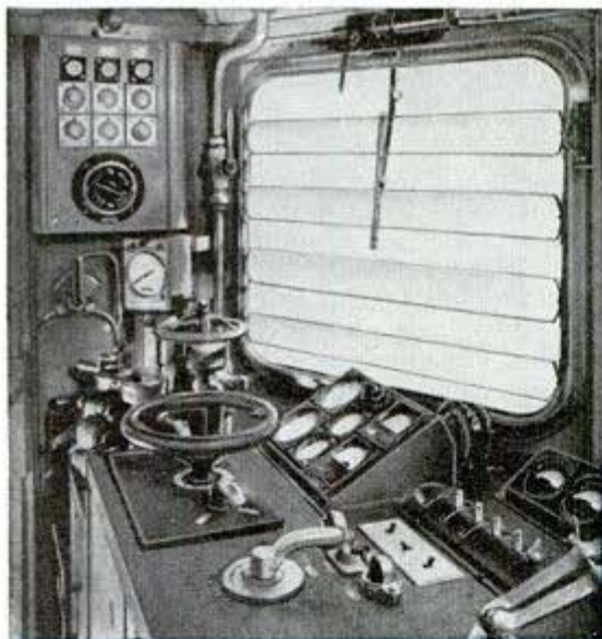
Left, engineer's room of gas turbine locomotive (below) built by Brown, Boveri for Swiss railways
