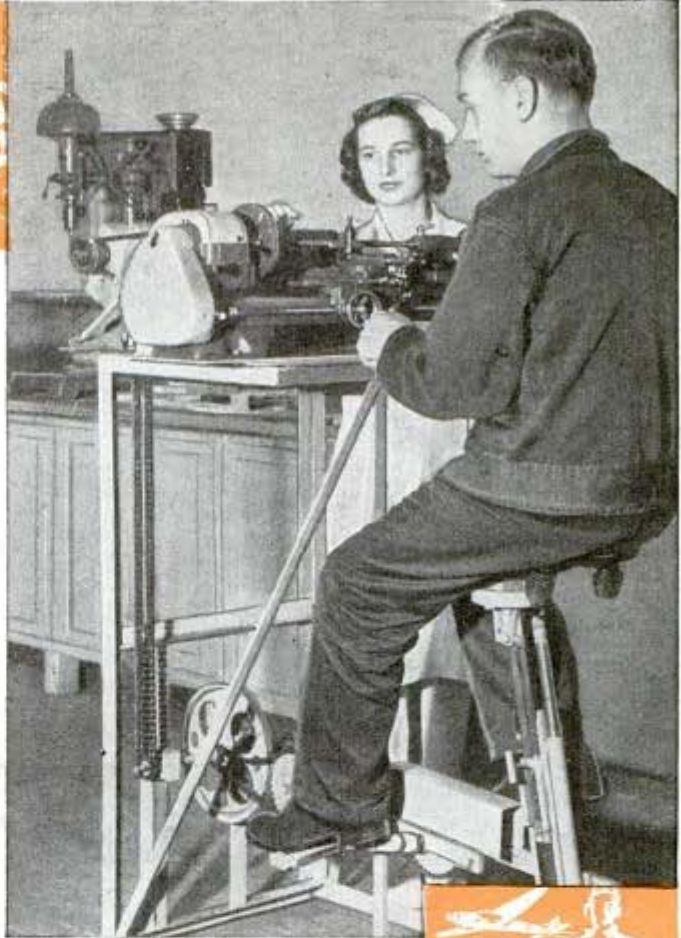
Motor is removed from lathe and foot-power substituted to strengthen leg
