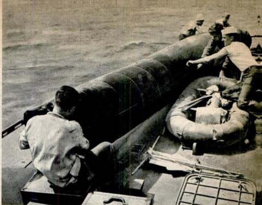
PT "cowboys" check their shootin' by examining aerial sleeve target that caught the fire of the motor torpedo boat's machine guns. Bullets used in the tests leave painted marks on sleeve to register individual hits
