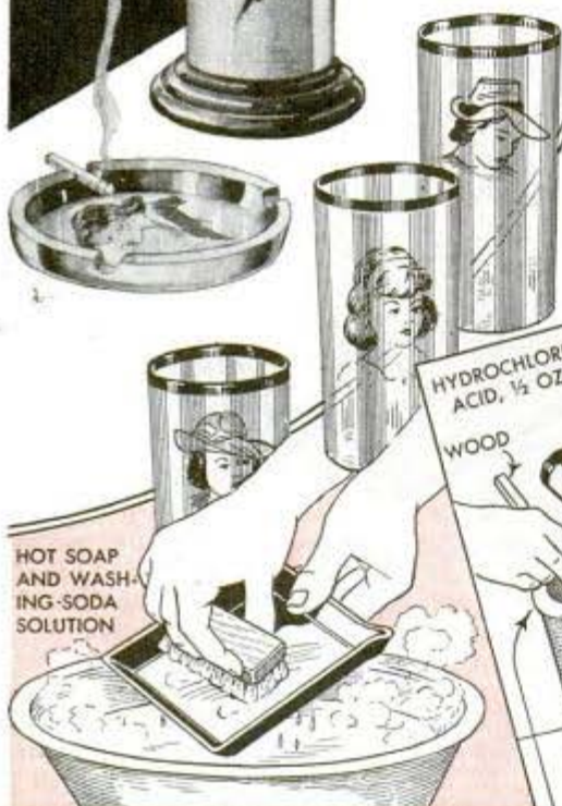
① METAL SURFACES THOROUGHLY CLEANED
