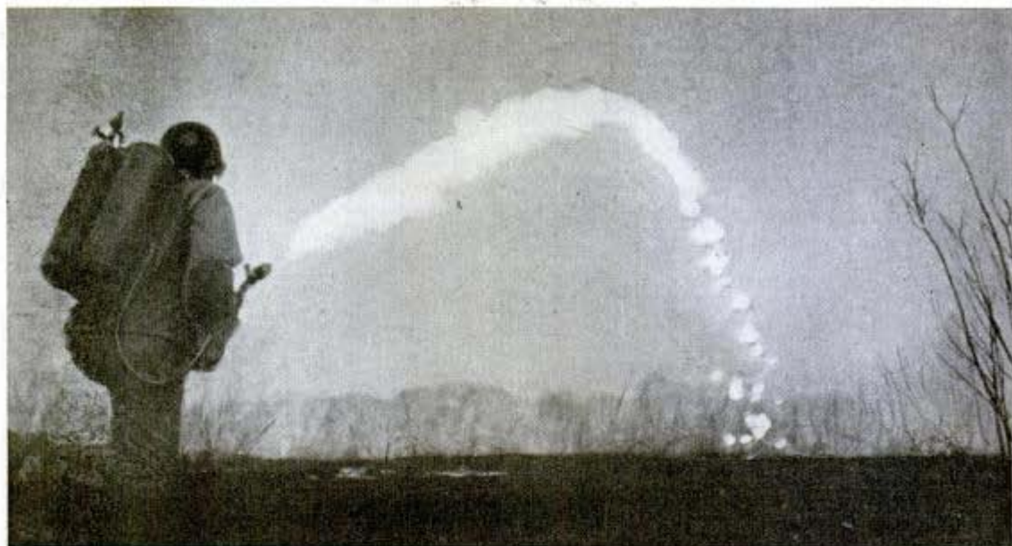
Jellied gasoline arches toward target, striking as a mass of flaming goo. In combat the trajectory is flatter
