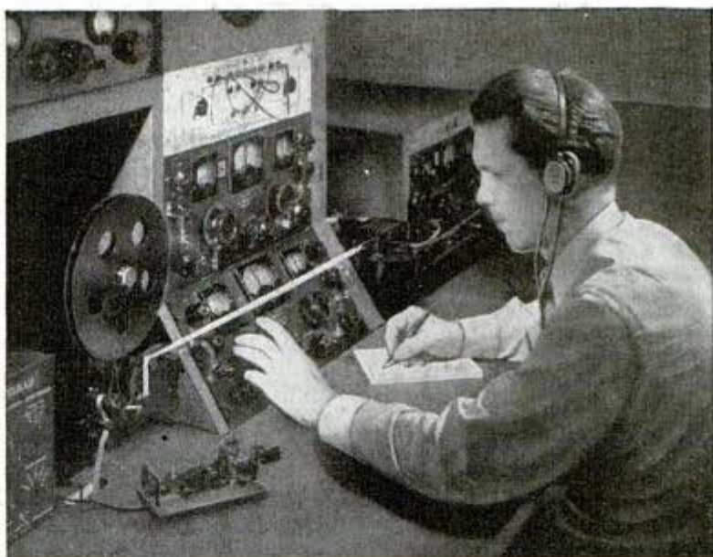
High speed recorder takes code signals at rate of 500 words per minute
