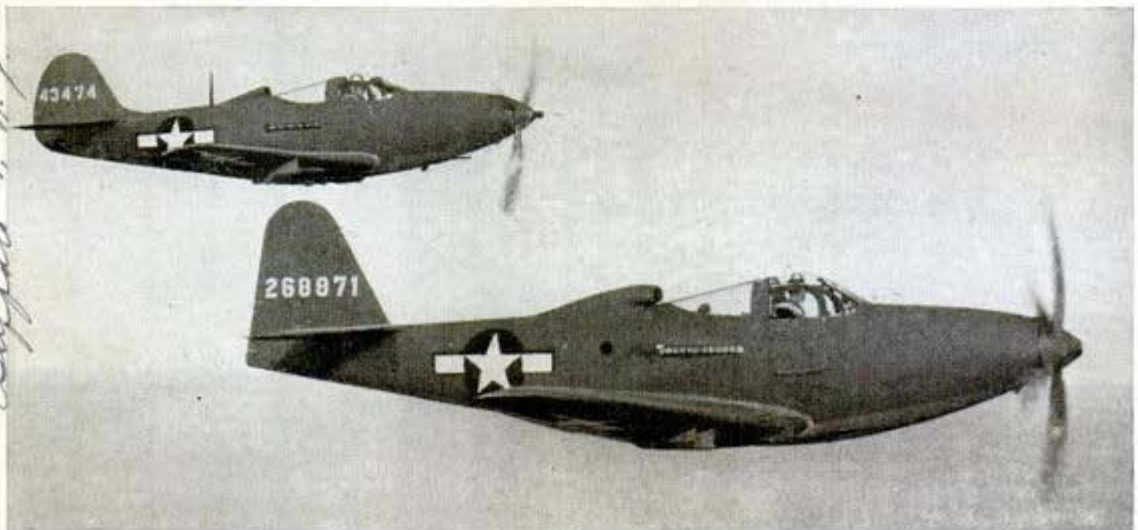
Profiles of Bell's two fighters—the P-63 Kingcobra (foreground) and the P-39 Airacobra—are compared in flight
