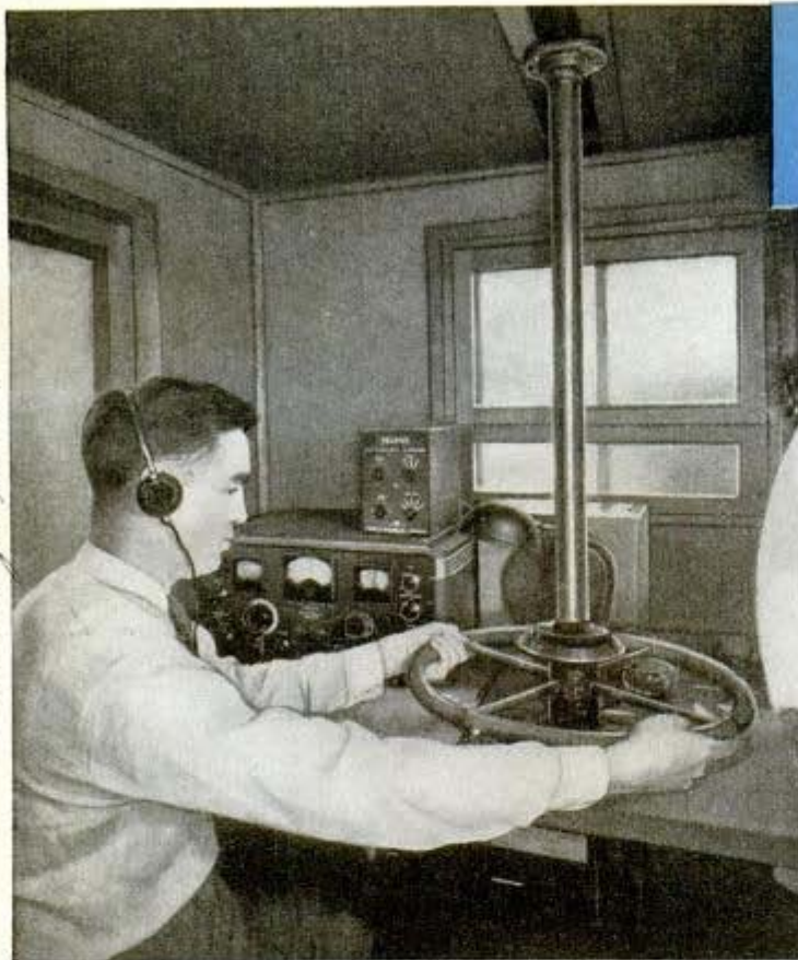
Hunting clandestine radio transmitter, operator rotates direction finder; calibrated scale indicates bearings of hunted signal. Above at right, huge direction finder has H-shaped antenna to locate signal within one or two degrees. Below, monitoring officer exchanges data over microphone with operator at direction finder
