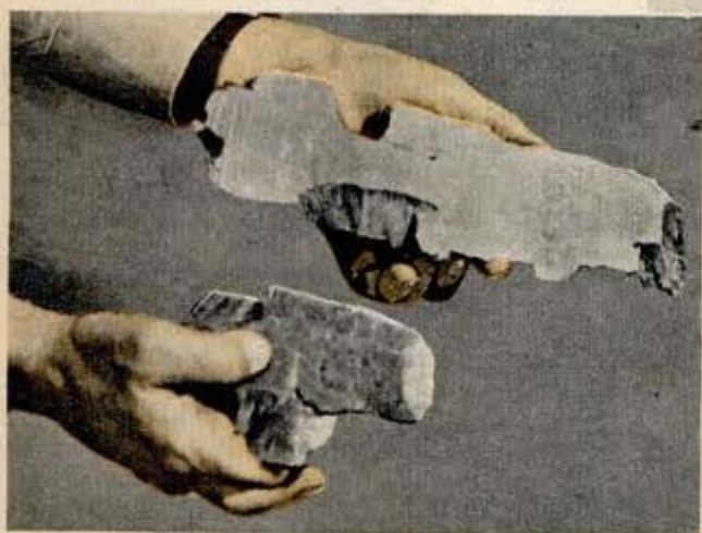
One-ton demolition bomb is shown (above) an instant after its release from two-engined plane. Below, parts of the same bomb after explosion—two jagged fragments of metal. These flying fragments cause only secondary damage; the effect depends on enormous blast
