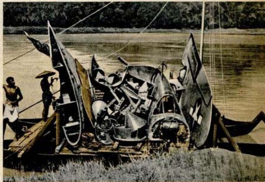
What looks like a mass of junk, above, is the disassembled P-40 on a barge, ready for day and a half trip to railroad. Below, aircraft repairman at a Middle East air depot installs propeller on a P-47
