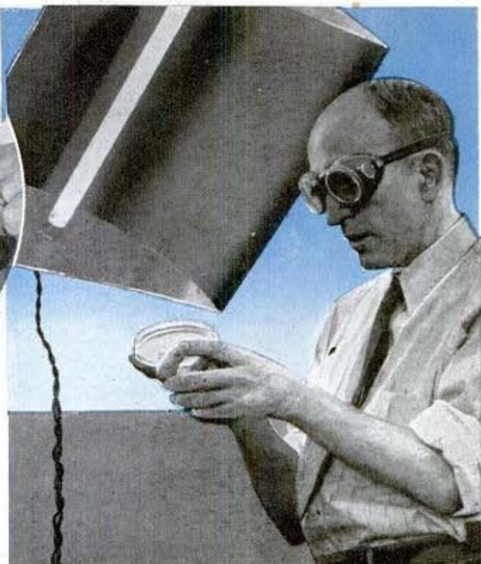
A colony of germs growing in petrie dish at General Electric company laboratory is killed by 15 seconds exposure to ultraviolet lamp. Below, filling penicillin vials
