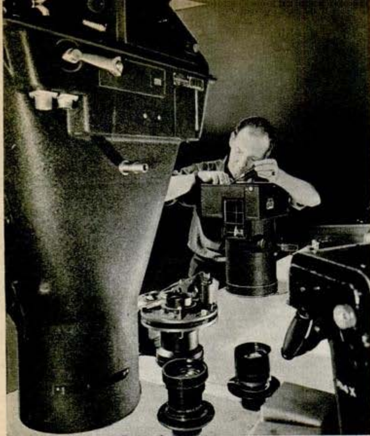
Above, giant aerial camera is checked carefully by skilled repairman in Navy's photo science laboratory before being taken aloft. Below, this striking picture of heavy seas washing the decks of a cruiser was made by a civilian press photographer
