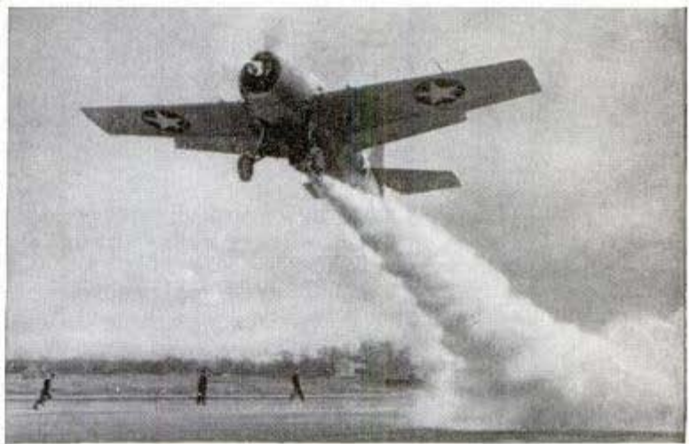
Army bomber (top) takes off from a short runway with rocket units under wings. Navy plane (right) has fuselage attachment
