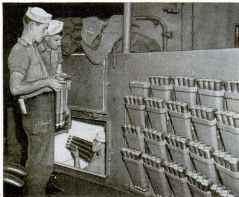
Racks on splinter shield of gun keep ammunition within reach
