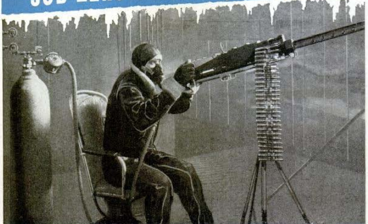
Lindberg Steel Treating Co. photo Above, testing machine gun and ammunition in stainless-steel- lined weather chamber at Wright Field. Below, officer at lookout post on ice-coated patrol boat U. S. Navy photo
