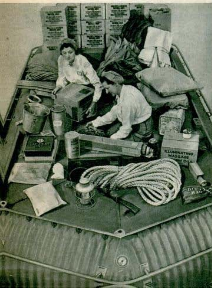
Above, a power nacelle in wind tunnel of aircraft plant in Los Angeles. Right, plywood glider wings in a western glider factory. Below, assembling the "ditty bag" of a ship's life raft, which includes blankets, awning, fishing gear, signal lamps and flares, first aid kit, oils and even magazines and games, besides the necessary food and water
