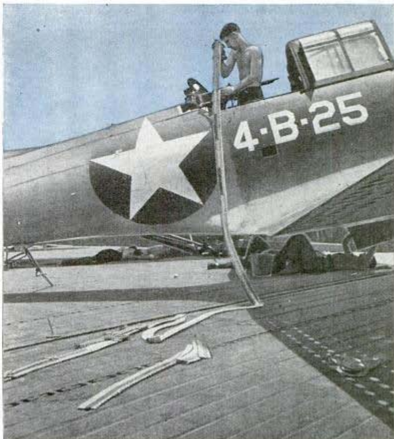
In "clay pigeon" test, student gunners practice with turret fixed with shotgun mount, learning to swing their bodies with the gun. Below, reloading twin .30-caliber guns on Navy Dauntless dive bomber on carrier
