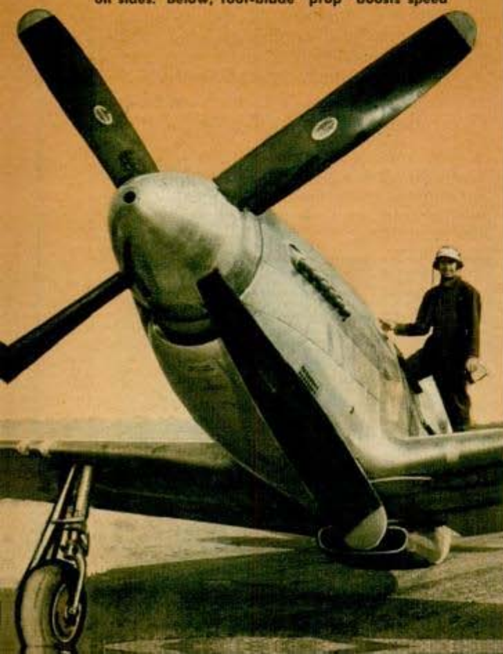
With "throat" bared, engine of new P-51 gets a final test. Note jet propulsion exhaust stacks on sides. Below, four-blade "prop" boosts speed
