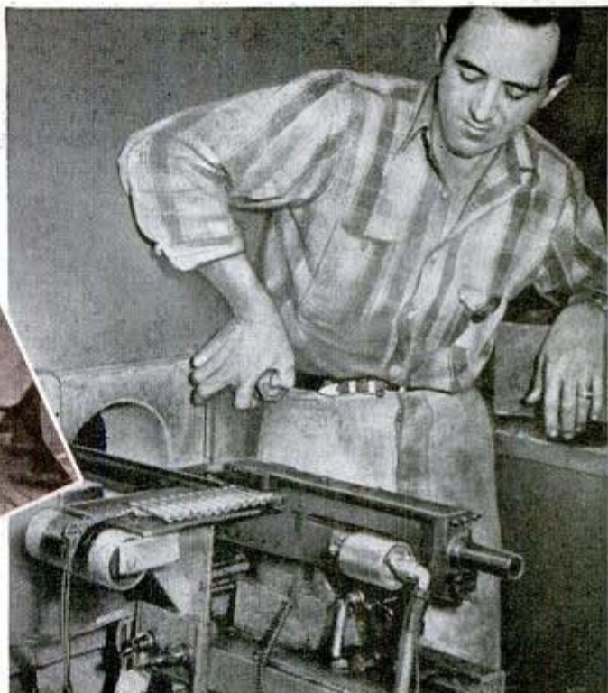
With his thumb on switch that cocks and fires weapon, an ordnance expert tests .30-caliber gun in an underground gallery
