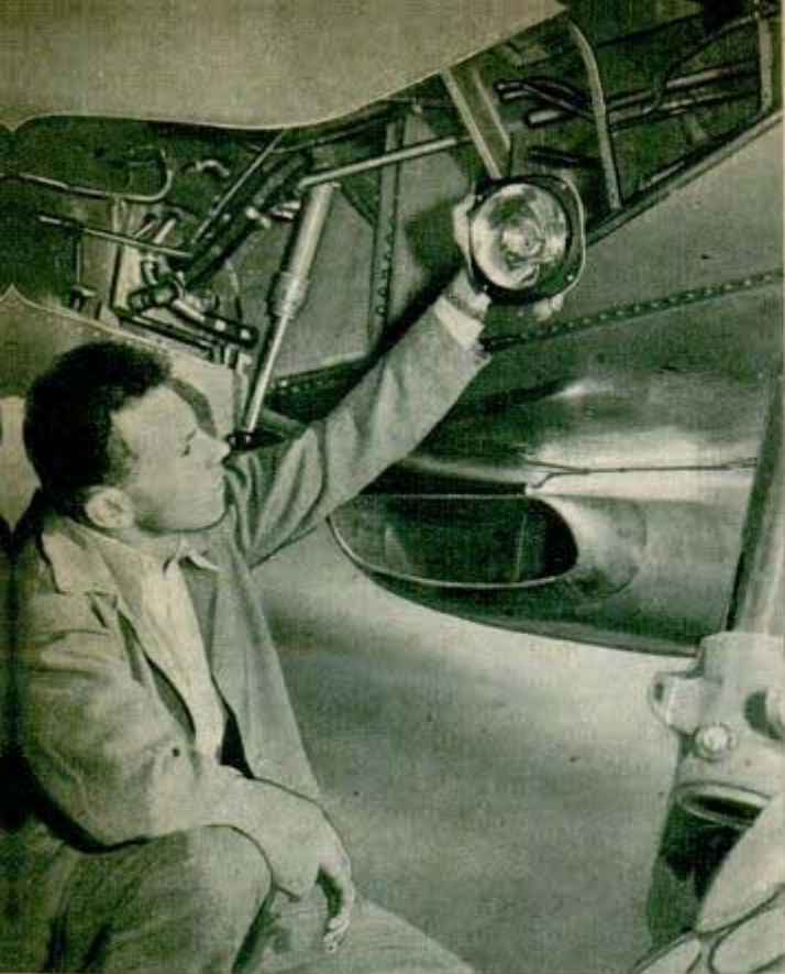
Sealed-beam type of landing light on P-51 retracts and folds into wheel well when wheels are retracted
