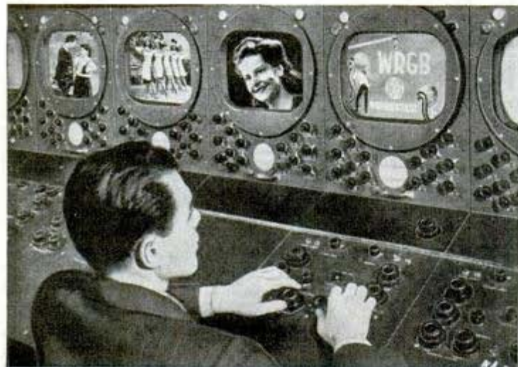
Quality of picture is controlled at "shading desk" in television studio
