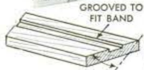
BLOCK TO CUT INLAY BANDS AT 45° ANGLE
