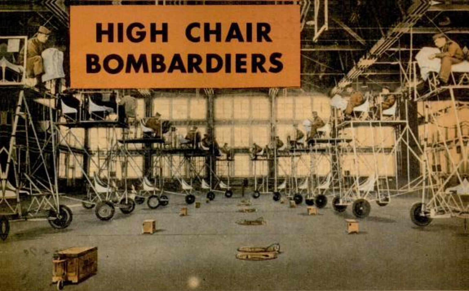
Bombardier cadets at Midland Army Air Field in Texas begin a bombing run on fixed targets. Below, a low seat in "highchair" trainer teaches bombing from low altitude
