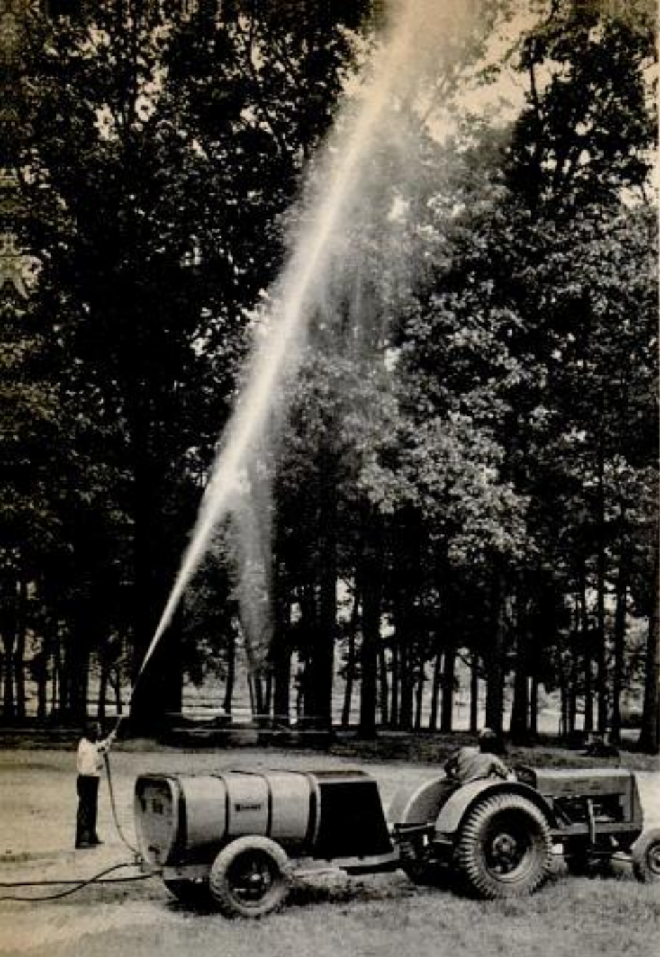
High-pressure jet protects shade trees in a Benton Harbor, Mich., park. Below, this spray rig forces vapor through nozzles at right, then propeller blows the spray into the trees
