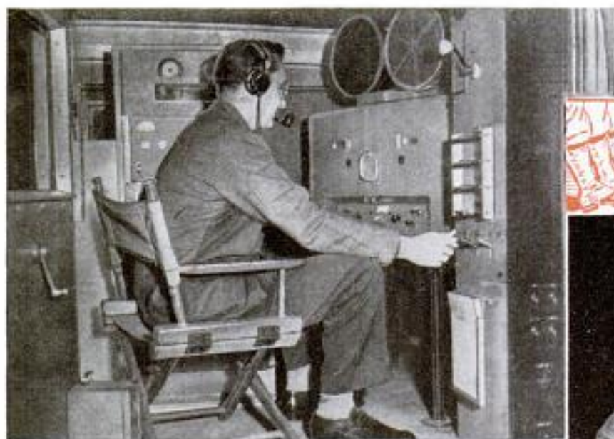
Turning the crank (above) slams the metal rod against a sounding board at right end of box. The result, to the movie audience, is the chatter of a machine gun. Below, the truck in which sound is recorded on film
