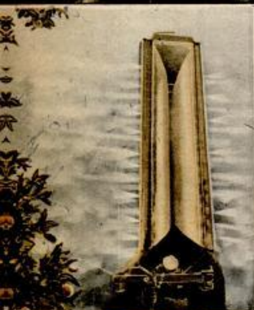
Top, spraying citrus grove with a multiple-nozzle boom. Left, dusting truck in action. Chemical dust is blown into trees through narrow openings at rear (see below) at 70-miles-an-hour initial speed
