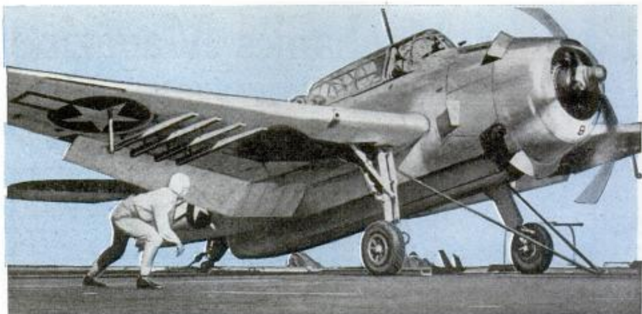
The carrier-borne Grumman Avenger above carries racks for four rockets under each wing
