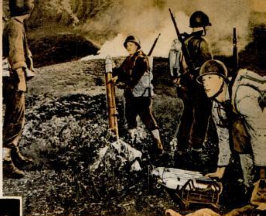
Above, chemical warfare service company starts a smoke screen with a 4.2 chemical mortar or "goon gun" which fires white phosphorus smoke and some high explosive
