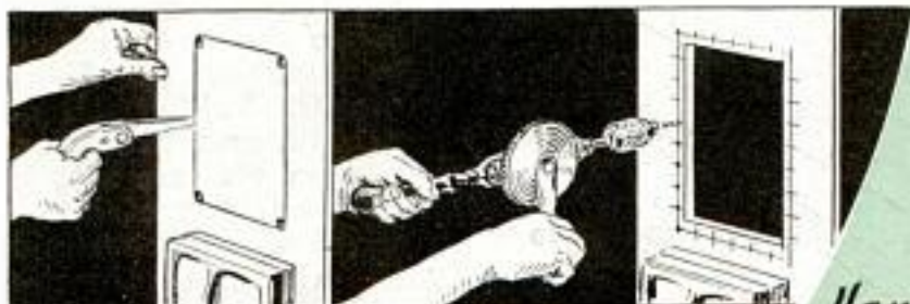
① SAW OUT THE OPENINGS ② DRILL HOLES FOR CORD
