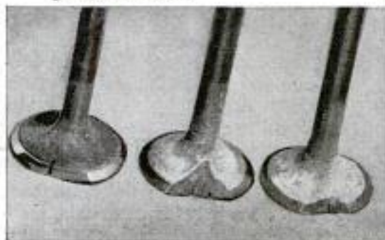
⑥ BURNED VALVES
