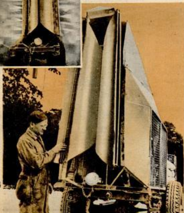
Top, spraying citrus grove with a multiple-nozzle boom. Left, dusting truck in action. Chemical dust is blown into trees through narrow openings at rear (see below) at 70-miles-an-hour initial speed
