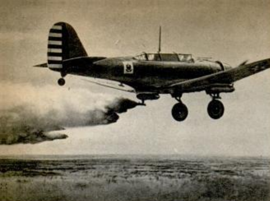
Above, how a plane releases sulphurtrioxide smoke from a belly tank. It can provide a 400-foot wall to screen paratroopers
