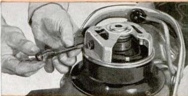
25 INSPECT BRUSHES AND FIT NEW ONES IF NEEDED
