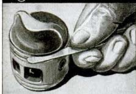
⑨ CHECK RING-GROOVE CLEARANCE
