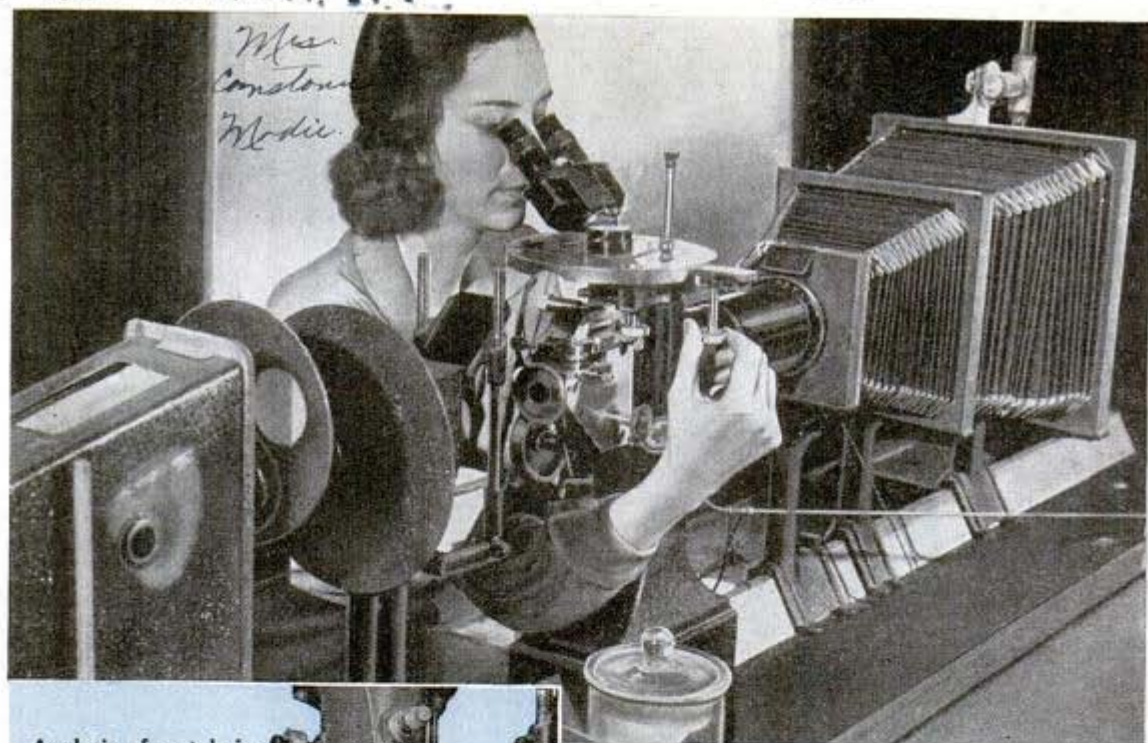
Analysis of metals is an important phase of research; above, G. E. worker studies specimen in eyepiece of camera-microscope. Below, studying molecular structure with an electron diffraction camera
