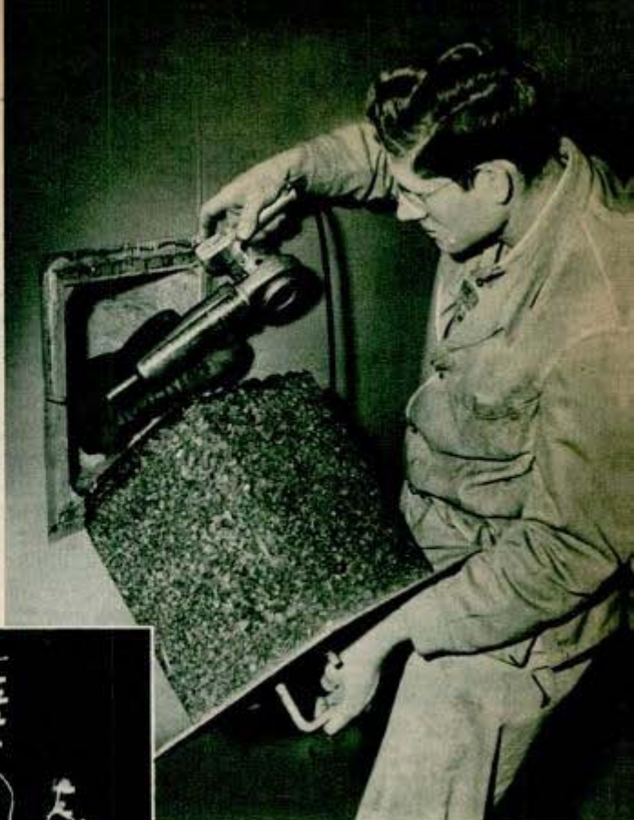
Above, passing hot air gun through hatch in two-foot thick wall of cold room; inside temperature may be as low as 130 degrees below zero. At left, test board with 144 contacts for quick check of bomber's wiring circuits. On panel below are gauges for testing strains at 78 different points of airplane structure
