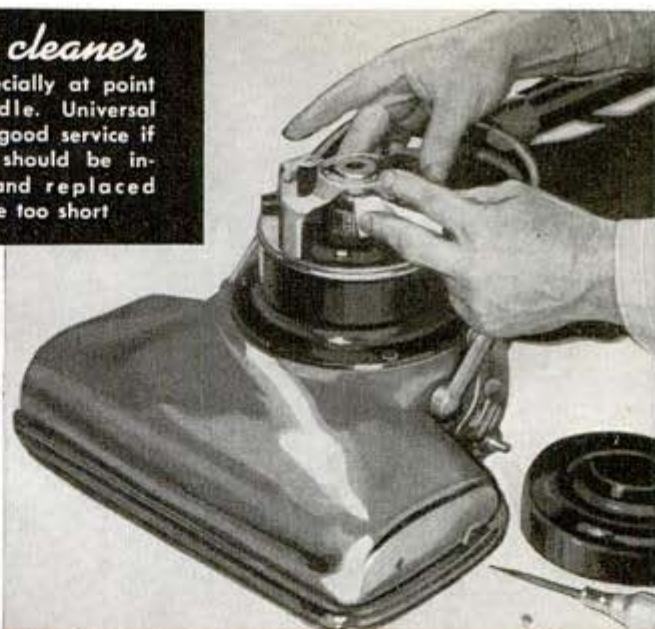
24 CLEAN COMMUTATOR WITH FINE (8-0) SANDPAPER
