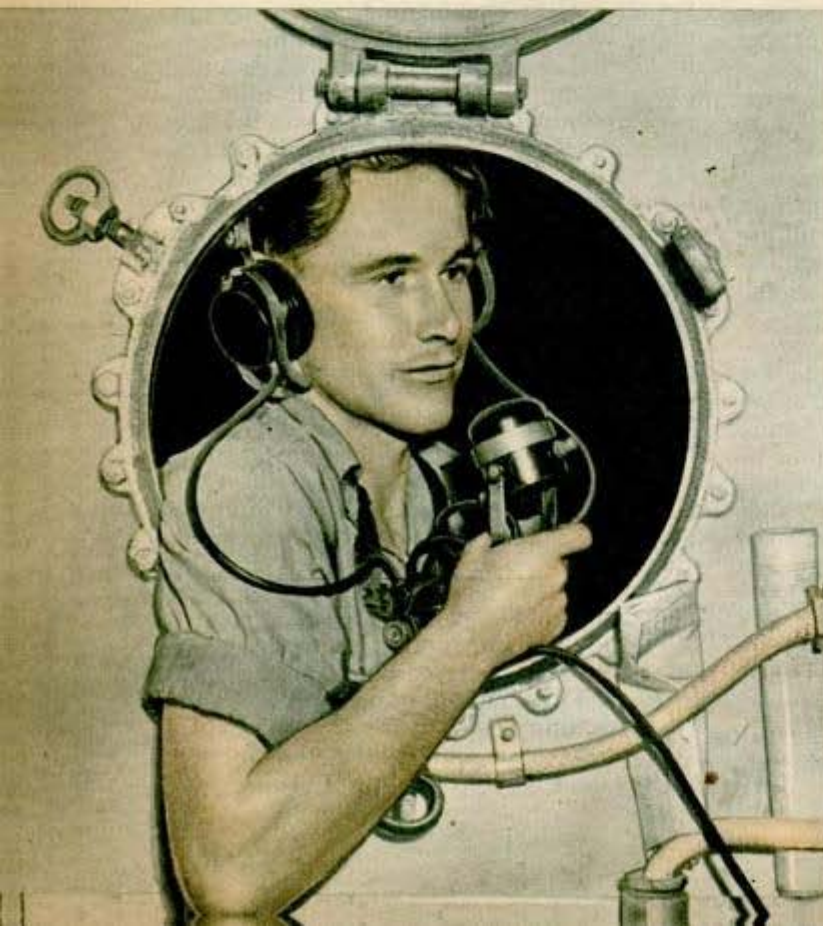
Sailor closing overhead valve in a warship's engine room. Below, port between engine rooms is closed during battle to make compartments watertight, and orders are given by phone
