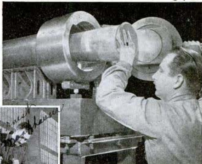
Above, shell is put in catapult gun to test breech. Left, officer watches as workman tries an inspection gauge on line of catapult guns in a plant
