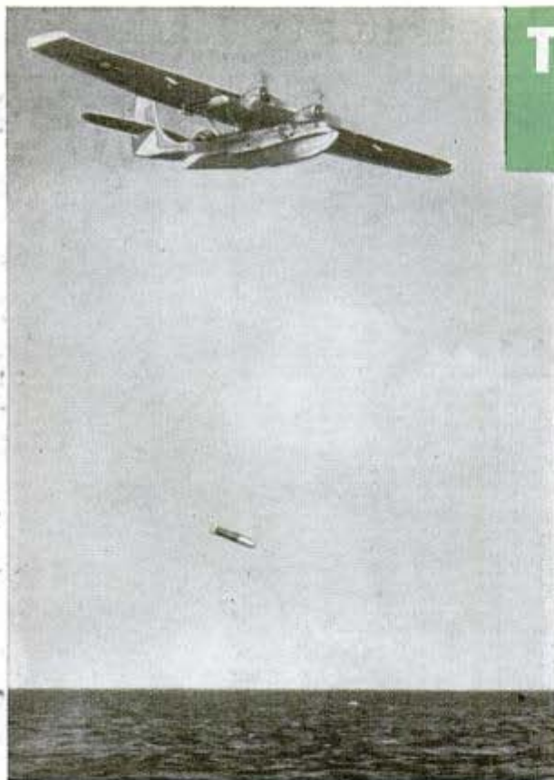
Flying boat drops aerial torpedo on Navy testing range; notice second "tin fish" under wing. Navy jeep (right) is used to tow torpedoes from repair shop. Below, dismantling "fish" after test
