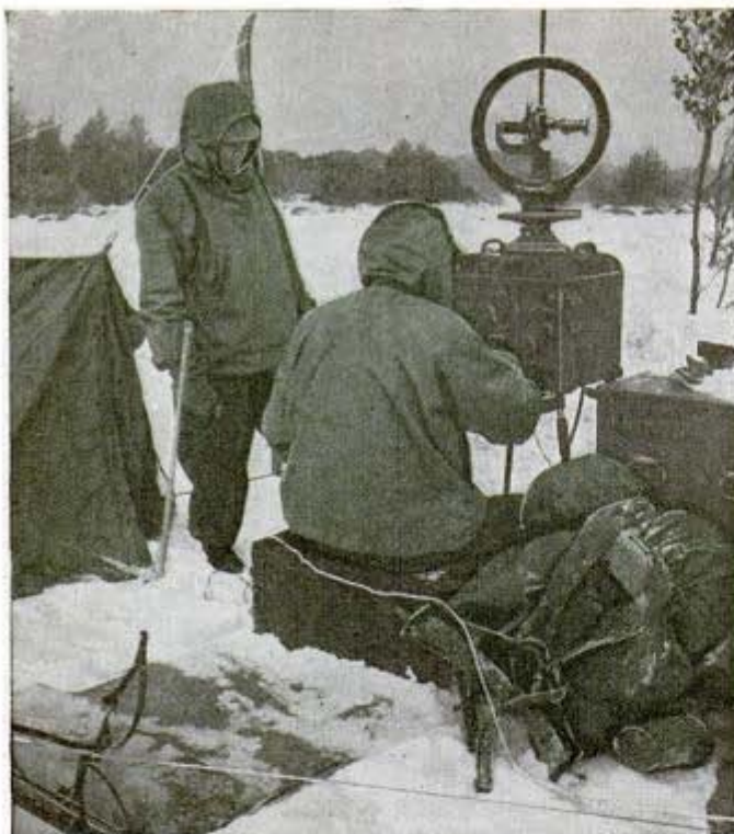
Radio direction finder locates enemy transmitters for bombing
