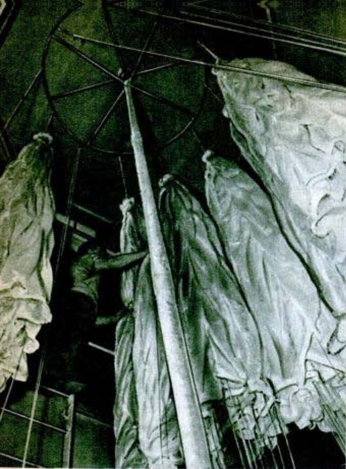
Navy parachutes hung in air-conditioned room to keep grit and moisture from damaging the fabric Official U. S. Navy photo
