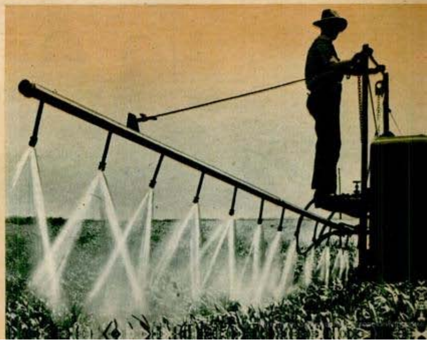
Erecting emergency crest on levee to hold back flood waters. Below, chemical weeding rig sprays poison that kills broad-leaf weeds and drains harmlessly off narrow leaves of grain
