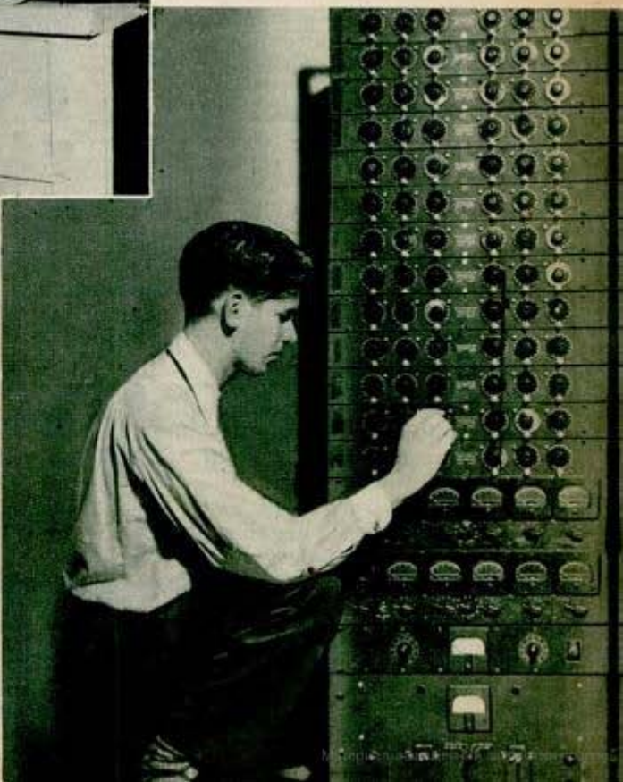
Above, passing hot air gun through hatch in two-foot thick wall of cold room; inside temperature may be as low as 130 degrees below zero. At left, test board with 144 contacts for quick check of bomber's wiring circuits. On panel below are gauges for testing strains at 78 different points of airplane structure
