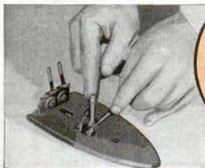
22 LAMP SHOULD LIGHT WHEN TEST LEADS ARE TOUCHED TO SWITCH TERMINALS
