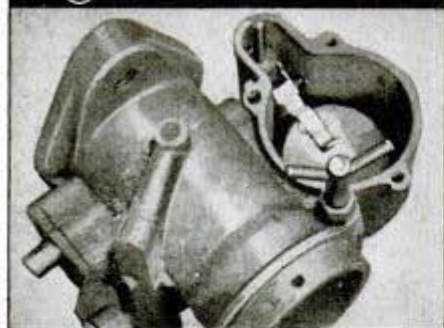
⑦ RESOLDER LOOSE METAL FLOAT
