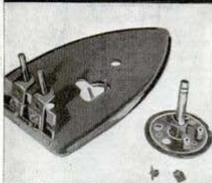
23 DEFECTIVE SWITCH CAN BE DISCARDED. ELEMENT WILL WORK WHEN WIRES ARE SPICED
