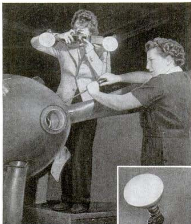
Special hand bracket (top and right) holding photofloods and 35-millimeter camera, was designed by Bell Aircraft for use on visual training picture assignments. Below, North American Aviation uses X-ray to activate fluorescent coating on metal template in this housing. Metal glows except where lines are scribed
