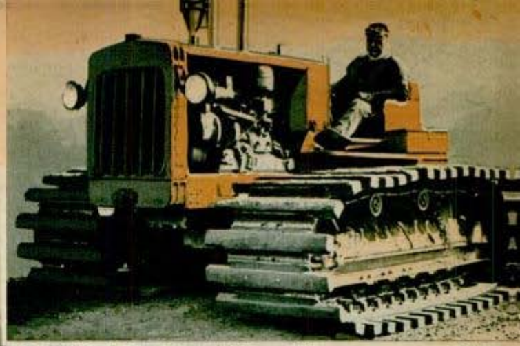
Swamp-type tracks with wide wood paddles attached support tractor on the loose soil
