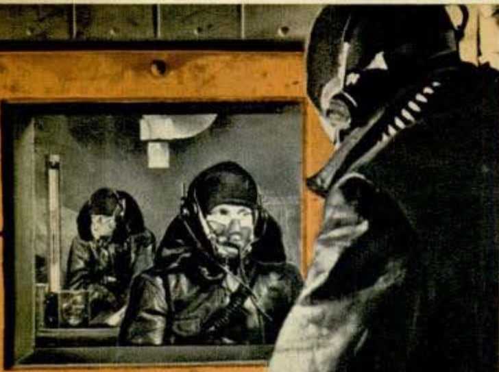
Refrigerating machinery and pumps dwarf "strato" tank in Sperry laboratory. Below, observer in sealed lock can open door quickly if anything goes wrong "upstairs." Below at right, naval officer questioning test crew inside tank
