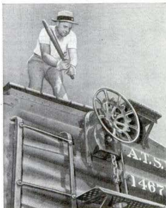
And here a Santa Fe switchman shows the wrong way to release brake, knocking it loose without holding on
