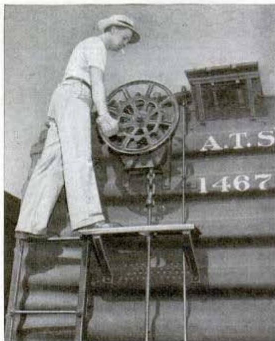
Santa Fe switchman shows safe way to release hand brake, feet braced and one hand gripping car ladder
