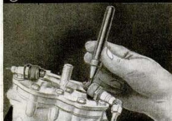
9 GRAPHITE ON PLUG THREADS
