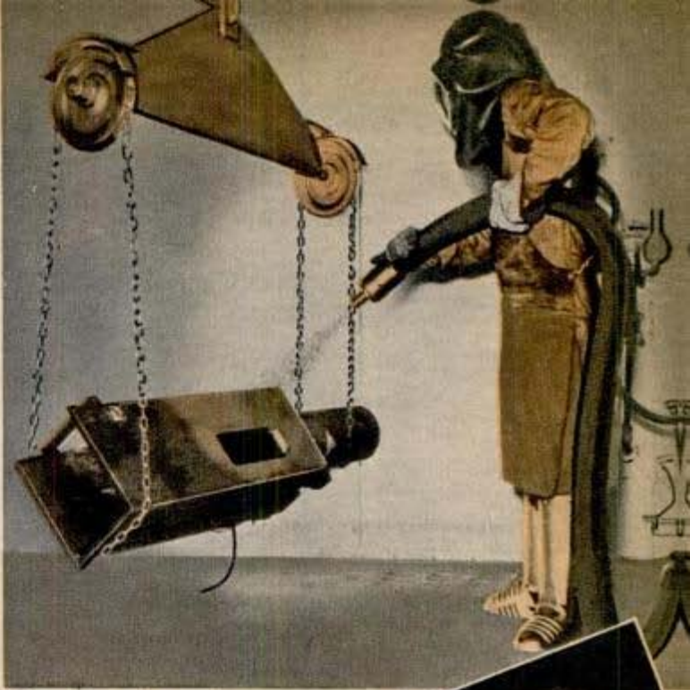
"Shot blaster" cleanses welding scale from breech casing for Bofors cannon
