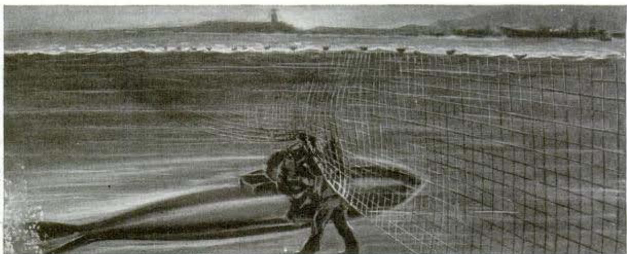
Above, rear man dismounts to lift net protecting harbor and let torpedo pass beneath. Photo shows how the "cowboys" act as their own periscope
