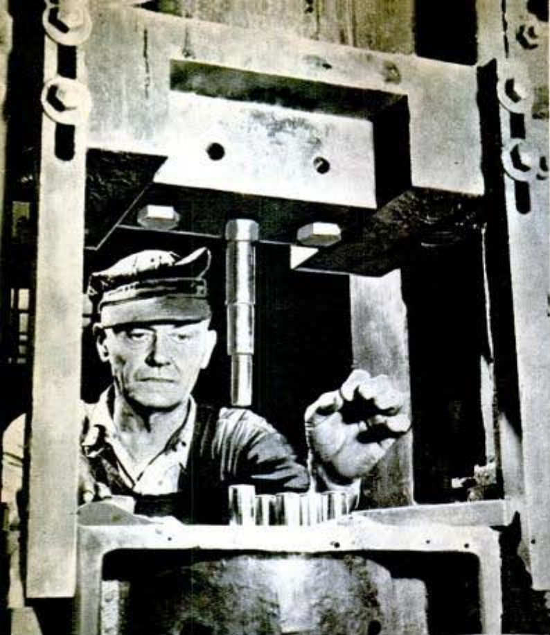
Above, filling steel dies with powdered metal "mix" in the first briquetting operation. Below, lifting oil-impregnated powdered-metal bearings out of bath to drain excess oil back into the tank
