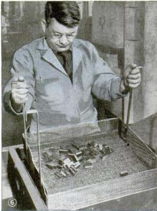
6—WIRE BASKET USED TO LOWER PARTS IN QUENCHING BATH. 7—QUENCHING BATH AND CARBURIZED PARTS DUMPED INTO CHUTE
