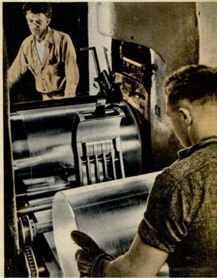
Eastman Kodak photo Rolls of 35 mm. motion picture film are stacked and ready for shipment to army units. Below, rolling a wide sheet of sterling silver at Handy & Harman plant, world's largest. Industrial use of silver has doubled twice in four years
