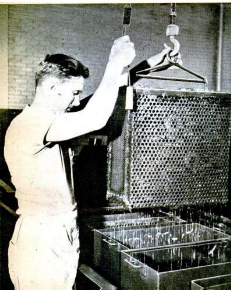
Above, filling steel dies with powdered metal "mix" in the first briquetting operation. Below, lifting oil-impregnated powdered-metal bearings out of bath to drain excess oil back into the tank
