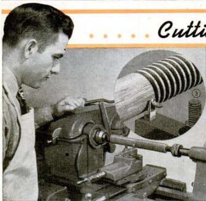
② TANGENT CUTTER CUTS COMPLETE THREAD IN ONE PASS
