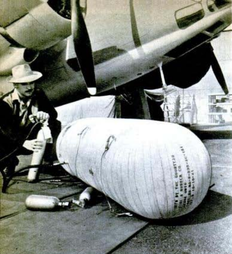
Weight engineers must determine a landplane's "water line" and length of time it will stay afloat, and specify location and size of flotation bags carried for emergency. Below, P-38's four machine guns and 20 mm. cannon present a problem of weight concentrated in nose
