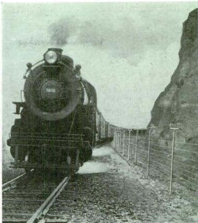
Electric fence flashes warning if rocks fall on tracks of a mountain line
