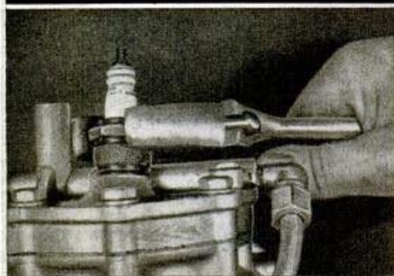
8 FORCING PLUGS STRIPS THREADS
