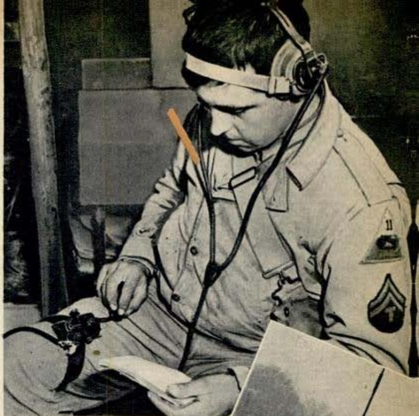
Radio operator in scout car is equipped with a transmission key clamped to his leg
