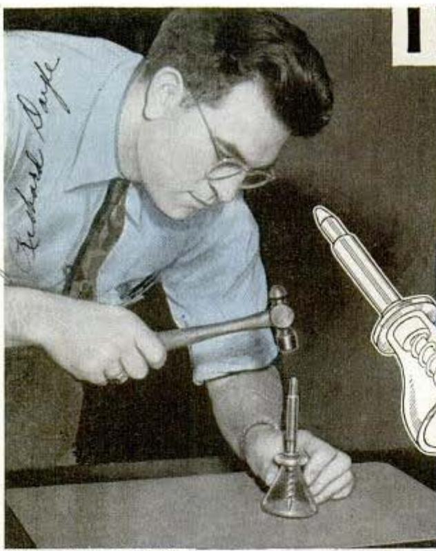
Courtesy Curtiss-Wright Corp. The "G. I. Joe's" of industry are showing ingenuity in discovering ways to increase the flow of war goods. Here are some innovations by workers: above, plastic bell cap center punch which locates the exact center of hole. Right, a polisher for interior of cylinders
