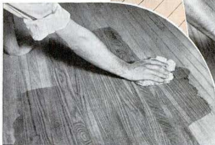
4 APPLY FILLER FIRST WITH, THEN ACROSS GRAIN
