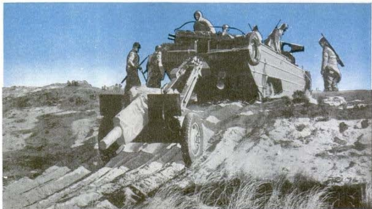
The amphibious cargo carrier for landing operations, this "Duck" is hauling a 105-mm. howitzer up the beach
