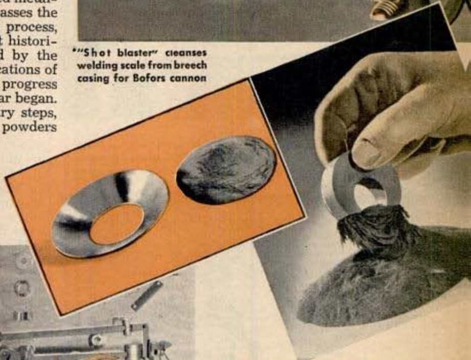
Left, above, a pile of metal powder and bronze part it becomes in seconds. Right, magnet illustrates properties of iron powder made of scrap iron
