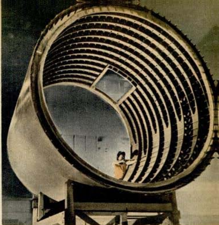
This 15-foot section of "barrel" fuselage of Constellation (above) weighs only 50 pounds more than the workman
