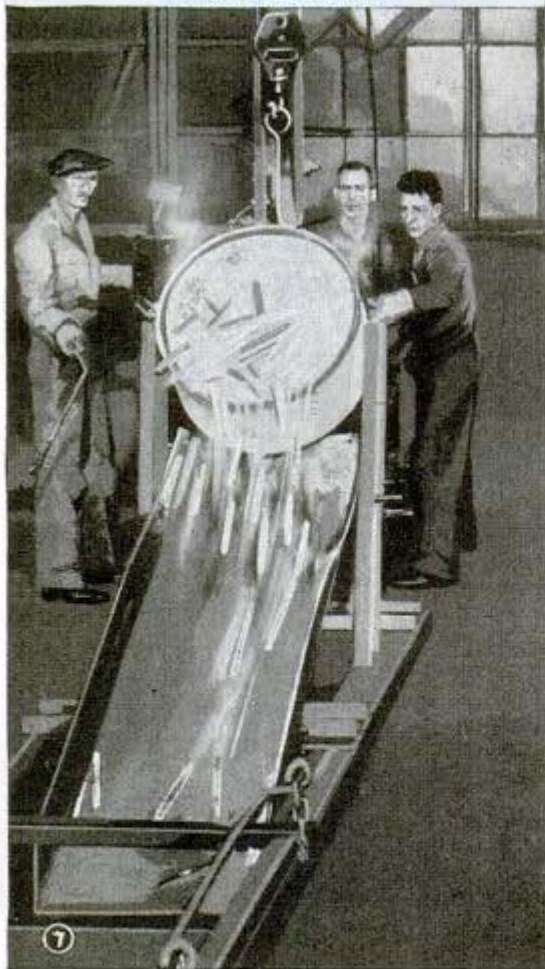
6—WIRE BASKET USED TO LOWER PARTS IN QUENCHING BATH. 7—QUENCHING BATH AND CARBURIZED PARTS DUMPED INTO CHUTE
