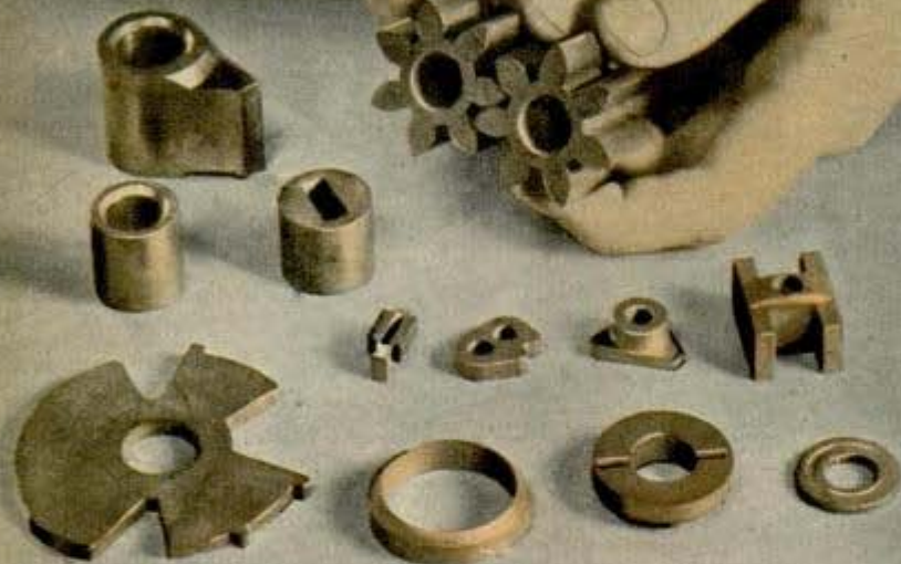
Left, some of the parts made from powdered metal. Below, hydraulic press for powdered metal, one of largest ever built
