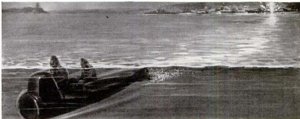
Approaching the target unseen, the men detach the warhead of the torpedo, fix it on victim's hull and set time fuse. In the interval before explosion (below) they have time to ride aft portion of torpedo to safety
