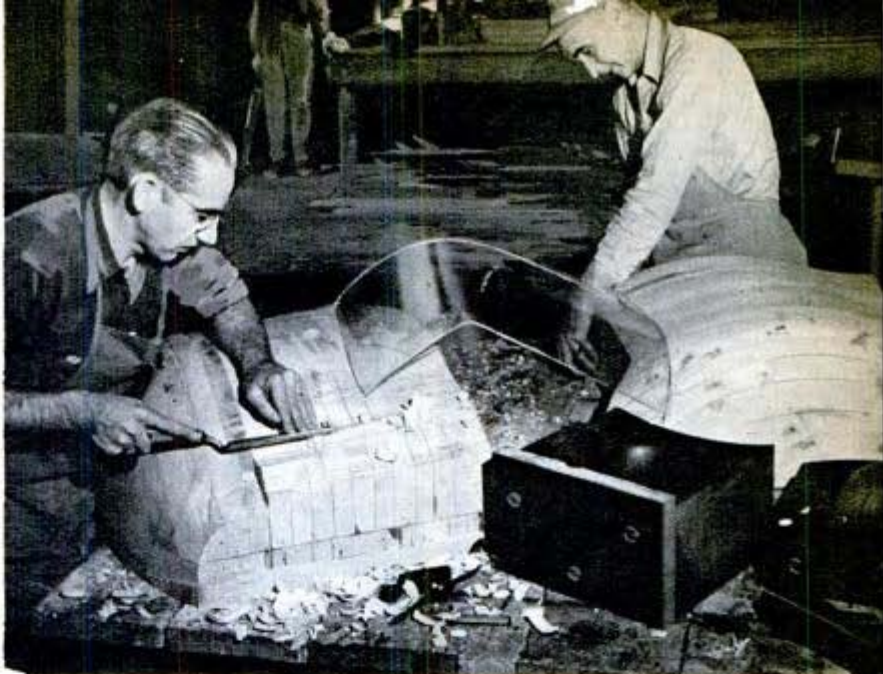
Plexiglas sections for turrets are formed by being heat-bent over chiseled-out wooden forms above. Form at left will cover nose turret
