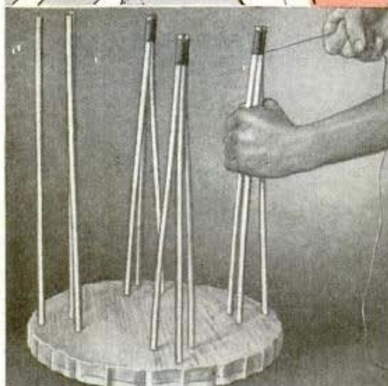
⑦ Wrapping ends of legs
