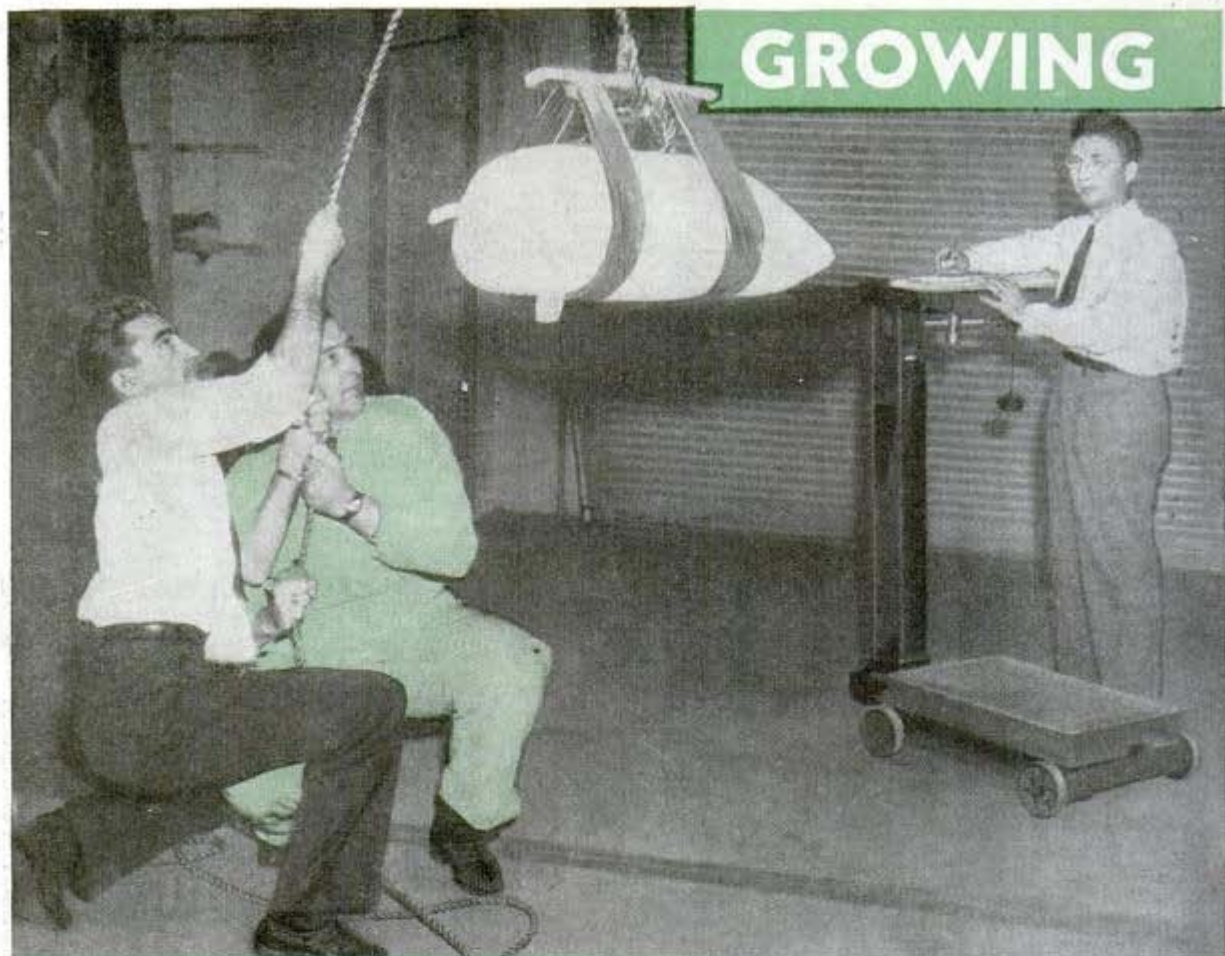
A rough dropping test for cotton bags measures their ability to stand shipping
