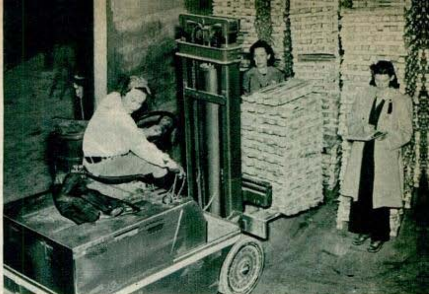
Finished bars of refined magnesium as they look when ready for shipment. The Nevada plant produces more than 50,000 tons a year
