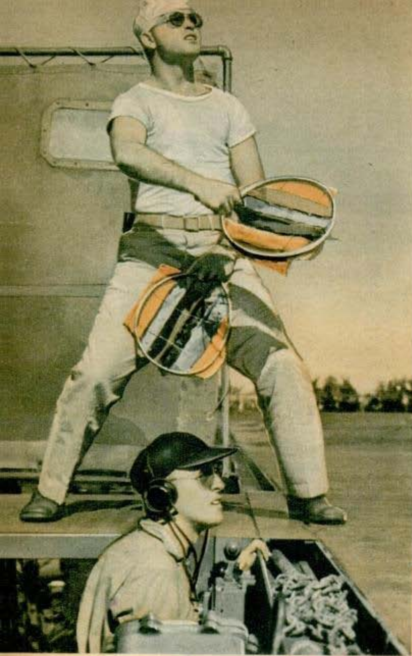
"Cut throttle and proceed to normal landing," officer signals to incoming pilot. The "talker" (foreground) relays orders. Below, scout plane drops message to alert deck crew
