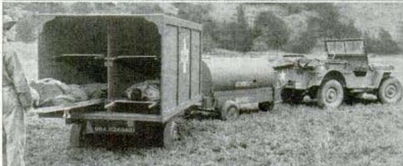
Light enough to be lifted by hand and transported by plane, plywood tanks are used to fly gasoline to advanced air bases. At left, jeep hauls tank and ambulance "train"
