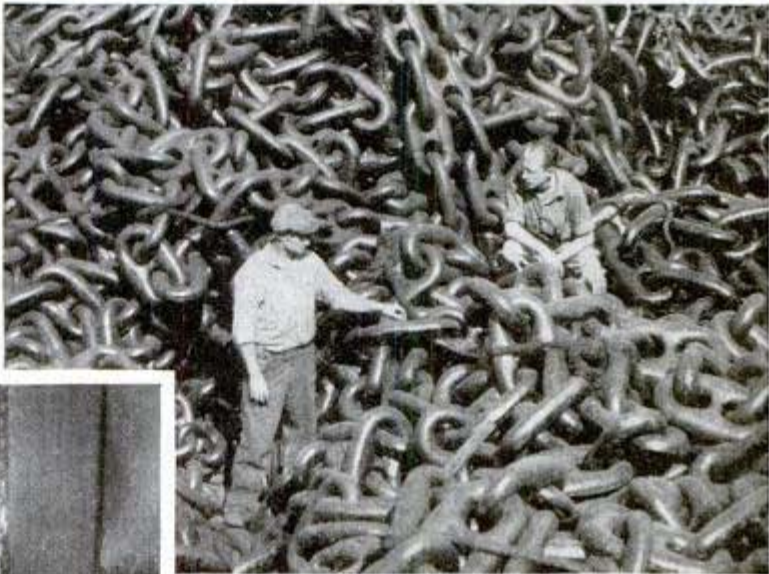
Strength of anchor chain in testing pit is gauged by a machine that exerts a 2,000,000-pound load, below
