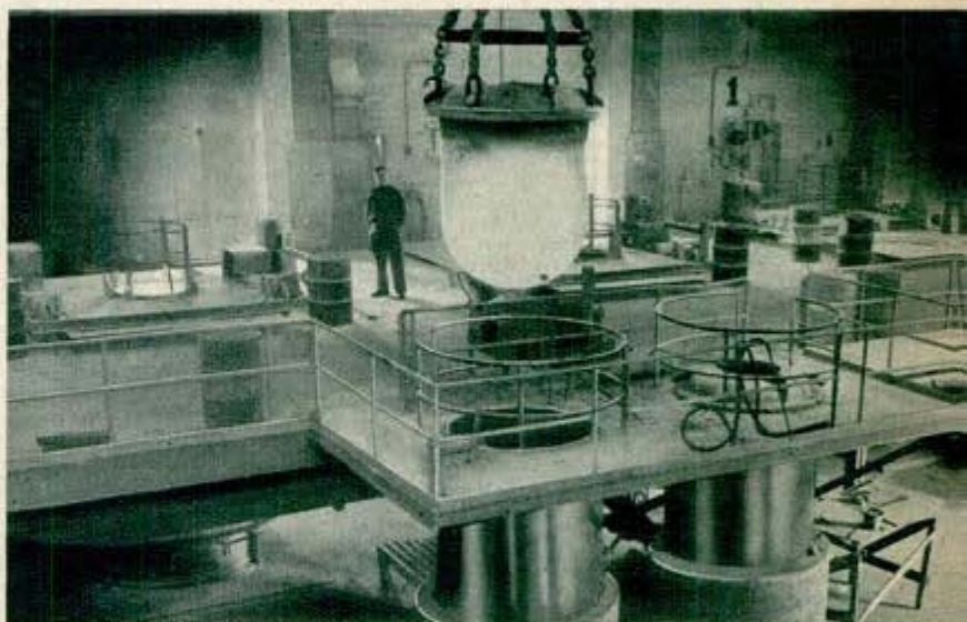
Lowering crucible of molten magnesium metal into cooling chamber. At Basic Magnesium, Inc., magnesite is changed into an oxide and then to a chlorine, which is broken down into metallic magnesium and chlorine gas. Below, water storage tanks under construction
