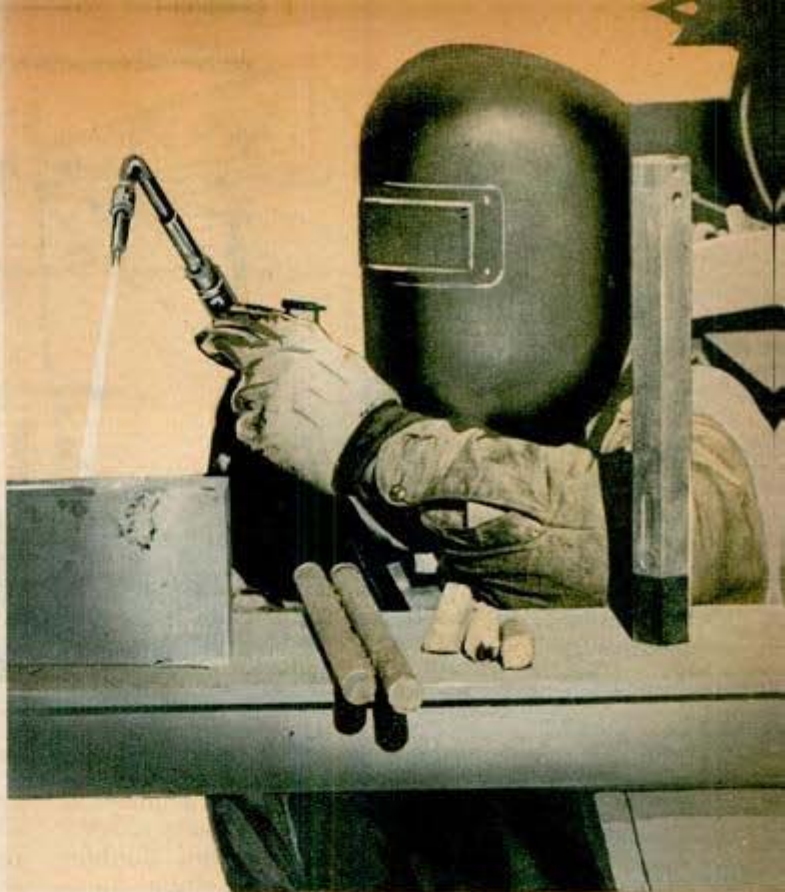
Welder cuts through solid magnesium to show that it resists combustion, except under special circumstances. Storage tanks (below) are at the Basic Magnesium, Inc., plant
