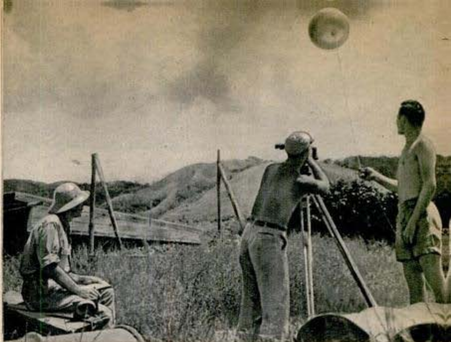
Sighting on balloon with theodolite to obtain wind direction and speed
