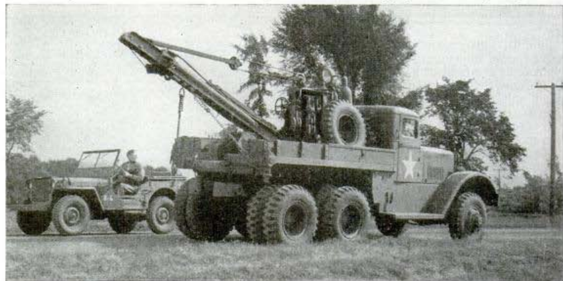
This giant wrecker can hoist 10 tons or eight vehicles like the tiny jeep it dwarfs in passing
