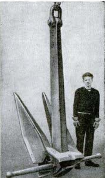
Anchor and reel ride stern of barge; closeup shows "flukes" that dig in
