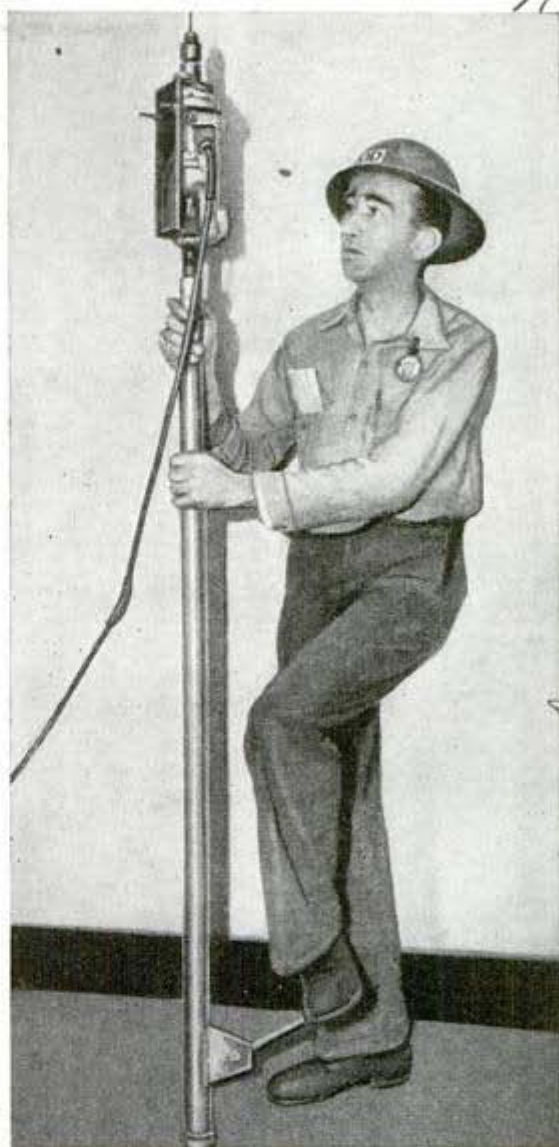
Shipyard worker steps on foot pedal which operates drill mounted on adjustable rod for overhead work
