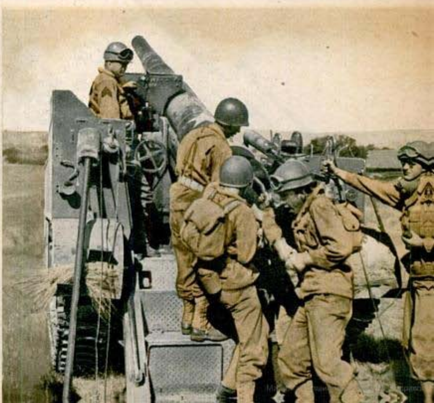
A far cry from horse-drawn guns of World War I is this self-propelled 155 mm. giant, the M-12, mounted on chassis of medium tank. Hinged supports at rear dig into ground. Below, loading the M-12
