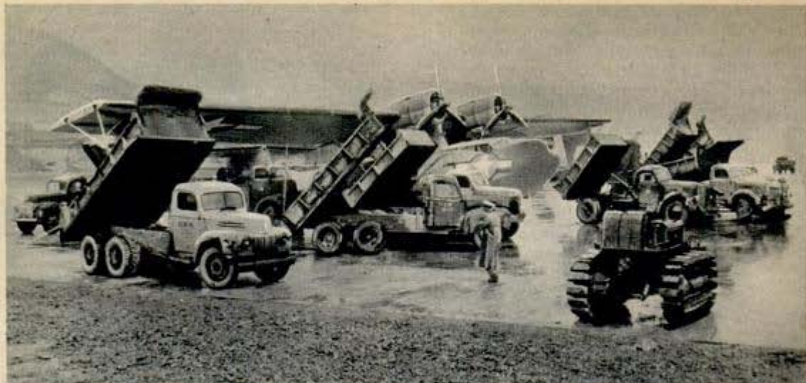
An Arctic squall in Alaska gave Navy trucks a new job—acting as anchors and windbreakers for a Catalina
