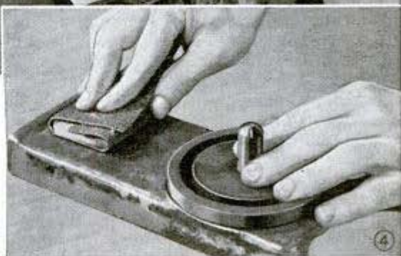
Above, using a backing block of felt or cork to build a level surface when sanding. Below, masking tape or compound will protect polished parts
