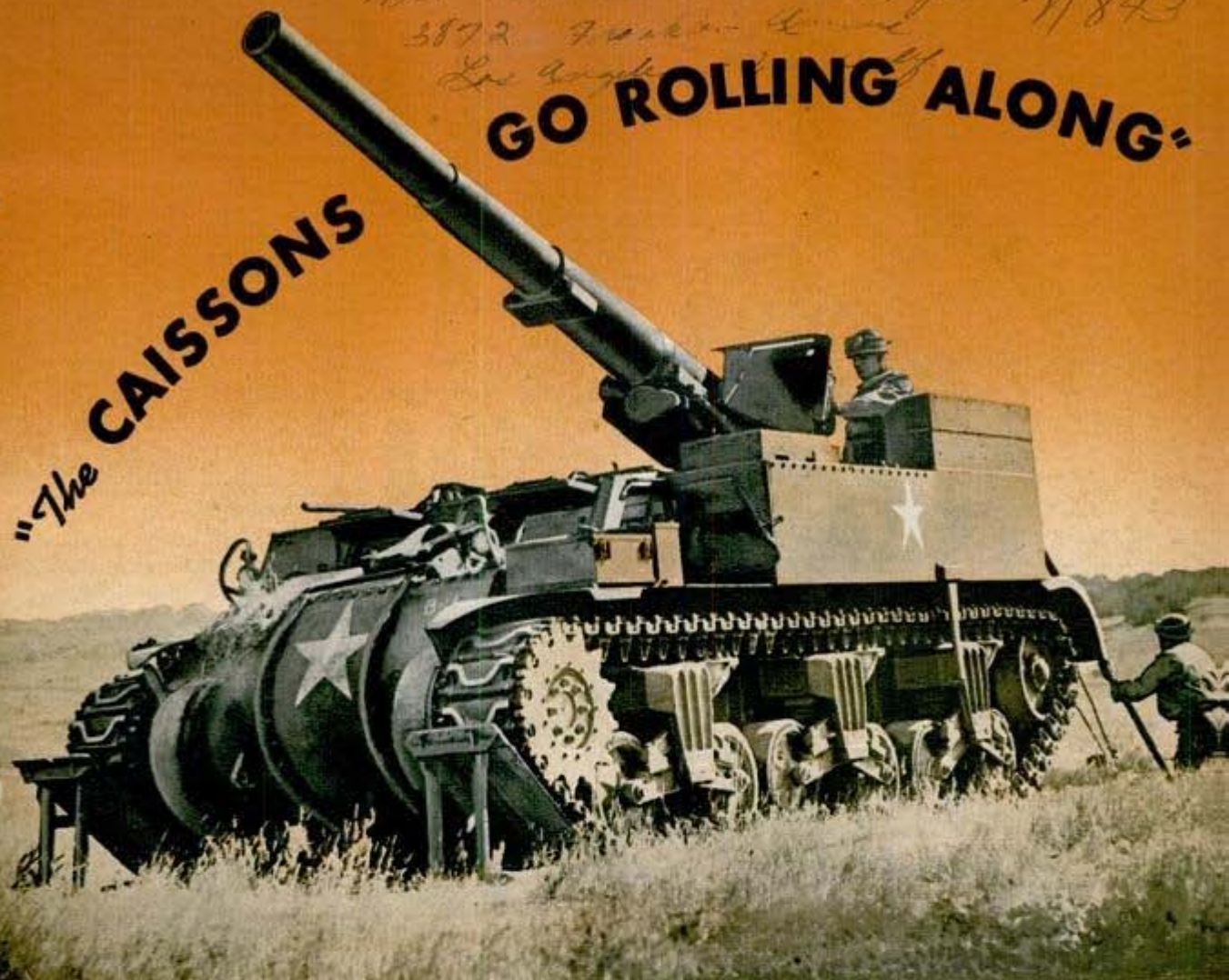
A far cry from horse-drawn guns of World War I is this self-propelled 155 mm. giant, the M-12, mounted on chassis of medium tank. Hinged supports at rear dig into ground. Below, loading the M-12
