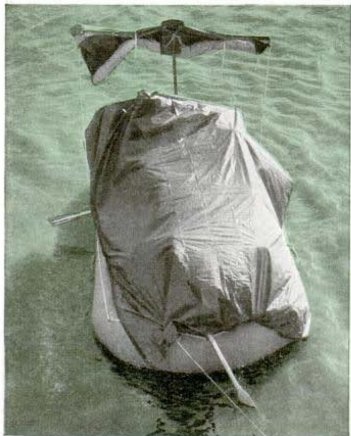
Concealed by camouflage resembling a tree stump, one Marine keeps watch while partner reports to command post by field telephone. Below, seven-man raft for Flying Fortresses, made by U. S. Rubber Co., has a sail and tarpaulin for sun protection
