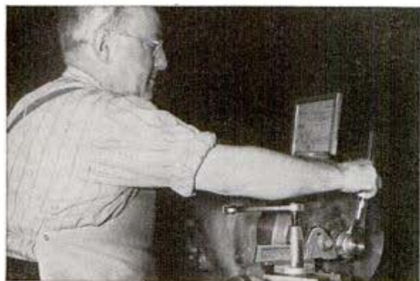
With Williams' Spring Cutting-Off Tool Holder, feed can be applied automatically leaving operator free to watch and thoroughly lubricate the work.
