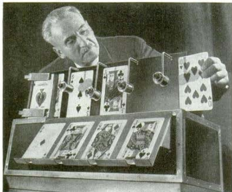
A Westinghouse research scientist demonstrates his electronic dealer—four electric eye circuits can sort cards into suits or deal poker hands
