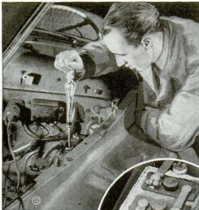
Condition of battery should be checked regularly with a hydrometer. Corroded battery at right indicates level of electrolyte is too high or charging rate is excessive, causing acid to overflow, thus reducing strength of electrolyte. Spring bolt below was worn and scored by lack of proper lubrication at regular intervals
