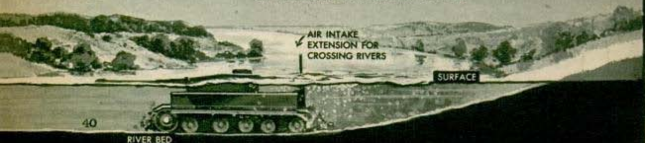
THE GERMAN "TIGER" TANK IS CAPABLE OF BEING MADE WATERTIGHT AND CROSSING RIVERS, ON THE RIVER BED, TO A DEPTH UP TO 15 FEET
