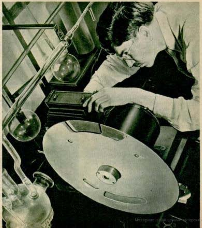
On platform suspended from crane, Hollywood cameramen record "The Inside of Arc Welding." Below, slit in edge of wheel allows 1/10,000 second for filming an electric arc Westinghouse photo
