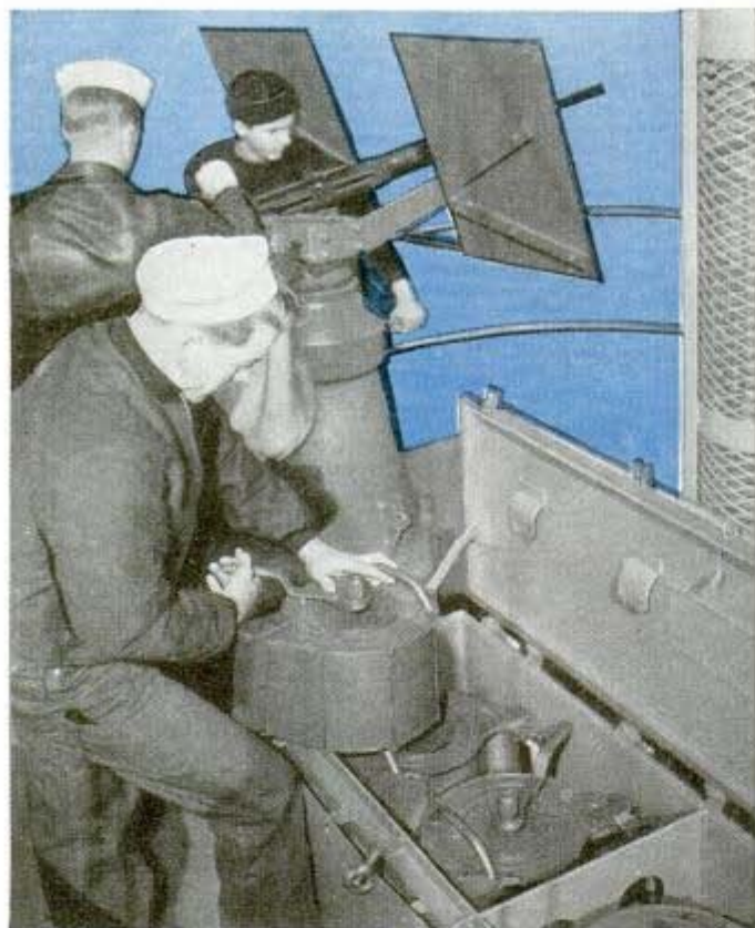
Winding up magazine of 20 mm. gun to force shells into breech
