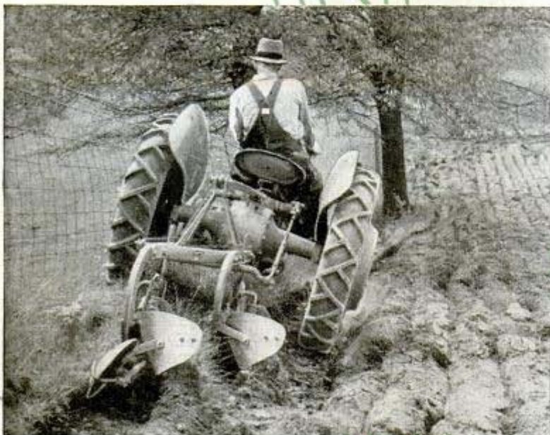
Courtesy Deere & Co. Sugar beet topper and lifter places the beets in one windrow and tops in another where they can be saved for stock feed. Below, Ford-Ferguson tractor has unit which enables farmer to turn furrow close to the fence
