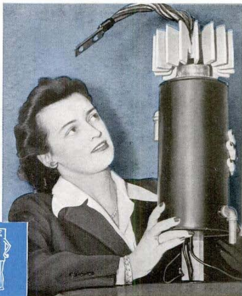
The bomblike Ignitron tube produces direct current for aluminum, magnesium and other industries. Left, positive voltage attracts electrons from filament to metal plate; by changing the voltage of a grid interposed like a Venetian blind between filament and plate, flow of electrons can be increased or diminished. Below, Westinghouse high-speed X-ray tube stopped all motion, seeing through foot and ball in millionth of a second
