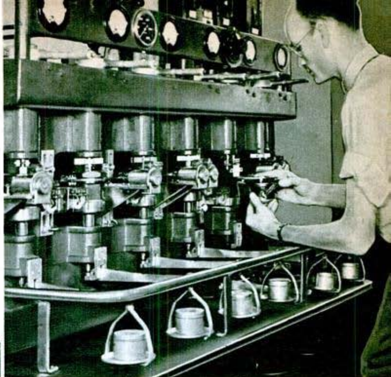
Test machines rub steel balls together to measure metallic wear under various pressures and lubricants
