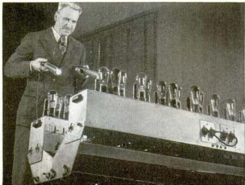
Instead of hand-driven hammers, light beams striking "electric eyes" evoke music from this marimba in Westinghouse Research Laboratories
