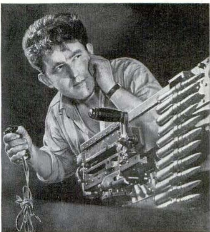
Above, "heavy artillery" on wings—a 75-millimeter gun in nose of a B-25 Mitchell. At right, machine guns and other weapons are test-fired to destruction in laboratory
