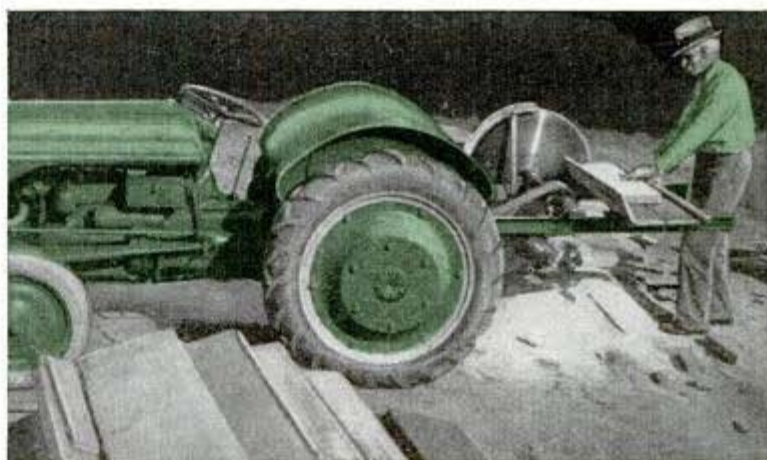
Portable saw mounted on back of Ford-Ferguson tractor enables farmers to take power to the wood instead of old way of taking wood to the saw
