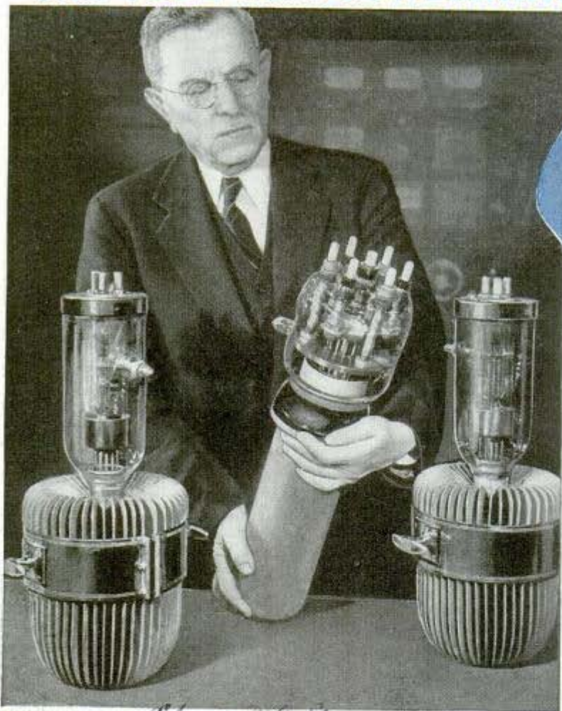
Left, tube used for electrolytic tinplating. Above, RCA radio "sewing machine" stitches thermoplastic
