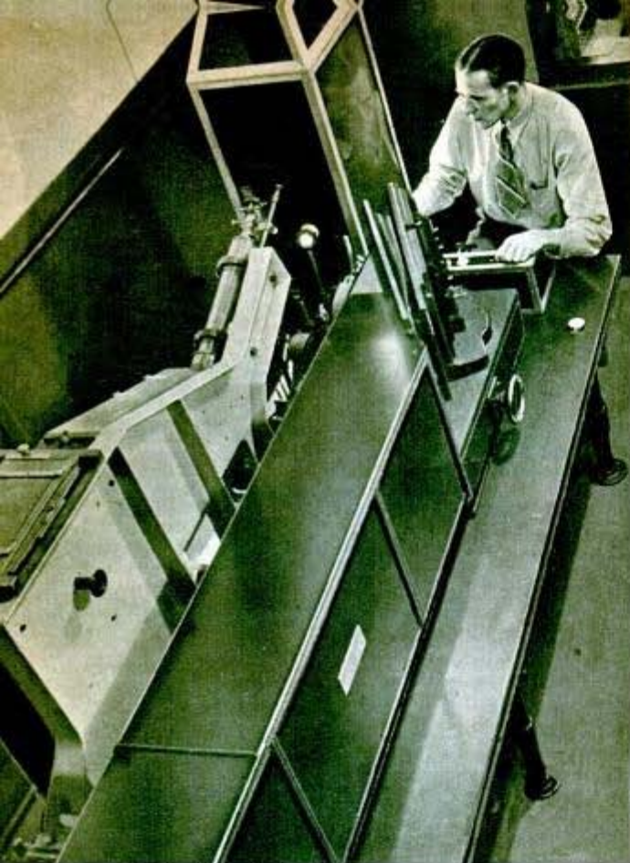
Westinghouse photo Spectrograph identifies elements of unknown materials on film which records light rays sorted by a prism
