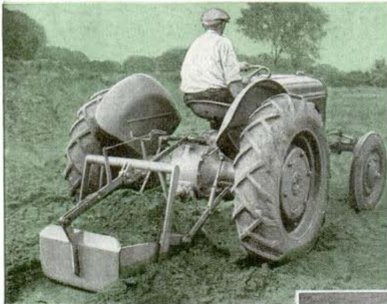
Ditch-digging scoop has hydraulic finger-tip control
