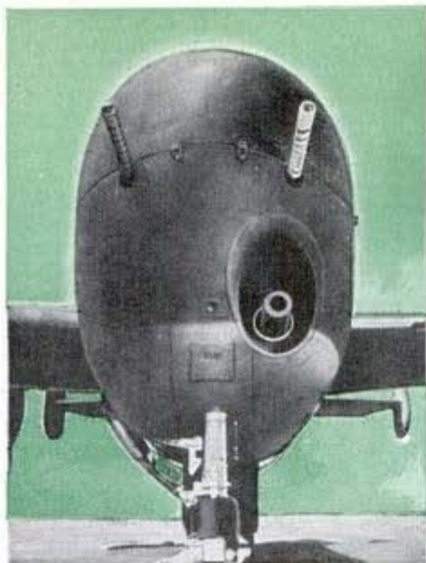
Above, "heavy artillery" on wings—a 75-millimeter gun in nose of a B-25 Mitchell. At right, machine guns and other weapons are test-fired to destruction in laboratory
