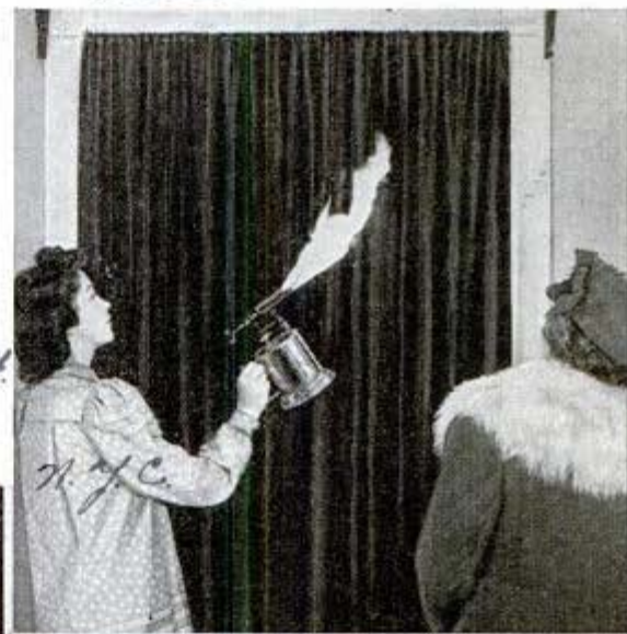
Fighting flames from explosion during test. Below, torch fails to ignite a fireproof blackout curtain Courtesy DuPont Company
