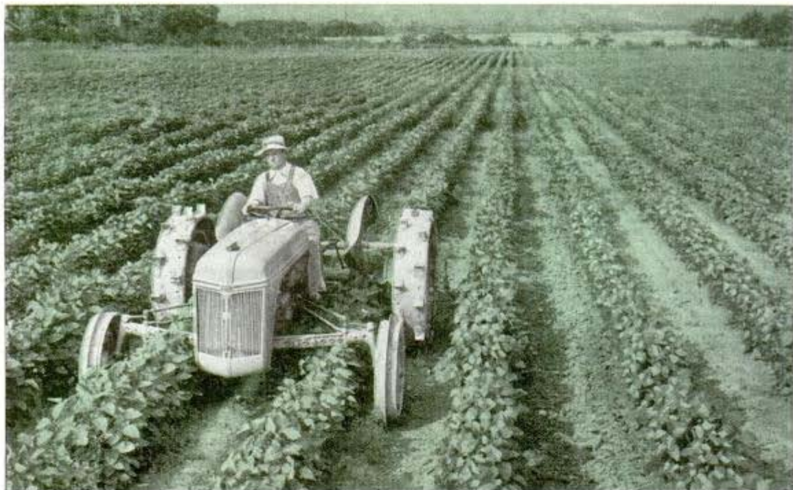
Width of soybean rows is no problem with Ferguson cultivator which has wheels that are easily extended
