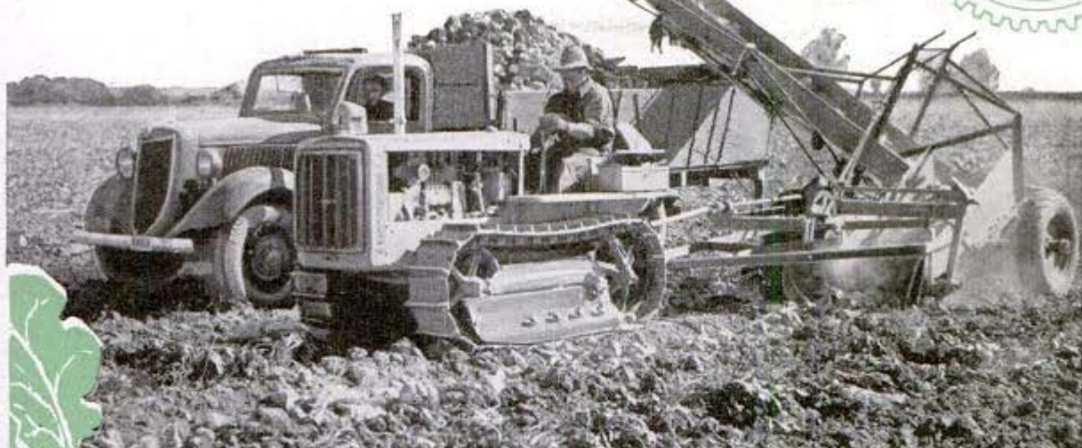
Courtesy Caterpillar Tractor Co. This beet loader can handle one ton of beets per minute
