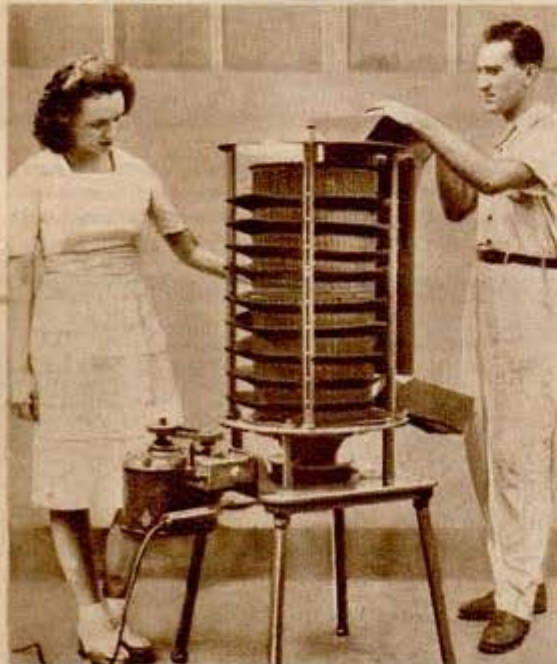
Berries fed into top hopper come out hulled below
