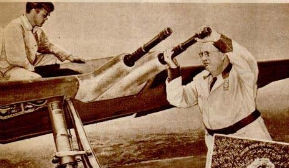
Left, installing 20-mm. cannon in Mustang's wing. Below, crescent of oil slick trails a Jap destroyer hit by Mitchell's bomb U. S. Army Air Forces photo
