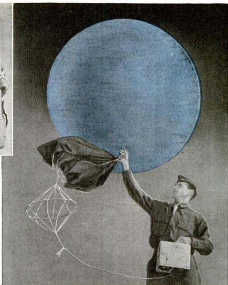
U. S. Army Air Forces photo Releasing radiosonde balloon which will transmit weather data by radio in box until balloon bursts and instrument descends by parachute. Below, barrage balloon carries anemometer to radio reports of wind speeds aloft
