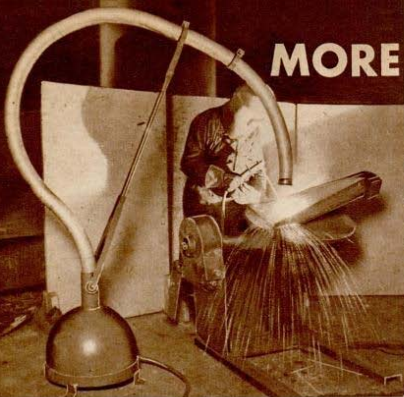
The "welding conditioner" at top sucks fumes away from welder's face. Below, safety styles for a girl riveter—headgear, mask, short sleeves and "hard" shoes Top photo, Lincoln Electric Co.; lower, National Safety Council
