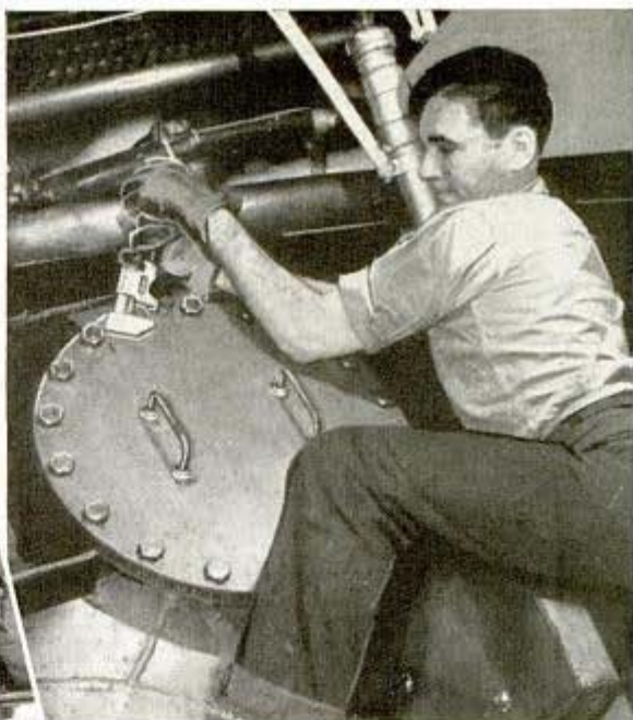
Above, tightening bolts of a condenser plate on ship disabled by enemy action. Left, tying down barrels in a Navy transport plane
