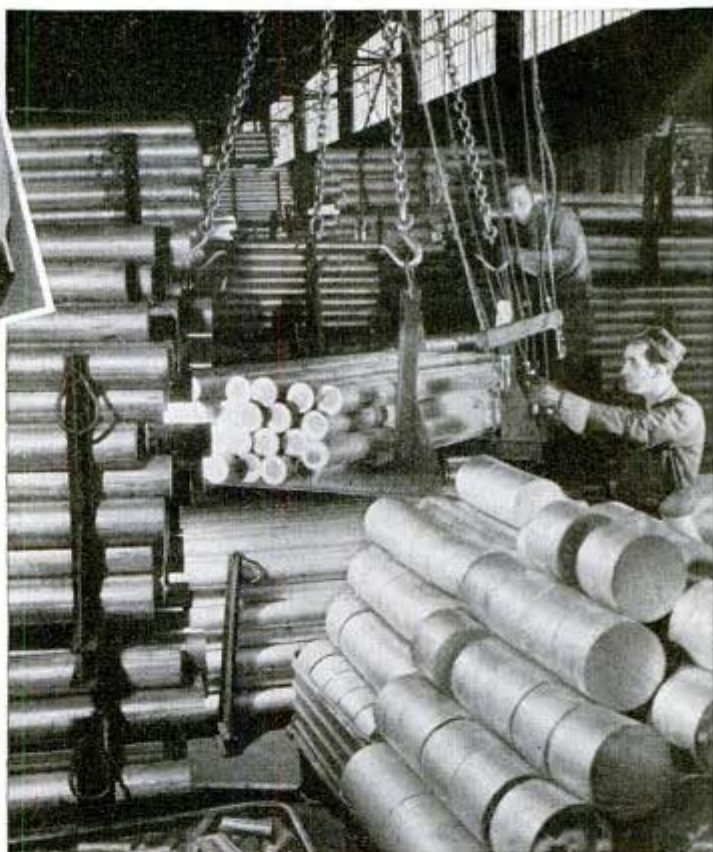
Above, a stock pile of aluminum alloy forging stock in an Aluminum Company of America plant. Below, inspecting marine speed reduction gears in Westinghouse gear-cutting works. It takes expert forging and machining to produce gears with 1/10,000-inch tolerance
