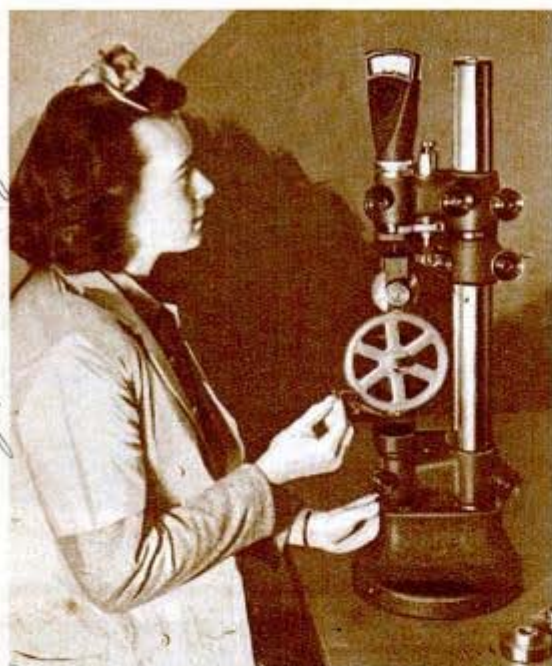
Portable tester shows any variation in gear teeth
