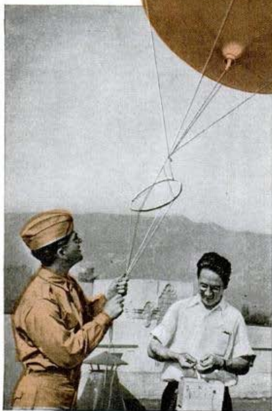
Adjusting the tiny radio transmitter of radiosonde balloon; at left is part of aerial weather station. Below, sending up captive balloon to calibrate weather instruments
