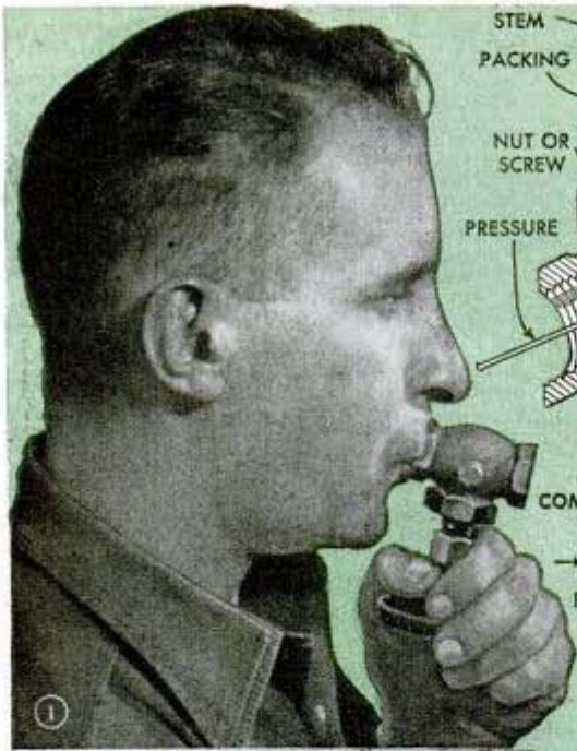
VALVES are usually globe compression type. Pressure end can be determined by blowing through valve as explained in text. Photos show simple repairs
