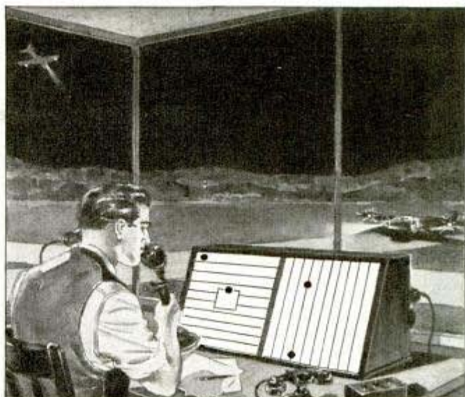
Proposed screens (above) would show horizontal and vertical position of planes near airport. Size and position of dots on cockpit screen below show proximity and position of other plane
