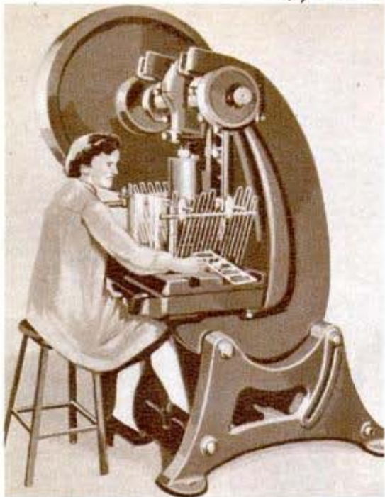
Staples of enclosure guard for press are adjustable
