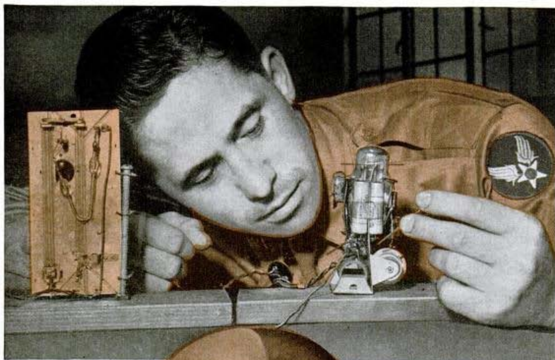
Adjusting the tiny radio transmitter of radiosonde balloon; at left is part of aerial weather station. Below, sending up captive balloon to calibrate weather instruments
