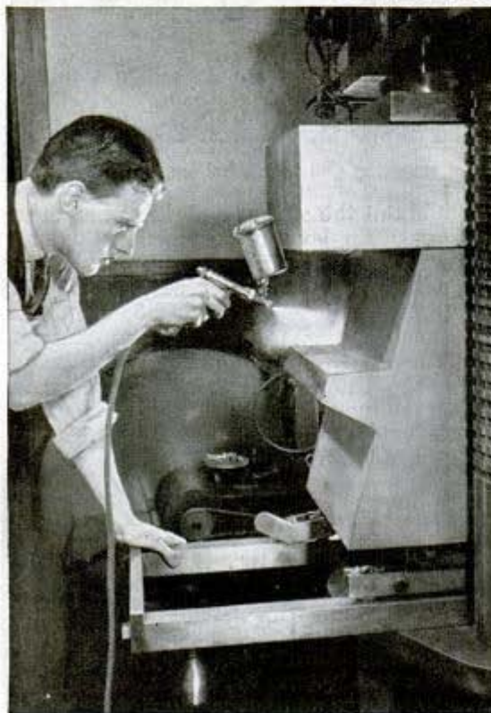
General Electric hammer with 1,600,000-pound wallop (top) forges one-ounce supercharger blade or 25-ton metal piece. Below, lacquer spray tests a forging Westinghouse photo
