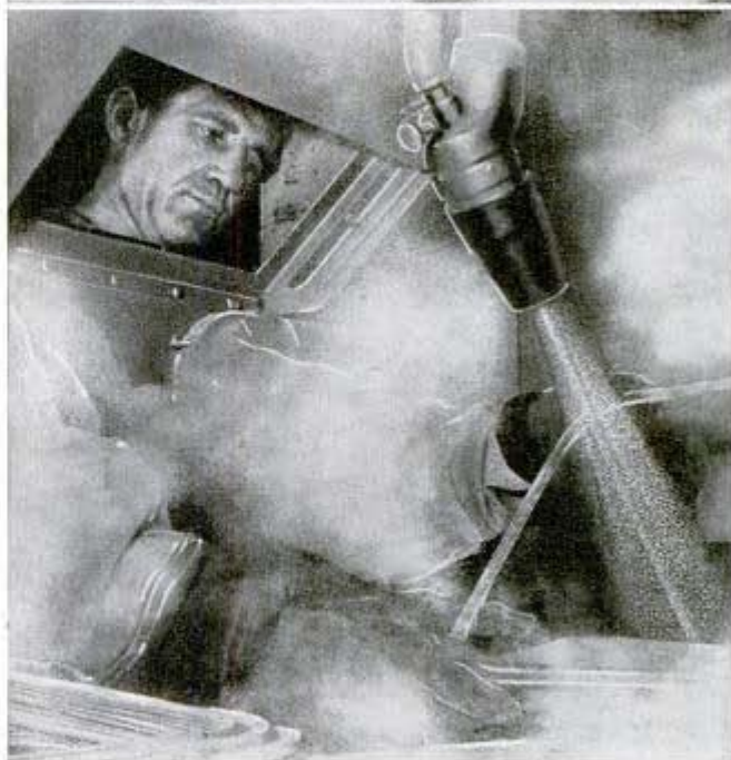
Helmeted like a diver, Boeing worker (top) cleans Flying Fortress engine mount. Below, window protects sandblaster at work
