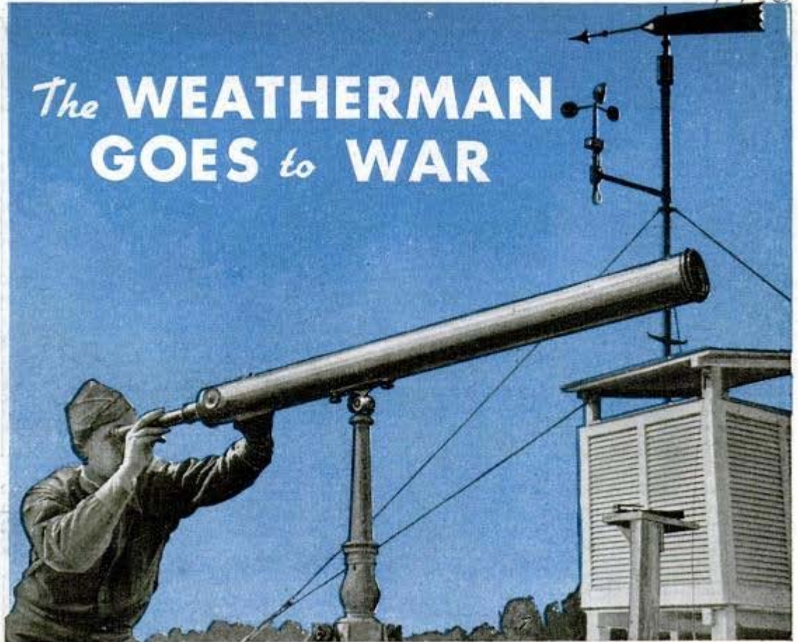
Through the telescope a meteorologist reads wind direction indicator on mountain top 10 miles away. Below, brushing the snow from a bomber before takeoff from a northern field
