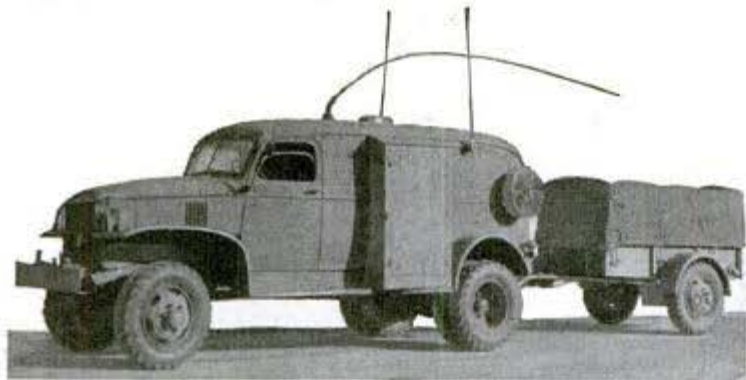
Mobile radio unit of Signal Corps used in city test to study interference of steel buildings and trolley wires. Below, control board of unit
