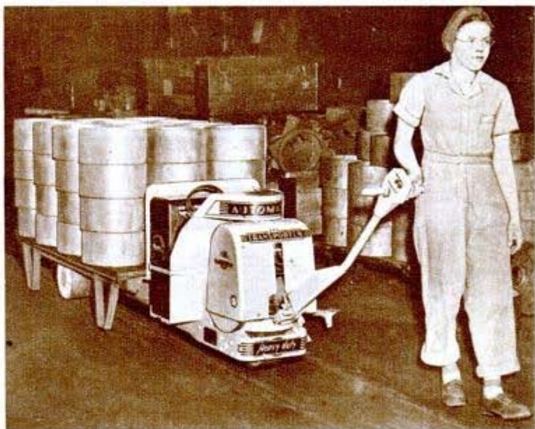
Battery-driven tractor does the work, controlled by pushbuttons on handle
