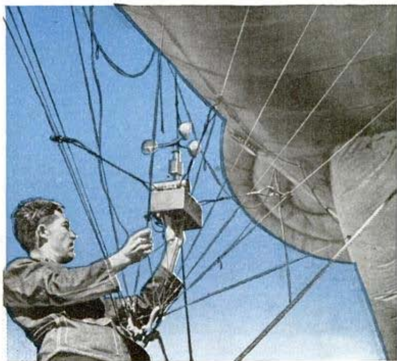
U. S. Army Air Forces photo Releasing radiosonde balloon which will transmit weather data by radio in box until balloon bursts and instrument descends by parachute. Below, barrage balloon carries anemometer to radio reports of wind speeds aloft
