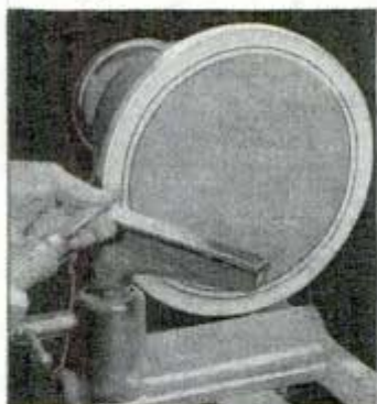
Fourth: Bowl bottom turned to fit recess in segment ring
