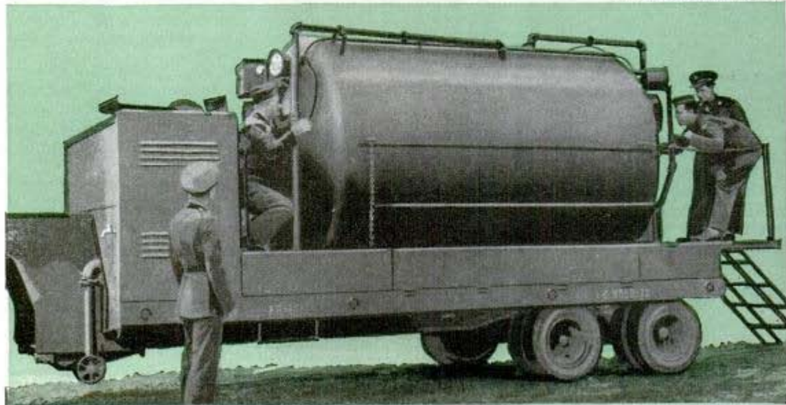
High altitude chamber mounted on trailer is taken to air fields to test substratosphere reactions of fliers
