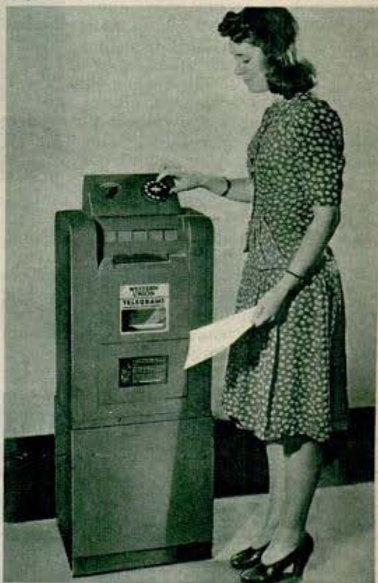
Dialing number puts both sending and receiving units in operation; then telegram is simply placed in slot
