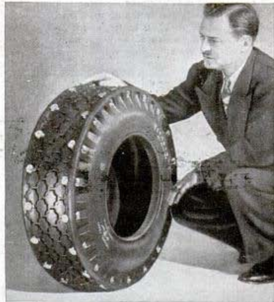
Non-skid lugs are bolted to shoulders of the tire
