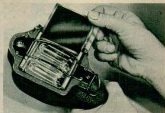
Prospector at left uses quartz-contained ultraviolet light in a hunt for a tungsten-bearing ore. Below is a closeup of the lamp. Light source is contained in the quartz tube; the dark filter allows only the ultraviolet to emerge.
