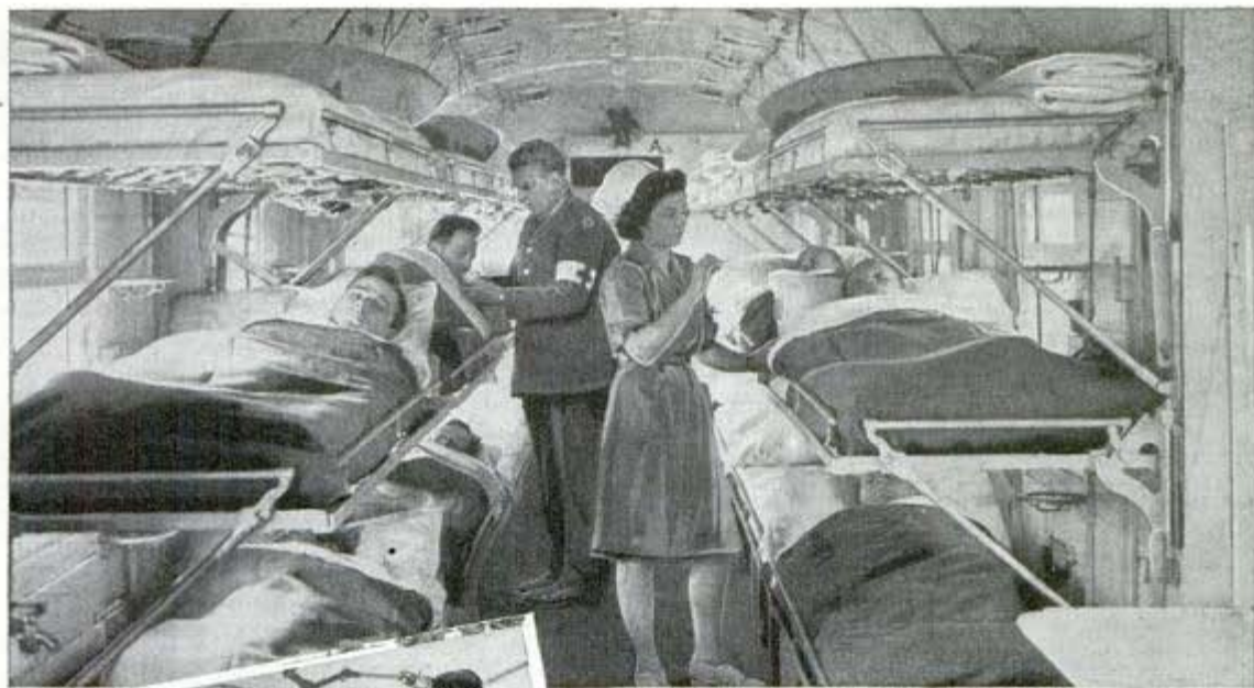
Built by the British and turned over to the Americans as an example of "reverse lend-lease," this hospital train is adaptable to any gage railroad in Britain, Africa or the continent, and built to pass through any tunnel, or over any bridge in the European war theater. Above is a view of one of the ward cars, showing the three-tiered bunks, 36 to a car. Below, lifting stretcher case aboard
