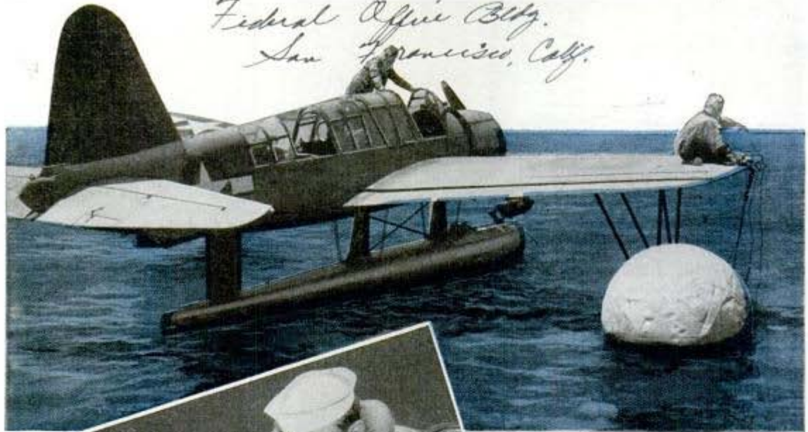
Wherever much over-water flying is done Navy crash boats stand by, at all times ready to speed to rescue of cracked-up plane's crew. Above, inflatable rubber sphere may be attached to prevent a plane's sinking. Left, lights used in night rescues. Below, man on deck is ready to toss line to occupants of disabled plane
