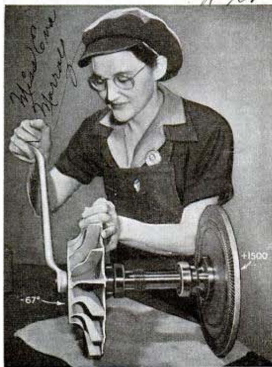
Tightening impeller that sucks frigid air into unit
