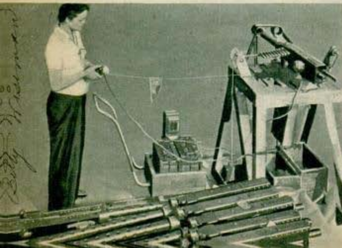
"Gun girl" below fires 10 rounds to test gun for a Mustang; switch she holds fires gun electrically
