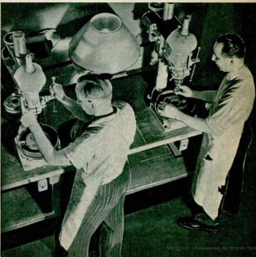
Above, steps in cutting oscillators, from natural crystal at left, rear, to square wafers in foreground. Chips in front are scrap. Below, lapping machines used in intermediate stage of grinding crystals
