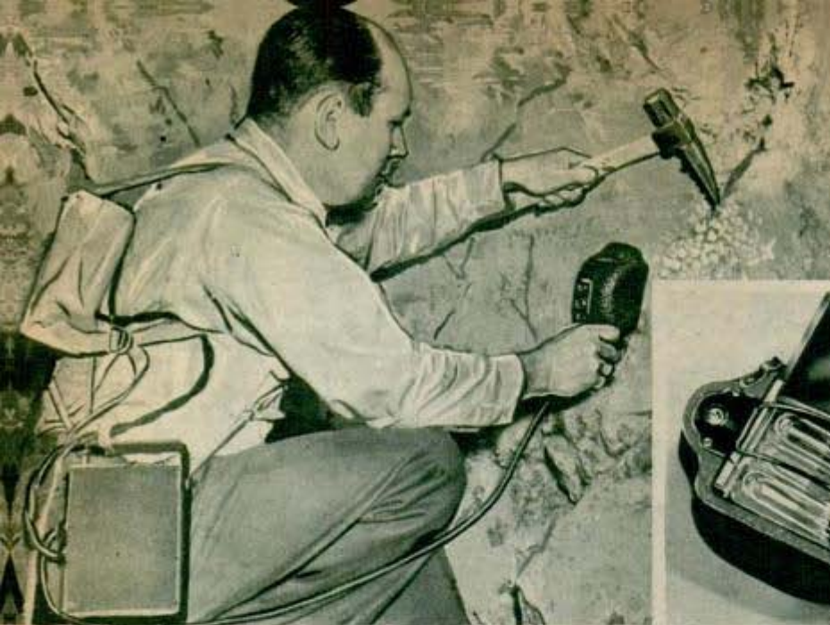
Prospector at left uses quartz-contained ultraviolet light in a hunt for a tungsten-bearing ore. Below is a closeup of the lamp. Light source is contained in the quartz tube; the dark filter allows only the ultraviolet to emerge.
