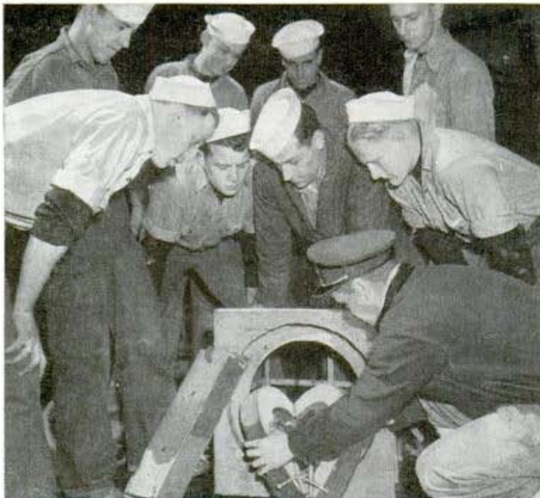
"Tooker patch" for sealing portholes is demonstrated to students, after which they will put on diving suits and go into the depths to operate one
