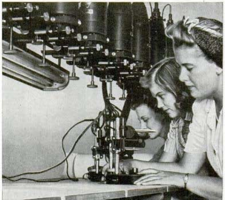
Projectors suspended above map sheet cast images of aerial photographs
