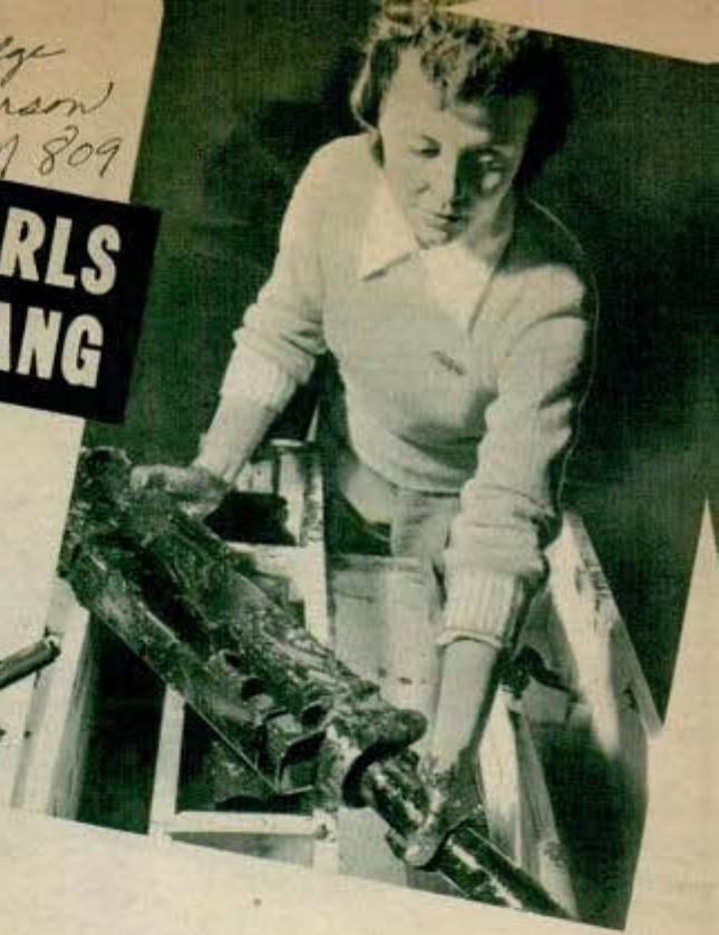
When the .50-caliber machine guns destined for turrets of Mitchell bombers and mounts of Mustang fighters arrive at North American's plane plant, "gun girls" take them from their packing of heavy grease (above), clean them, reassemble their 219 different parts, check them for timing, charging and mounting, and even test-fire them. To test twin-gun turret's ejectors (left) a belt of dummy bullets is fed through. Turret below checks o.k.
