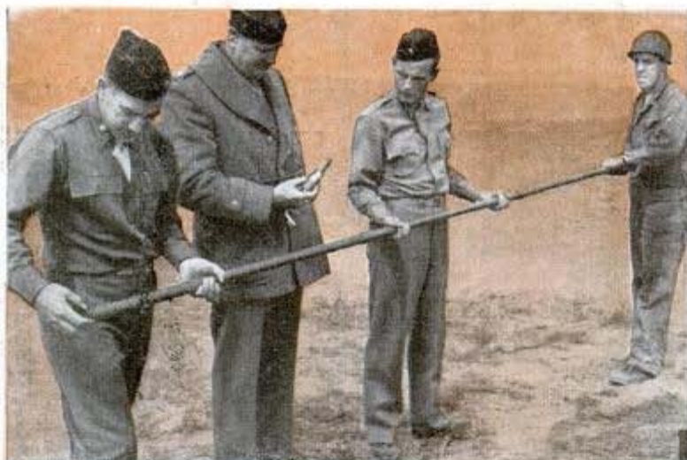
Jap Bangalore torpedo is made of 1½-inch pipe sections filled with TNT
