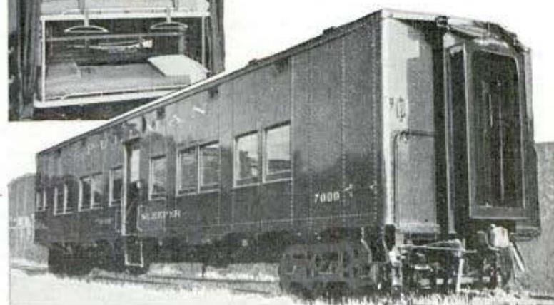
Built specially for transporting troops, this all-steel Pullman car may reduce travel rates after the war. View at top shows berth arrangement
