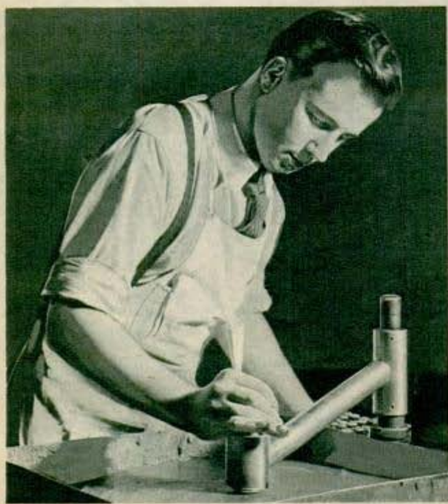
This is one stage in grinding flat parallel surfaces on a quartz-crystal wafer.
