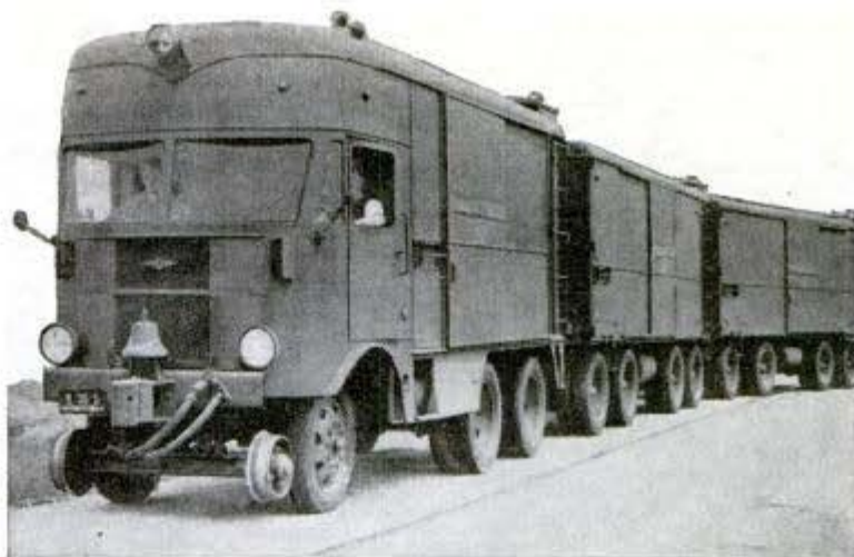
Here the rail train of the opposite page leaves the rails for the highway
