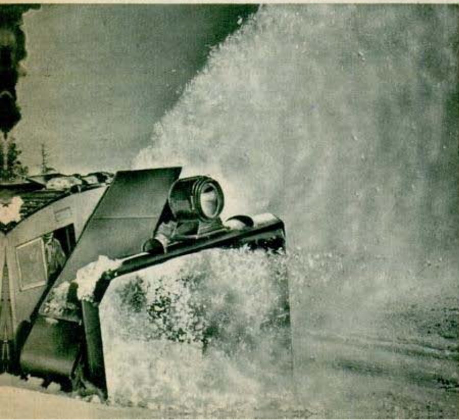
A railway rotary plow bites into a fresh snowbank on the line
