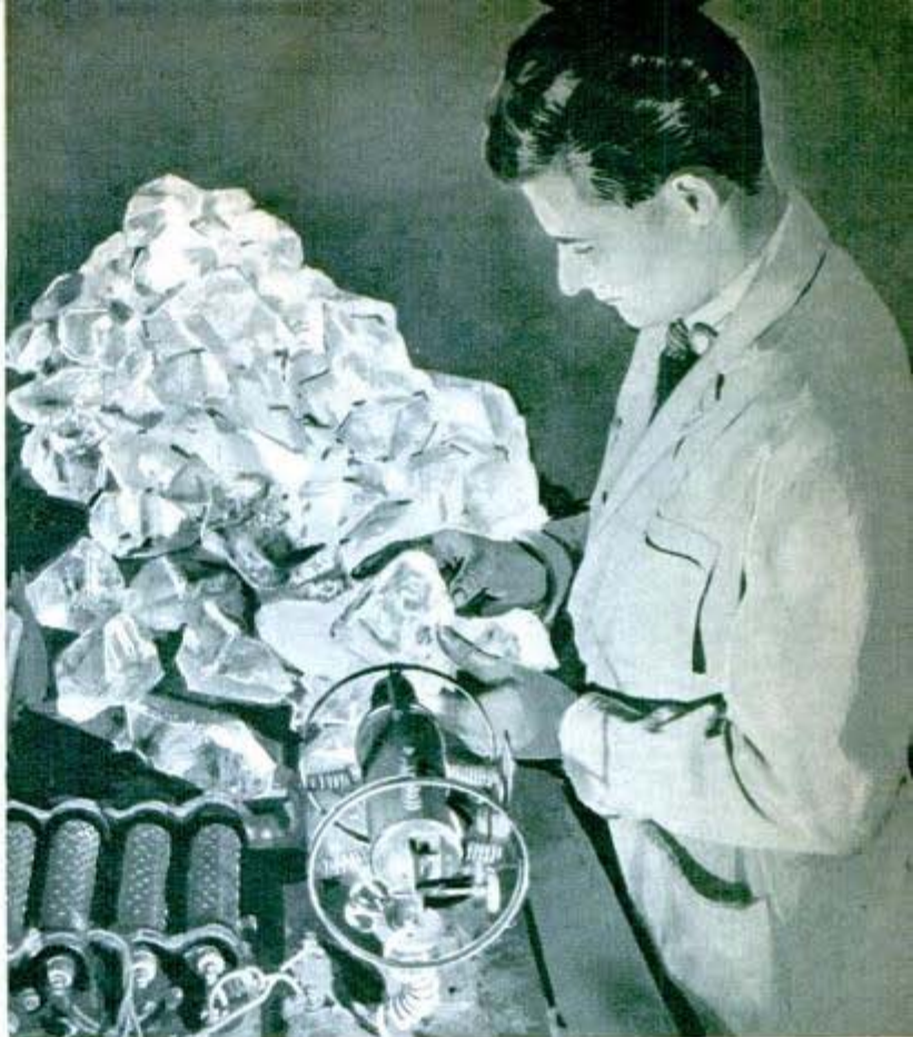
Inspecting quartz crystals from Brazil under an arc light
