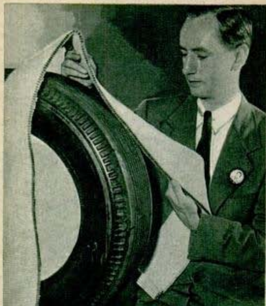
Carpeted retread for worn tires uses thin rubber layer
