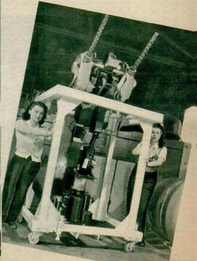
"Gun girl" below fires 10 rounds to test gun for a Mustang; switch she holds fires gun electrically
