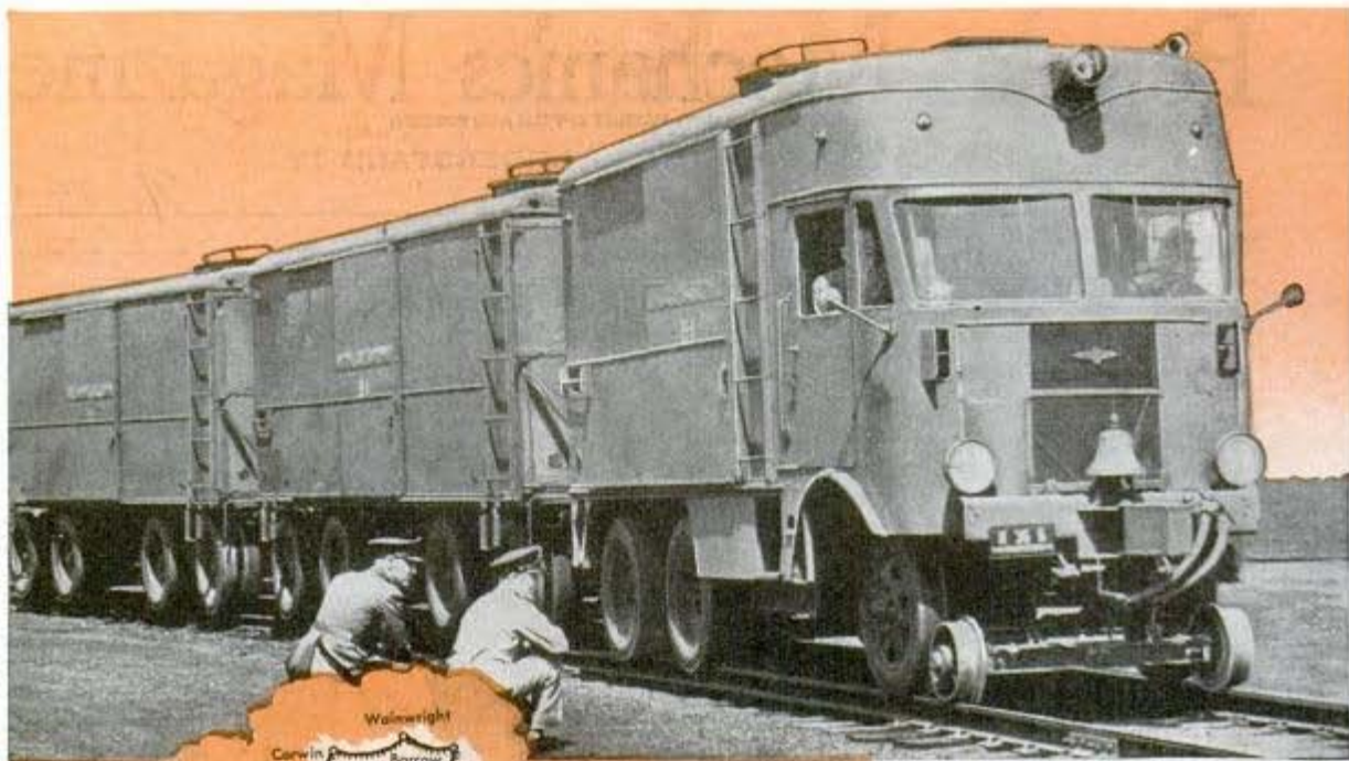
With steel pilot wheels lowered, the pneumatic tires of the auto-rail freighter ride on the rails
