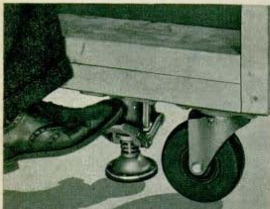
Touch of the foot locks or releases floor truck brake
