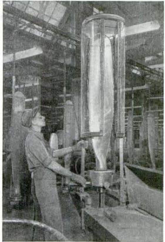
Shield keeps air from swaying balanced "prop" blade
