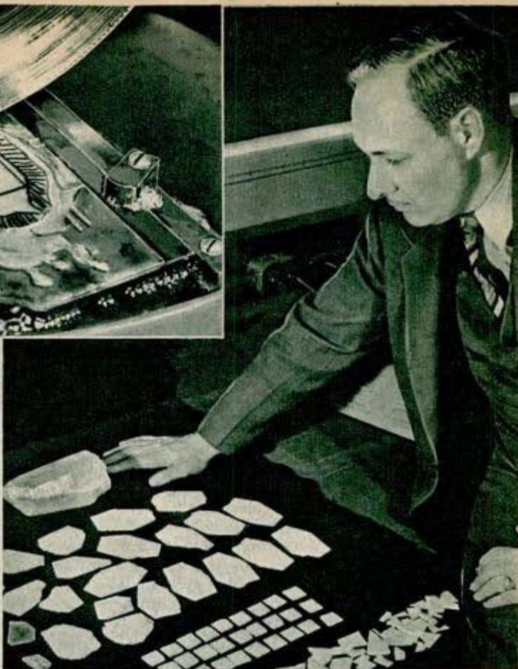
Above, steps in cutting oscillators, from natural crystal at left, rear, to square wafers in foreground. Chips in front are scrap. Below, lapping machines used in intermediate stage of grinding crystals
