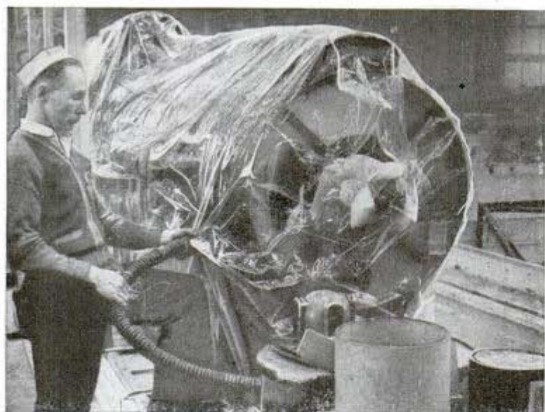
Removing air from the Pliofilm bag helps protect parts
