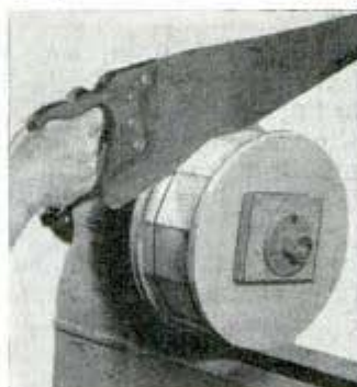
Sixth: Work is cut through with saw while on faceplate, lathe being turned off
