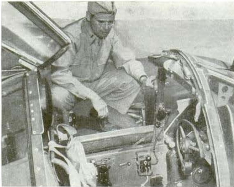
Ordnance officer inspecting gun controls in P-38 cockpit. Button on arm of wheel fires 20-mm. cannon; button on back of wheel fires machine guns
