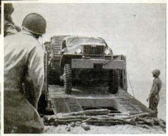
Assault boats used by the engineers lead a versatile existence. Above, a platform is laid across a pair of them to form a light ferry capable of carrying peep. The impromptu ferryboat is paddled across the river Signal Corps photos
