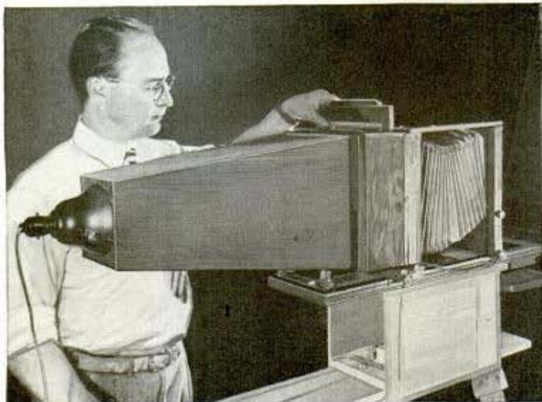
Ordinary "8x10" is converted into an enlarger with homemade lamp house
