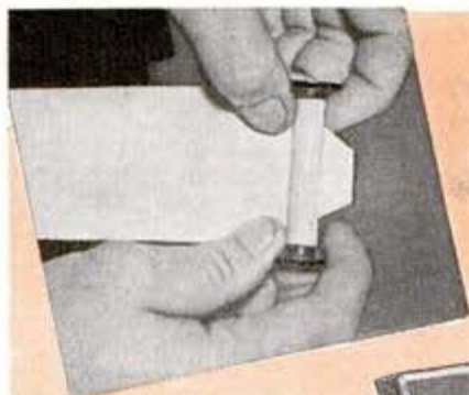
Above, inserting paper into film spool, emulsion side in. Below, load paper negative in darkness or by safelight
