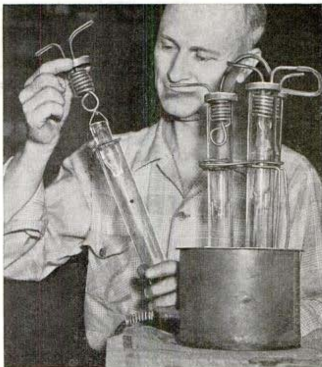
Distillation apparatus to extract oils from tissue of plants
