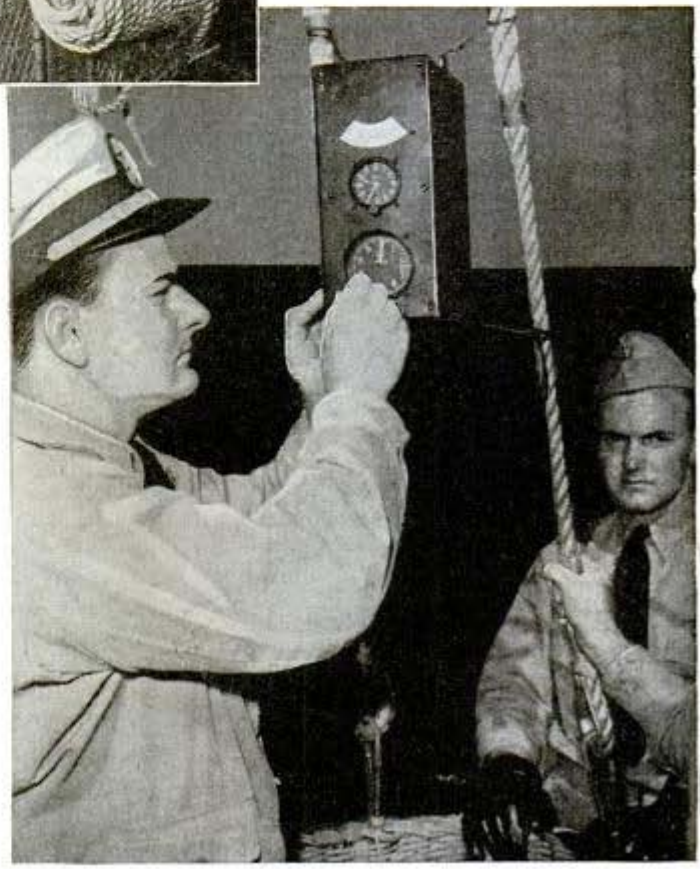
Basket of free balloon at Moffett Field gets change of crew. Below, instrument box for navigation boasts altimeter, clock
