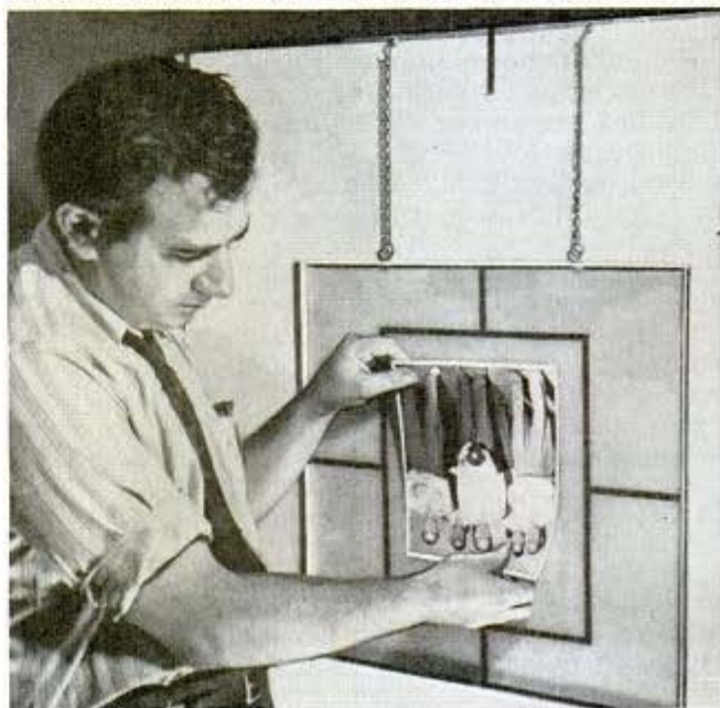
Homebuilt paper holder for enlarging or copying made of shallow tray with tacky surface of hardened hectograph compound
