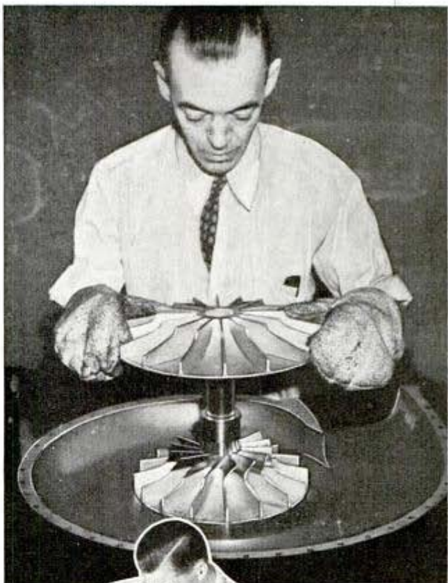
Above, fitting heated units of supercharger to shaft; left, adjusting the supercharger
