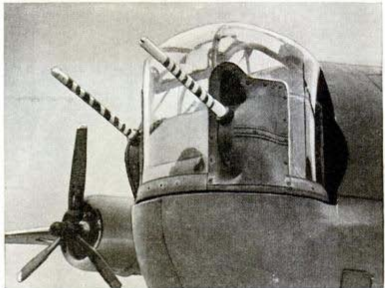
Liberator's nose turret can fire 26 projectiles a second from twin guns
