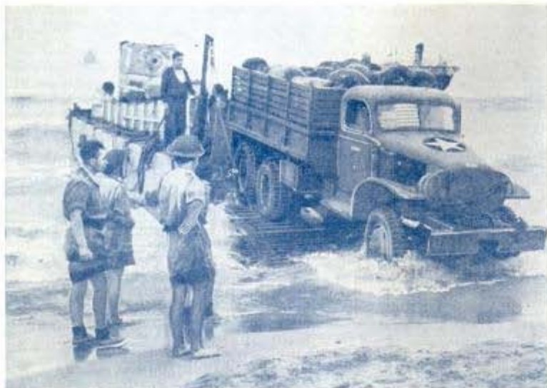
An "LCM" craft puts ashore a 10-wheel cargo truck on an African beach
