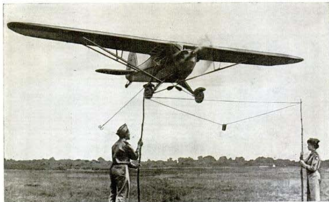
Pilot lowering hook to pick up a message on the fly—a handy trick in districts observing radio silence
