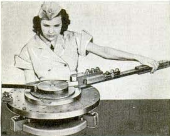
Bender cold-forms metals without danger of fracture
