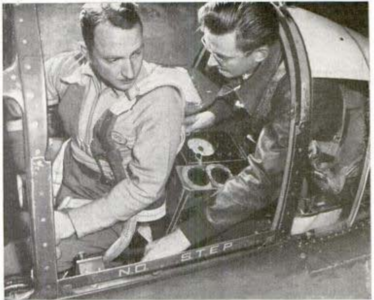
Student pilot gets a "piggy-back" ride in one-man P-38. The students are squeezed in for demonstration flights on the plane's radio shelf
