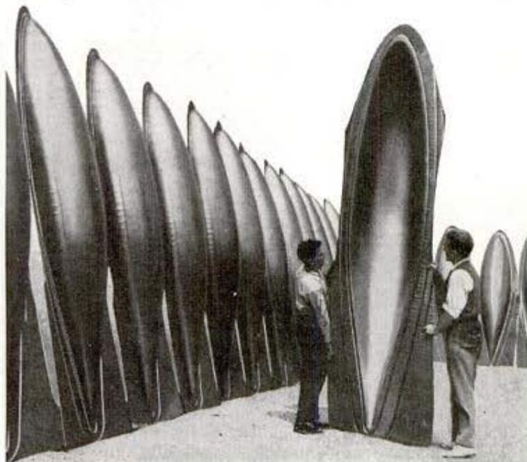
These pressed metal shells will be joined to form auxiliary gas tanks for the long range P-38s
