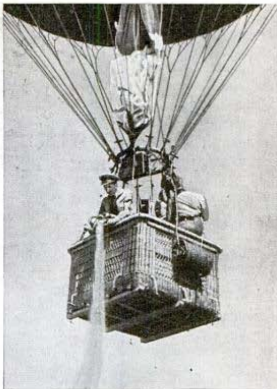
Spilling sand ballast over the side to speed ascent of balloon. Below, landing in field as blimp watches
