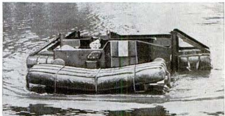
Kapok pads keep Bren gun carrier afloat, while tracks are used to steer
