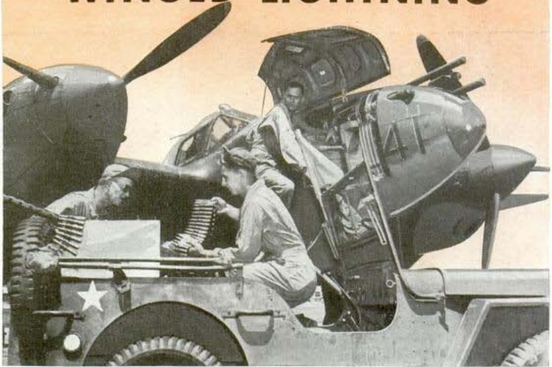
Ordnance crew servicing P-38's nose artillery—four .50-caliber machine guns and one cannon
