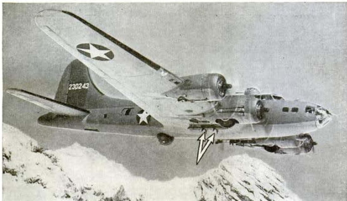
Arrows point to one of the two external bomb racks mounted beneath wing of Fortress, increasing bomb load
