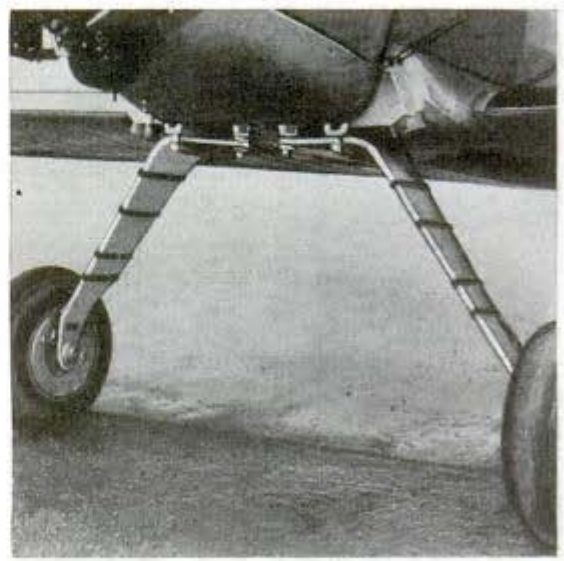
Strut spreads out to cushion the shock of landing
