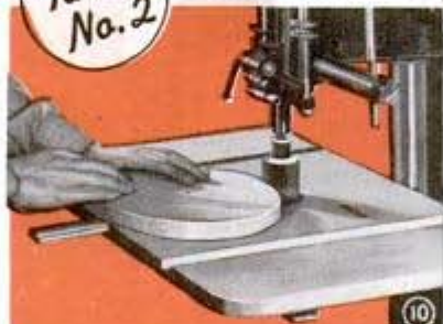
SANDING OR SHAPING CIRCULAR WORK
