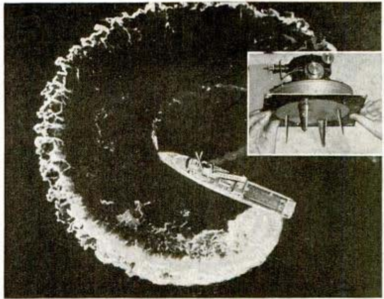
Wake shows extreme maneuverability of ship with propeller-rudder in inset
