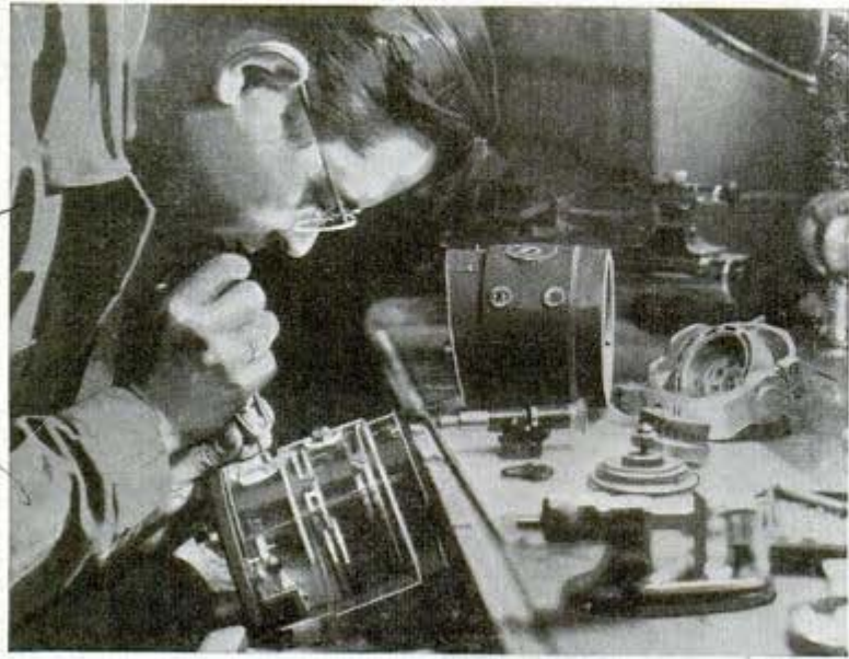
Transparent plastic and condemned plane parts make visual study aids for aviation cadets. Above, mockup of hydraulic system of advanced trainer. Below, duplicating instrument housing in Plexiglas; workings are visible
