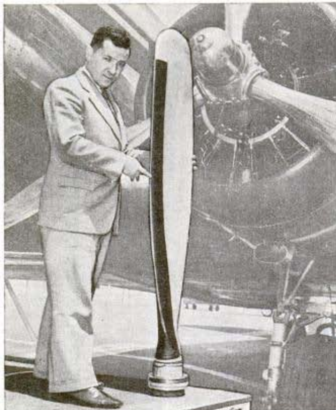
Rubber strip on edge of blade carries warming electric current
