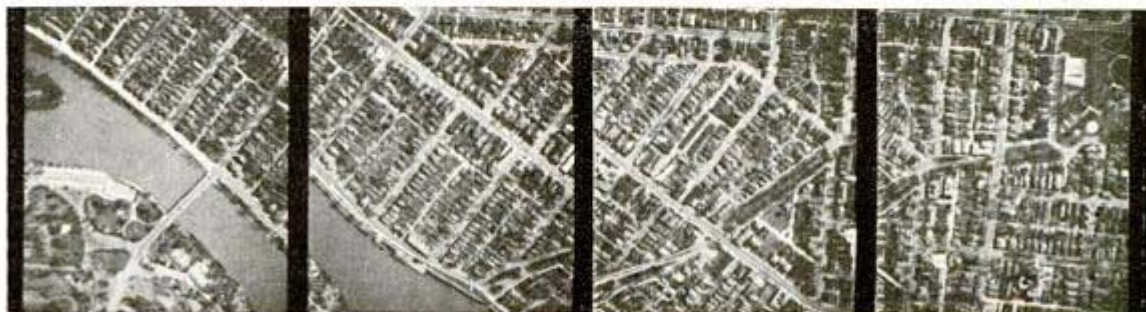
Above is the sectional type of picture formerly standard; below, the new continuous-strip photograph
