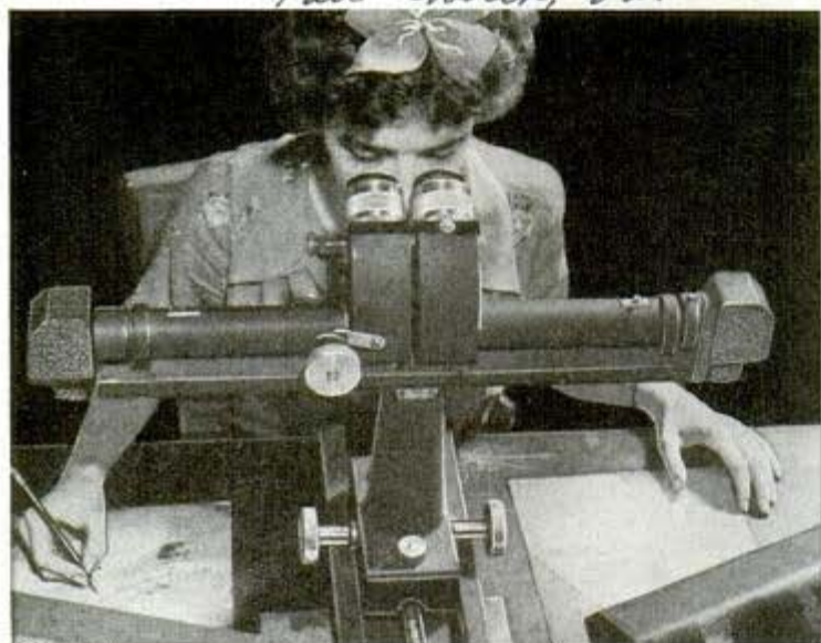
OWI photo Making a magnified stereoscopic examination of Army Air Force photos to select topographical data which will be applied to the base map
