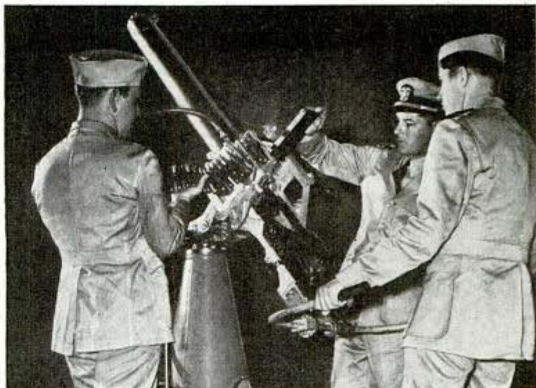
Cadets above are learning to load belts of .50-caliber bullets into an anti-aircraft machine gun. They must be able to handle the gun blindfolded
