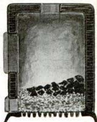
22 SHALLOW FIRE WASTES FUEL AND HEAT
