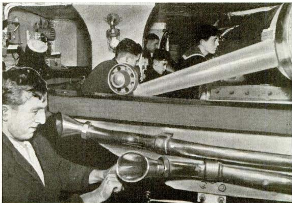
Inside the gun-house of the main turret on a battlewagon, the guns (above) are loaded and trained on the target, the order "broadside" has been received. Men wait for the sound of the fire gong, their signal to turn the firing switch that sends the shells on their way. Below, in the rear of the gun-house, gun captains transmit orders through speaking tube to gun layers. Sailor, right, uses eyepiece of a big range finder
