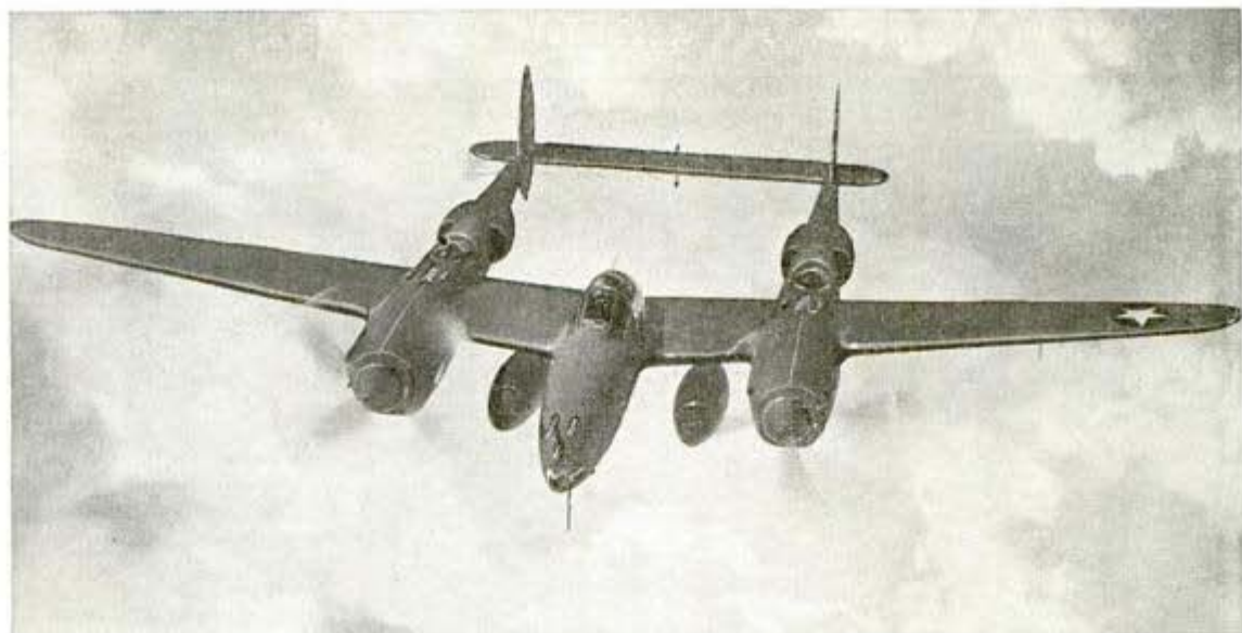
This Lightning interceptor carries auxiliary fuel tanks which it will drop before going into combat
