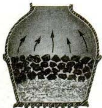
18 SMALLER LUMP SIZES ADMIT LESS AIR, BURN MORE EFFICIENTLY; APPLIES TO ANTHRACITE COAL AND COKE
