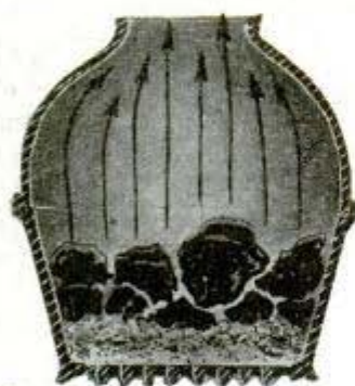
17 LARGE LUMP FUEL RESULTS IN EXCESSIVE HEAT LOSS
