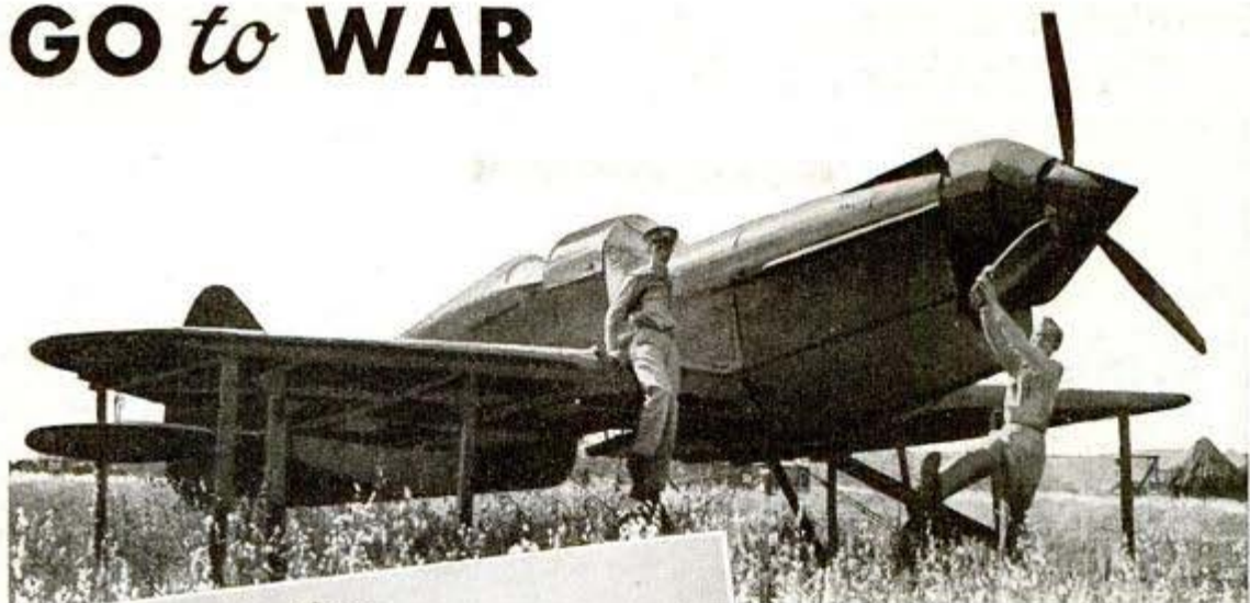
From the air the fighter plane (above) looks like a real P-40 parked alongside an advance landing strip. It is made from scrap wood and sheet metal
