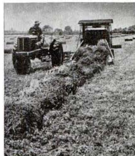
Operating by power takeoff from tractor, baler rolls up hay like carpet
