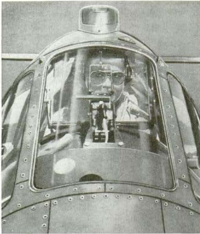
Squinting into the square of glass set at an angle, the P-38 pilot sights his weapons by reflection of his electric gunsight
