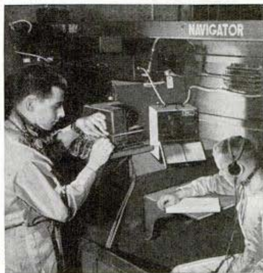
"Semi-mockup" is what students call plywood replicas of bombers in which radio equipment is placed exactly as in real planes. They are used to teach radio men. Above, general view of a mockup. Note name places for crewmen. Right, "navigator" in his position
