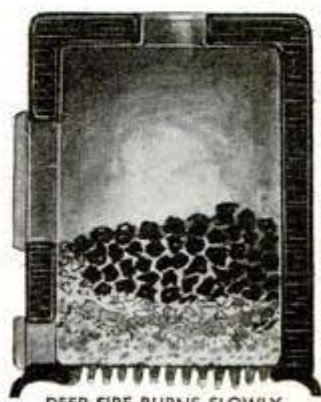
23 DEEP FIRE BURNS SLOWLY, CONSERVES HEAT AND COAL. APPLIES TO HARD AND SOFT FUELS
