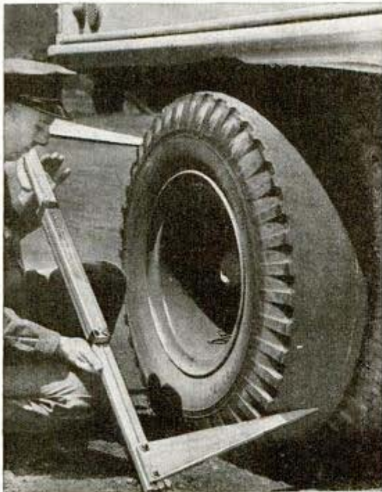
Measuring dual tires on truck without removing them from wheels. Matched tires eliminate wasteful drag
