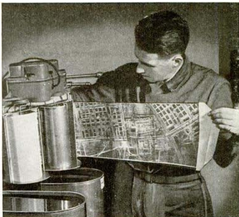
The continuous strip printer above, developed at Wright Field laboratory, is portable and can be used at advanced bases for rapid printing of aerial photos. Below, loading photoflash bombs for reconnaissance flight
