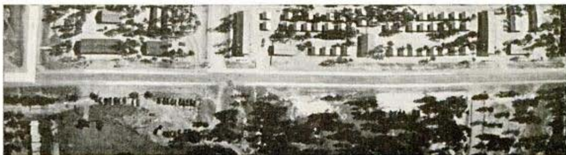
Above is the sectional type of picture formerly standard; below, the new continuous-strip photograph
